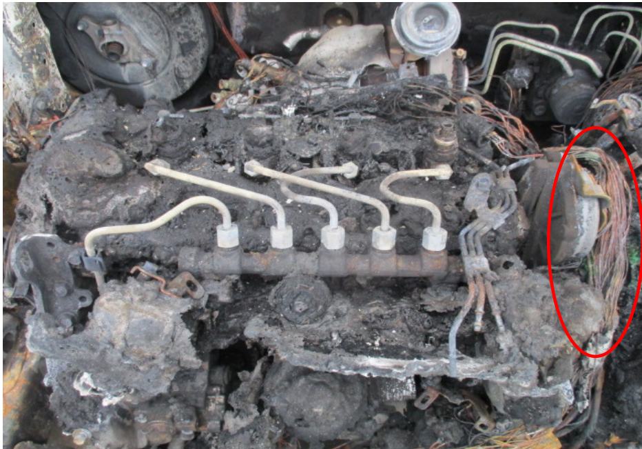
Photo 9 shows the original factory fitted wirings around the centre right portion of the engine compartment, which is in the immediate vicinity where the fire to the Insured Vehicle had likely started. We had found greenish residue on several burnt stretches of these wirings (circled). The presence of such greenish residue indicates internal heating of copper wires, a sign of an electrical short circuit occurring. The greenish residue is normally left behind from oxidation as a result of chemical reaction involving the copper wires.
