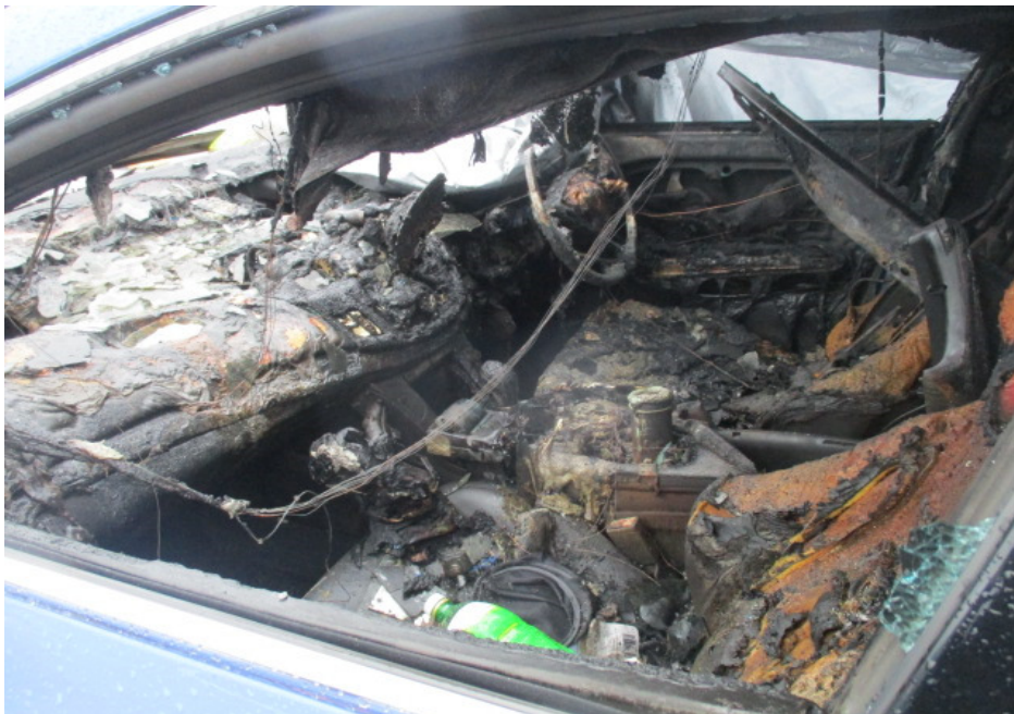
Photo 6 shows the interior compartment of the Insured Vehicle, which was significantly affected by the fire.
