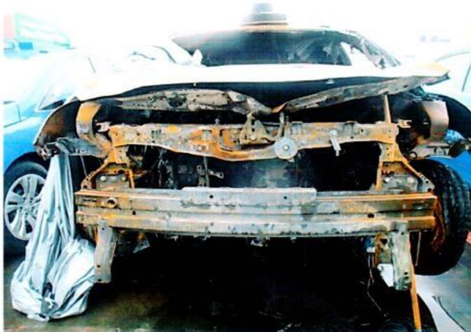
Photo 3 shows the closer view of the front portion of the Insured Vehicle at the time of our inspection. The fire damage to the Insured Vehicle was confined to its front portion. Its front bumper, front bonnet, front support panel, front tyres and front headlamps were amongst the body parts that were found to have been affected by the fire.
