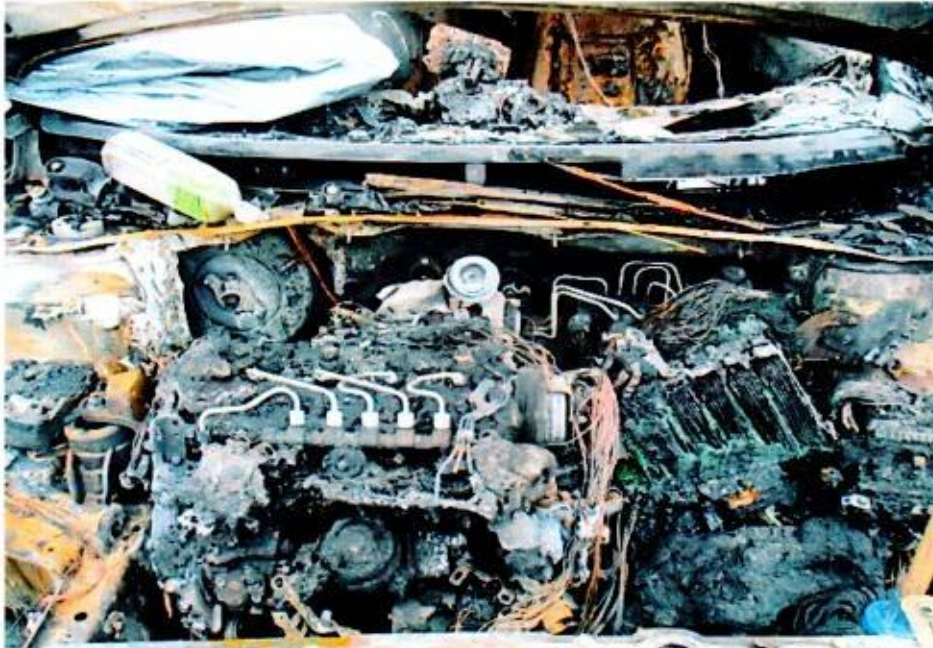
Photo 5 shows the engine compartment of the Insured Vehicle at the time of our inspection. The entire engine compartment of the Insured Vehicle was observed to be severely burnt. Most of the parts inside the engine compartment were found to be burnt and/or melted as a result of the fire.
