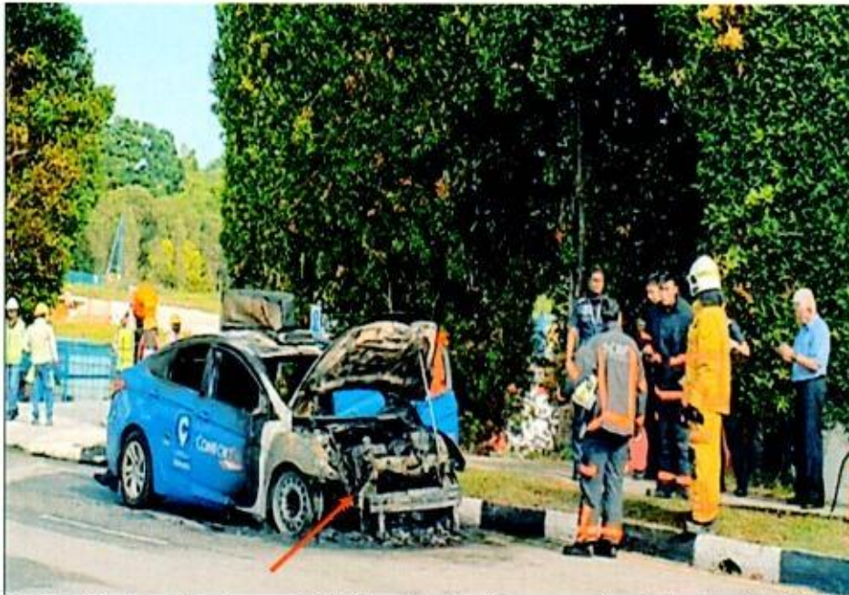
Photo 13 shows the Insured Vehicle after the fire was extinguished by the SCDF. In general, the information that could be gathered from this photograph had corresponded to the events that were related to us by Mr Ho, which is the fire had started from the engine compartment (arrowed).
