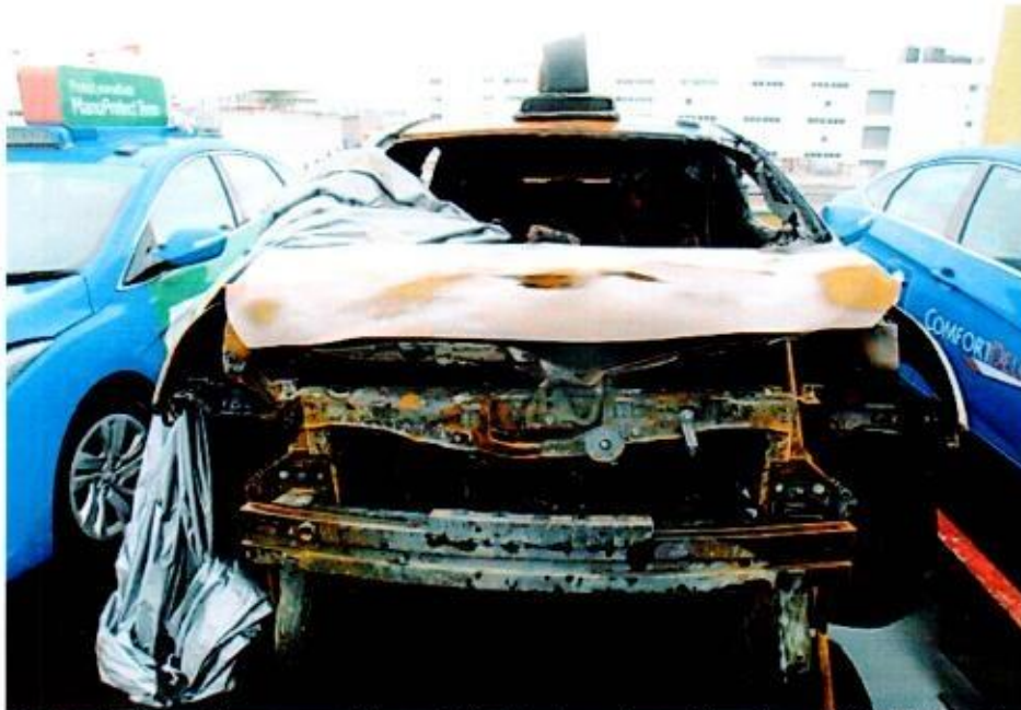
Photo 2 shows the general view of the front portion of the Insured Vehicle at the time of our inspection. The fire damage to the Insured Vehicle was confined to its front portion. Its front bumper, front bonnet, front support panel, front grille, front headlamps, front windscreen, front rims and front tyres were amongst the body parts that were found to have been affected as a result of the fire.
