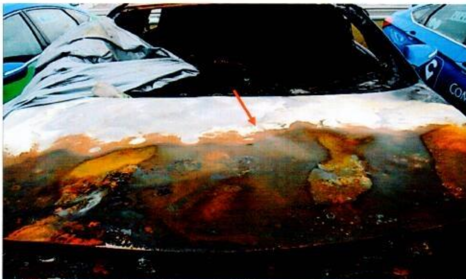
Photo 7 shows the burn pattern and whitish burn marks that were found on the rear portion of the front bonnet of the Insured Vehicle (arrowed). Such whitish burn marks are a result of exposure to prolonged heat intensity, which may indicate where the fire had started. Rust would also begin to develop on these areas soon after the fire.
