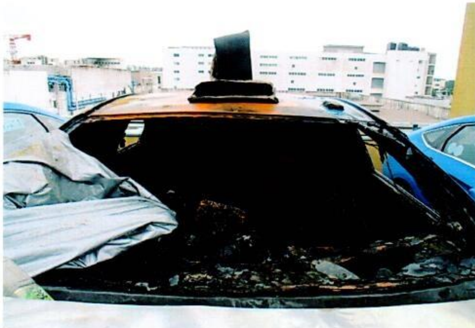
Photo 4 shows the general view of the front windscreen of the Insured Vehicle at the time of our inspection. The fire damage to the windscreen was extensive.
