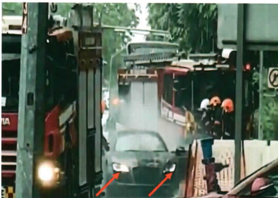
Photo 21 shows the Insured Vehicle at the incident location after the fire was extinguished by SCDF personnel. Firefighters can be seen to be extinguishing the fire and inspecting the extent of damage. The day lights (arrowed) were still lighted up after the fire was extinguished.
