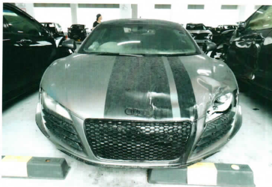
Photo 4 shows the general view of the front portion of the Insured Vehicle, it was unaffected by the fire however its front bonnet and front left headlamp was damaged by a collision accident which was prior to the fire incident.
