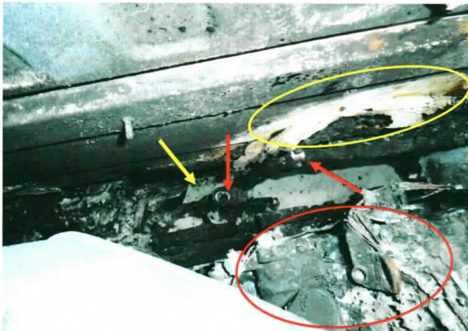
Photo 16 shows the close up view area where the fire had likely started and spread around the engine compartment. Observed was a broken fuel hose (red arrow) which caused a fuel leakage onto and around the hot surface of the running engine components which was likely the caused of fire and left over greenish fuel additives residue (red circle) around the area and on the floor (yellow arrow). The fire's high heat intensity burn had also resulted in (whitish burn marks) on the body panel (yellow circle) of the Insured Vehicle.
