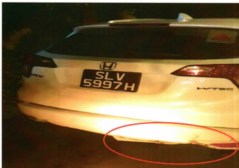
Photo 17 shows collision damage at the rear right bumper on the third party vehicle, which is consistent to the damage sustained on the front left portion of Mr. Brendan's Insured Vehicle.
