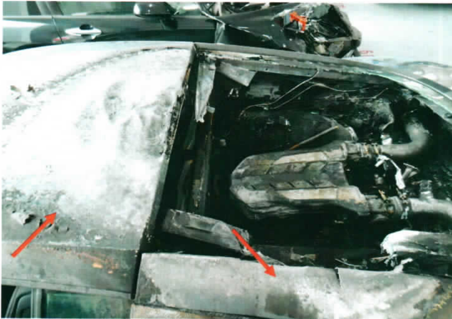
Photo 13 shows the roof and the surrounding of the middle portion (arrowed) of the Insured Vehicle at the time of our inspection. The high heat intensity burn marks (whitish burn marks) and rust that had development found on the exterior surface of the roof metal body and the surrounding area indicates that the fire had originated from the engine compartment of the Insured Vehicle.
