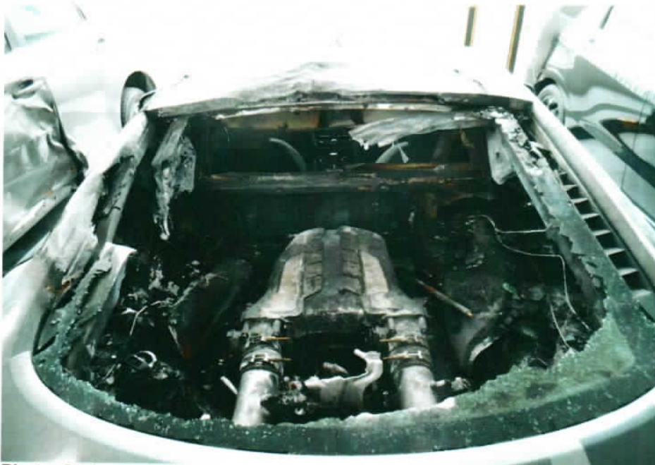
Photo 6 shows the general view of the engine compartment of the Insured Vehicle at the time of our inspection. The Insured Vehicle was observed to have sustained severe fire damage. Its engine cover and engine compartment was completely burnt. Rust had accumulated around the engine compartment of the Insured Vehicle as a result of exposure to environmental condition for a period of time.
