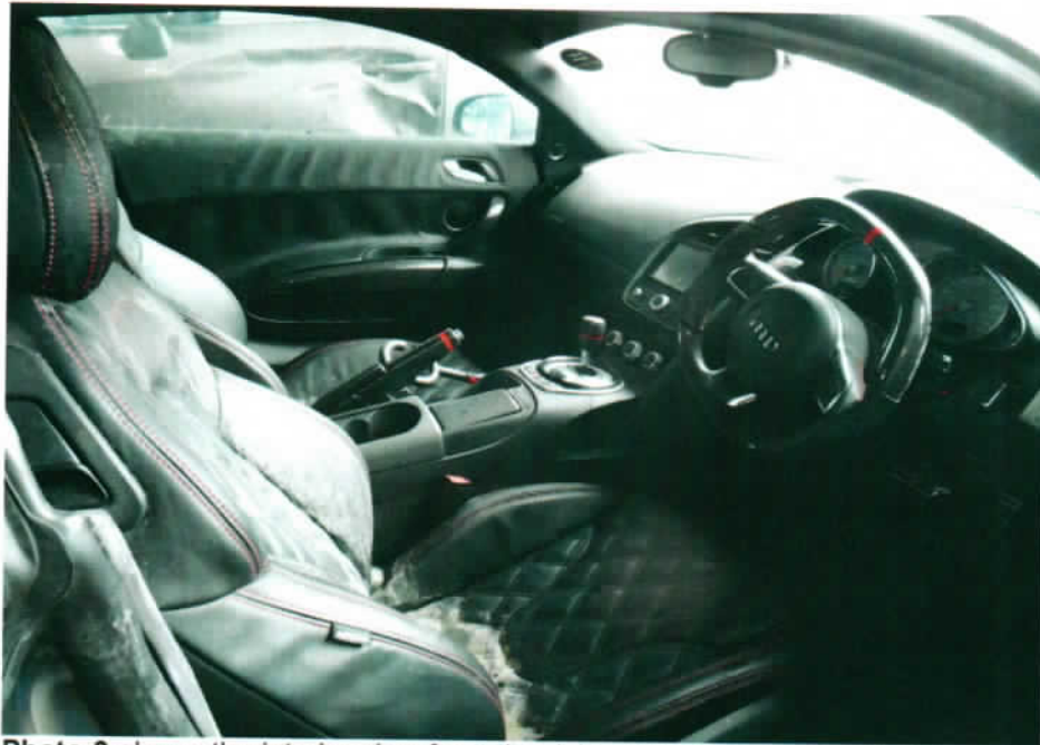
Photo 9 shows the interior view from the right side of the Insured Vehicle at the time of our inspection. The interior fittings of the Insured Vehicle were observed to suffer smoke and heat damage as a result of the fire.
