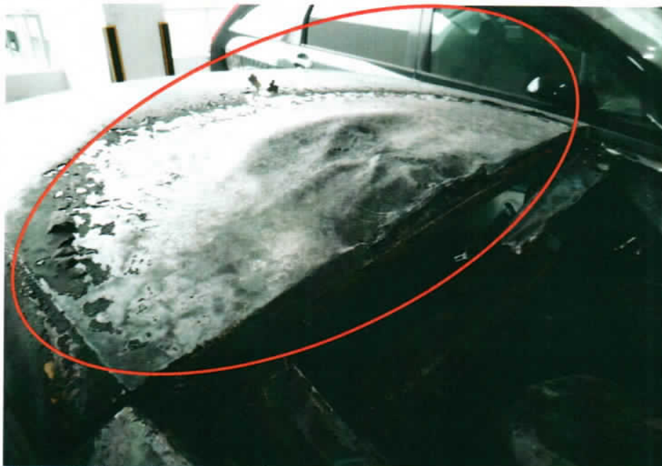
Photo 14 shows the roof and the surrounding of the middle portion (circled) of the Insured Vehicle at the time of our inspection. The high heat intensity burn marks (whitish burn marks) and rust that had development found on the exterior surface of the roof metal body and the surrounding area indicates that the fire had originated from the engine compartment of the Insured Vehicle.
