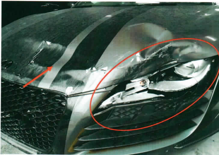
Photo 5 shows the front portion of the Insured Vehicle it was unaffected by the fire however its front bonnet (arrowed) and front left headlamp (circled) was damaged by a collision accident which was prior to the fire incident. (Refer to photo 17-19 below)
