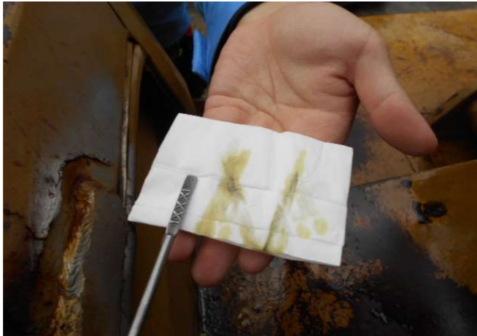
Photo 15 shows the ATF transmission fluid dip stick of the Komatsu Forklift at the time of my inspection. The observed was differential gear oil (yellow colour) instead of the supposed ATF transmission fluid (pink colour) which was the wrong type of fluid used.
