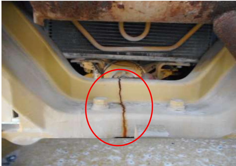
Photo 4 shows a rear view of the Komatsu Forklift's at the time of my inspection. Its rear frame (circled) was amongst the body parts that were damaged as a result of the accident.
