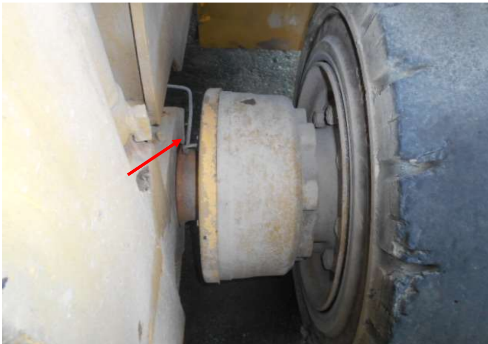
Photo 19 shows the brake hose/pipe (arrowed) at the front left wheel of the Mitsubishi Forklift. I did not observe any leakage of brake fluid at the time of my inspection of the Mitsubishi Forklift.
