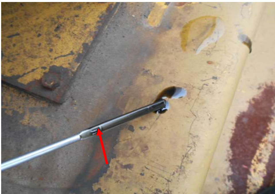
Photo 14 shows the engine oil dip stick of the Komatsu Forklift at the time of my inspection. The engine oil was observed to be of sufficient level (arrowed)
