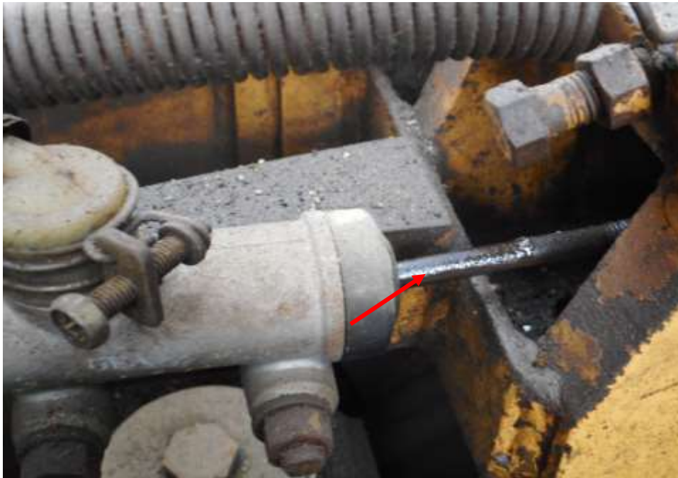
Photo 20 shows the brake cylinder piston (arrowed) there were sign(s) of old and fresh brake fluid stains leaking out from the brake cylinder piston.
