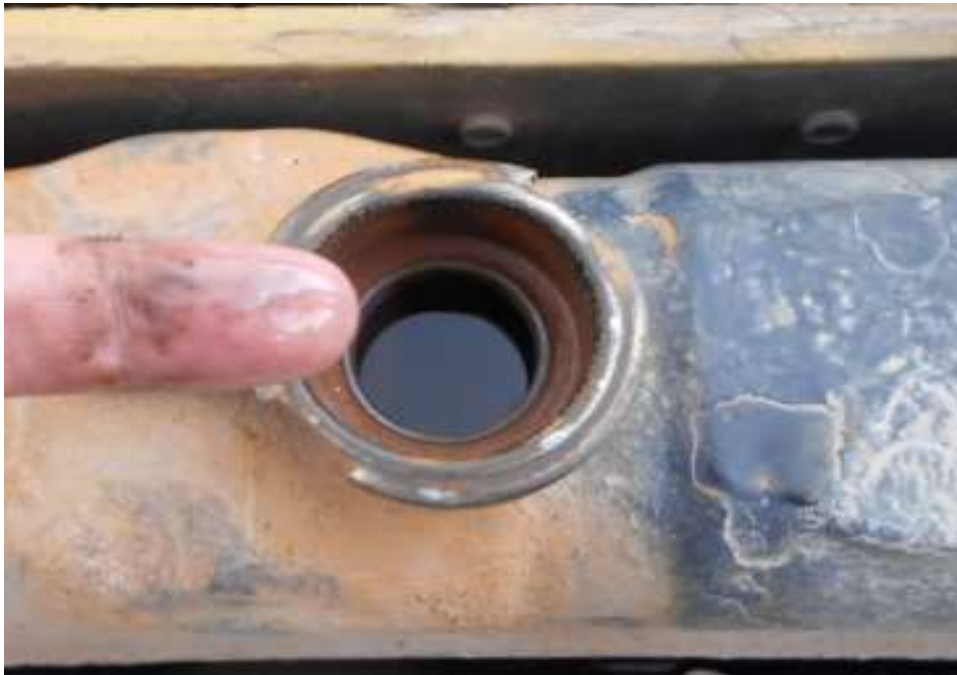
Photo 13 shows checks being carried out to the engine coolant of the Komatsu Forklift at the time of my inspection. The engine coolant was observed to be of sufficient level and without any visible contamination.
