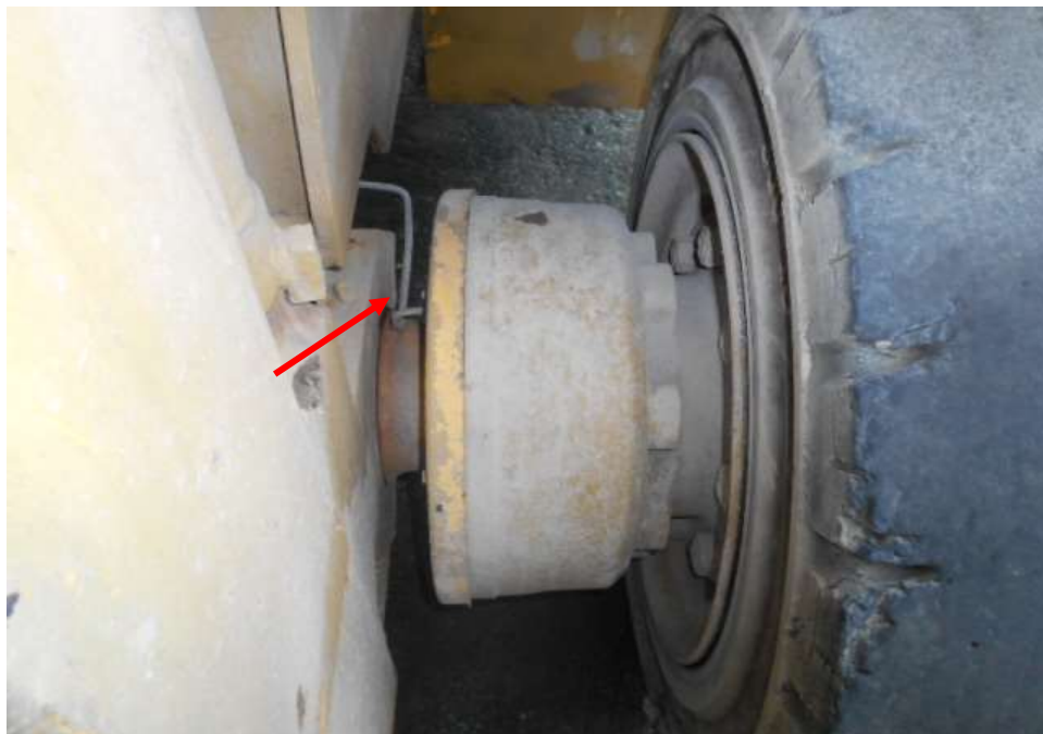
Photo 19 shows the brake hose/pipe (arrowed) at the front left wheel of the Komatsu Forklift. I did not observe any leakage of brake fluid at the time of my inspection of the Komatsu Forklift.
