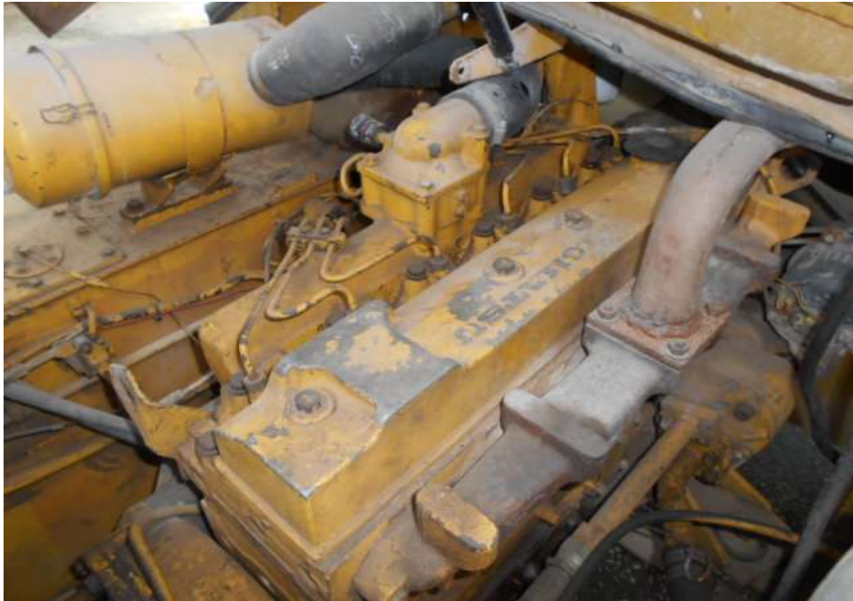
Photo 11 shows a general view of the Komatsu Forklift's engine compartment. The various parts and components inside the engine compartment were unaffected by the accident. There was also no sign(s) or indication(s) of fluid leakage and/or fluid stain within the engine compartment.
