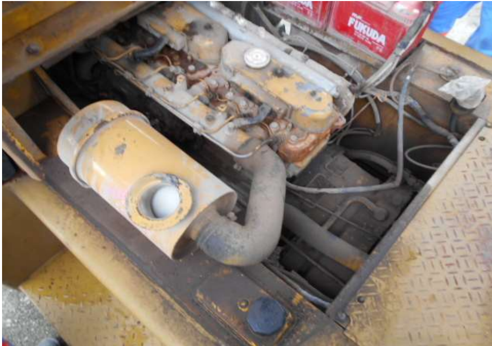
Photo 9 shows a general view of the Mitsubishi Forklift's engine compartment. The various parts and components inside the engine compartment were unaffected by the accident. There was also no sign(s) or indication(s) of fluid leakage and/or fluid stain within the engine compartment.
