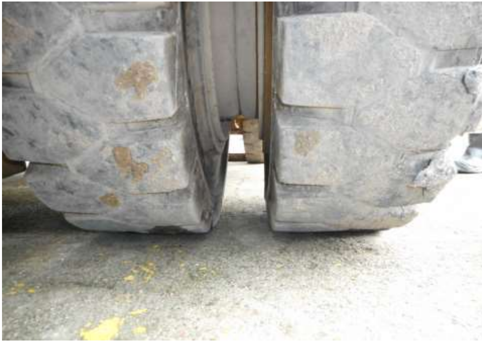
Photo 8 shows the condition of the front left tyre of the Mitsubishi Forklift, which was observed to be in serviceable condition with remaining tread depth of approximately 10.6mm. There was also no tear, cut or burst mark(s) on the outer and the inner sidewalls as well as across the tread of the Mitsubishi Forklift's 6 tyres.
