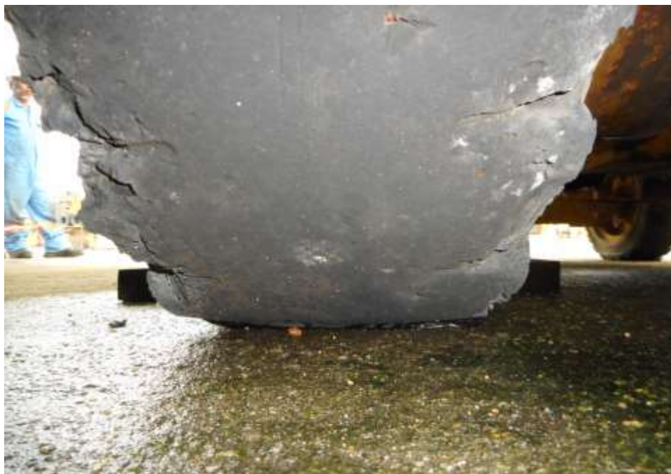
Photo 7 shows the condition of the front right tyre of the Komatsu Forklift, which was observed to be in unserviceable condition with remaining tread depth of approximately 0mm. The tyre was sufficiently inflated for vehicular operation with no tear, cut or burst mark(s) on the outer and the inner sidewalls as well as across the tread. The 4 tyres of the Komatsu Forklift were wrapped around standard steel wheel rims without any damage.
