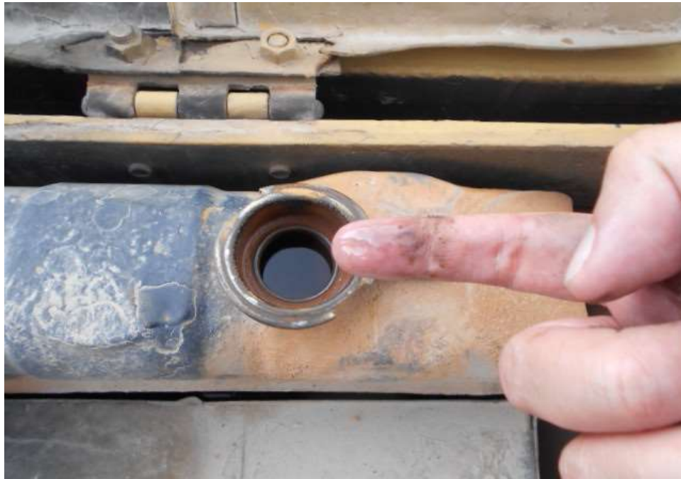
Photo 11 shows checks being carried out to the engine coolant of the Mitsubishi Forklift at the time of my inspection. The engine coolant was observed to be of sufficient level without any visible contamination.
