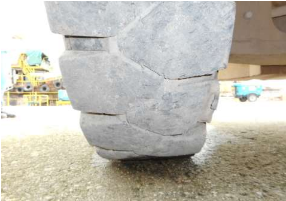
Photo 6 shows the condition of the rear right tyre of the Mitsubishi Forklift, which was observed to be in serviceable condition with remaining tread depth of approximately 8.5mm. The tyre was also observed to be sufficiently inflated for vehicular operation with no tear, cut or burst mark(s).
