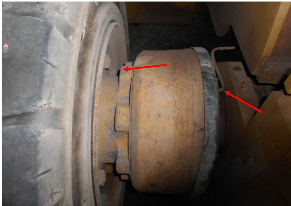
Photo 18 shows the brake hose/pipe (arrowed) at the front right wheel of the Komatsu Forklift. I did not observe any leakage of brake fluid at the time of my inspection of the Komatsu Forklift.
