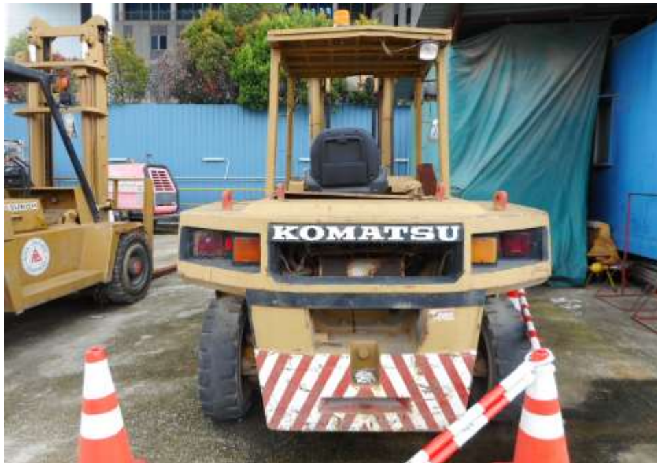
Photo 26 shows the both left and right signal and brake lights of the Komatsu Forklift were observed to be not working at the time of inspection.
