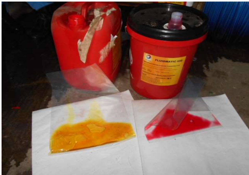
Photo 16 shows the differential gear oil (yellow colour) and the ATF transmission fluid (pink colour) used by the Komatsu Forklift and stored at the site warehouse at the time of my inspection.
