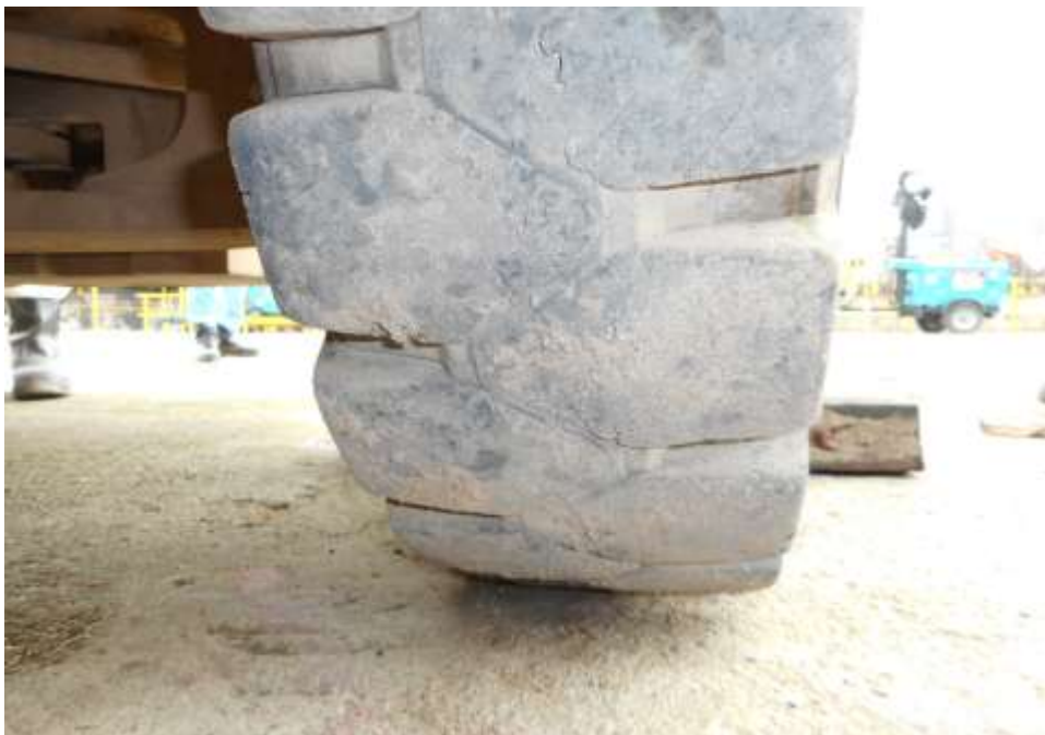
Photo 7 shows the condition of the rear left tyre of the Mitsubishi Forklift, which was observed to be in serviceable condition with remaining tread depth of approximately 7mm. The tyre, which was wrapped around steel wheel rim, was also observed to be sufficiently inflated for vehicular operation. The 6 tyres of the Mitsubishi Forklift were wrapped around standard steel wheel rims.
