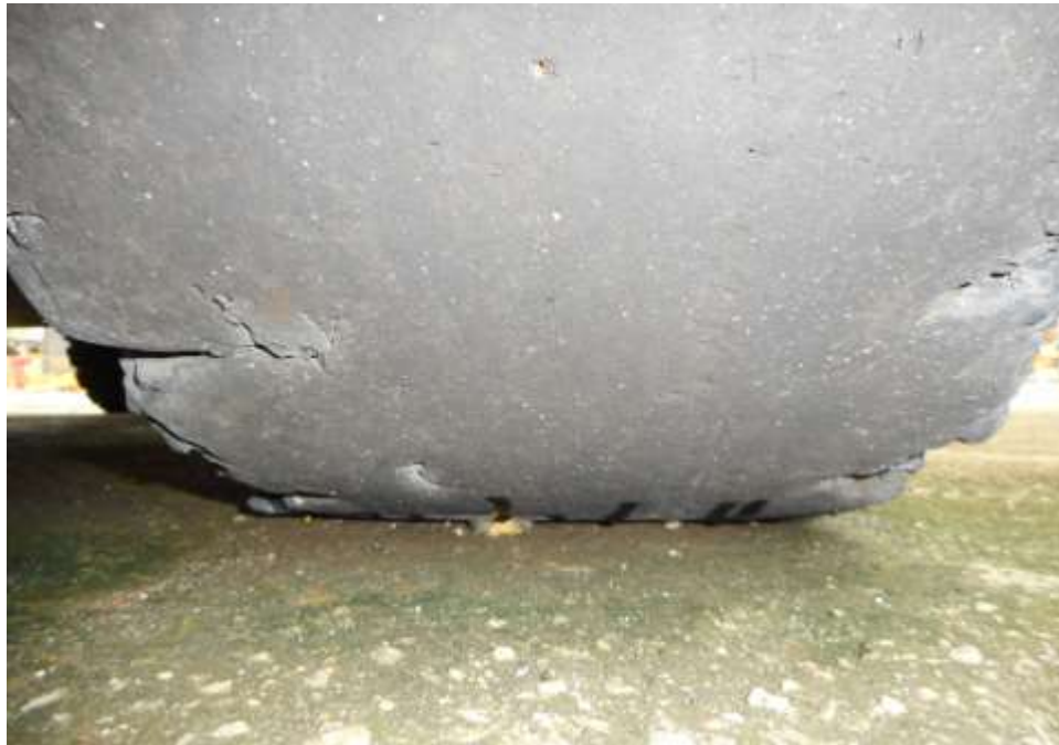
Photo 10 shows the condition of the front left tyre of the Komatsu Forklift, which was observed to be in unserviceable condition with remaining tread depth of approximately 0mm. There was also no tear, cut or burst mark(s) on the outer and the inner sidewalls as well as across the tread of the Komatsu Forklift's 4 tyres.
