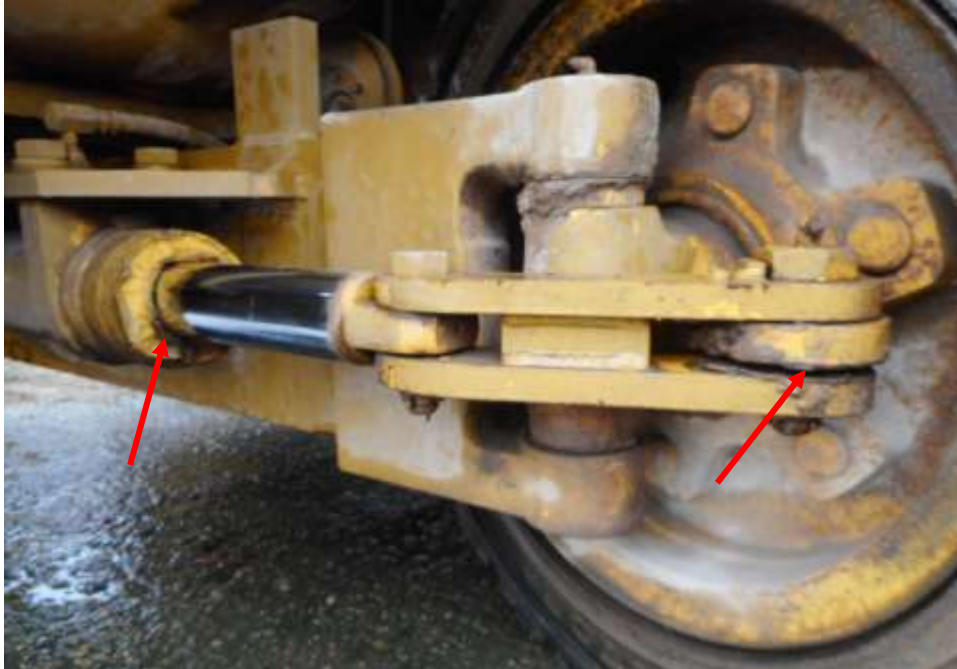
Photo 20 shows the various undercarriage components at the front right wheel of the Komatsu Forklift, in particular the steering cylinder and joints (red arrows). The various steering components were all found to be intact, suggesting that the steering system of the Komatsu Forklift was likely to be in serviceable condition at the material time of accident. There was also no sign of fluid stain observed on the various undercarriage components at the front right wheel of the Komatsu Forklift.
