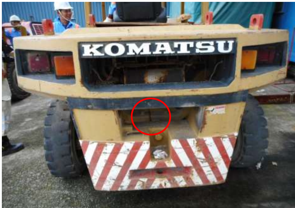
Photo 3 shows a rear view of the Komatsu Forklift's at the time of my inspection. Its rear frame (circled) was amongst the body parts that were damaged as a result of the accident.
