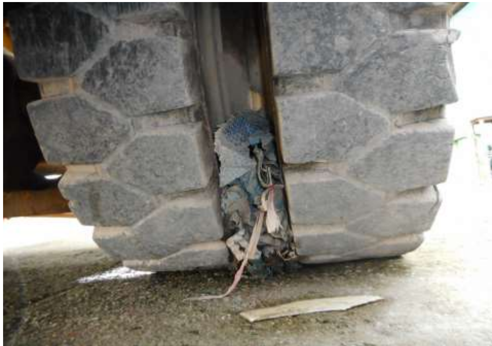
Photo 5 shows the condition of the front right tyre of the Mitsubishi Forklift, which was observed to be in serviceable condition with remaining tread depth of approximately 10.6mm. The tyre was sufficiently inflated for vehicular operation with no tear, cut or burst mark(s) on the outer and the inner sidewalls as well as across the tread. The 6 tyres of the Mitsubishi Forklift were wrapped around standard steel wheel rims without any damage.
