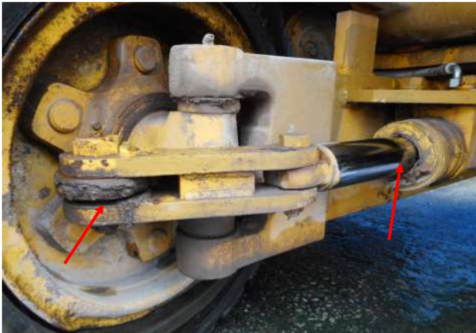
Photo 21 shows the various undercarriage components at the front left wheel of the Komatsu Forklift, in particular the steering cylinder and joints (red arrow). The various steering components were all found to be intact, suggesting that the steering system of the Komatsu Forklift was likely to be in serviceable condition at the material time of accident. There was also no sign of fluid stain observed on the various undercarriage components at the front left wheel of the Komatsu Forklift.
