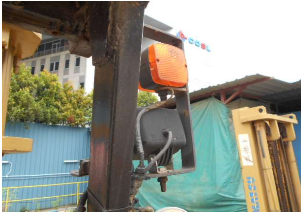
Photo 27 shows the right signal and headlights of the Mitsubishi Forklift to be intact and serviceable condition at the time of inspection.
