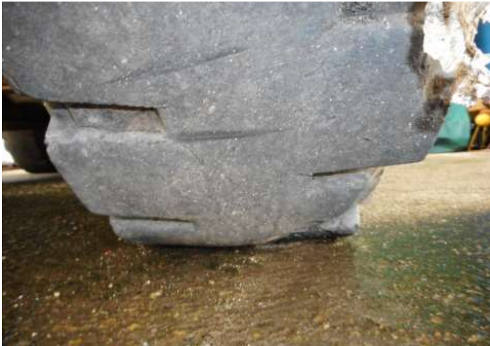
Photo 8 shows the condition of the rear right tyre of the Komatsu Forklift, which was observed to be in serviceable condition with remaining tread depth of approximately 9.4mm. The tyre was also observed to be sufficiently inflated for vehicular operation with no tear, cut or burst mark(s).
