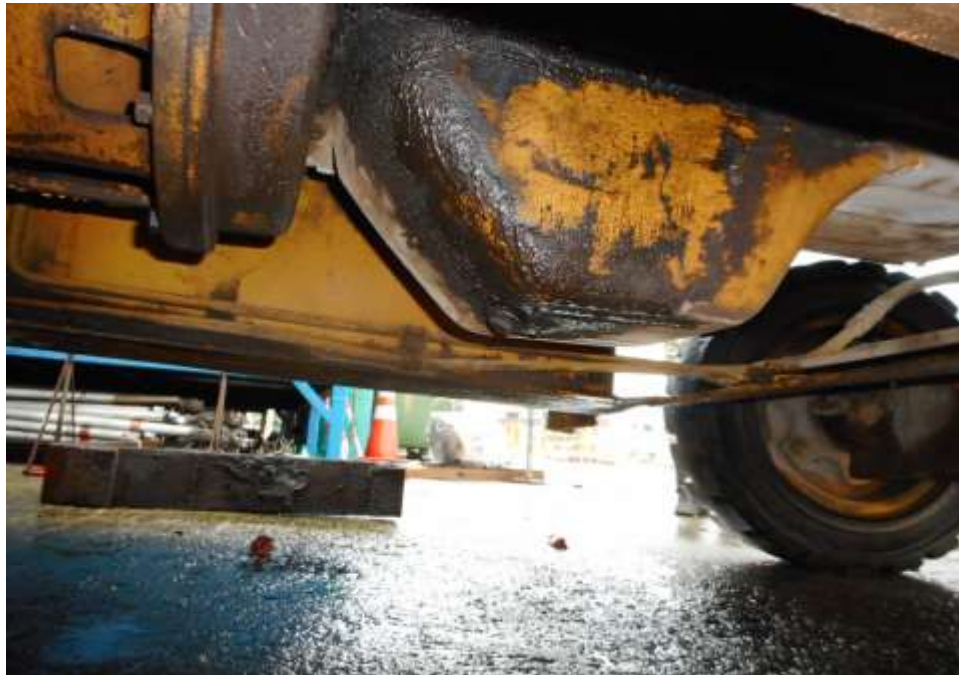
Photo 17 shows the undercarriage of the Komatsu Forklift, at the area where the engine housing and transmission housing are located. I observed old fluid stain(s) on the underside of the Komatsu Forklift.
