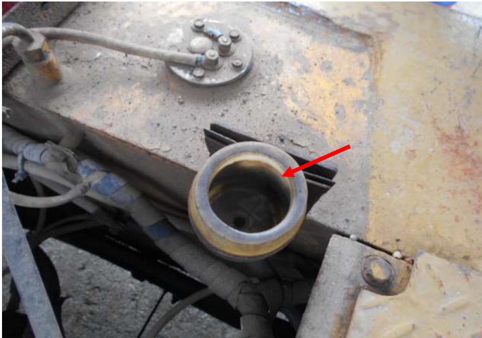
Photo 10 shows the brake fluid reservoir of the Mitsubishi Forklift at the time of my inspection. The brake fluid was observed to be insufficient level (arrowed)
