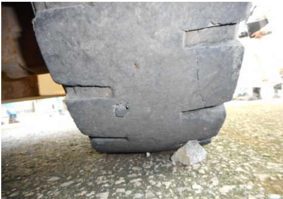
Photo 9 shows the condition of the rear left tyre of the Komatsu Forklift, which was observed to be in serviceable condition with remaining tread depth of approximately 9.6mm. The tyre, which was wrapped around steel wheel rim, was also observed to be sufficiently inflated for vehicular operation. The 4 tyres of the Komatsu Forklift were wrapped around standard steel wheel rims.
