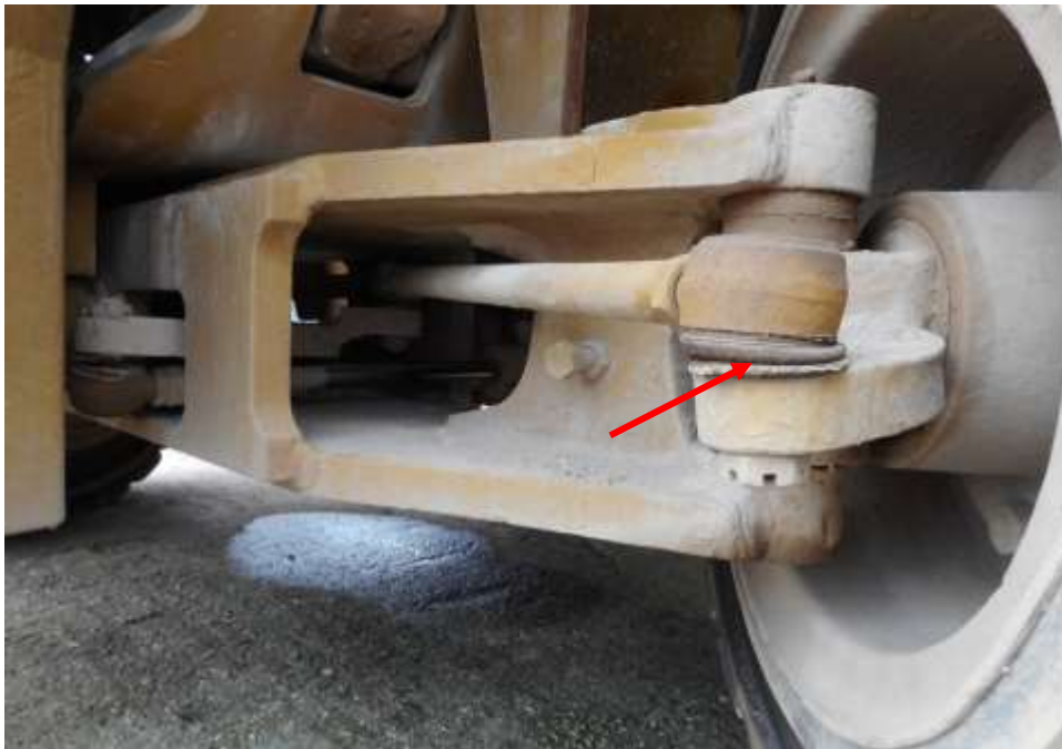
Photo 21 shows the various undercarriage components at the front right wheel of the Mitsubishi Forklift, in particular the steering tie rod (red arrow). The various steering components were all found to be intact, suggesting that the steering system of the Mitsubishi Forklift was likely to be in serviceable condition at the material time of accident. There was also no sign of fluid stain observed on the various undercarriage components at the front right wheel of the Mitsubishi Forklift.
