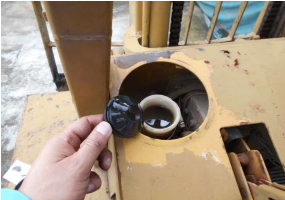
Photo 12 shows checks being carried out to the brake fluid of the Komatsu Forklift at the time of my inspection. The brake fluid was observed to be of sufficient level and without any visible contamination.
