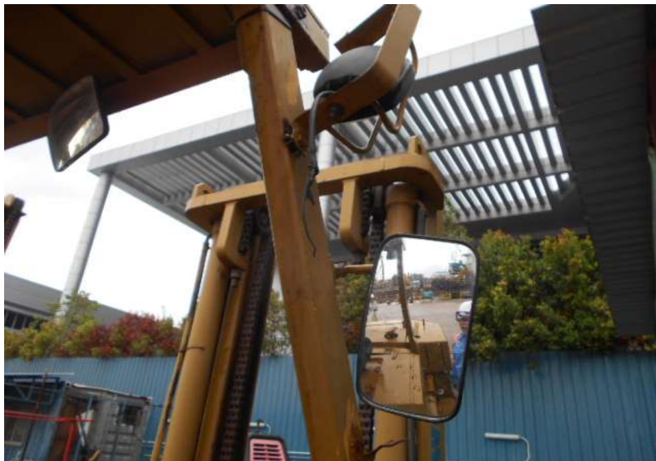
Photo 24 shows a disconnected right headlight and no right signal light installed. However, a right rear view mirror was observed on the Komatsu Forklift at the time of inspection.
