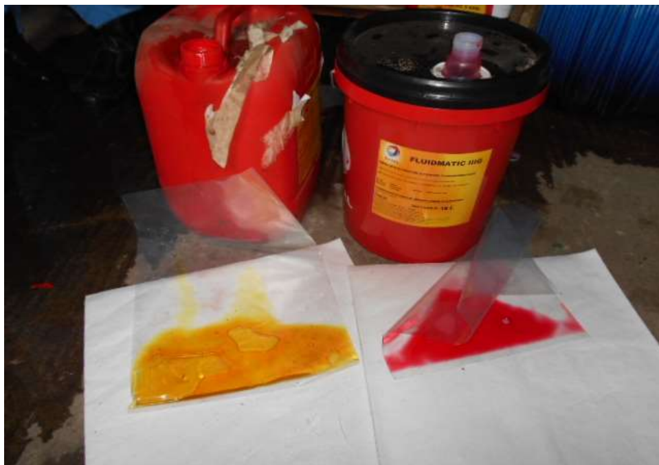
Photo 14 shows the differential gear oil (yellow colour) and the ATF transmission fluid (pink colour) used by the Mitsubishi Forklift and stored at the site warehouse at the time of my inspection.
