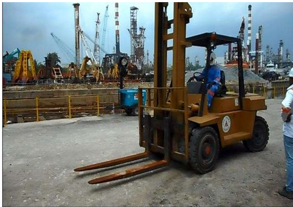
Photo 23 shows the rear left wheel of the Mitsubishi Forklift turned to its full right. During my steering system test, I did not experience any abnormal free play and/or resistance when I had turned the steering wheel towards the left and right. This would suggest that the steering system of the Mitsubishi Forklift was likely to be in serviceable condition at the material time of accident.
