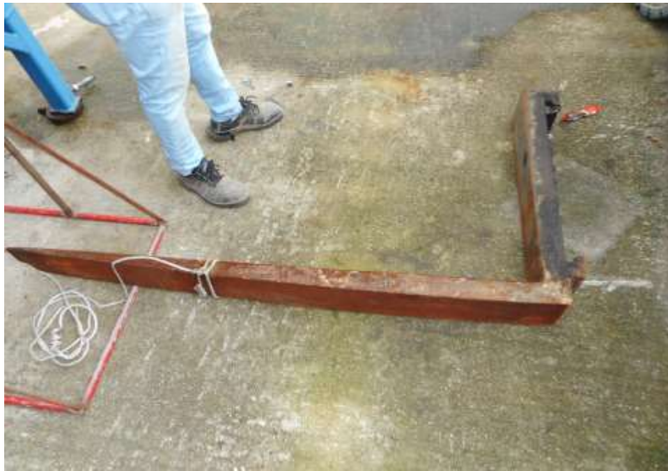
Photo 2 shows a close up view of the Komatsu Forklift's Fork at the time of my inspection. Its left fork was amongst the body parts that were damaged as a result of the accident.
