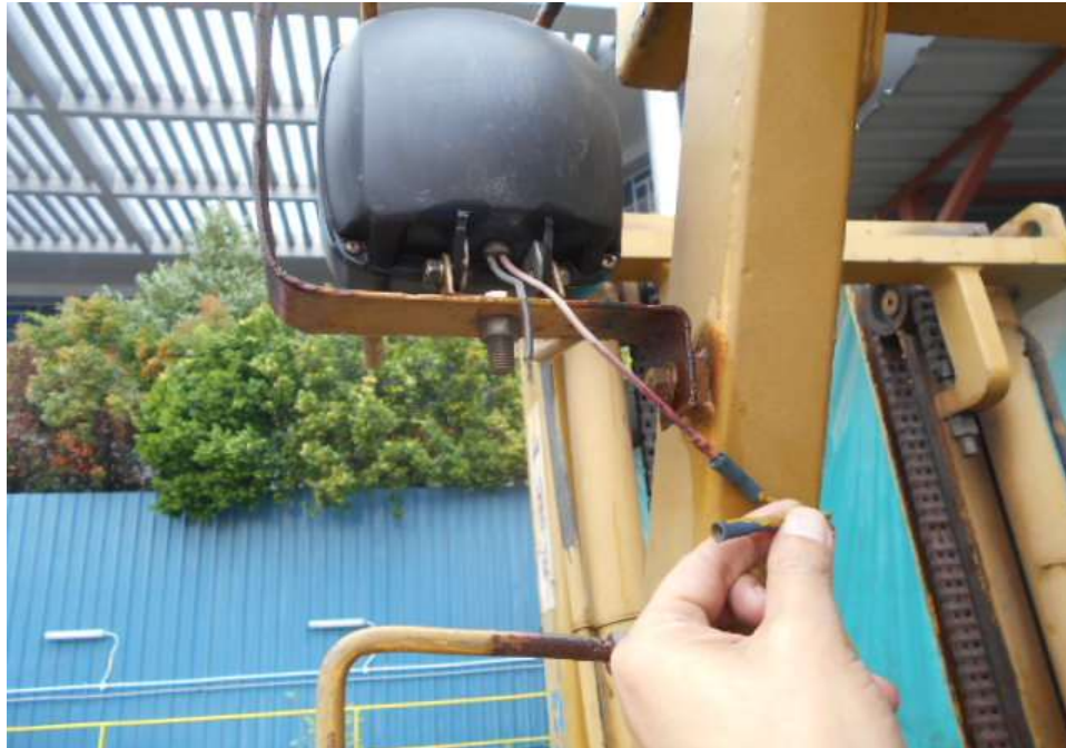
Photo 23 shows a disconnected left headlight. No left rear view mirror and front signal lights were installed on the Komatsu Forklift at the time of inspection.
