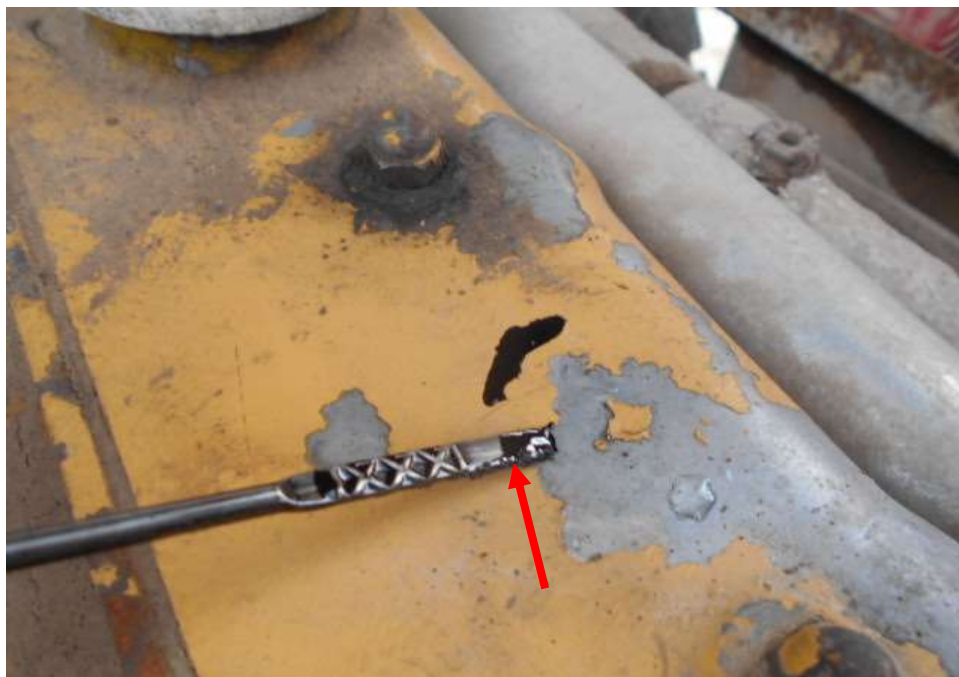
Photo 12 shows the engine oil dip stick of the Mitsubishi Forklift at the time of my inspection. The engine oil was observed to be of insufficient level (arrowed)
