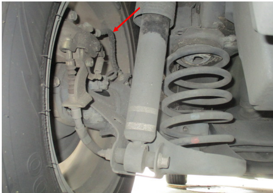
Photo 13 shows the brake hose/pipe (arrowed) at the rear left wheel of the Motor Taxi. We did not observe any leakage of brake fluid at the time of our inspection of the Motor Taxi. Static tests of the Motor Taxi's braking system had indicated that there was no internal leakage of pressure/vacuum. Hence the braking system was likely to be in serviceable condition at the material time of accident. The undercarriage components of the Motor Taxi were also all found to be intact and without any visible damage.
