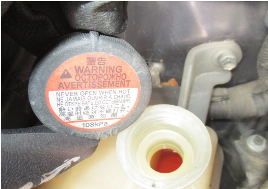
Photo 10 shows checks being carried out to the engine coolant of the Motor Taxi at the time of our inspection. The engine coolant was observed to be of sufficient level and without any visible contamination.
