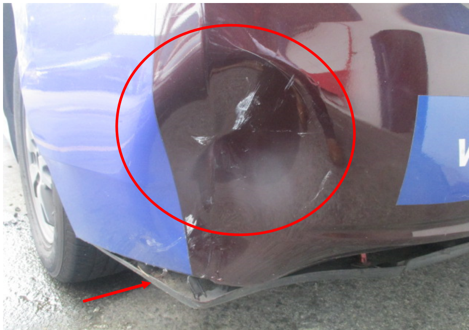
Photo 3 shows a closer view of the deformed rear bumper (circled) and rear bumper under cover (arrowed).
