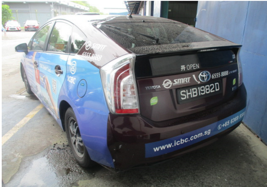
Photo 2 shows a general view of the left rear body of the Motor Taxi at the time of our inspection. The Motor Taxi was observed to be in good general condition. However we had observed relatively minor impact damage that was confined to its rear portion. The rear bumper and rear bumper undercover were observed to be deformed.
