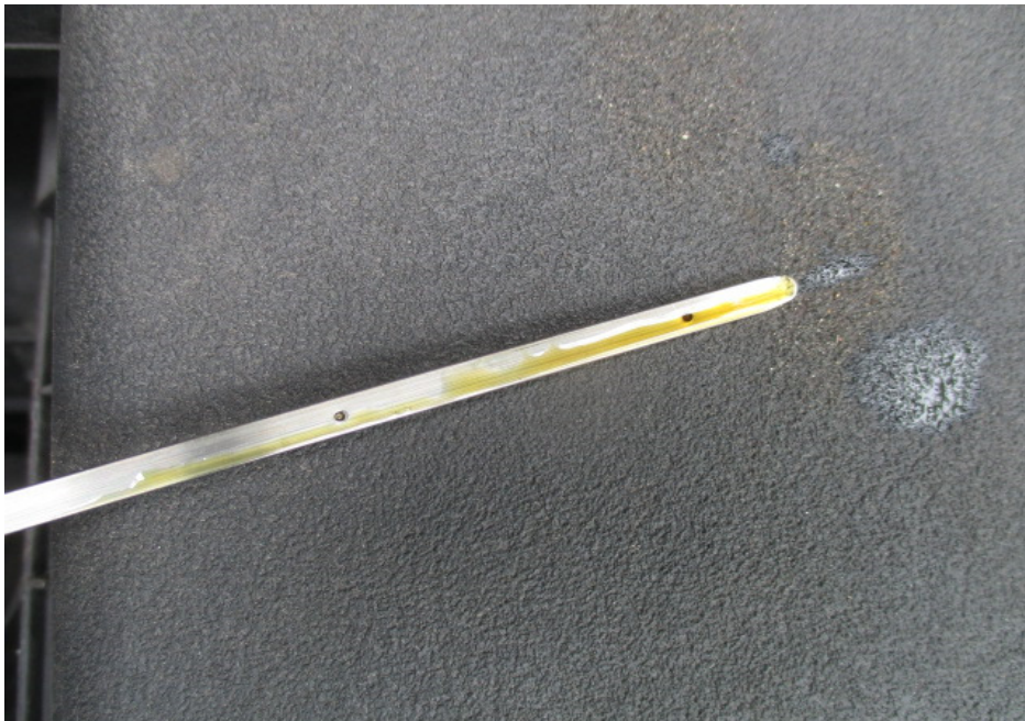
Photo 12 shows the engine oil dip stick of the Motor Taxi at the time of our inspection. The engine oil was observed to be of sufficient level and without any visible contamination.
