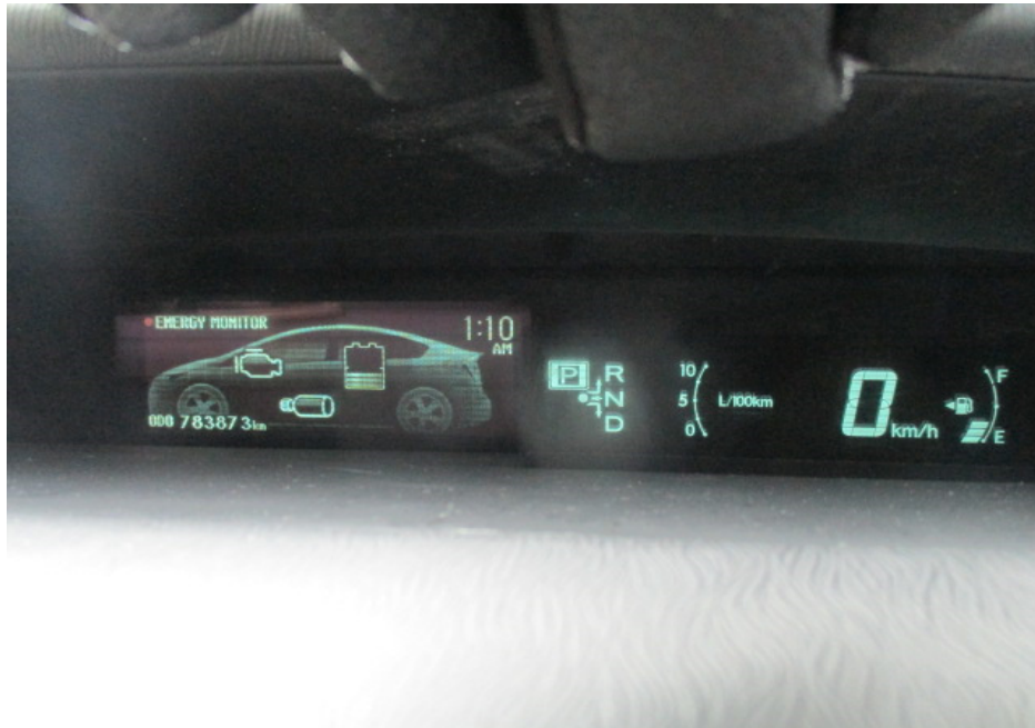
Photo 21 shows no warning lights illuminated on the instrument panel of the Motor Taxi after the engine was cranked. This would suggest that there was no abnormality to the various electronic operating systems of the Motor Taxi, like the EPS, ABS and ESC etc.
