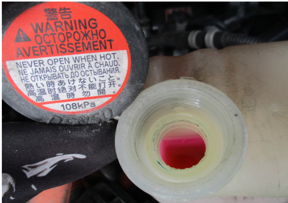
Photo 11 shows the coolant reservoir for the hybrid system of the Motor Taxi at the time of our inspection. The hybrid system coolant was observed to be of sufficient level and without any visible contamination
