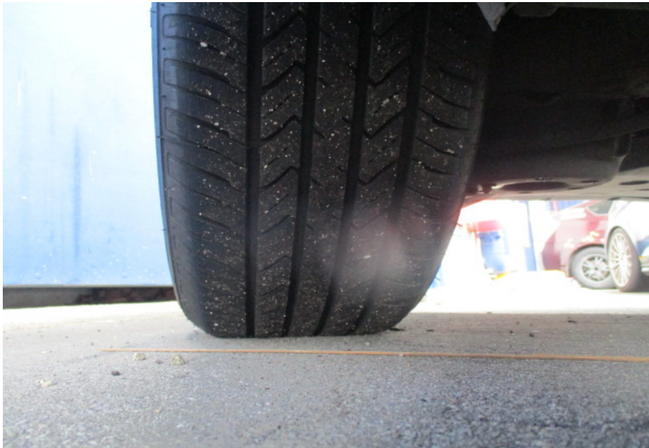
Photo 7 shows the condition of the rear right tyre of the Motor Taxi, which was observed to be in serviceable condition with remaining tread depth of approximately 5mm. There was also no tear, cut or burst mark(s) on the outer and the inner sidewalls as well as across the tread of the 4 tyres.
