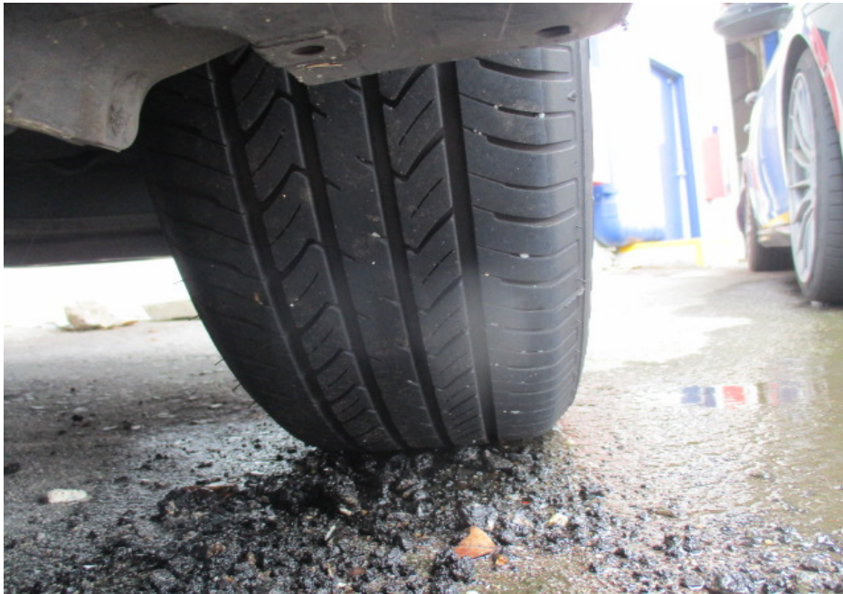
Photo 6 shows the condition of the rear left tyre of the Motor Taxi, which was observed to be in serviceable condition with remaining tread depth of approximately 5mm. The tyre, which was wrapped around alloy wheel rim, was also observed to be sufficiently inflated for vehicular operation. There was also no damage found on the 4 wheel rims of the Motor Taxi.
