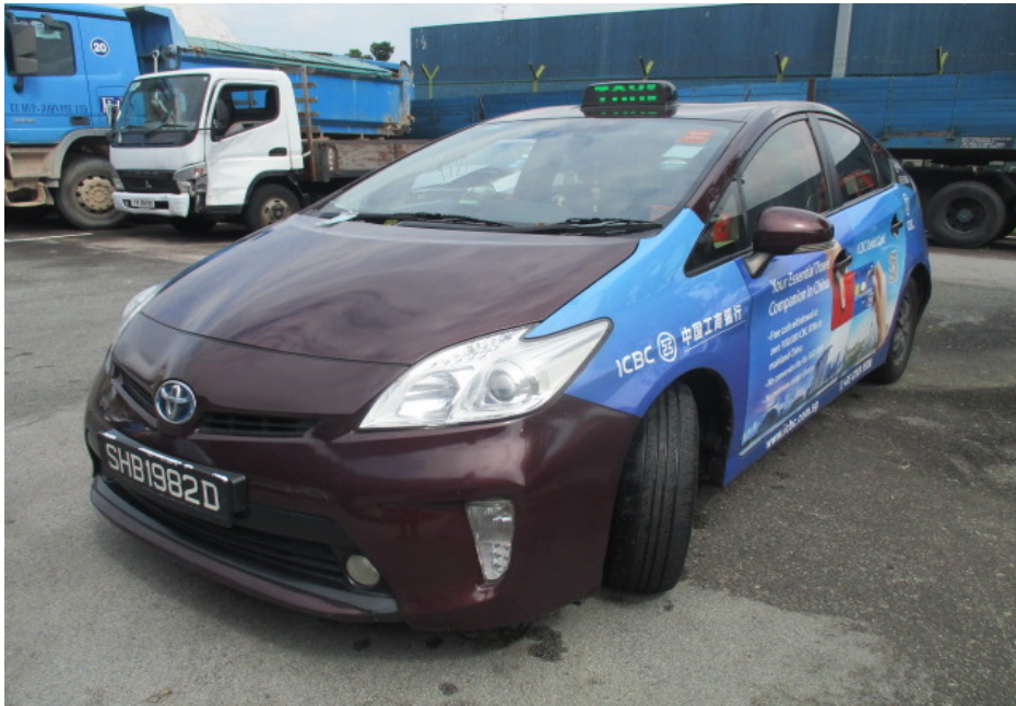
Photo 18 shows the front left wheel of the Motor Taxi turned to its full left. During our steering system test, we did not experience any abnormal free play and/or resistance when we had turned the steering wheel towards the left and right. This would suggest that the steering system of the Motor Taxi was likely to be in serviceable condition at the material time of accident.
