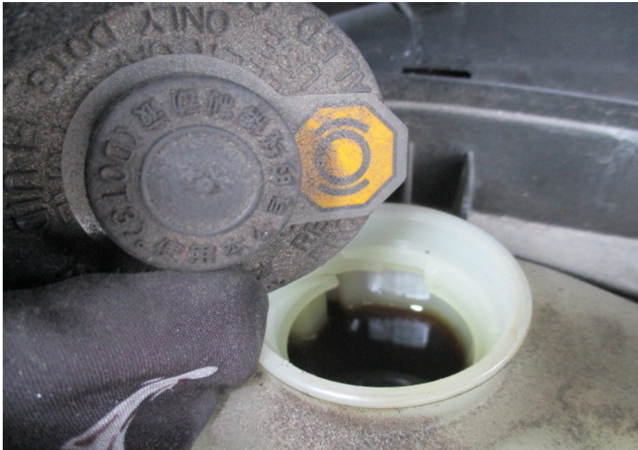
Photo 9 shows the brake fluid reservoir of the Motor Taxi at the time of our inspection. The brake fluid was observed to be of sufficient level and without any visible contamination.
