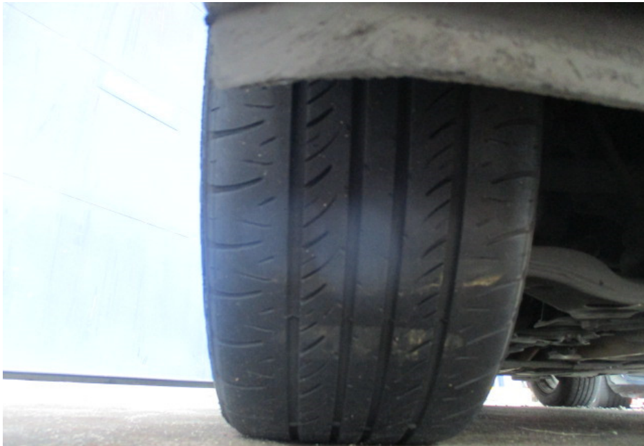
Photo 5 shows the condition of the front right tyre of the Motor Taxi, which was observed to be in serviceable condition with remaining tread depth of approximately 4mm. The tyre, which was wrapped around alloy wheel rim, was also observed to be sufficiently inflated for vehicular operation.
