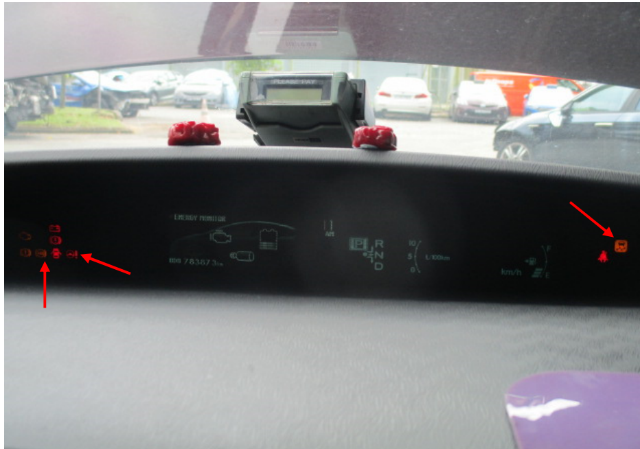
Photo 20 shows the warning lights for the various electronic operating systems of the Motor Taxi appearing on its instrument panel during the self-test when the engine is cranked, in particular the EPS light, ABS light and ESC light (arrowed).
