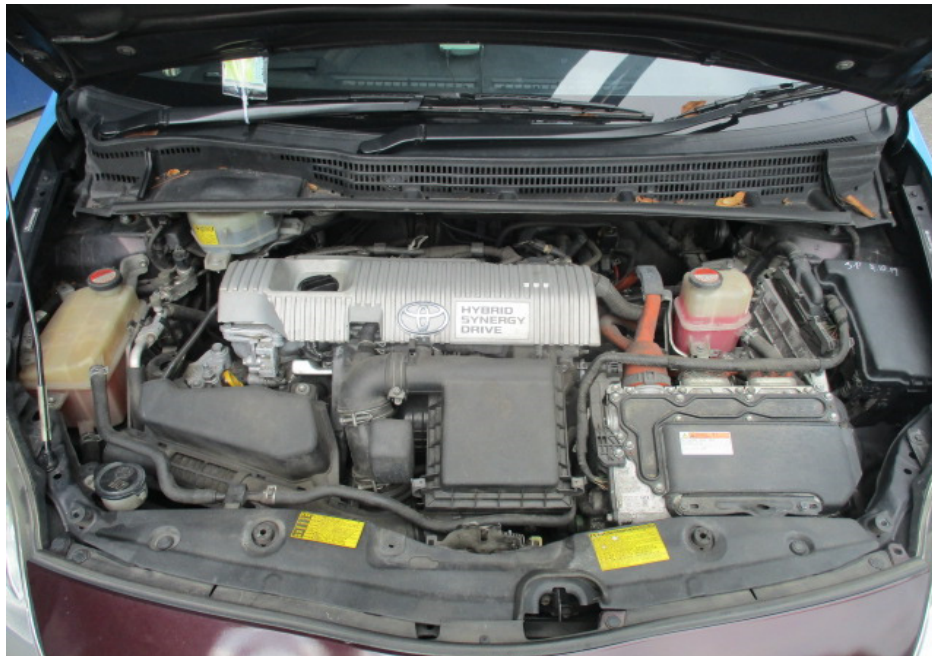
Photo 8 shows a general view of the Motor Taxi's engine compartment. The various parts and components inside the engine compartment were unaffected by the accident. The wirings and cables for the hybrid system were all further observed to be intact and adequately secured to their respective terminals and/or connecting ports. There was also no sign(s) or indication(s) of fluid leakage and/or fluid stain within the engine compartment.
