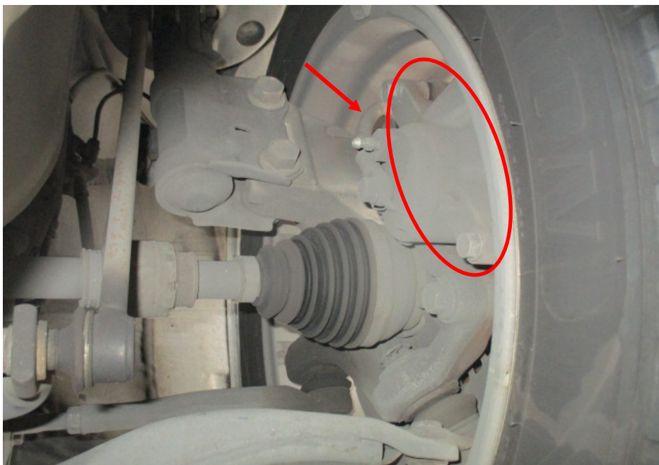
Photo 15 shows the brake hose/pipe (arrowed) at the front left wheel of the Motor Taxi. No leakage of brake fluid was observed. Visual examination of the various components of the braking system like the brake caliper (circled), brake pedal etc. had revealed all to be intact and without visible damage.
