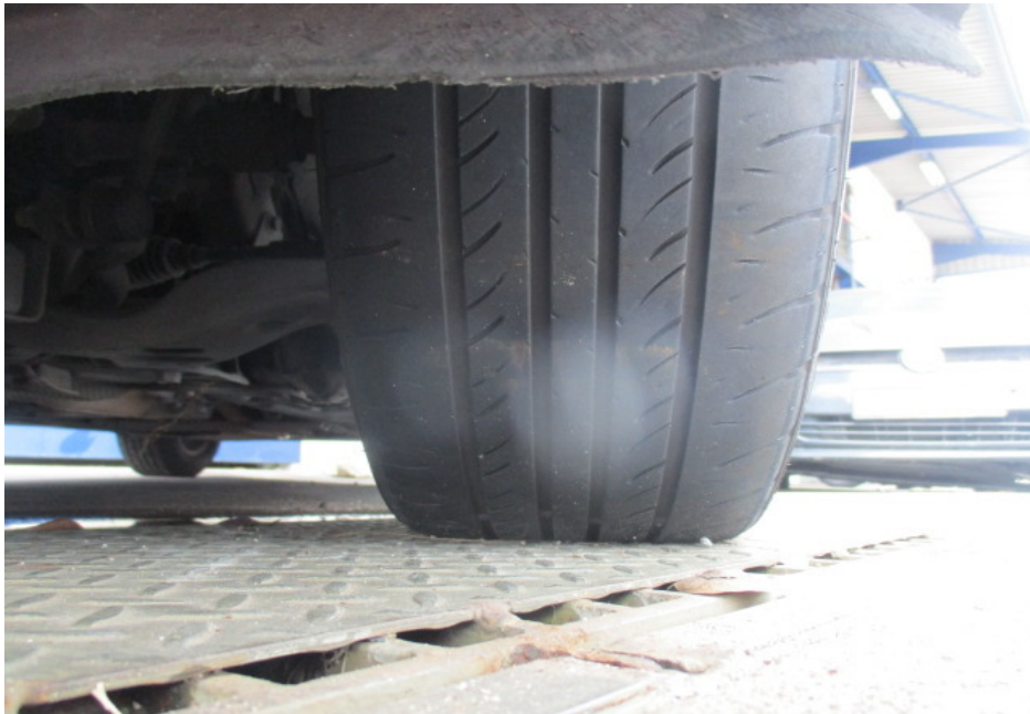
Photo 4 shows the condition of the front left tyre of the Motor Taxi, which was observed to be in serviceable condition with remaining tread depth of approximately 5mm. The tyre, which was wrapped around alloy wheel rim, was also observed to be sufficiently inflated for vehicular operation. There was no tear, cut or burst mark(s) on the outer and the inner sidewalls as well as across the tread of the 4 tyres.
