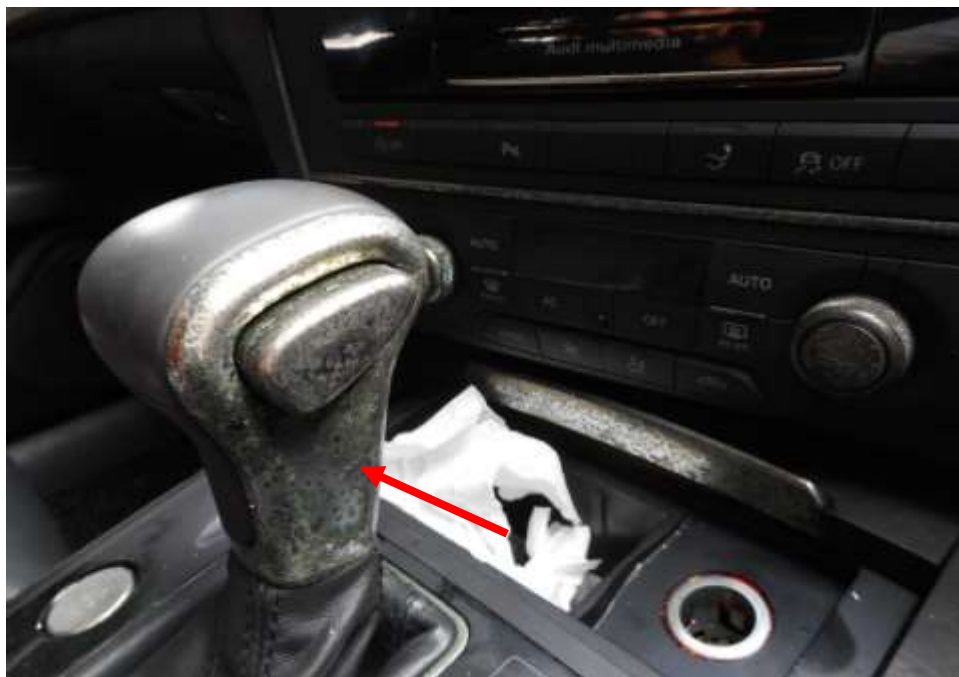
Photo 11 shows the general view of the gear knob trims of the Insured Vehicle at the time of our inspection. The surface had also suffered heat and smoke damages (arrowed) as a result of the fire.
