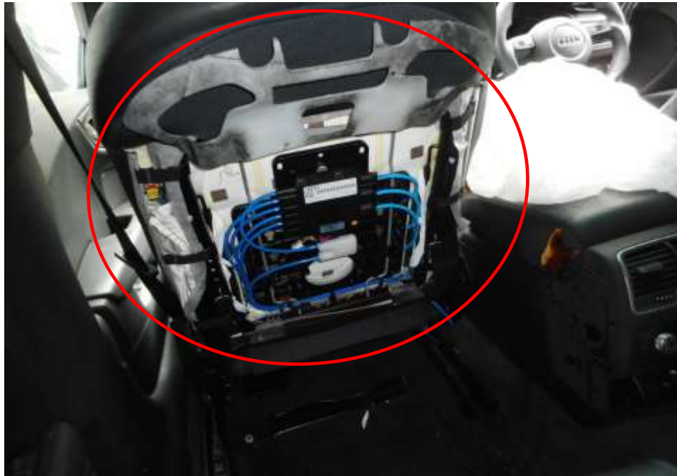
Photo 17 shows the close up view of the from rear left passenger seating compartment of the Insured Vehicle at the time of our inspection. The rear of left seat backing cover (circled) was found to have been missing at the time of the inspection.
