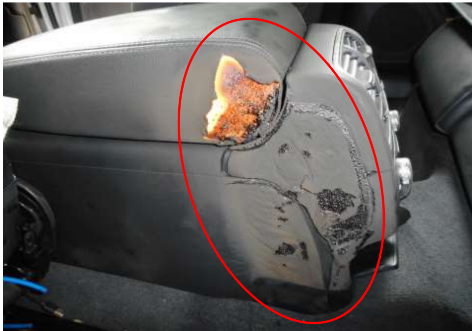
Photo 14 shows the close up view of the from rear left passenger seating compartment of the Insured Vehicle at the time of our inspection. Its centre console armrest (circled) was found to have been burnt and melt as a result of the fire.
