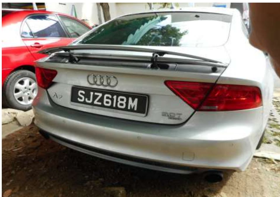
Photo 5 shows the general view of the rear portion of the Insured Vehicle at the time of our inspection. The fire damage to the Insured Vehicle was confined to its interior portion. Its exterior is observed to be unaffected by the fire.
