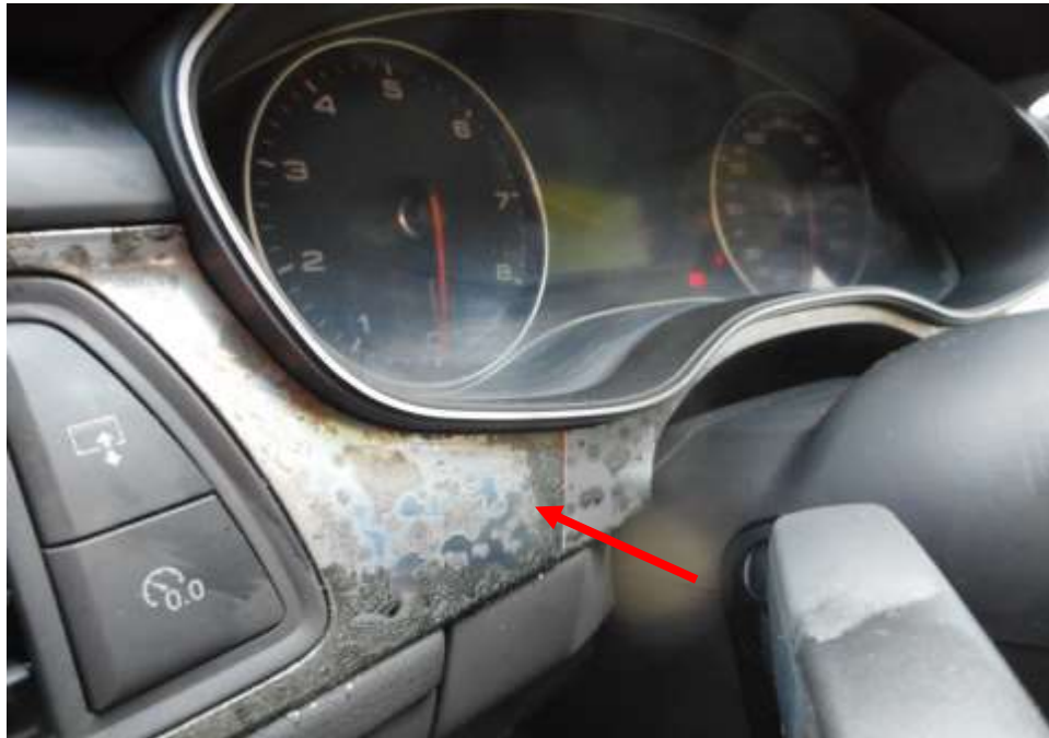
Photo 10 shows the general view of the dashboard trims of the Insured Vehicle at the time of our inspection. The surface had suffered heat and smoke damages (arrowed) as a result of the fire.
