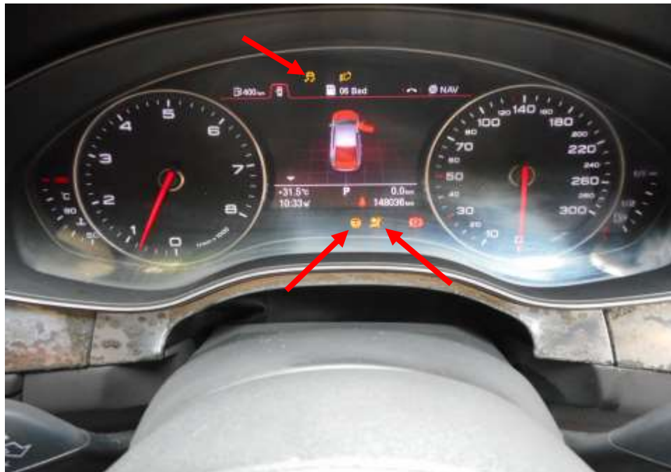
Photo 8 shows the general view of the driver instrument panel of the Insured Vehicle at the time of our inspection. The various error codes (arrowed) on the Insured Vehicle were lighted up due to the smoke and heat damages that had inference sensors of the electronic components causing them to be illuminated.
