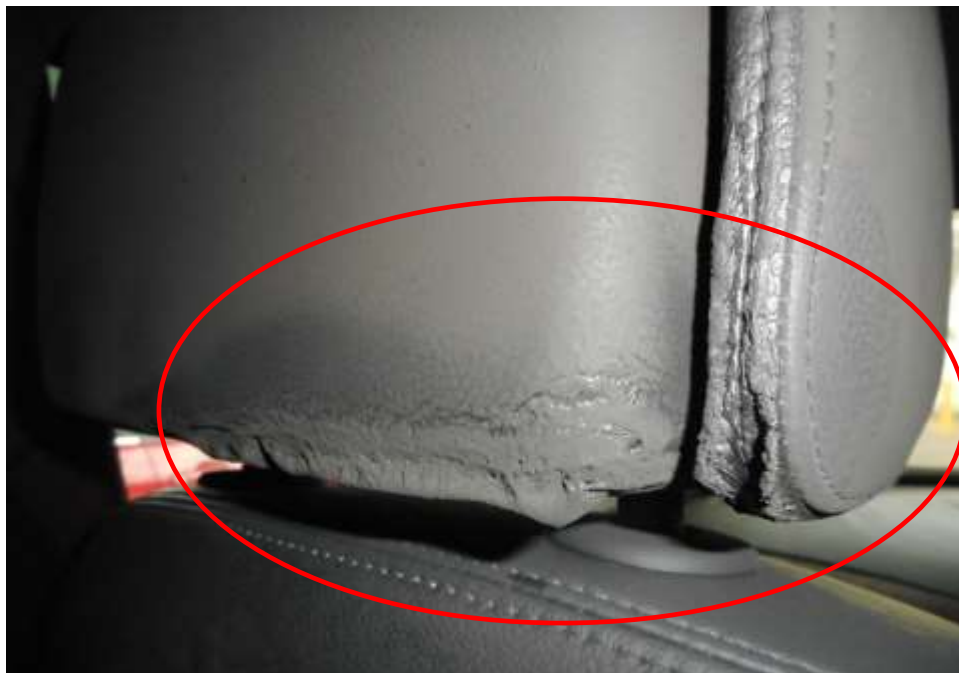
Photo 18 shows the close up view of the from rear left passenger seating compartment of the Insured Vehicle at the time of our inspection. The rear of the left seat headrest (circled) was found to have been burnt and melted as a result of the fire.
