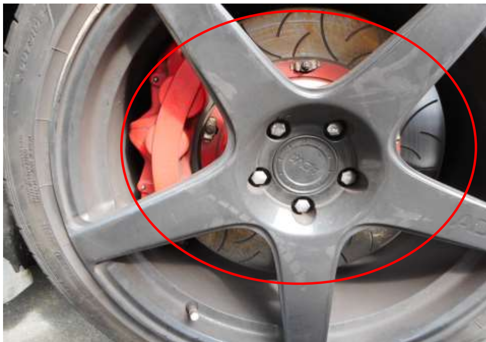
Photo 12 shows a set of aftermarket brake calipers and disc brakes on the Insured Vehicle, which was observed to be unaffected by the fire.
