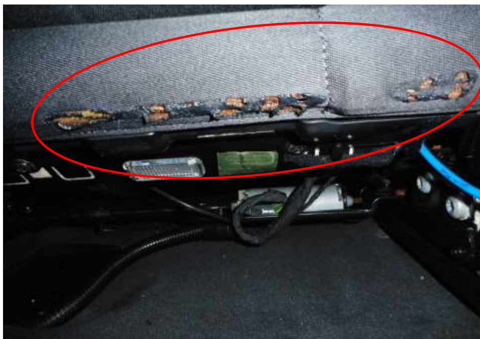
Photo 16 shows the close up view of the from rear left passenger seating compartment of the Insured Vehicle at the time of our inspection. The rear of the left seat (circled) was found to have been burnt as a result of the fire.
