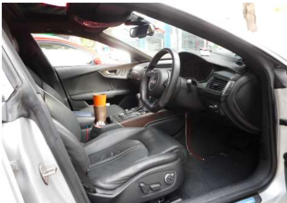
Photo 7 shows the general view of the interior compartment of the Insured Vehicle at the time of our inspection. The fire was confined to its rear left passenger seat portion, however the fire had resulted in the various components located in the interior of the Insured Vehicle suffer from heat and smoke damages, this includes the driver instrument panel, multimedia infotainment head-unit, driver steering, signalling equipment's, electronic components and several parts inside the other interior compartment that were also observed to sustain damages included centre console armrest, front left seat and dashboard trims.
