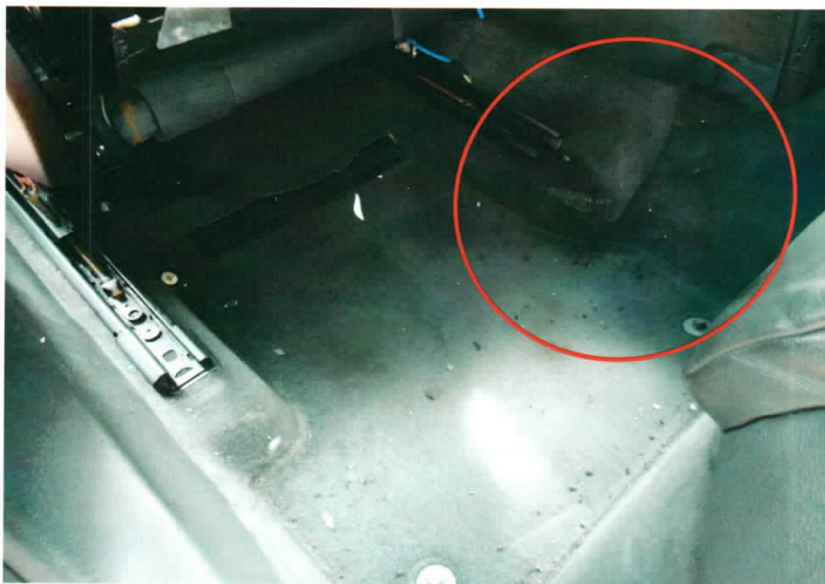
Photo 15 shows the close up view of the from rear left passenger seating compartment of the Insured Vehicle at the time of our inspection. Its rear left foot well (circled) was found to have been burnt as a result of the fire.
