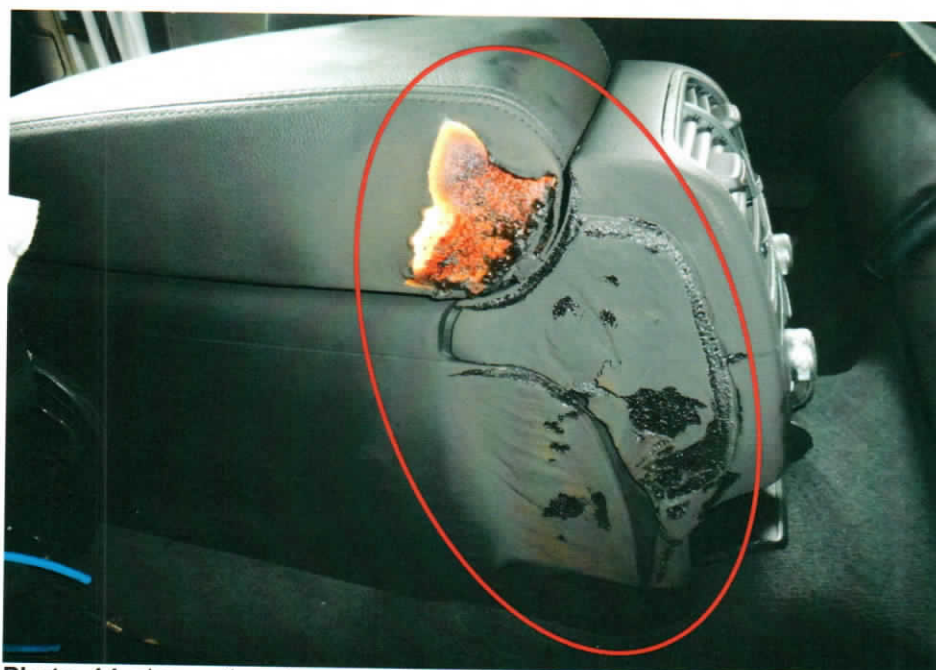
Photo 14 shows the close up view of the rear left passenger seating compartment of the Insured Vehicle at the time of our inspection. Its centre console armrest (circled) was found to have been burnt and melt as a result of the fire.
