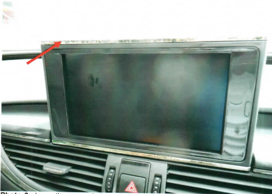
Photo 9 shows the general view of the multimedia infotainment head-unit of the Insured Vehicle at the time of our inspection. The unit was not illuminated when turned on and the surface on it had suffered heat and smoke damages (arrowed) as a result of the fire.
