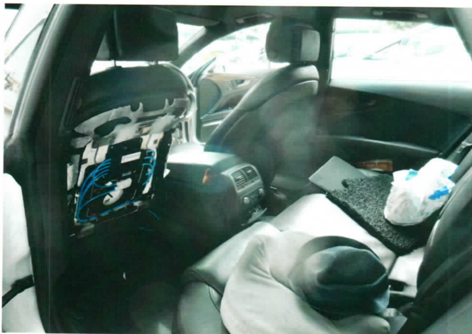
Photo 13 shows the general view of the rear passenger seating compartment of the Insured Vehicle at the time of our inspection. The fire damage to the Insured Vehicle was confined to its left seating portion. Its centre console armrest and rear of the front left seat are amongst the body parts that were found to have been affected as a result of the fire.
