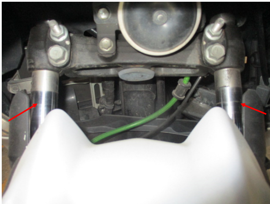
Photo 21 shows the front forks (arrowed) of the Motorcycle. The front forks and fork brackets of the Motorcycle were both found to be intact and undamaged. Turning the Motorcycle's handle bar towards the left and right did not produce any abnormal free play and/or resistance. The steering system of the Motorcycle was in serviceable condition at the time of our inspection.
