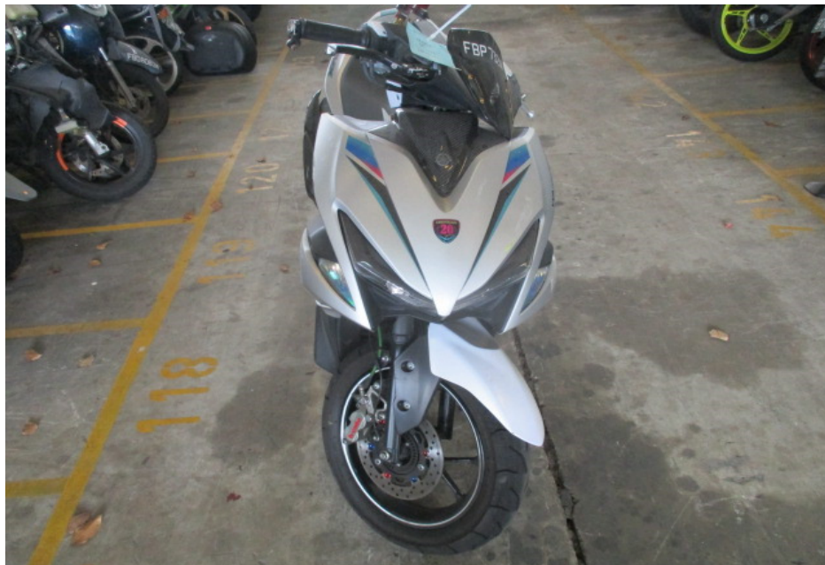
Photo 23 shows the front wheel of the Motorcycle turned towards its full left. Turning the Motorcycle's handle bar towards the left and right did not produce any abnormal free play and/or resistance. This would indicate that the steering system of the Motorcycle was in serviceable condition at the time of our inspection.
