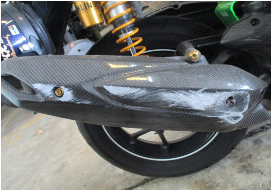
Photo 9 shows a closer view of the exhaust muffler heat shield of the Motorcycle which had sustained damage due to the accident.
