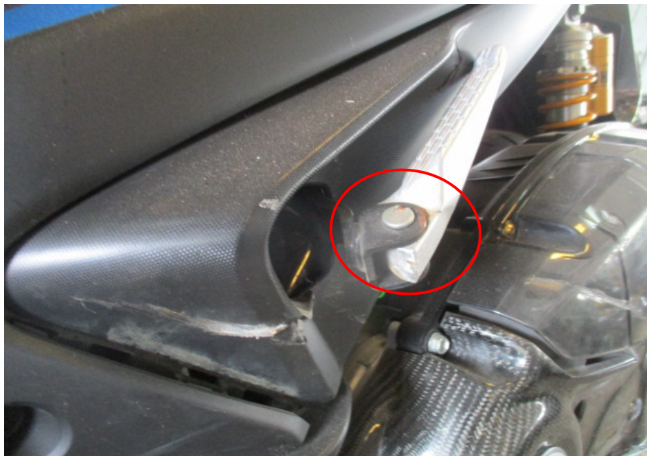
Photo 14 shows a closer view of the grazed left pillion footrest (circled) of the Motorcycle at the time of our inspection.
