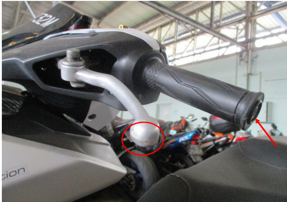
Photo 11 shows a closer view of the rear brake lever (circled) and right handlebar end (arrowed) of the Motorcycle which were observed to be damaged due to the accident
