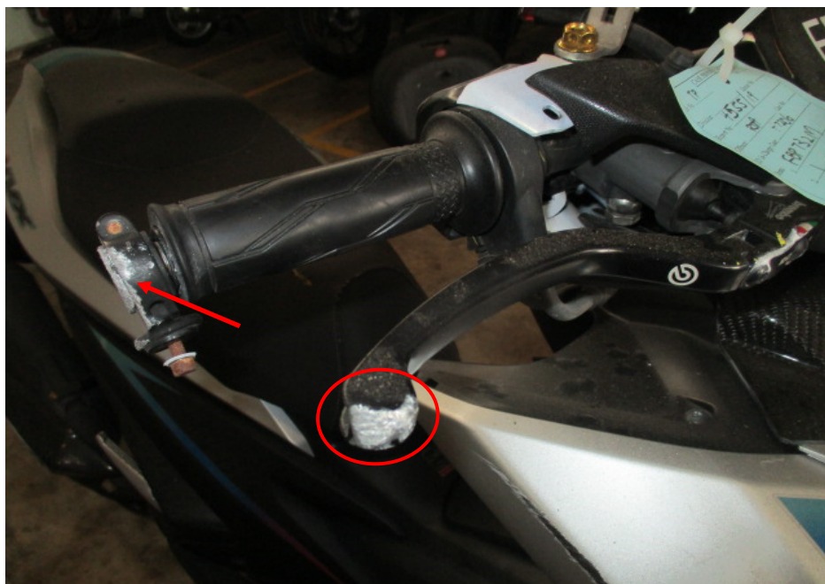
Photo 6 shows a closer view of the front brake lever (circled) and right handlebar end (arrowed) of the Motorcycle which were observed to be damaged due to the accident
