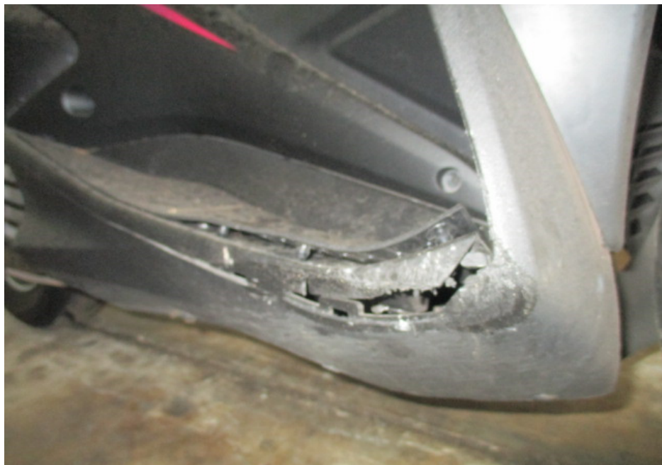
Photo 8 shows a closer view of the right bottom cowling of the Motorcycle which was observed to be damaged due to the accident.
