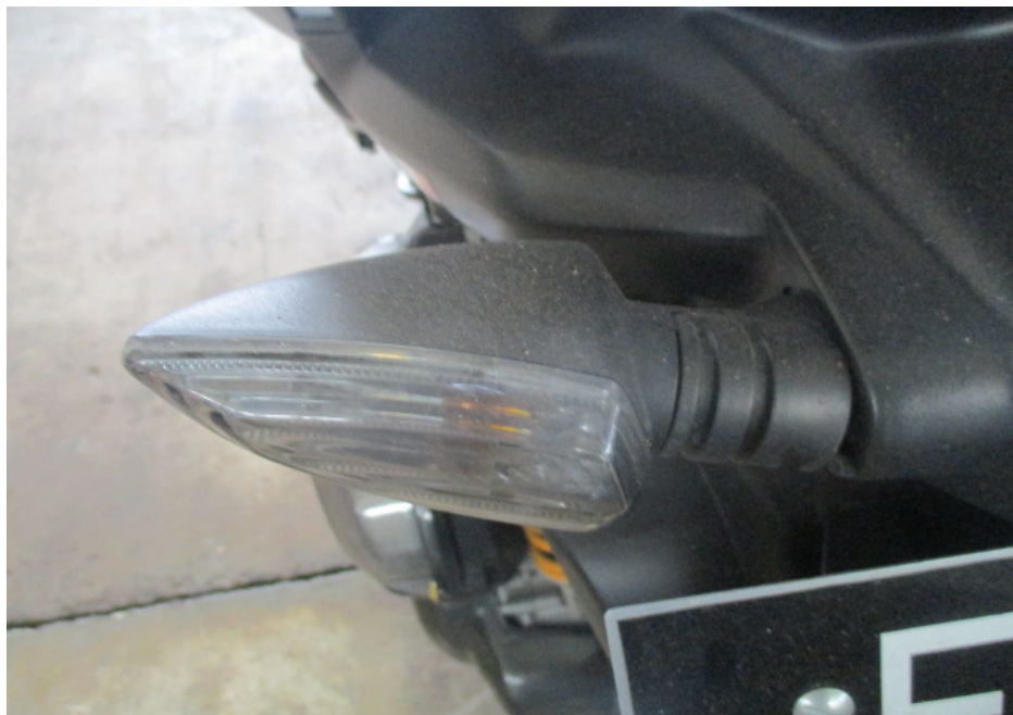
Photo 12 shows the broken left rear signal lamp of the Motorcycle.
