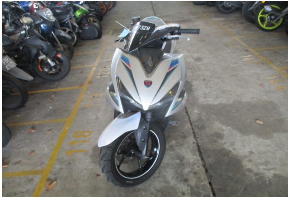
Photo 22 shows the front wheel of the Motorcycle turned towards its full right. Turning the Motorcycle's handle bar towards the left and right did not produce any abnormal free play and/or resistance. This would indicate that the steering system of the Motorcycle was in serviceable condition at the time of our inspection.
