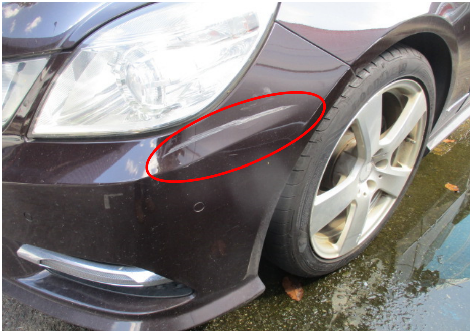
Photo 4 shows a closer view of the grazed front bumper of the Motor Car at the time of our inspection (circled).
