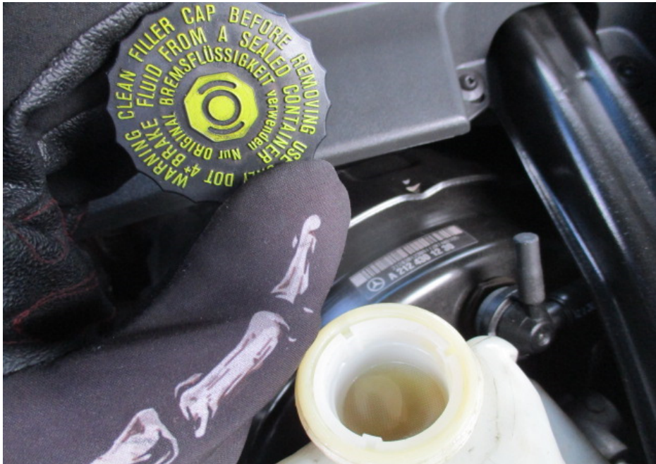
Photo 11 shows the brake fluid reservoir of the Motor Car at the time of our inspection. The brake fluid was observed to be of sufficient level and without any visible contamination.
