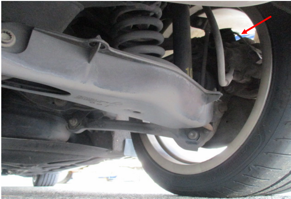
Photo 14 shows the brake hose/pipe (arrowed) at the rear right wheel of the Motor Car. We did not observe any leakage of brake fluid at the time of our inspection of the Motor Car. Static tests of the Motor Car's braking system had indicated that there was no internal leakage of pressure/vacuum. Hence the braking system was likely to be in serviceable condition at the material time of accident. The undercarriage components of the Motor Car were also all found to be intact and without any visible damage.
