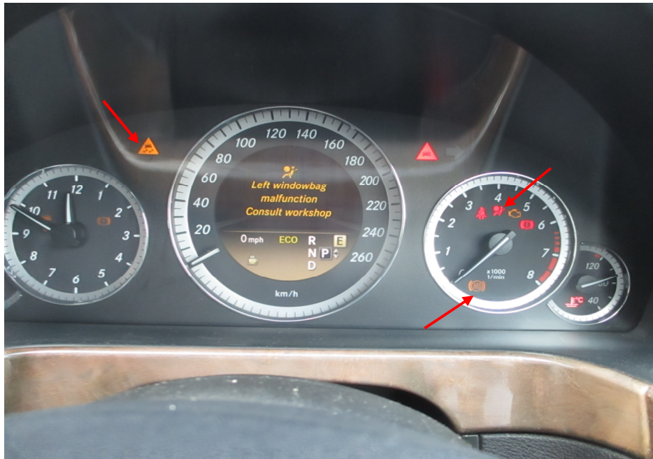
Photo 20 shows the warning lights for the various electronic operating systems of the Motor Car appearing on its instrument panel during the self-test when the engine is cranked, in particular the ABS light, ESC light and SRS light (arrowed).
