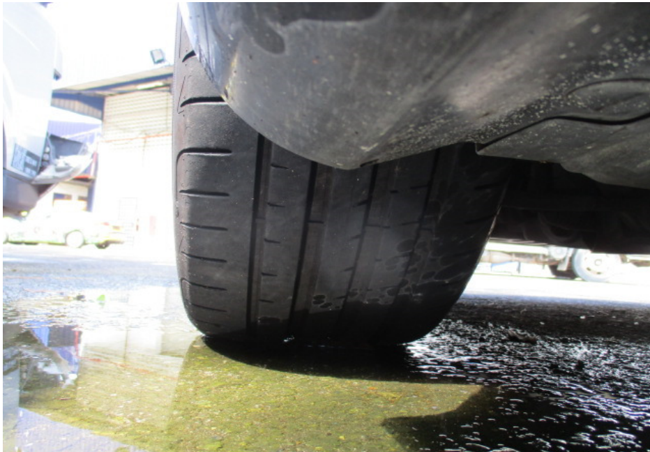
Photo 6 shows the condition of the front left tyre of the Motor Car, which was observed to be in serviceable condition with remaining tread depth of approximately 5mm. The tyre, which was wrapped around alloy wheel rim, was also observed to be sufficiently inflated for vehicular operation. There was no tear, cut or burst mark(s) on the outer and the inner sidewalls as well as across the tread of the 4 tyres.
