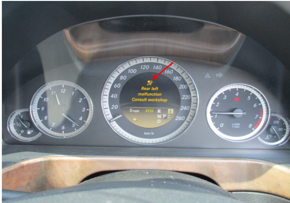
Photo 21 shows no warning lights illuminated on the instrument panel of the Motor Car after the engine was cranked. This would suggest that there was no abnormality to the various electronic operating systems of the Motor Car, like the ABS, ESC and SRS etc. The left window bag SRS warning light had however remained illuminated after the self-test (arrowed). This was due to the activation of the left front passenger and left rear passenger airbags as a result of the accident.
