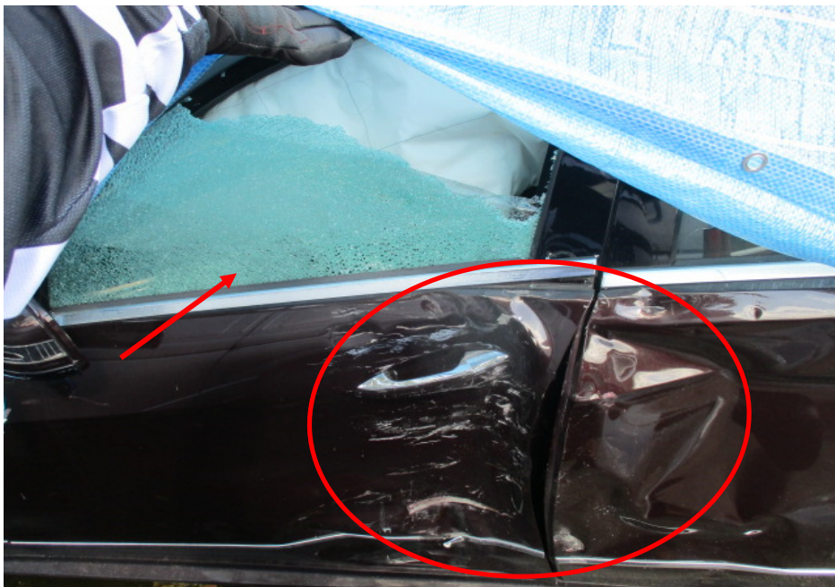
Photo 5 shows a closer view of the shattered left front passenger door glass (arrowed) as well as the dented left front and rear passenger doors (circled) of the Motor Car at the time of our inspection.
