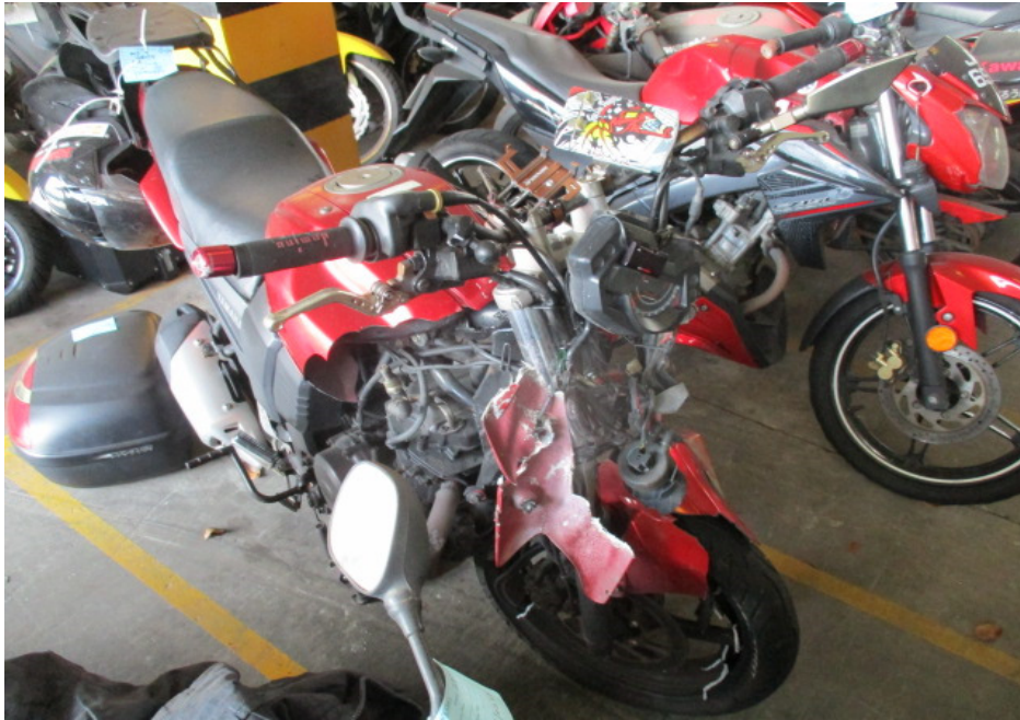
Photo 2 shows a general view of the right front body of the Motorcycle at the time of our inspection. Body parts that were found to have been damaged include its headlamp assembly, front fork assembly, front wheel rim, side mirrors, clutch lever, fuel tank, right rear side cover, rear brake pedal and exhaust muffler, amongst others.
