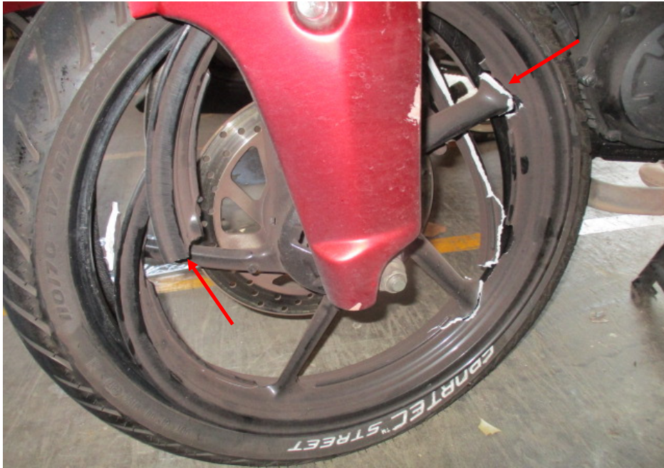
Photo 14 shows the broken front wheel rim of the Motorcycle at the time of our inspection (arrowed).
