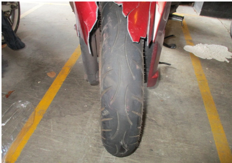
Photo 13 shows the front tyre of the Motorcycle at the time of our inspection. The pattern of the tread was clearly visible with remaining tread depth of approximately 3mm. We did not observe any tear, burst mark(s) and/or punctured hole(s) on the sidewalls as well as across the tread of the front tyre. However we did observe that the front tyre was deflated due to the broken front wheel rim.
