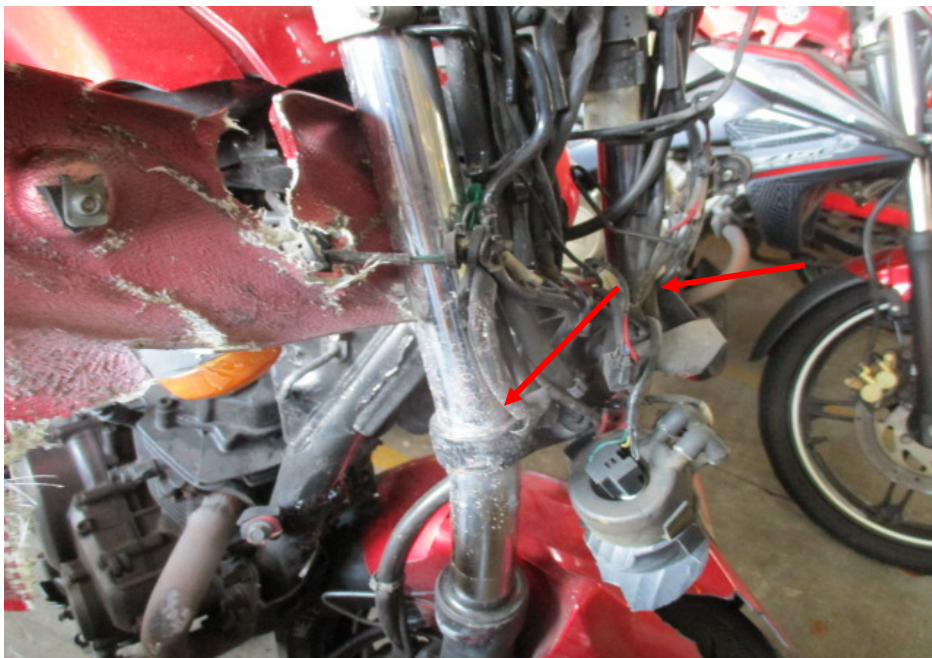
Photo 5 shows a closer view of the front forks (arrowed) which were amongst the body parts at the front body of the Motorcycle that had sustained damage as a result of the accident.
