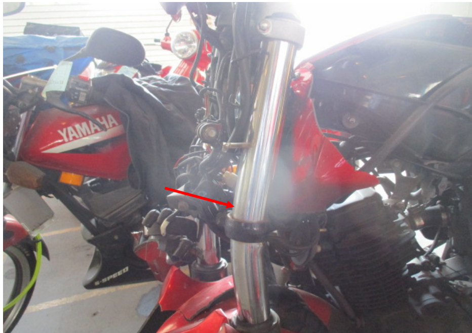
Photo 20 shows the front left fork of the Motorcycle. The front left fork was observed to be bent as a result of the accident (arrowed). We were hence not able to conduct any tests on the steering system of the Motorcycle.
