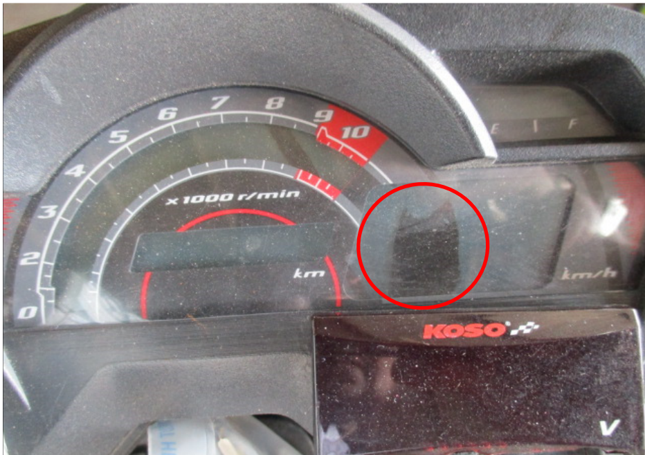
Photo 3 shows the speedometer gauge of the Motorcycle. The mileage of the Motorcycle could not be recorded at the time of our inspection due to the damages sustained to the speedometer gauge (circled).
