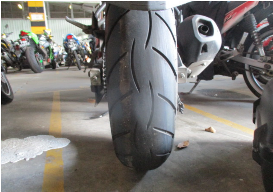
Photo 15 shows the condition of the Motorcycle's rear tyre. The pattern of the tread was clearly visible with remaining tread depth of approximately 3mm. We did not observe any tear, burst mark(s) and/or punctured hole(s) on the sidewalls as well as across the tread of the rear tyre.
