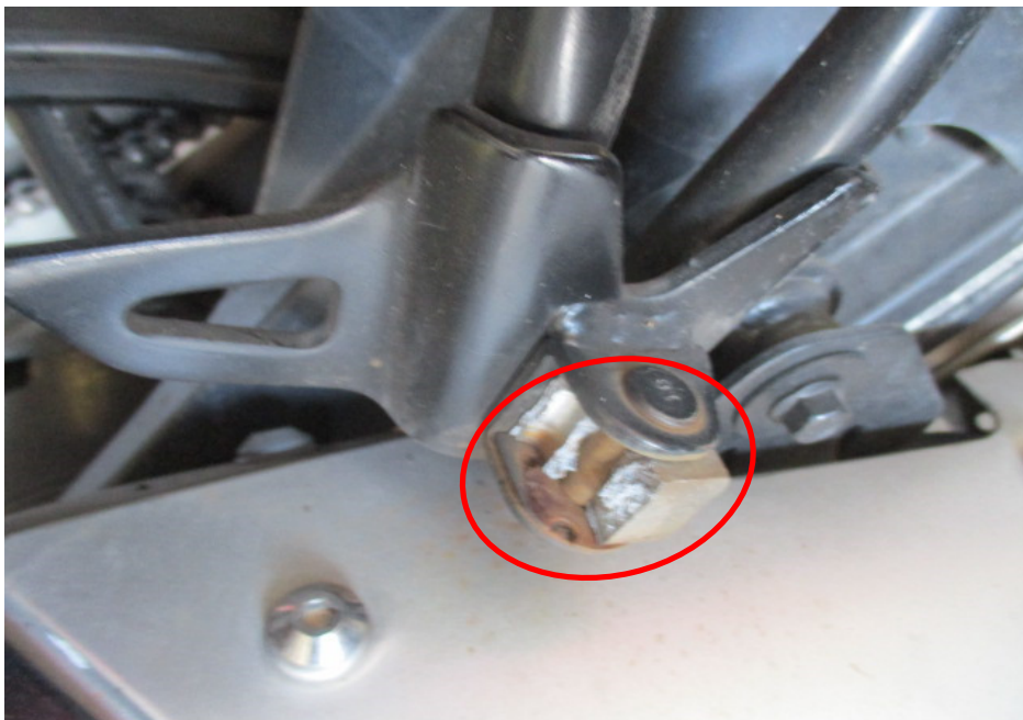
Photo 11 shows a closer view of the broken right pillion footrest which was amongst the body parts of the Motorcycle that had sustained damage as a result of the accident (circled).
