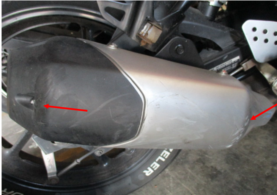
Photo 12 shows the exhaust muffler of the Motorcycle which had sustained damage as a result of the accident (arrowed).
