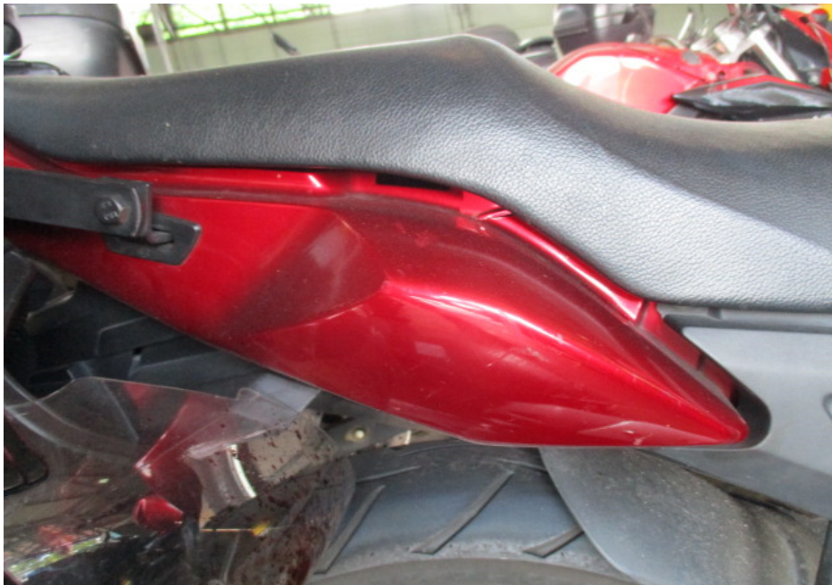
Photo 9 shows a closer view of the right rear side cover, which was amongst the body parts of the Motorcycle that had sustained damages of grazing nature as a result of the accident.
