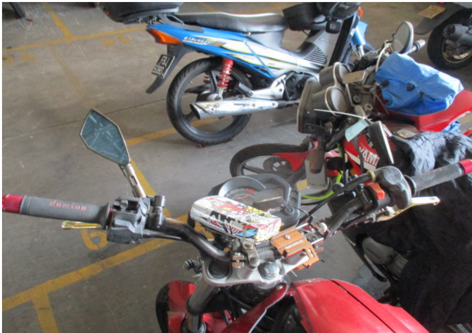
Photo 7 shows a closer view of the side mirrors, clutch lever, front brake lever, handlebars, handlebar grips and handlebar ends of the Motorcycle. These parts were amongst the body parts of the Motorcycle which were damaged as a result of the accident.
