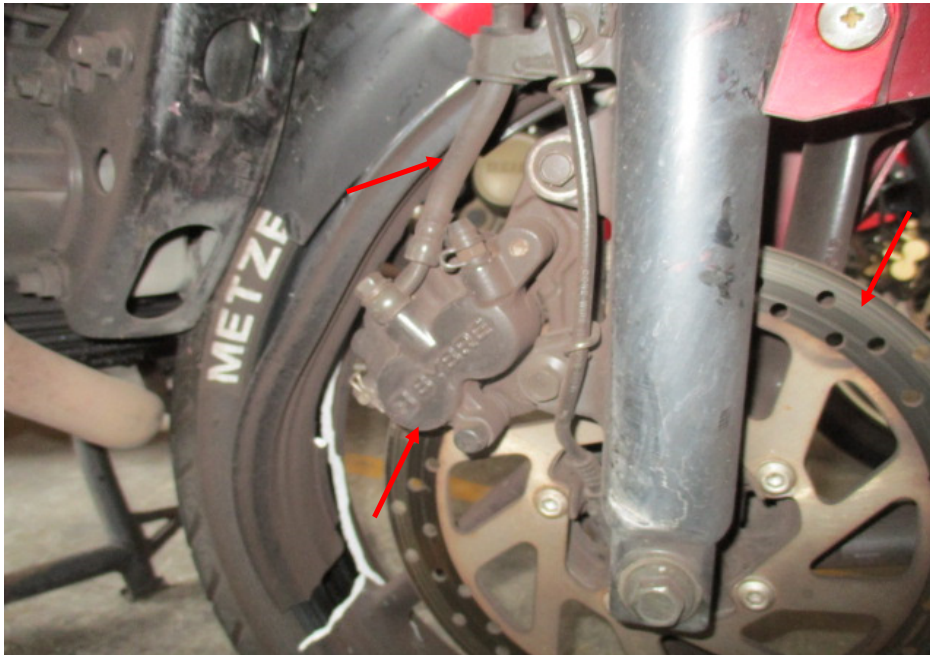
Photo 21 shows a close up view of the front brake caliper, front brake disc and front brake hose (arrowed) of the Motorcycle, which are all part of the components in the hydraulic front brake system of the Motorcycle. Our visual checks of these various components had revealed all to be intact with no visible damage. No leakage of brake fluid was also observed.
