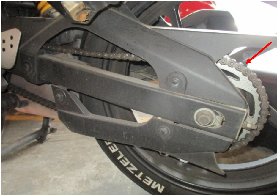
Photo 18 shows the gear chain (arrowed) of the Motorcycle, which was observed to be intact with no misalignment. It was also adequately lubricated for operating purposes. The gear chain rotates the rear wheel of the Motorcycle.
