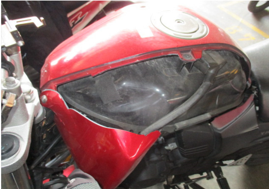
Photo 8 shows a closer view of the petrol tank which was amongst the body parts of the Motorcycle that had sustained damage as a result of the accident.
