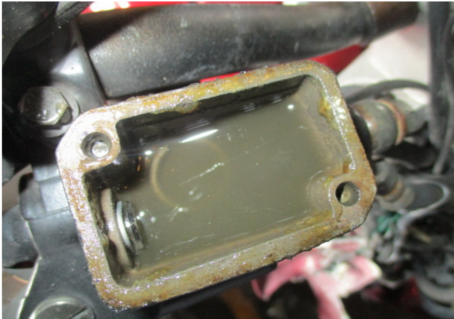
Photo 22 shows the brake fluid reservoir for the front brake of the Motorcycle. The brake fluid was observed to be without contamination and of sufficient level for operational purposes.
