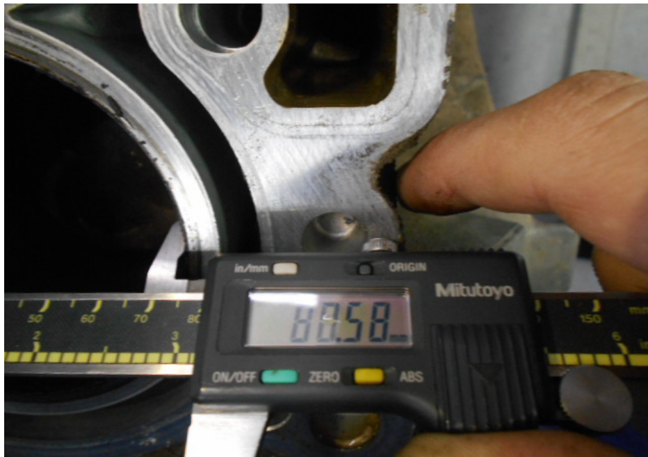
Photo 19 shows the bore measurement of cylinder 4, which was recorded to be 80.58mm.
