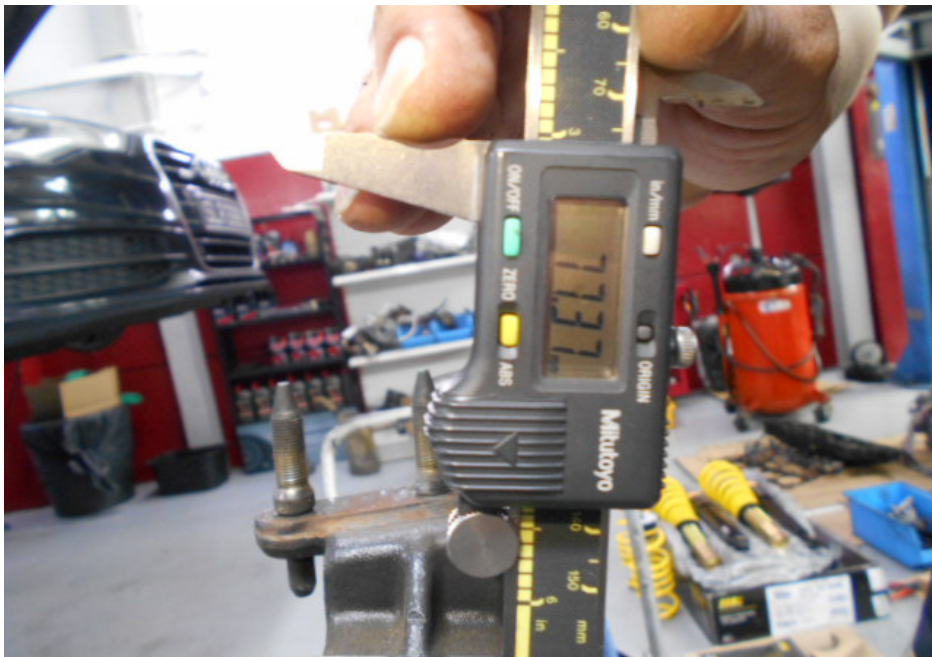
Photo 10 shows the stroke measurement of cylinder 1, which was recorded to be 77.37mm.
