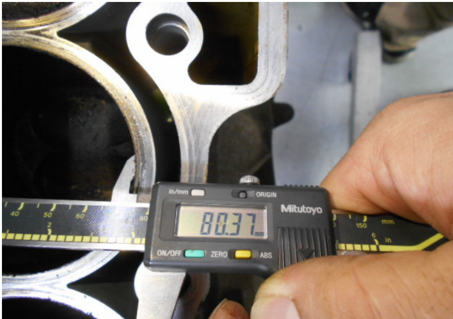
Photo 12 shows the bore measurement of cylinder 2, which was recorded to be 80.37mm.
