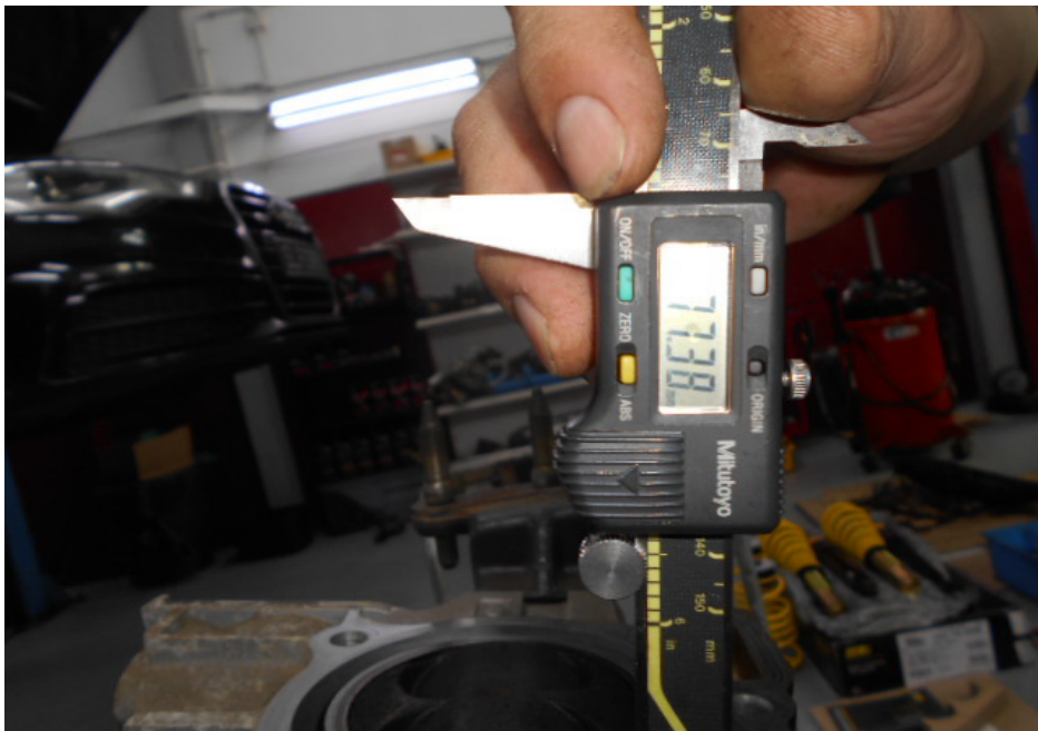
Photo 14 shows the stroke measurement of cylinder 2, which was recorded to be 77.38mm.
