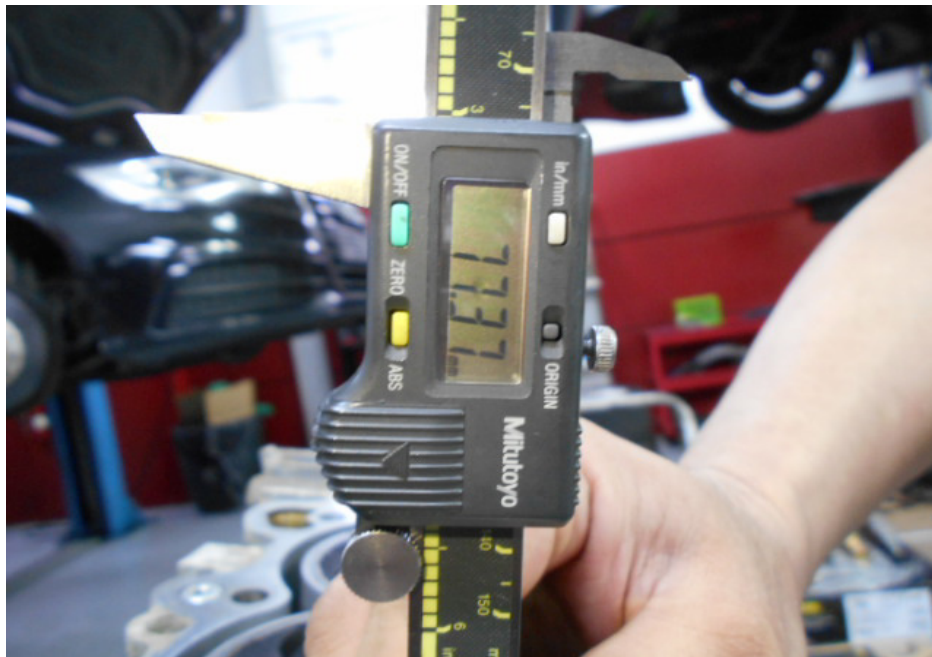
Photo 21 shows the stroke measurement of cylinder 4, which was recorded to be 77.37mm.
