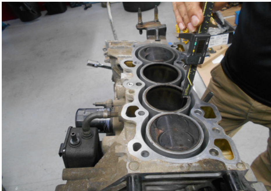
Photo 16 shows measurement of the stroke (arrowed) of cylinder 3 of the Honda engine that I had inspected. The stroke measurement of cylinder 3, which was recorded to be 77.29mm.
