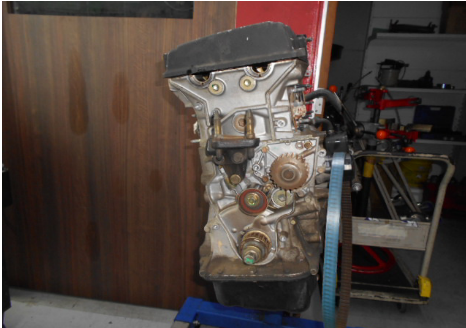
Photo 3 shows a general view of the Honda engine that I had inspected. My visual examination of the engine housing revealed the housing to be of serviceable/satisfactory condition. There was no crack and/or hole observed on the engine housing.
