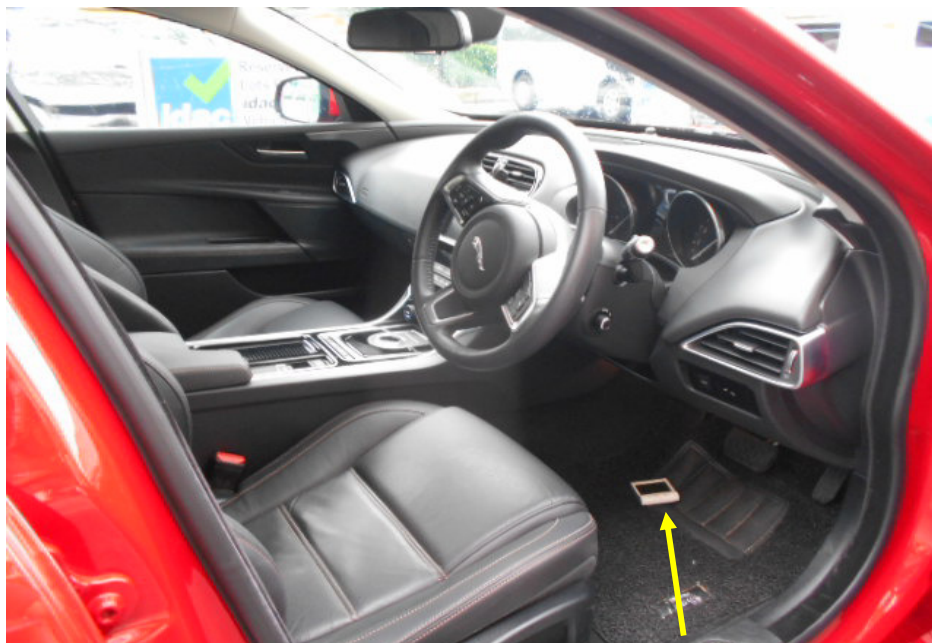
Photo 6 shows the digital temperature gauge placed at the driver footwell area of the Motor Car. Temperatures at the driver and front left passenger footwell areas were periodically checked during the test drive of the Motor Car. The temperature of the air-conditioning system of the Motor Car was set to the range of 20°C to 23°C, which is around the 22°C to 23°C temperature range that Mr Kung would usually set whilst driving the Motor Car.
