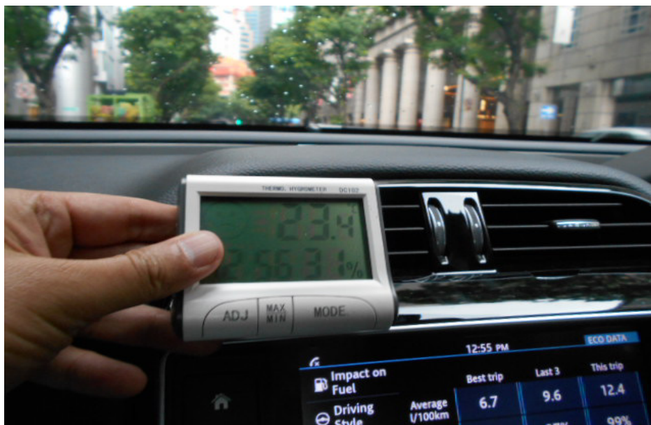
Photo 8 shows the digital temperature gauge placed near the front of the upper air-conditioning vents at the centre of the front dashboard. This was to check on the accuracy of the temperature displayed by the gauge. At the 22°C temperature that was set for the Motor Car's air-conditioning system, the temperature displayed by the gauge was 23.4°C. This would indicate that the temperature gauge was in a normal working condition and that temperatures displayed by the temperature gauge are relatively accurate.
