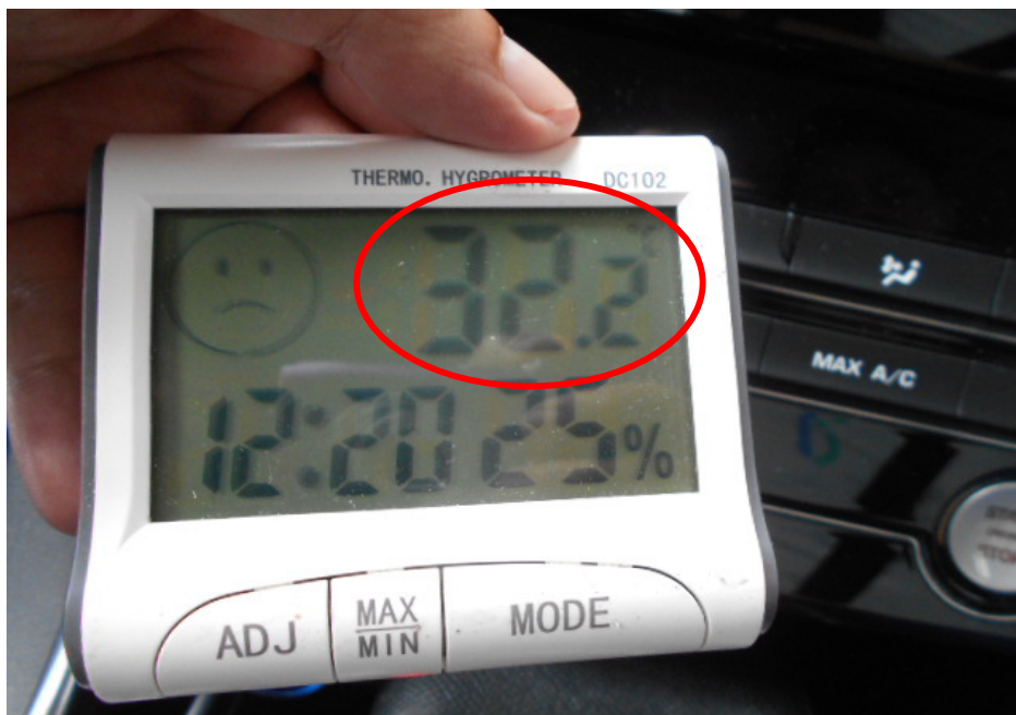
Photo 10 shows the temperature (circled) displayed by the temperature gauge at the driver footwell area. Generally, it was observed that although the Motor Car's air-conditioning system was in the range of 20°C to 23°C, the temperature at the driver footwell area was in the above 30°C range throughout my test drive of the Motor Car.
