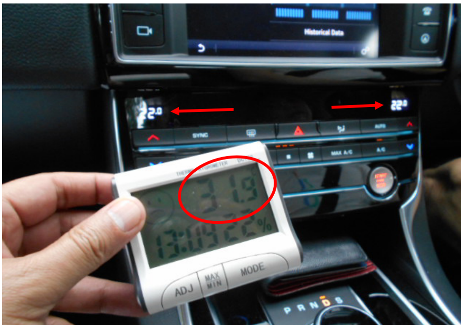
Photo 12 shows the temperature (circled) displayed by the temperature gauge at the front left passenger footwell area. Generally, it was observed that the temperature at the driver footwell area was in the above 30°C range during my test drive of the Motor Car. The temperature of the Motor Car's air-conditioning system can be seen to be at 22°C (arrowed).
