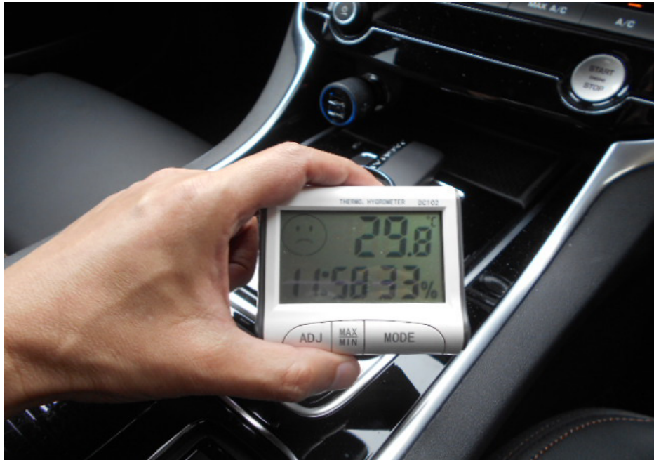
Photo 5 shows the digital temperature gauge that was used to verify the complaint of hot air being blown from the air-conditioning vents at the driver and front left passenger footwell area of the Motor Car during a test drive that was carried out on 06 June 2019.
