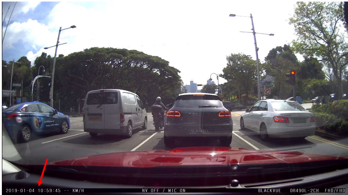
Photo 13 shows a screenshot extracted from one of the video recordings that were provided by Mr Kung for my review. At this time stamp of 10:59:45 on 04 January 2019 (arrowed), the front proximity sensors of the Motor Car were triggered. Beeping sounds can be heard from the video recording however from what can be seen, there was no object(s) close to the front of the Motor Car. The 3 motor vehicles ahead of the Motor Car were not close to the front of the Motor Car (entire rear portion of the 3 motor vehicles can be seen).
