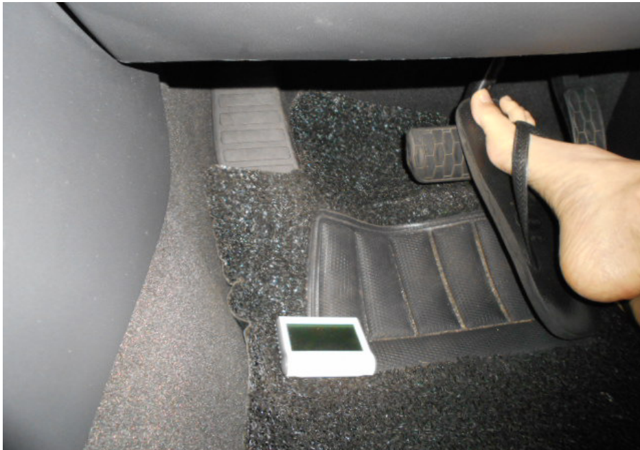
Photo 9 shows the digital temperature gauge placed near the air-conditioning vent at the driver footwell area of the Motor Car during the test drive. The temperature displayed by the temperature gauge was periodically checked and it was observed that the temperature at the driver footwell area throughout the test drive was in the above 30°C range.
