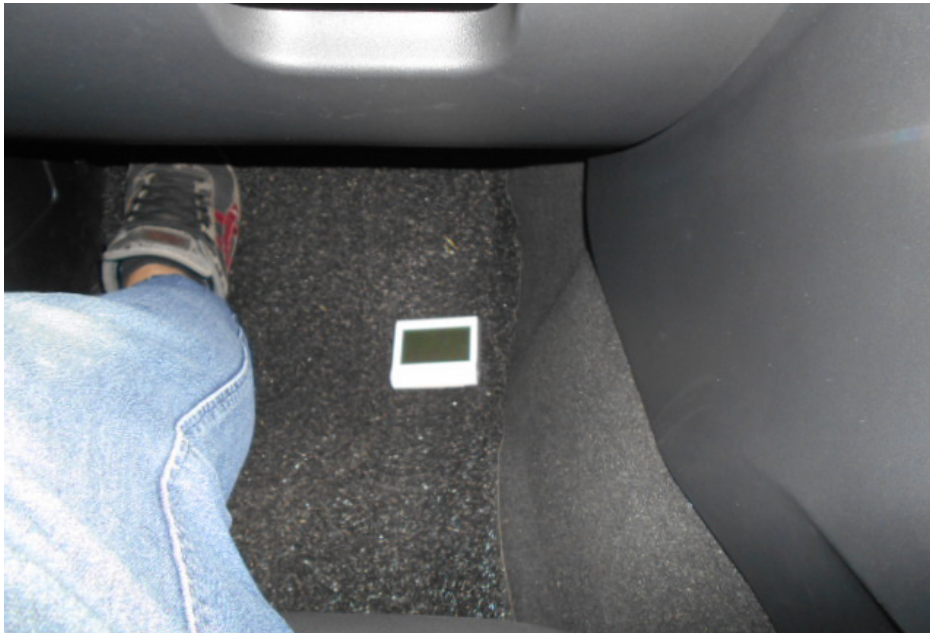
Photo 11 shows the digital temperature gauge placed near the air-conditioning vent at the front left passenger footwell area of the Motor Car during the test drive. The temperature displayed by the temperature gauge was periodically checked and it was observed that the temperature at the front left passenger footwell area was in the above 30°C range, similar to the temperature at the driver footwell area of the Motor Car.
