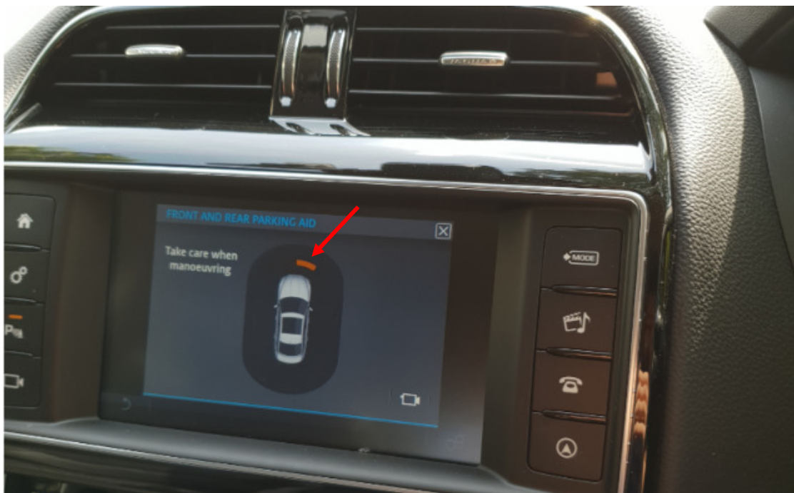
Photo 14 shows the infotainment screen of the Motor Car at the time when the front proximity sensors of the Motor Car was triggered as per photograph 13 above. The indication (arrowed) of the illustration shows an object(s) that is close to the front right of the Motor Car. However as seen from photograph 13 above, there was no object(s) close to the front right of the Motor Car.
