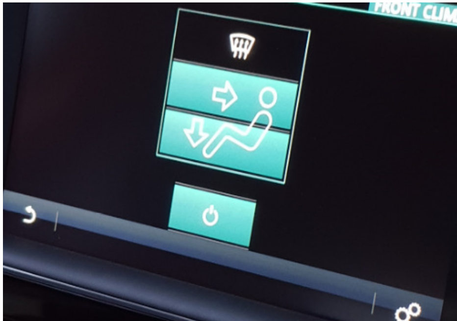
Photo 7 shows the default air-distribution settings, with both the upper (face distribution) and lower (body/feet distribution) areas selected during the test drive on 06 June 2019.
