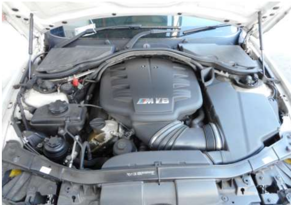
Photo 12 shows a general view of the Motor Car's engine compartment, which was accessed by lifting the front cabin of the Motor Car. The various parts and components inside the engine compartment were unaffected by the accident. There was also no sign(s) or indication(s) of fresh fluid leakage, however there was old fluid stain observed at the engine cover within the engine compartment
