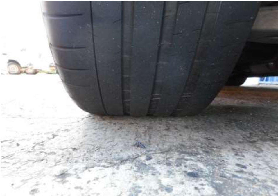
Photo 10 shows the condition of the rear left tyres of the Motor Car, which was observed to be in serviceable condition with remaining tread depth of approximately 3.9mm. The tyres, which were wrapped around standard alloy wheel rim, were also observed to be sufficiently inflated for vehicular operation. There was also no damage found on all 4 alloy wheel rims of the Motor Car.
