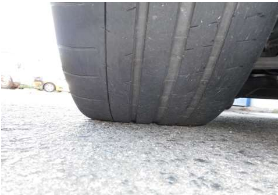
Photo 11 shows the condition of the rear right tyres of the Motor Car, which were observed to be in serviceable condition with remaining, tread depth of approximately 6.6mm. There was also no tear, cut or burst mark(s) on the outer and the inner sidewalls as well as across the tread of the 4 tyres that were fitted on the Motor Car.
