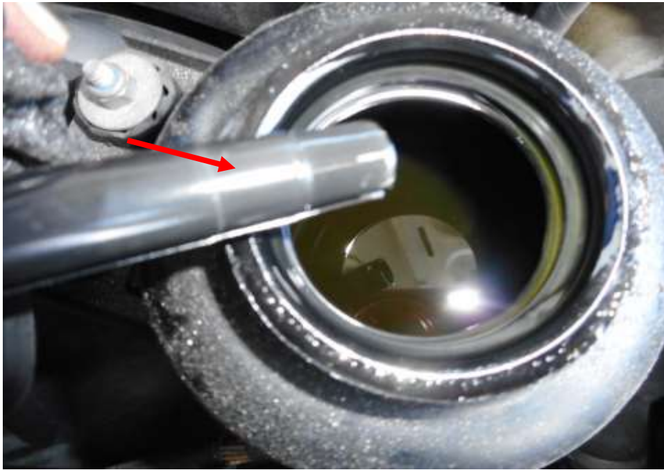
Photo 15 shows the power steering dipstick and reservoir of the Motor Car at the time of my inspection. The steering fluid was observed to be of sufficient level (arrowed) and without any visible contamination.
