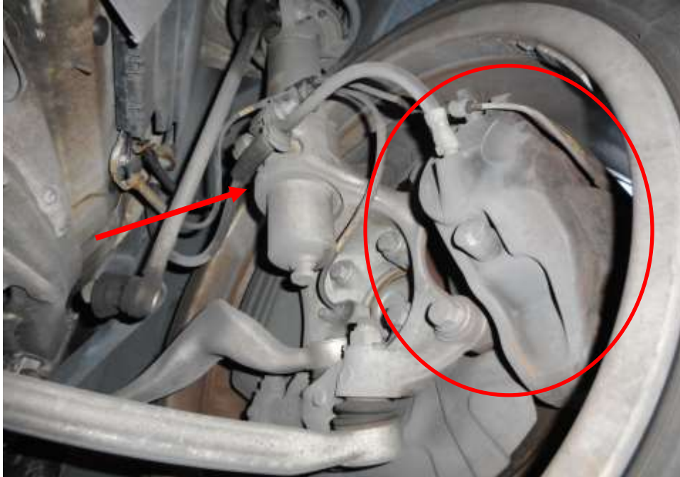
Photo 22 shows the brake hose/pipe (arrowed) at the front right wheel of the Motor Car. No leakage of brake fluid was observed. Visual examination of the various components of the braking system like the brake caliper (circled), brake booster, brake pedal etc had revealed all to be intact and without visible damage at the time of accident. There was also no sign of fluid stain(s) observed on the various undercarriage components.
