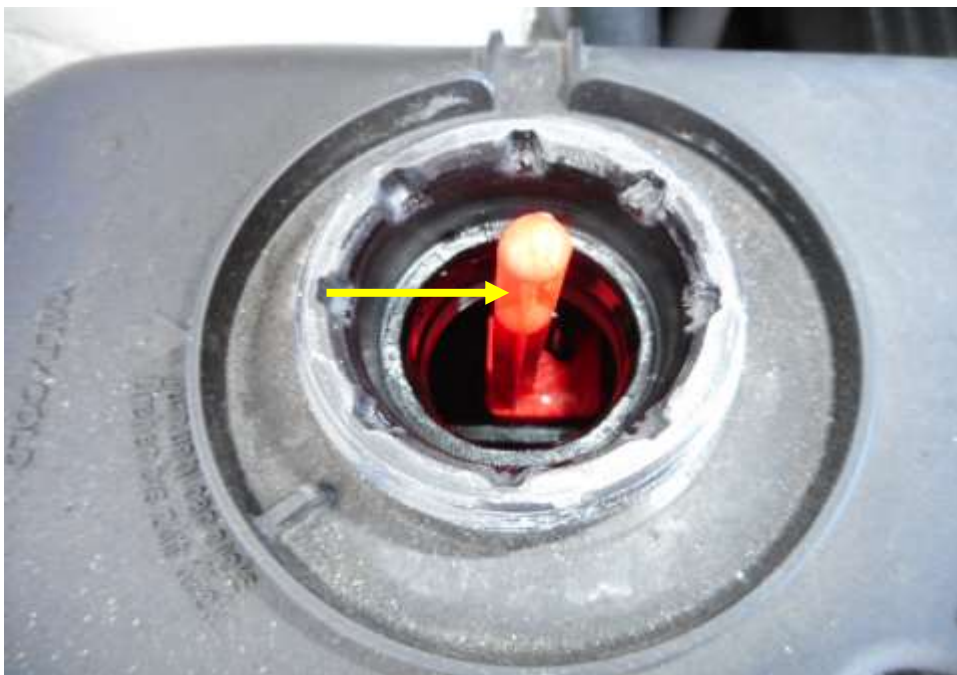
Photo 14 shows the engine coolant reservoir of the Motor Car at the time of my inspection. The engine coolant was observed to be of sufficient level (arrowed) and without any visible contamination.
