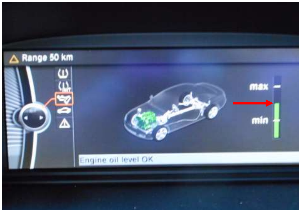
Photo 16 shows the engine level of the Motor Car at the time of my inspection. The engine oil was observed to be of sufficient level (arrowed) and without any visible contamination.
