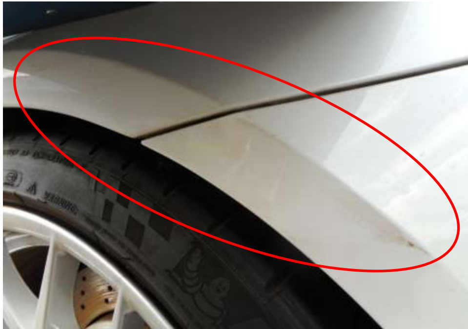
Photo 4 shows a close up view of the left body of the Motor Car at the time of my inspection. Its rear left wheel fender (circled) was damaged as a result of the accident.
