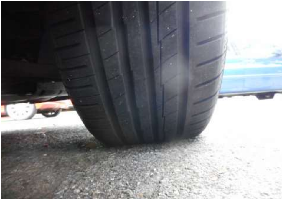
Photo 8 shows the condition of the front right tyre of the Motor Car, which was observed to be in serviceable condition with remaining tread depth of approximately 4.7mm. The tyre, which was wrapped around standard alloy wheel rim, was also observed to be sufficiently inflated for vehicular operation. There was no tear, cut or burst mark(s) on the outer and the inner sidewalls as well as across the tread of the 4 tyres that were fitted on the Motor Car.
