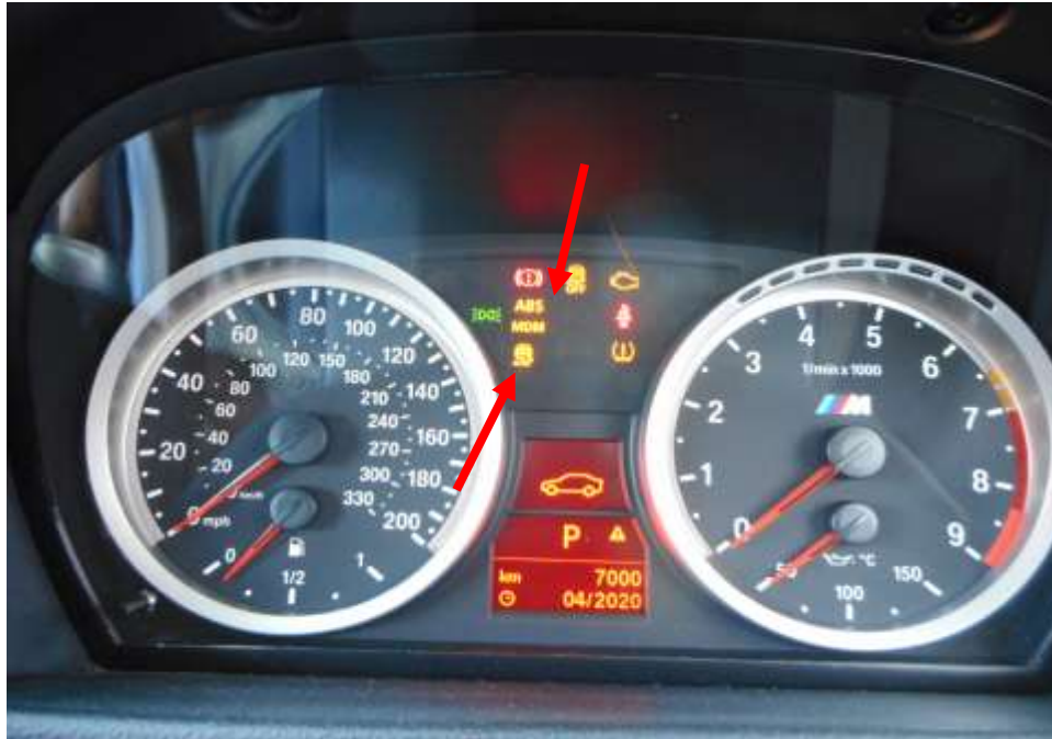
Photo 25 shows the warning light for Anti-Lock Brake System (ABS) and Traction Control System (TC) appearing on the instrument panel of the Motor Car during the self-test of its various electronic operating systems when its engine was cranked.
