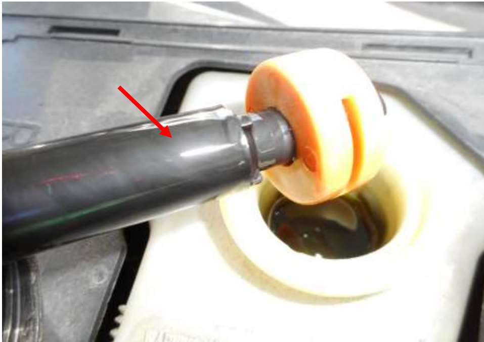
Photo 13 shows the brake fluid reservoir of the Motor Car at the time of my inspection. The brake fluid was observed to be of sufficient level (arrowed) and without any visible contamination.
