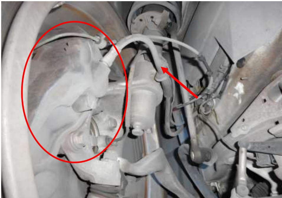
Photo 23 shows the brake hose/pipe (arrowed) at the front left wheel of the Motor Car. No leakage of brake fluid was observed. Visual examination of the various components of the braking system like the brake caliper (circled), brake booster, brake pedal etc had revealed all to be intact and without visible damage at the time of accident. There was also no sign of fluid stain(s) observed on the various undercarriage components.
