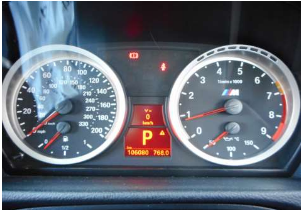
Photo 26 shows no warning lights illuminated on the instrument panel of the Motor Car after the engine was cranked. This would suggest that there was no abnormality to the various electronic operating systems of the Motor Car, like the ABS and TC...
