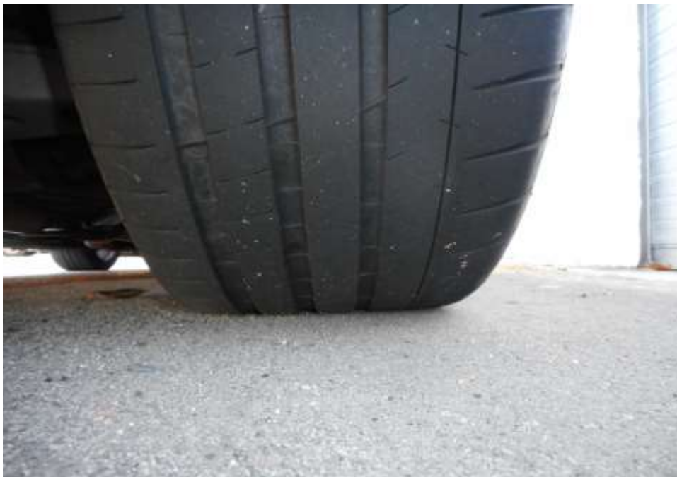
Photo 9 shows the condition of the rear right tyre of the Motor Car, which was observed to be in serviceable condition with remaining tread depth of approximately 4mm. The tyre, which was wrapped around standard alloy wheel rim, was also observed to be sufficiently inflated for vehicular operation.
