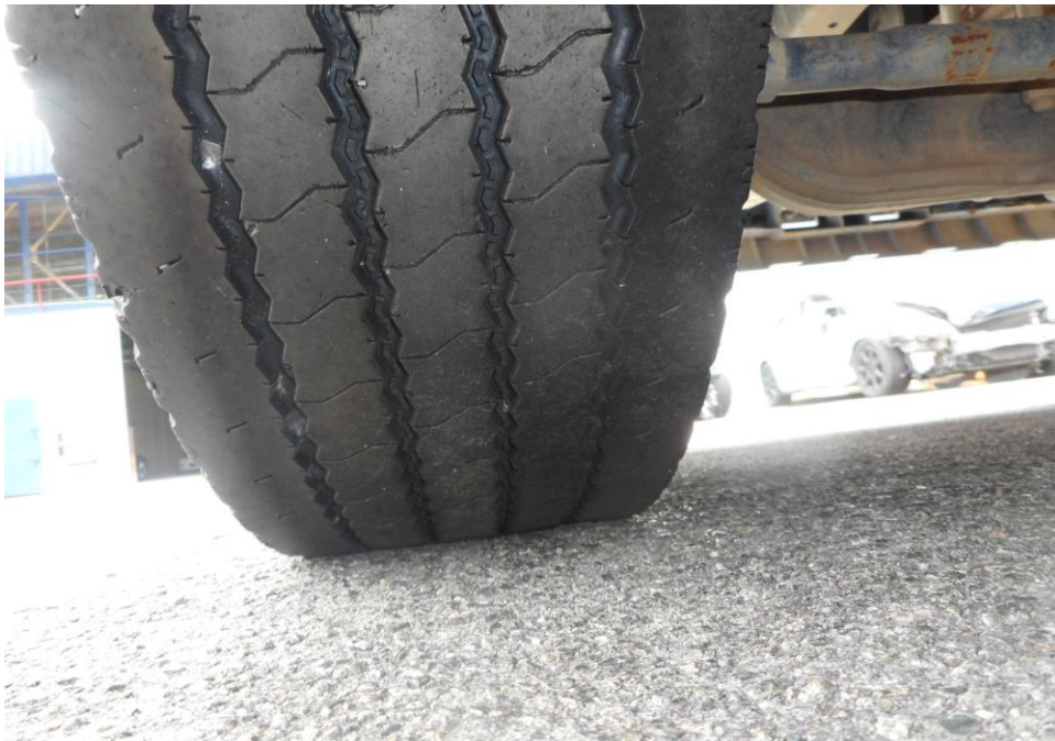
Photo 9 shows the condition of the front left tyre of the Motor Lorry, which were observed to be in serviceable condition with remaining, tread depth of approximately 4.8mm. There was also no tear, cut or burst mark(s) on the outer and the inner sidewalls as well as across the tread of the 6 tyres that were fitted on the Motor Lorry.
