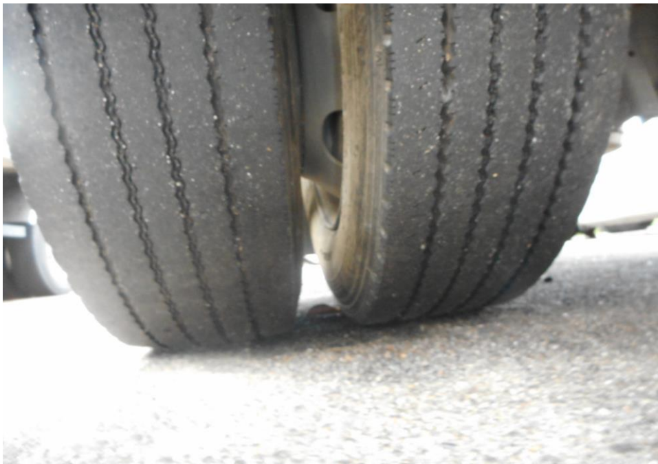
Photo 7 shows the condition of the rear right tyres of the Motor Lorry, which was observed to be in serviceable condition with remaining, tread depth of approximately 4.7mm. The tyres, which were wrapped around standard steel wheel rim, were also observed to be sufficiently inflated for vehicular operation. There was also no damage found on all 6 steel wheel rims of the Motor Lorry.
