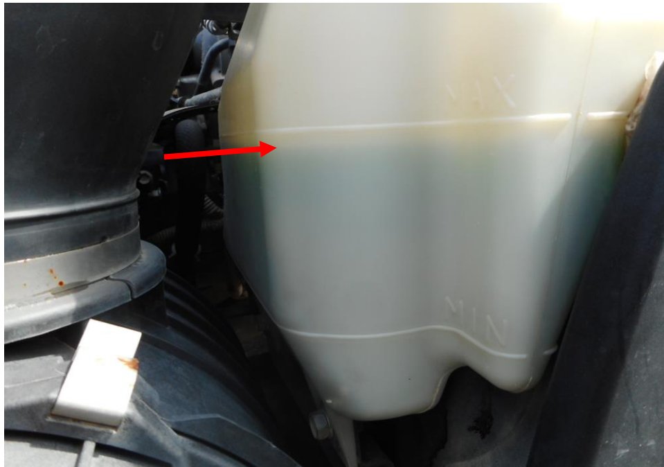
Photo 12 shows the engine coolant reservoir of the Motor Lorry at the time of my inspection. The engine coolant was observed to be of sufficient level (arrowed) and without any visible contamination.
