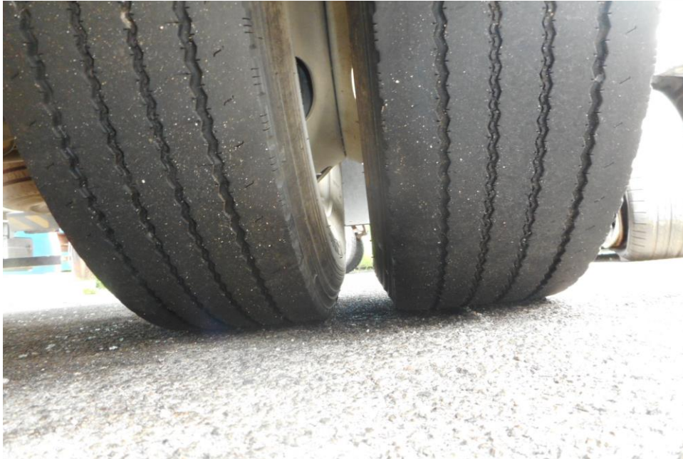
Photo 8 the condition of the rear left tyres of the Motor Lorry, which was observed to be in serviceable condition with remaining, tread depth of approximately 4.8mm. The tyres, which were wrapped around standard steel wheel rim, were also observed to be sufficiently inflated for vehicular operation. There was also no damage found on all 6 steel wheel rims of the Motor Lorry.
