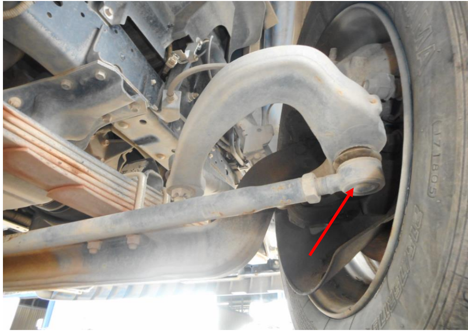
Photo 16 shows the various undercarriage components at the front right wheel of the Motor Lorry, in particular the steering tie rod end (arrowed). The various steering components were all found to be intact, suggesting that the steering system of the Motor Lorry was likely to be in serviceable condition at the material time of accident. There was also no sign of fluid stain(s) observed on the various undercarriage components.
