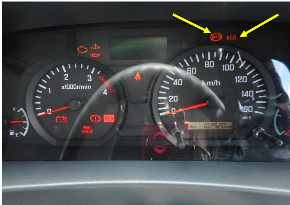
Photo 23 shows the warning light for Anti-Lock Brake System (ABS) and Traction Control System (SRS/ASR) (arrowed) appearing on the instrument panel of the Motor Lorry during the self-test of its various electronic operating systems when its engine was cranked.
