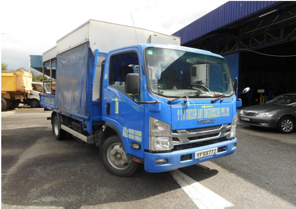
Photo 22 shows the front right wheel of the Motor Lorry turned to its full left. During my steering system test, I did not experience any abnormal free play and/or resistance when I had turned the steering wheel towards full left and full right. This would suggest that the steering system of the Motor Lorry was likely to be in serviceable condition at the material time of accident.
