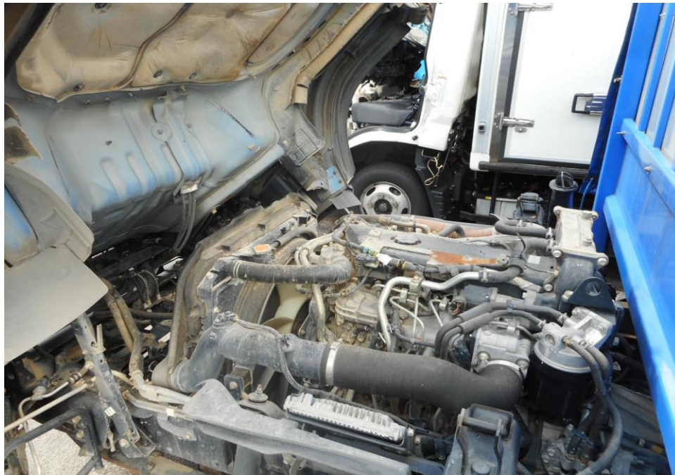
Photo 10 shows a general view of the Motor Lorry's engine compartment, which was accessed by lifting the front cabin of the Motor Lorry. The various parts and components inside the engine compartment were unaffected by the accident. There was also no sign(s) or indication(s) of fresh fluid leakage and/or fluid stain within the engine compartment
