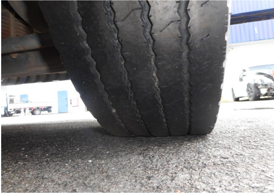
Photo 6 shows the condition of the front right tyre of the Motor Lorry, which was observed to be in serviceable condition with remaining tread depth of approximately 4.9mm. The tyre, which was wrapped around standard steel wheel rim, was also observed to be sufficiently inflated for vehicular operation. There was no tear, cut or burst mark(s) on the outer and the inner sidewalls as well as across the tread of the 6 tyres that were fitted on the Motor Lorry.
