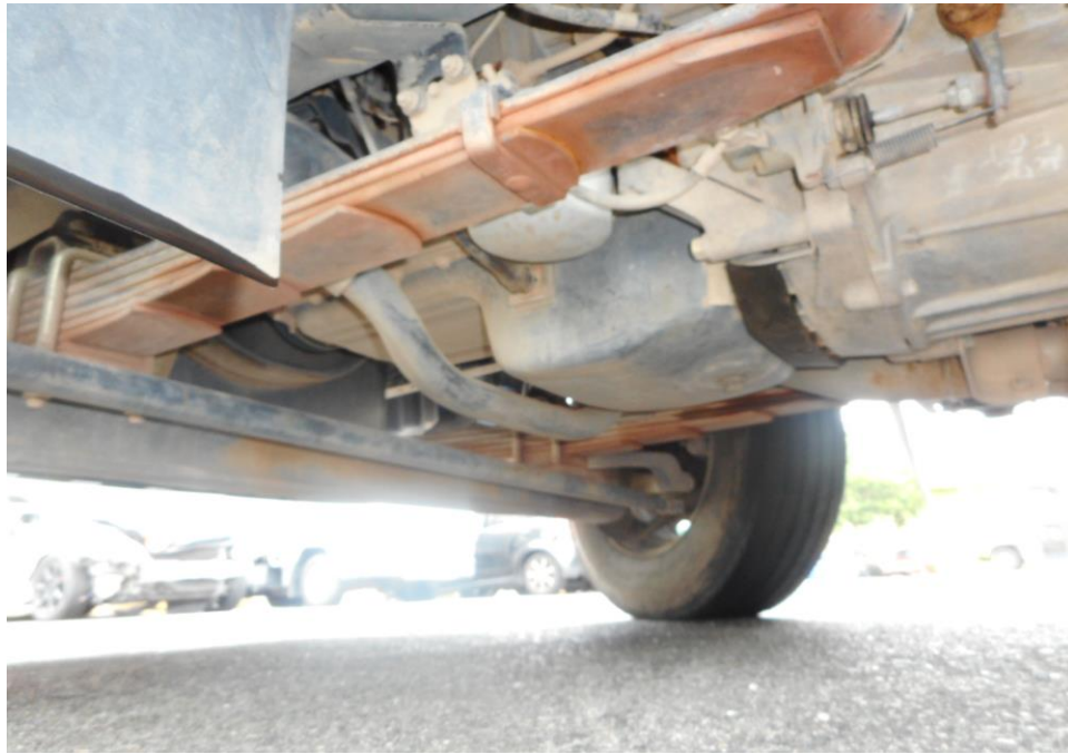
Photo 15 shows the undercarriage of the Motor Lorry, at the area where the engine housing and transmission housing are located. I did find old fluid stain on the underside of the Motor Lorry.
