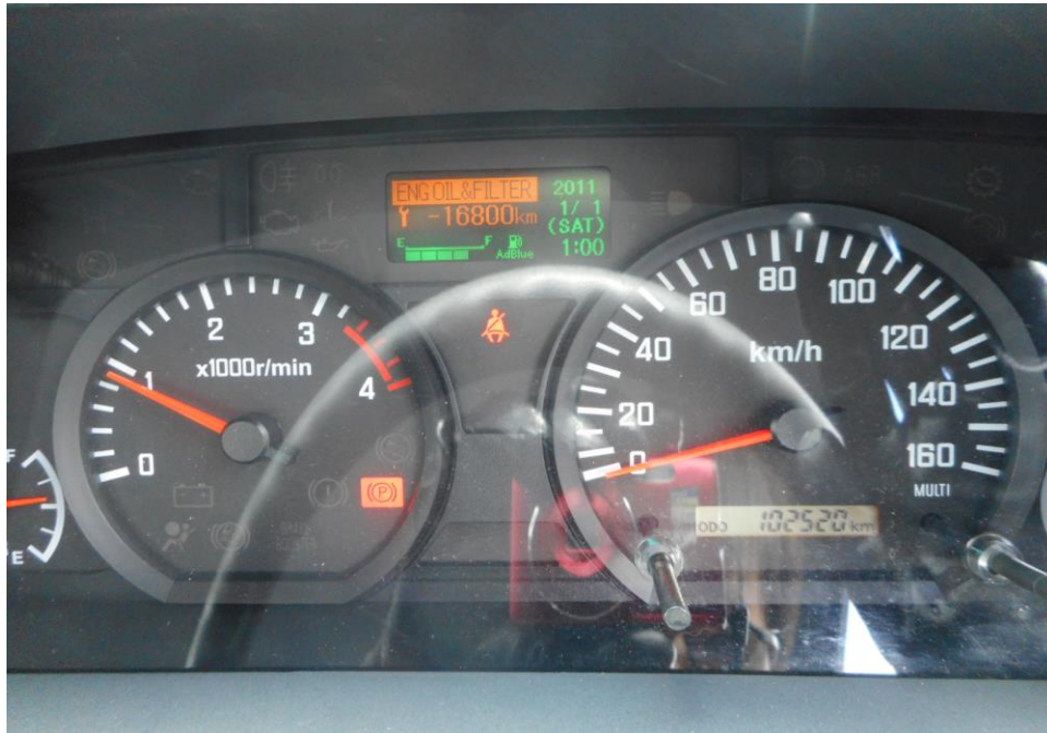
Photo 24 shows no warning lights illuminated on the instrument panel of the Motor Lorry after the engine was cranked. This would suggest that there was no abnormality to the electronic operating system of the Motor Lorry, like the ABS, TC/ASR and etc.
