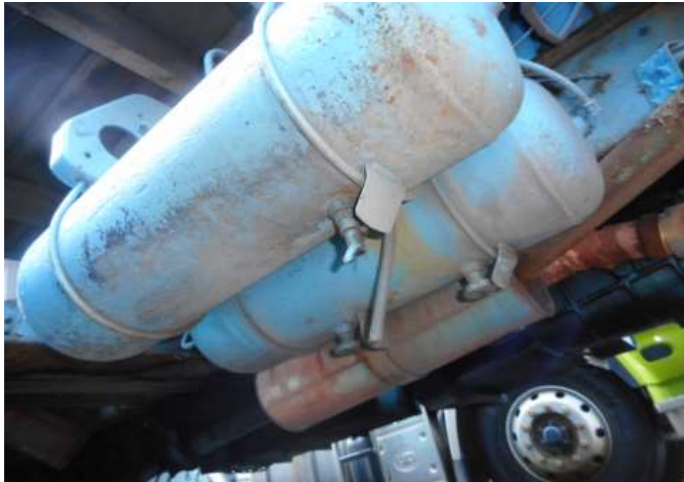
Photo 15 shows a general view of the air tank, valves, pipes and hoses, which are some of the components for the air-assisted braking system of the Motor Lorry. I was however not able to carry out any operational test(s) to the braking system of the Motor Lorry as its engine was unable to be started.
