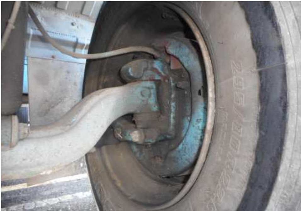
Photo 17 shows the brake air cylinder and air pipes at the front right wheel of the Motor Lorry. My visual inspection of the mechanical components of the Motor Lorry's braking system appear to suggest that its braking system was in serviceable condition at the material time of accident.
