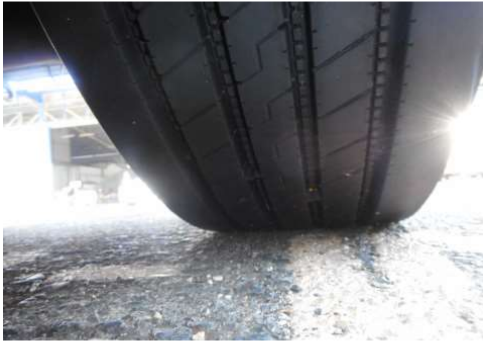
Photo 8 shows the condition of the front right tyre of the Motor Lorry, which was observed to be in serviceable condition with remaining tread depth of approximately 9.6mm. The tyre, which was wrapped around standard alloy wheel rim, was also observed to be sufficiently inflated for vehicular operation with no tear, cut or burst mark(s) on the outer and the inner sidewalls.
