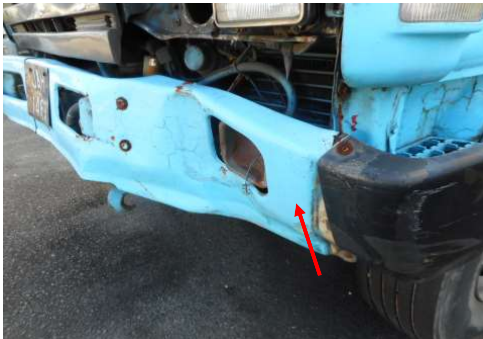
Photo 3 shows a close up view of the front body of the Motor Lorry at the time of my inspection. The Motor Lorry was observed to have sustained relatively minor impact damage at its front portion. Its front bumper (arrowed) was observed to be damaged as a result of the accident.
