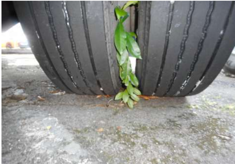
Photo 9 shows the condition of the rear left tyres of the Motor Lorry, which were observed to be in serviceable condition with remaining tread depth of approximately 7.4mm. The tyres, which were wrapped around standard alloy wheels rims, were also observed to be sufficiently inflated for vehicular operation. There was also no damage found on all the 6 alloy wheel rims of the Motor Lorry.
