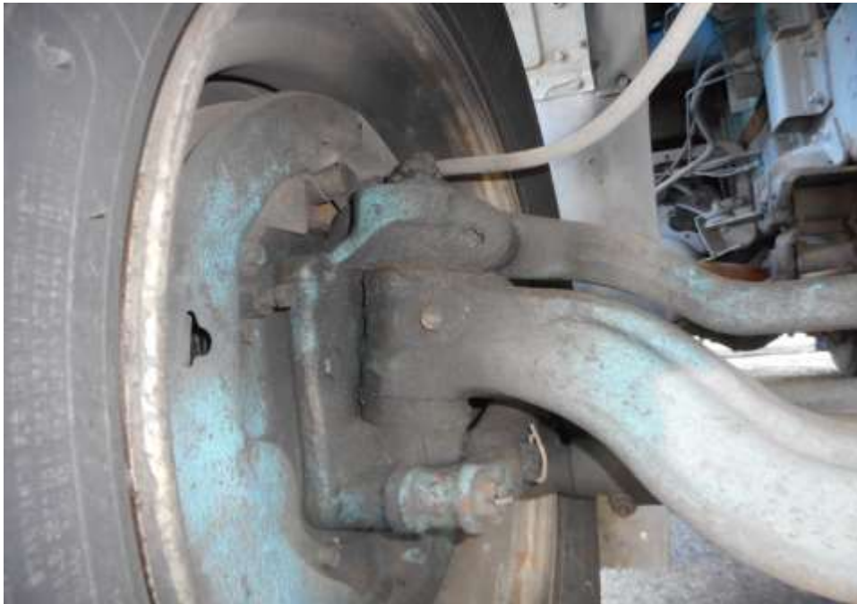
Photo 16 shows the brake air cylinder and air pipes at the front left wheel of the Motor Lorry. My visual inspection of the mechanical components of the Motor Lorry's braking system appear to suggest that its braking system was in serviceable condition at the material time of accident.
