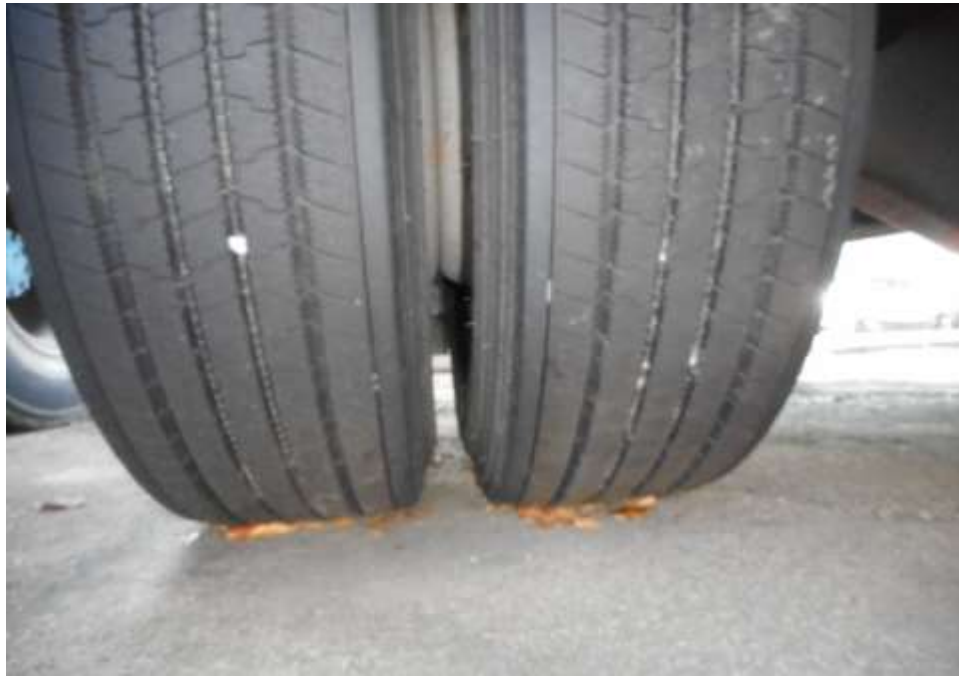
Photo 10 shows the condition of the rear right tyres of the Motor Lorry, which were observed to be in serviceable condition with remaining tread depth of approximately 8.7mm. The tyres, which were wrapped around standard alloy wheel rims, were also observed to be sufficiently inflated for vehicular operation with no tear, cut or burst mark(s) on the outer and the inner sidewalls. There was also no damage found on all the 6 alloy wheel rims of the Motor Lorry.
