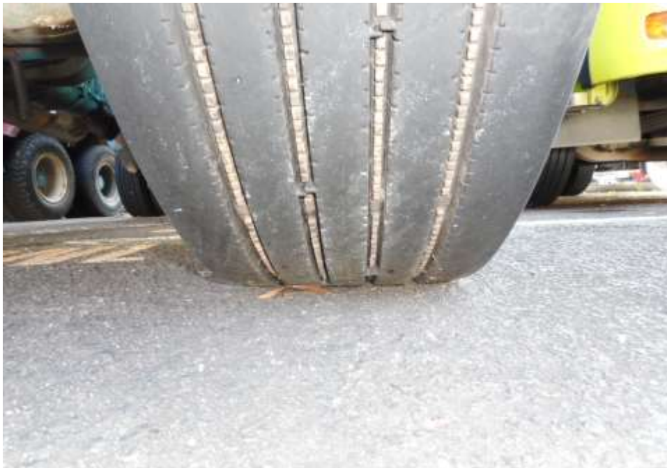
Photo 7 shows the condition of the front left tyre of the Motor Lorry, which was observed to be in serviceable condition with remaining tread depth of approximately 11mm. The tyre, which was wrapped around standard alloy wheel rim, was also observed to be sufficiently inflated for vehicular operation with no tear, cut or burst mark(s) on the outer and the inner sidewalls.
