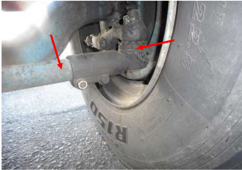
Photo 13 shows the undercarriage components at the front right wheel of the Motor Lorry. The various undercarriage components of the Motor Lorry were all observed to be intact and without any visible damage. This had included the steering rack and steering ball joints (arrowed) of the Motor Lorry. Visual examinations of the mechanical components of the steering system appear to indicate that the Motor Lorry's steering system was in serviceable condition.
