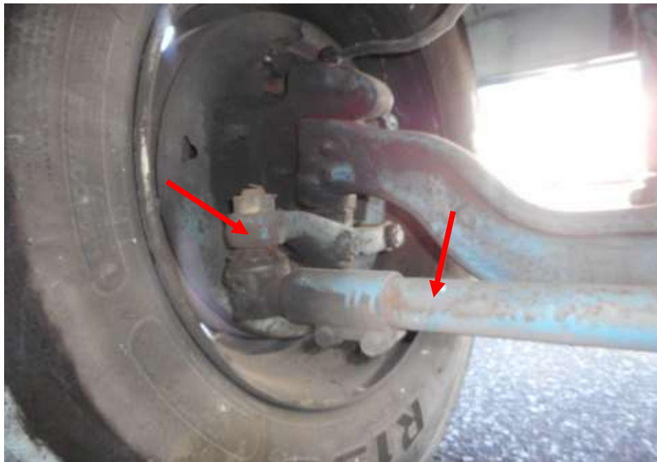
Photo 14 shows the undercarriage components at the front left wheel of the Motor Lorry. The various undercarriage components of the Motor Lorry were all observed to be intact and without any visible damage. This had included the steering rack and steering ball joints (arrowed) of the Motor Lorry, which were observed to be securely attached to the front left wheel and front right wheel.
