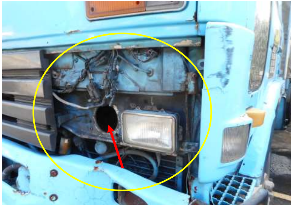
Photo 2 shows a close up view of the front body of the Motor Lorry at the time of my inspection. The Motor Lorry was observed to have sustained relatively minor impact damage at its front portion. Its front left headlight (arrowed) and front grille (circled) was observed to be damaged as a result of the accident.
