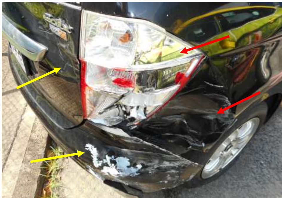
Photo 3 shows a close up view of the rear body of the Motor Car at the time of my inspection. The Motor Car was observed to have sustained damage at its rear portion. Its rear bonnet (yellow arrow), rear bumper (yellow arrow), rear right brake lamp (red arrow), rear right fender (red arrow) was amongst the body parts damaged as a result of the accident.
