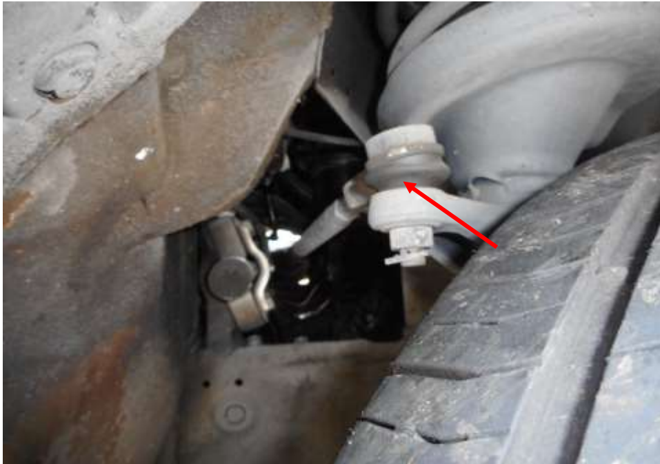
Photo 16 shows the various undercarriage components at the front right wheel of the Motor Car, in particular the steering tie rod end (red arrowed). The various steering components were all found to be intact, suggesting that the steering system of the Motor Car was likely to be in serviceable condition at the material time of accident. There was also no sign of fluid stain(s) observed on the various undercarriage components.
