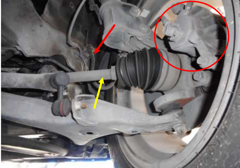
Photo 20 shows the brake hose/pipe (red arrowed) and drive shaft (yellow arrow) at the front right wheel of the Motor Car. No leakage of brake fluid was observed. Visual examination of the various components of the braking system like the brake caliper (circled), brake booster, brake pedal etc had revealed all to be intact and without visible damage at the time of accident. There was also no sign of fluid stain(s) observed on the various undercarriage components.
