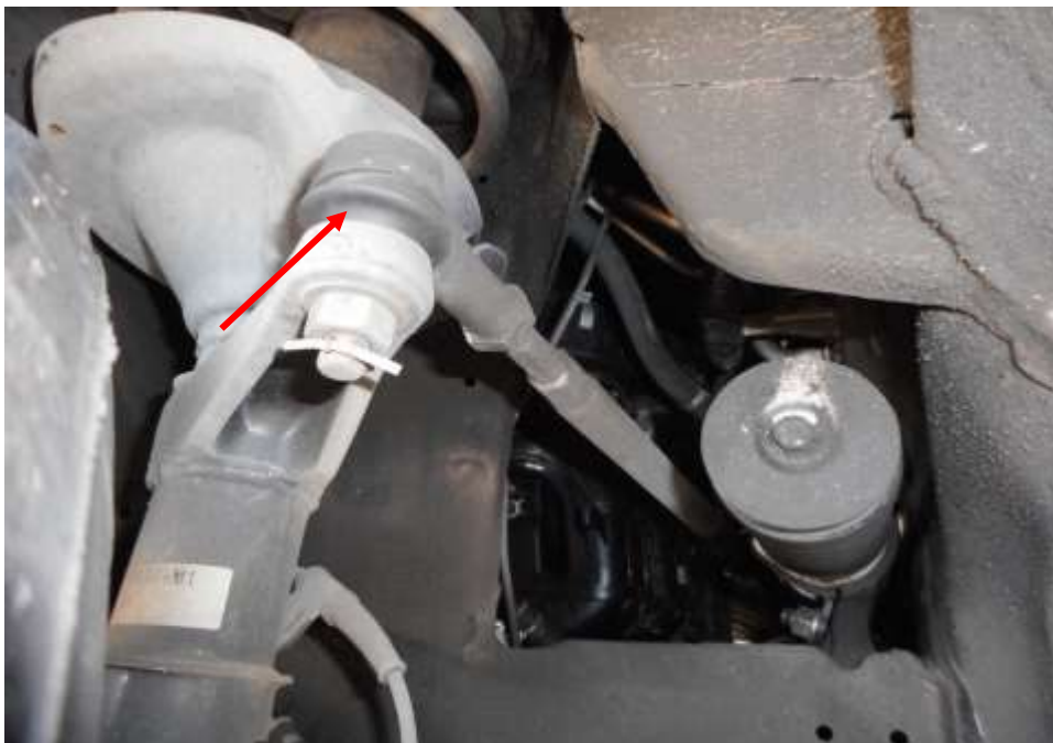
Photo 17 shows the various undercarriage components at the front left wheel of the Motor Car, in particular the steering tie rod end (arrowed). The various undercarriage components of the Motor Car were all found to be intact without any visible damage. There was also no sign of fluid stain(s) observed on the various undercarriage components.
