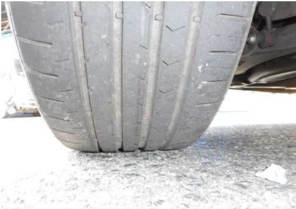
Photo 9 shows the condition of the rear right tyres of the Motor Car, which were observed to be in serviceable condition with remaining, tread depth of approximately 4.7mm. There was also no tear, cut or burst mark(s) on the outer and the inner sidewalls as well as across the tread of the 4 tyres that were fitted on the Motor Car.
