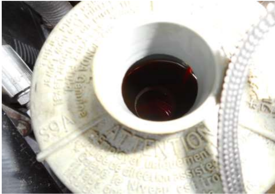
Photo 15 shows the power steering reservoir of the Motor Car at the time of my inspection. The power steering fluid was observed to be of sufficient level and without any visible contamination.
