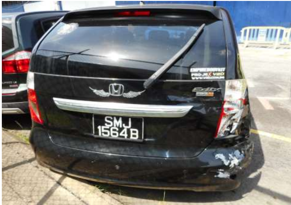
Photo 2 shows a general view of the rear body of the Motor Car at the time of my inspection. The Motor Car was observed to have sustained damage at its rear portion. Its rear bonnet, rear bumper, rear right brake lamp, rear right fender was amongst the body parts damaged as a result of the accident.
