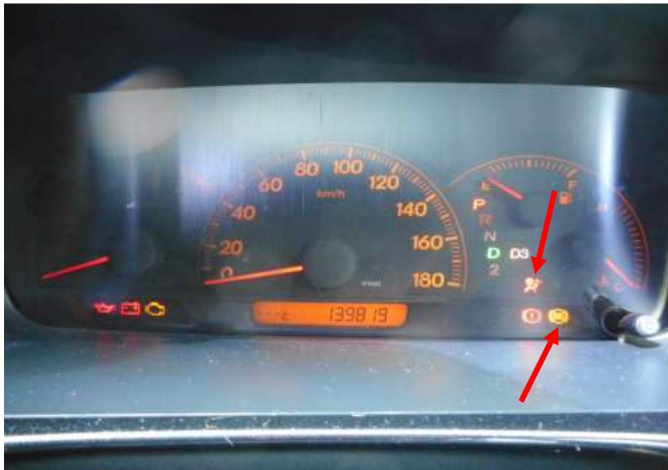
Photo 23 shows the warning light for Anti-Lock Brake System (ABS) and Supplemental Restraint System (SRS) appearing on the instrument panel of the Motor Car during the self-test of its various electronic operating systems when its engine was cranked.
