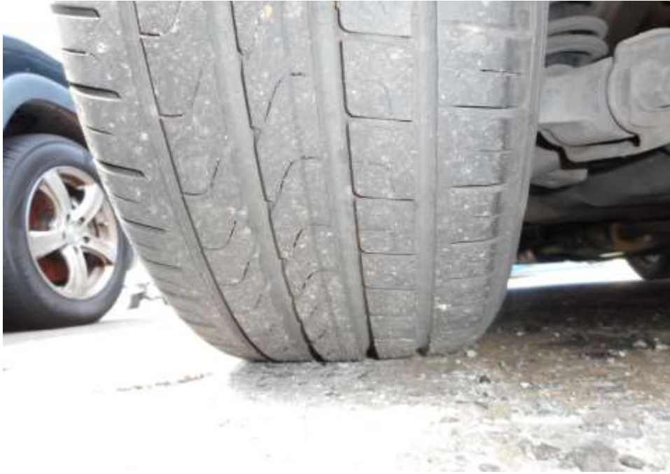
Photo 8 shows the condition of the rear left tyres of the Motor Car, which was observed to be in serviceable condition with remaining tread depth of approximately 6.4mm. The tyres, which were wrapped around standard alloy wheel rim, were also observed to be sufficiently inflated for vehicular operation. There was also no damage found on all 4 alloy wheel rims of the Motor Car.
