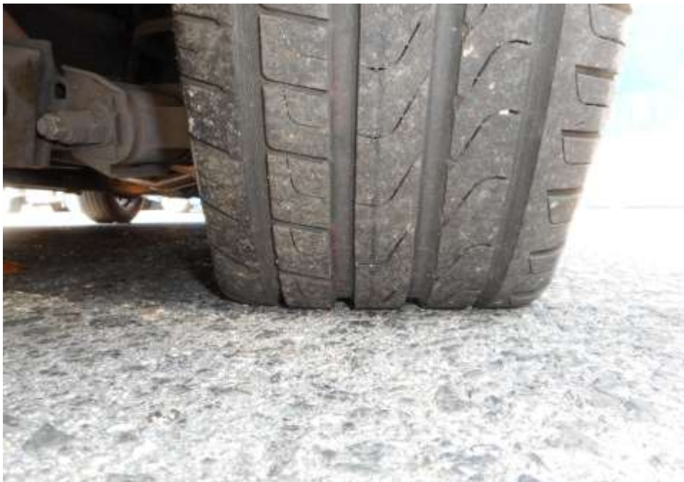
Photo 7 shows the condition of the rear right tyre of the Motor Car, which was observed to be slightly deflated however in serviceable condition with remaining tread depth of approximately 4.8mm. The tyre, which was wrapped around standard alloy wheel rim
