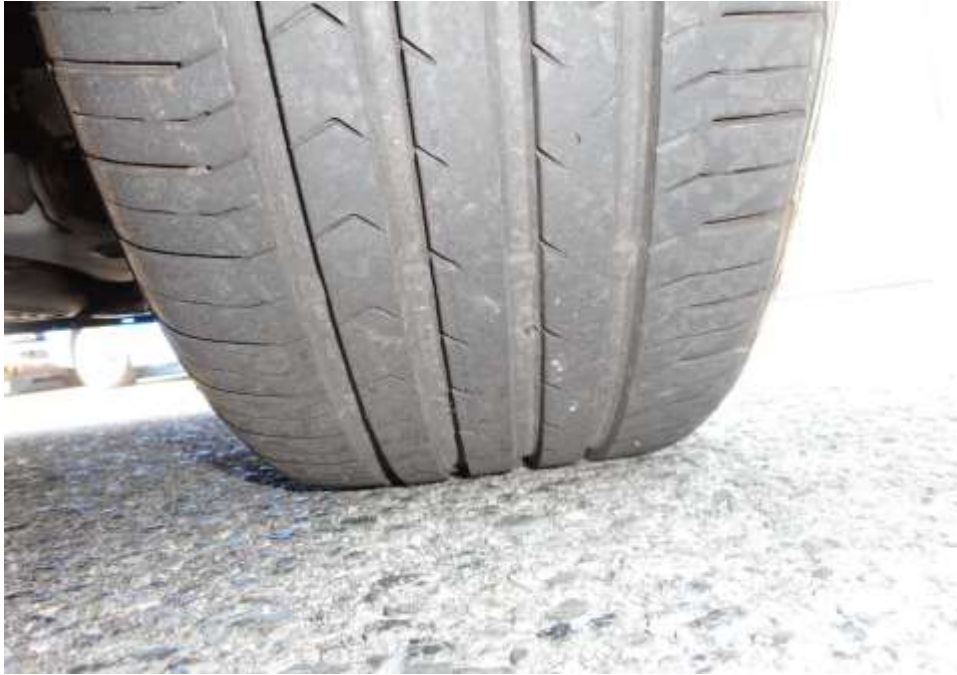
Photo 6 shows the condition of the front right tyre of the Motor Car, which was observed to be in serviceable condition with remaining tread depth of approximately 6.2mm. The tyre, which was wrapped around standard alloy wheel rim, was also observed to be sufficiently inflated for vehicular operation. There was no tear, cut or burst mark(s) on the outer and the inner sidewalls as well as across the tread of the 4 tyres that were fitted on the Motor Car.
