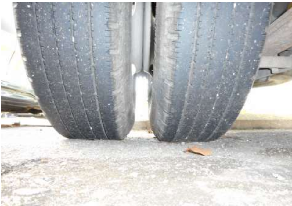
Photo 7 shows the condition of the rear right tyre of the Motor Lorry, which was observed to be in serviceable condition with remaining tread depth of approximately 4.8mm. The tyre, which was wrapped around standard steel wheel rim, was also observed to be sufficiently inflated for vehicular operation.
