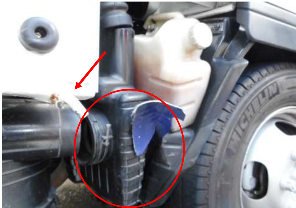
Photo 3 shows a close up view of the Motor Lorry's rear portion at the time of my inspection. Its cabin body panel (arrowed) and air filter box (circled) were damage as a result of the accident at the time of my inspection.
