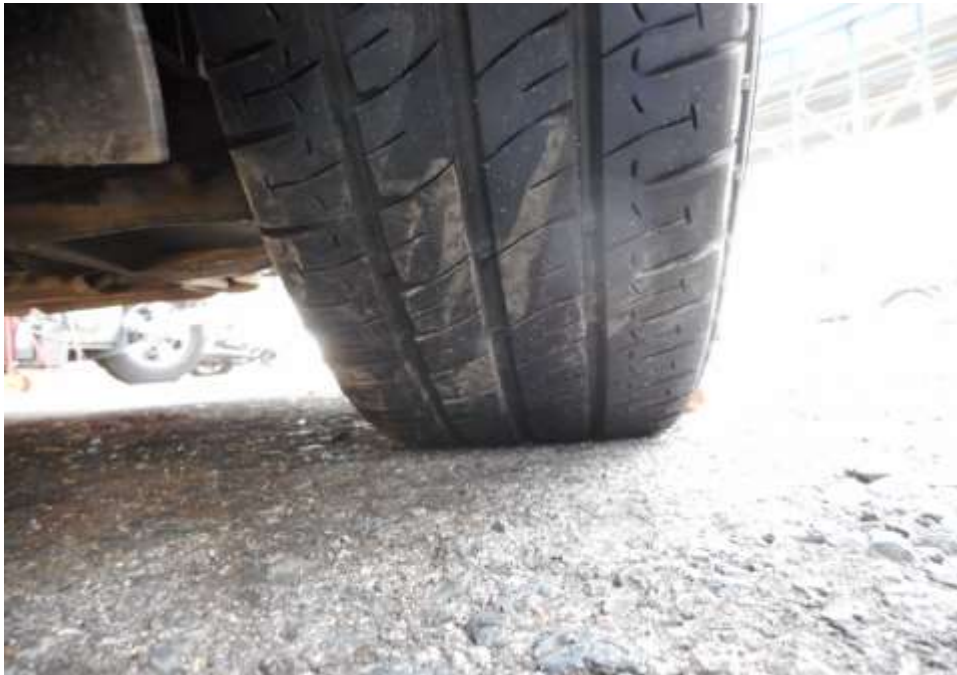
Photo 6 shows the condition of the front right tyre of the Motor Lorry, which was observed to be in serviceable condition with remaining tread depth of approximately 6.9mm. The tyre, which was wrapped around standard steel wheel rim, was also observed to be sufficiently inflated for vehicular operation. There was no tear, cut or burst mark(s) on the outer and the inner sidewalls as well as across the tread of the 6 tyres that were fitted on the Motor Lorry.
