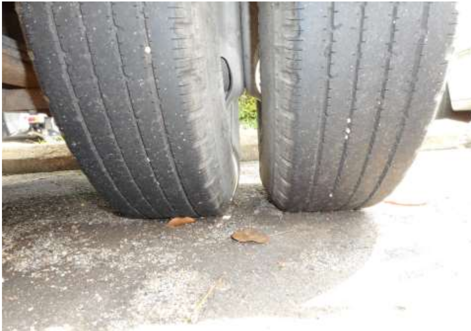
Photo 8 shows the condition of the rear left tyres of the Motor Lorry, which was observed to be in serviceable condition with remaining tread depth of approximately 5.1mm. The tyres, which were wrapped around standard steel wheel rim, were also observed to be sufficiently inflated for vehicular operation. There was also no damage found on all 6 steel wheel rims of the Motor Lorry.
