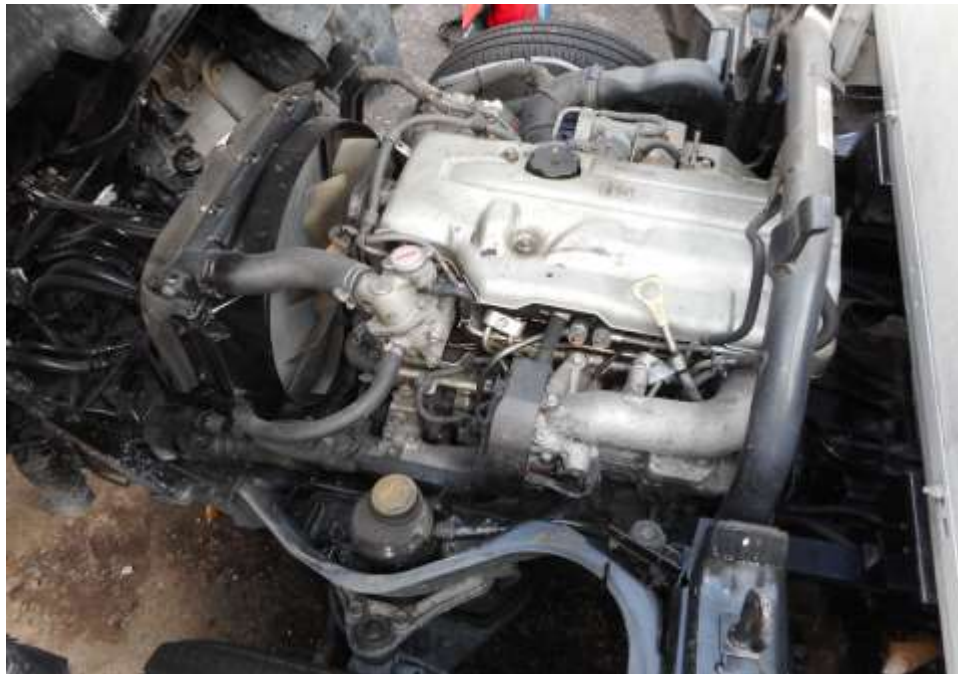
Photo 10 shows a general view of the Motor Lorry's engine compartment, which was accessed by lifting the front cabin of the Motor Lorry. The various parts and components inside the engine compartment were unaffected by the accident. There was also no sign(s) or indication(s) of fresh fluid leakage and/or fluid stain within the engine compartment (photograph shows the engine compartment as viewed from the right front side of the Motor Lorry).
