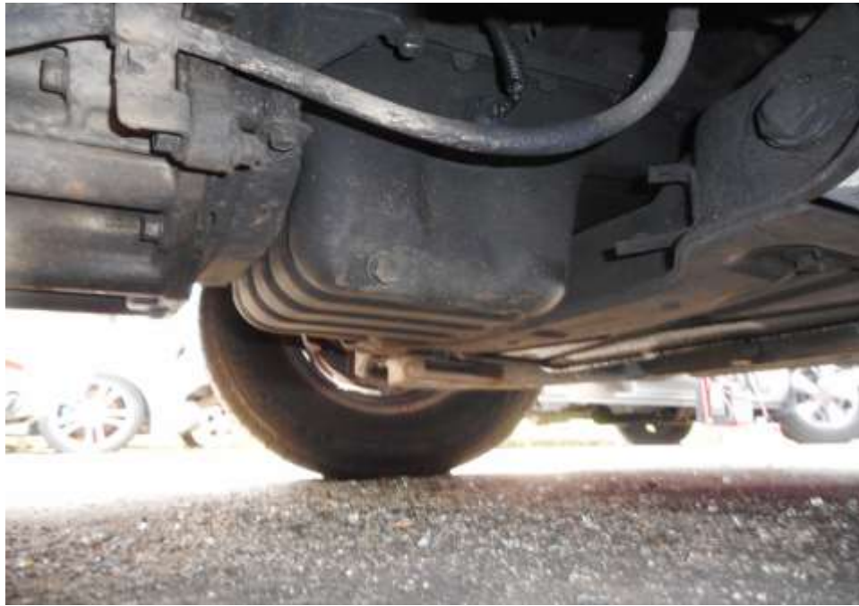
Photo 15 shows the undercarriage of the Motor Lorry, at the area where the engine housing and transmission housing are located. Observed was minor old engine oil stain on the housing of the engine oil sump
