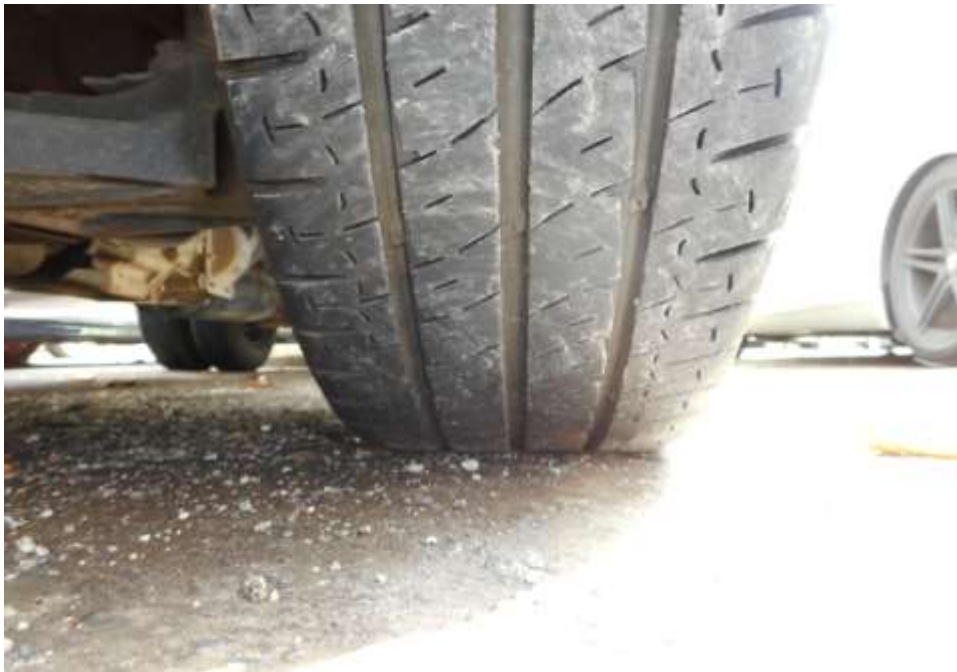
Photo 9 shows the condition of the rear right tyres of the Motor Lorry, which were observed to be in serviceable condition with remaining, tread depth of approximately 5.5mm. There was also no tear, cut or burst mark(s) on the outer and the inner sidewalls as well as across the tread of the 6 tyres that were fitted on the Motor Lorry.
