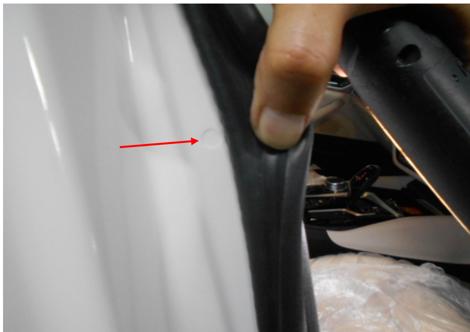
Photo 15 shows the right “B” pillar of the Motor Car. I did not find any weld marks other than original spot weld marks (arrowed) on the non-detachable body panels of the Motor Car, indicating that there was no re-welding works carried out; and that the non-detachable body panels of the Motor Car were originally fitted.
