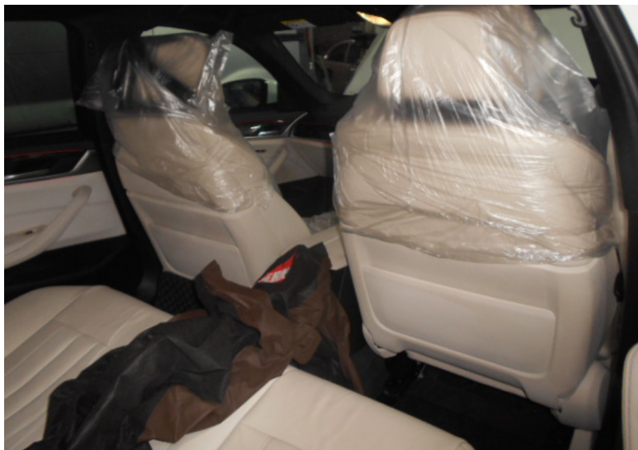
Photo 5 shows the seats of the Motor Car, which were secured via seat rails to the floor board. All the seats of the Motor Car were fitted with a retractable seat belt reel and pre-tensioner. The seat belts were also able to be fastened into the respective pre-tensions that were fitted on the side of each individual seat.
