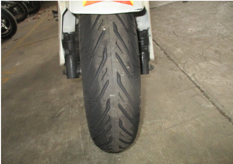
Photo 11 shows the condition of the Motorcycle's front tyre. The front tyre was observed to be in serviceable condition with remaining tread depth of approximately 4mm. There was no tear, burst mark(s) and/or punctured hole(s) on the sidewalls as well as across the tread of the front tyre.
