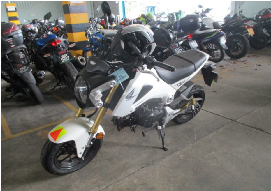
Photo 3 shows a general view of the left body of the Motorcycle at the time of our inspection. The Motorcycle was observed to have sustained damages along its frontal and left portion. Amongst the body parts that were found to have been damaged include its front number plate, headlight assembly, left front signal lamp, front mudguard, left cowling, clutch lever, gear shift rod, gear shift pedal, left front footrest and left front footrest bracket, amongst others.
