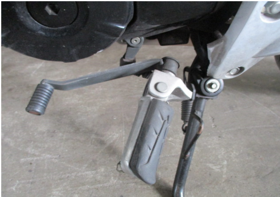
Photo 9 shows a closer view of the broken gear shift rod, gear shift pedal, left front footrest and left front footrest bracket, which were amongst the body parts of the Motorcycle that had sustained damage as a result of the accident.
