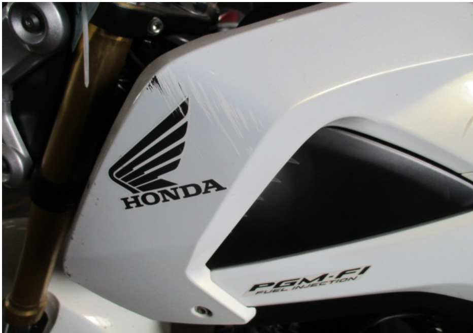
Photo 7 shows a closer view of the left cowling of the Motorcycle that had sustained damage as a result of the accident.
