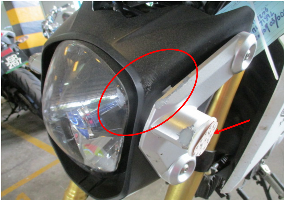
Photo 5 shows a close up view of the headlight assembly (circled) and left front signal lamp (arrowed) which were amongst the body parts of the Motorcycle that had sustained damage as a result of the accident.
