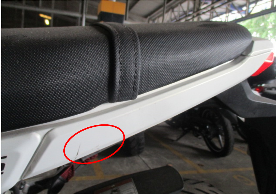
Photo 10 shows the left rear side cover of the Motorcycle which was observed to be damaged as a result of the accident (circled).
