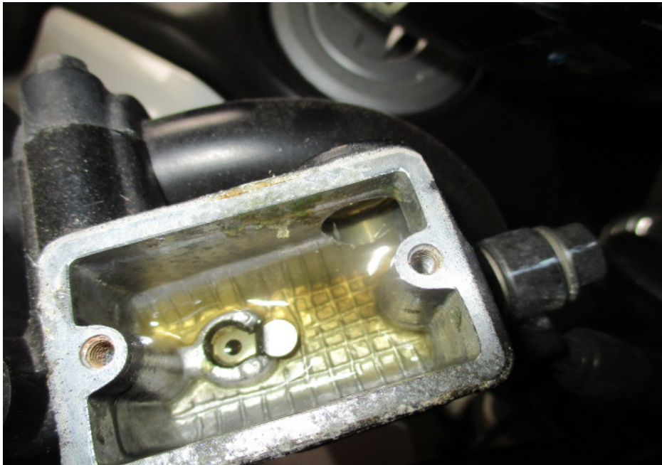
Photo 21 shows the brake fluid reservoir for the front brake of the Motorcycle. The brake fluid was observed to be without contamination. However it was found to be of insufficient level for operational purposes.
