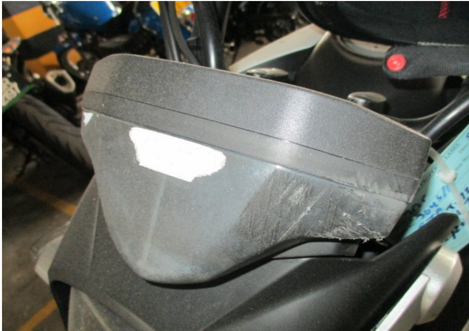
Photo 4 shows a closer view of the speedometer outer cover which was amongst the body parts at the front body of the Motorcycle that had sustained damage as a result of the accident.
