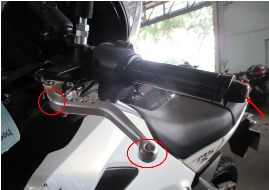
Photo 8 shows a closer view of the clutch lever (circled) and left handlebar end (arrowed) which were amongst the body parts of the Motorcycle that had sustained damage as a result of the accident.
