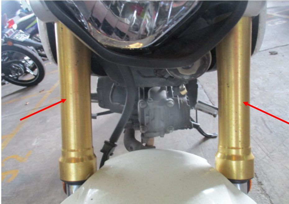
Photo 17 shows the front fork (arrowed) of the Motorcycle. The front fork and fork bracket of the Motorcycle were both found to be intact and undamaged. Turning the Motorcycle's handle bar towards the left and right did not produce any abnormal free play and/or resistance. The steering system of the Motorcycle was in serviceable condition at the time of our inspection.
