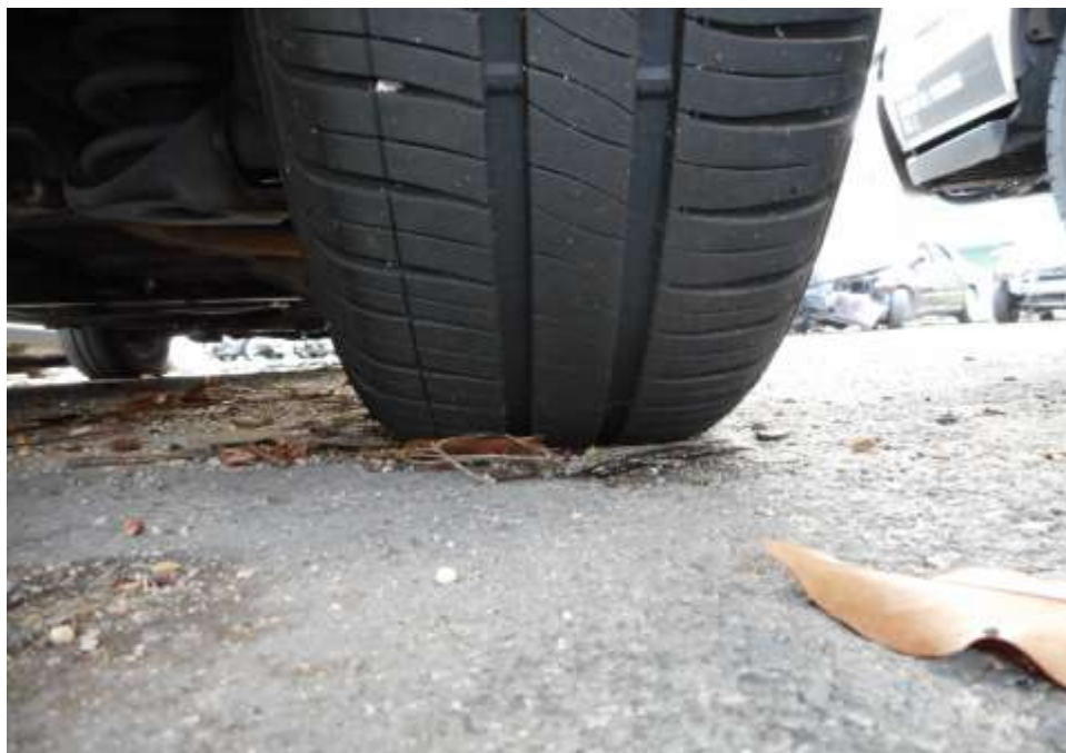
Photo 7 shows the condition of the rear right tyre of the Motor Car, which was observed to be in serviceable condition with remaining tread depth of approximately 6.6mm. The tyre, which was wrapped around standard alloy wheel rim, was also observed to be sufficiently inflated for vehicular operation.
