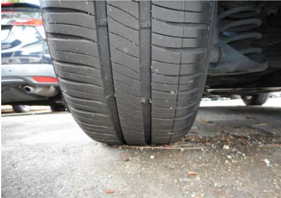
Photo 8 shows the condition of the rear left tyres of the Motor Car, which was observed to be in serviceable condition with remaining tread depth of approximately 6.7mm. The tyres, which were wrapped around standard alloy wheel rim, were also observed to be sufficiently inflated for vehicular operation. There was also no damage found on all 4 alloy wheel rims of the Motor Car.
