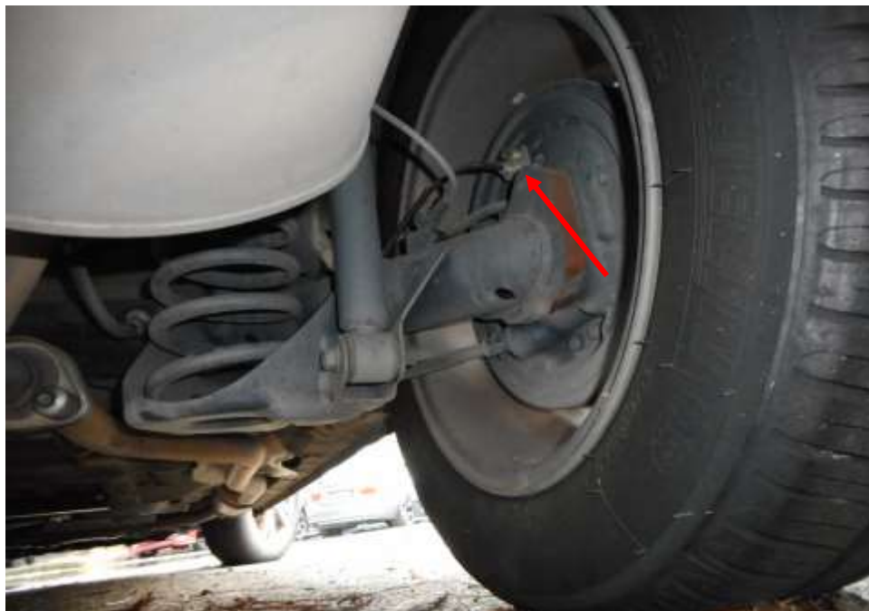
Photo 17 shows the brake pipe (arrowed) at the rear right wheel of the Motor Car. I did not observe any leakage of brake fluid at the time of my inspection of the Motor Car. My static tests of the Motor Car's braking system, along with my visual examination of the various mechanical components in the braking system, had indicated that there was no internal leakage of pressure/vacuum. Hence the braking system of the Motor Car was likely to be in serviceable condition at the material time of accident.
