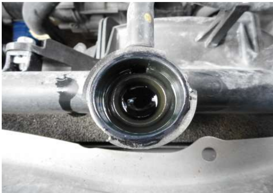
Photo 12 shows the engine coolant reservoir of the Motor Car at the time of my inspection. The engine coolant was observed to be of sufficient level and without any visible contamination.
