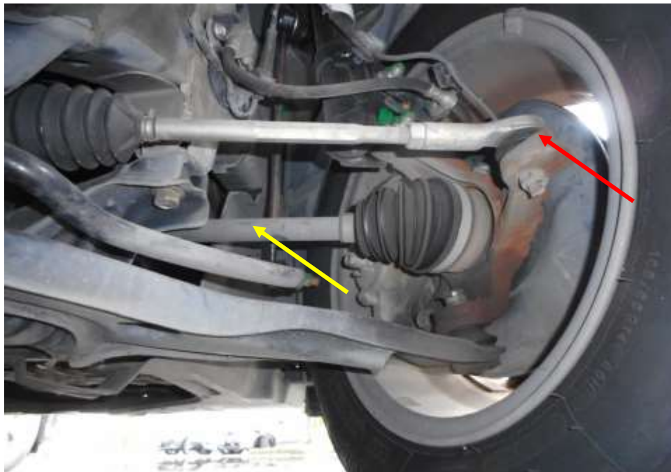
Photo 15 shows the various undercarriage components at the front right wheel of the Motor Car, in particular the steering tie rod end (arrowed) and drive shaft (yellow arrow). The various steering components were all found to be intact, suggesting that the steering system of the Motor Car was likely to be in serviceable condition at the material time of accident. There was also no sign of fluid stain(s) observed on the various undercarriage components.
