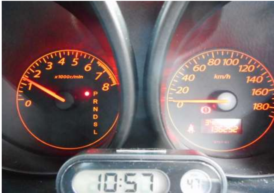
Photo 23 shows no warning lights illuminated on the instrument panel of the Motor Car after the engine was cranked. This would suggest that there was no abnormality to the various electronic operating systems of the Motor Car, like the ABS, SRS and EPS.
