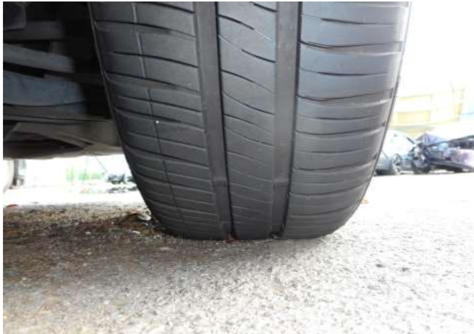
Photo 6 shows the condition of the front right tyre of the Motor Car, which was observed to be in serviceable condition with remaining tread depth of approximately 6mm. The tyre, which was wrapped around standard alloy wheel rim, was also observed to be sufficiently inflated for vehicular operation. There was no tear, cut or burst mark(s) on the outer and the inner sidewalls as well as across the tread of the 4 tyres that were fitted on the Motor Car.
