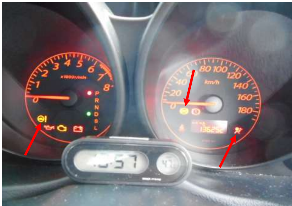
Photo 22 shows the warning light for Anti-Lock Brake System (ABS) and Supplemental Restraint System (SRS) and Electric Power Steering System (EPS) appearing on the instrument panel of the Motor Car during the self-test of its various electronic operating systems when its engine was cranked.
