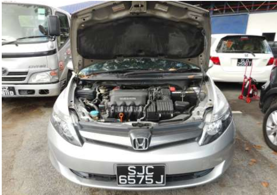
Photo 10 shows a general view of the Motor Car's engine compartment, which was accessed by lifting the front cabin of the Motor Car. The various parts and components inside the engine compartment were unaffected by the accident. There was also no sign(s) or indication(s) of fresh fluid leakage and/or fluid stain within the engine compartment
