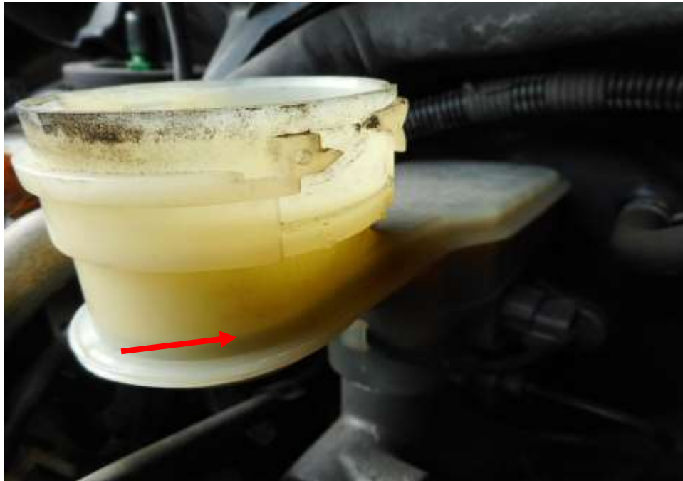
Photo 11 shows the brake fluid reservoir of the Motor Car at the time of my inspection. The brake fluid was observed to be of sufficient level (arrowed) and without any visible contamination.
