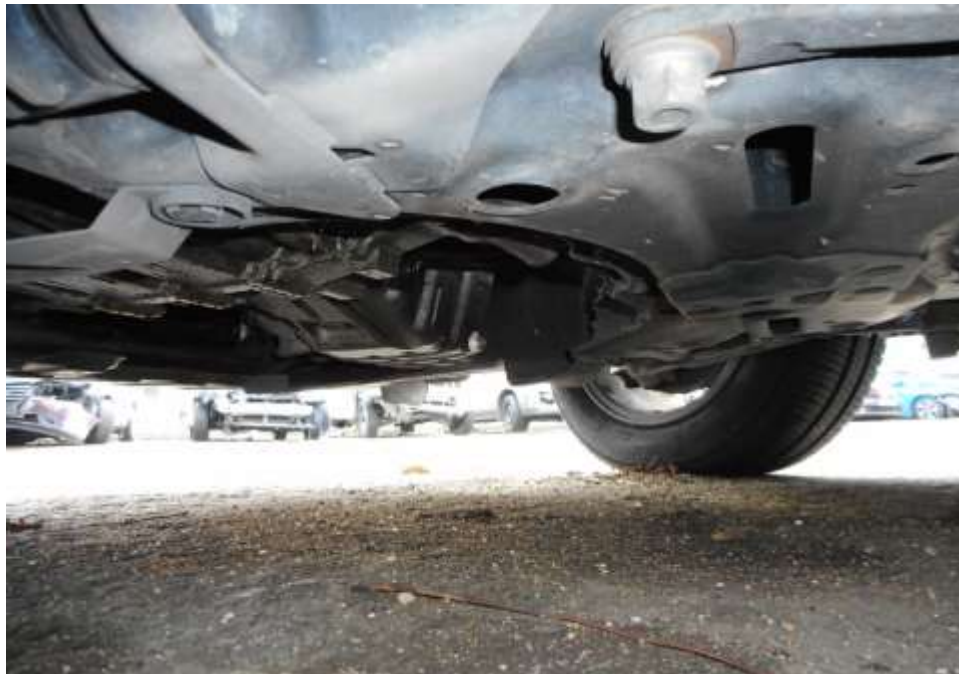
Photo 14 shows the undercarriage of the Motor Car, at the area where the engine housing and transmission housing are located. . I did not find any sign(s) or indication(s) of fluid leak and/or fluid stain(s) on the underside of the Motor Car.
