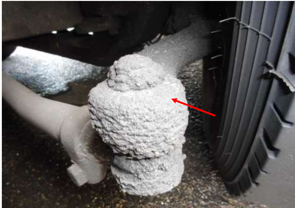
Photo 20 shows the various undercarriage components at the front right wheel of the Motor Bus, in particular the steering tie rod end (arrowed). The various steering components were all found to be intact, suggesting that the steering system of the Motor Bus was likely to be in serviceable condition at the material time of accident. There was also no sign of fluid stain(s) observed on the various undercarriage components.
