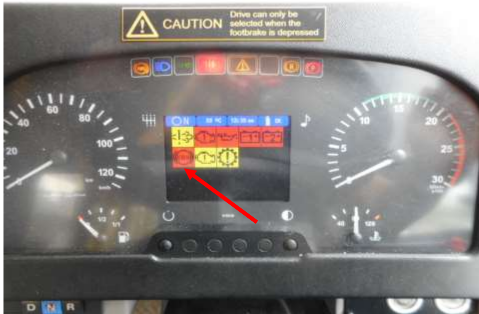
Photo 25 shows the warning light for Anti-Lock Brake System (ABS) appearing on the instrument panel of the Motor Bus during the self-test of its various electronic operating systems when its engine was cranked.
