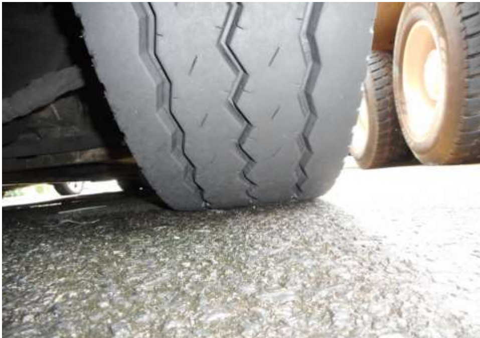
Photo 9 shows the condition of the front left tyres of the Motor Bus, which were observed to be in serviceable condition with remaining tread depth of approximately 10.8mm. There was also no tear, cut or burst mark(s) on the outer and the inner sidewalls as well as across the tread of the 10 tyres that were fitted on the Motor Bus.
