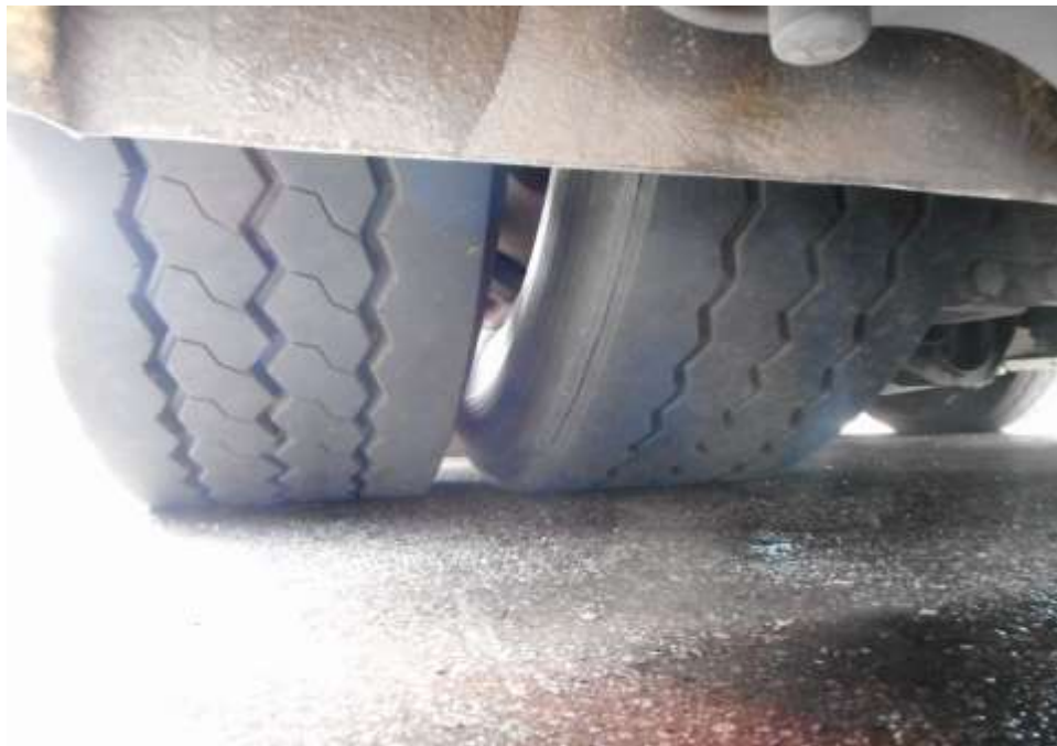
Photo 7 shows the condition of the rear right tyre of the Motor Bus, which was observed to be in serviceable condition with remaining tread depth of approximately 10.6mm. The tyre, which was wrapped around standard steel wheel rim, was also observed to be sufficiently inflated for vehicular operation.
