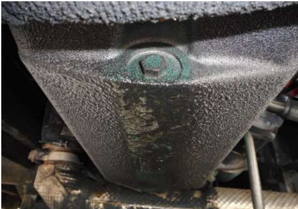
Photo 23 shows the undercarriage of the Motor Bus, at the area where the engine housing located. We observed minor old fluid stains on the surface of the engine oil sump. However the Motor Bus is still in serviceable condition.
