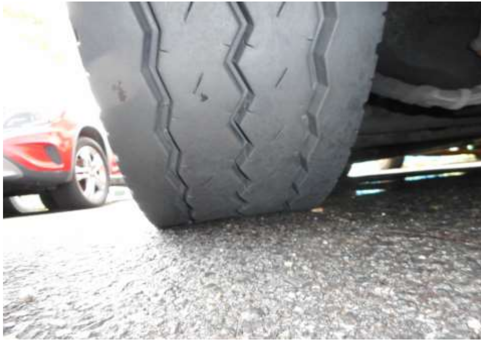
Photo 6 shows the condition of the front right tyre of the Motor Bus, which was observed to be in serviceable condition with remaining tread depth of approximately 11mm. The tyre, which was wrapped around standard steel wheel rim, was also observed to be sufficiently inflated for vehicular operation. There was no tear, cut or burst mark(s) on the outer and the inner sidewalls as well as across the tread of the 10 tyres that were fitted on the Motor Bus.
