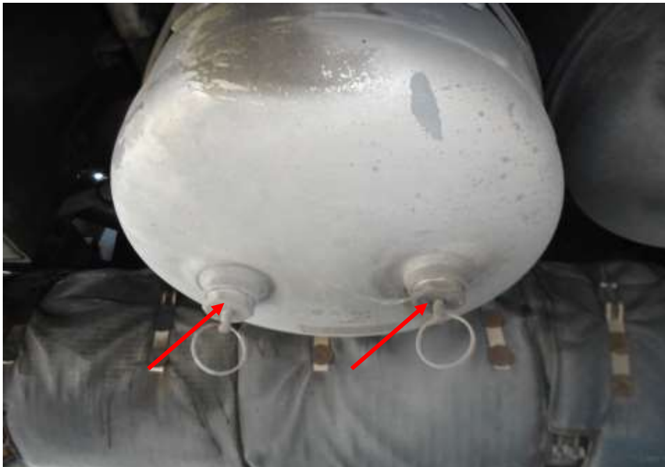
Photo 19 shows the air brake cylinder (arrowed) at the undercarriage of the Motor Bus. I did not observe any leakage of air brake fluid at the time of my inspection of the Motor Bus. My static tests of the Motor Bus's braking system, along with my visual examination of the various mechanical components in the braking system had indicated that there was no internal leakage of pressure/vacuum. Hence the braking system of the Motor Bus was likely to be in serviceable condition at the material time of accident.
