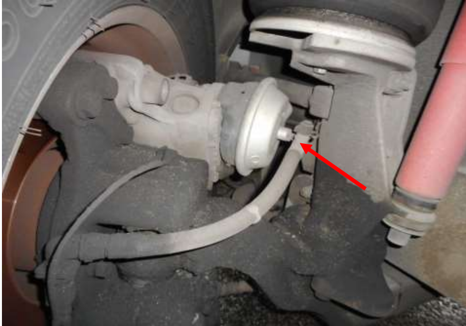
Photo 18 shows the brake pipe (arrowed) at the front left wheel of the Motor Bus. I did not observe any leakage of brake fluid at the time of my inspection of the Motor Bus. My static tests of the Motor Bus's braking system, along with my visual examination of the various mechanical components in the braking system had indicated that there was no internal leakage of pressure/vacuum. Hence the braking system of the Motor Bus was likely to be in serviceable condition at the material time of accident.
