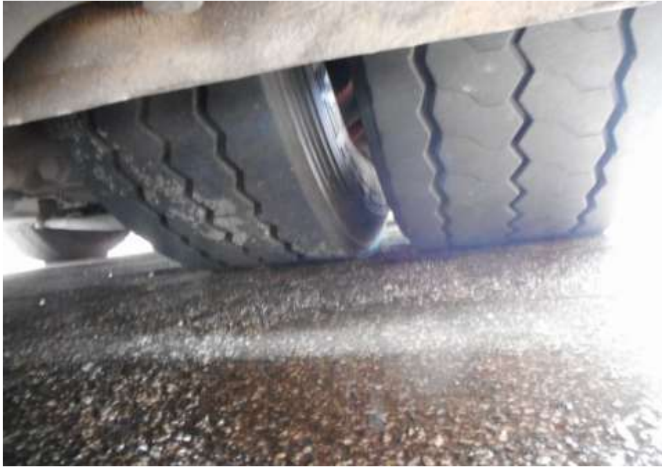
Photo 8 shows the condition of the rear left tyres of the Motor Bus, which was observed to be in serviceable condition with remaining tread depth of approximately 9.5mm. The tyres, which were wrapped around standard steel wheel rim, were also observed to be sufficiently inflated for vehicular operation. There was also no damage found on all 10 steel wheel rims of the Motor Bus.
