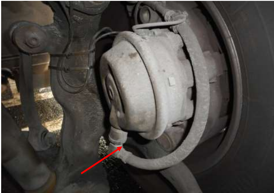
Photo 20 shows the brake pipe (arrowed) at the front left wheel of the Motor Bus. The braking components were observed to be intact at the time of my inspection of the Motor Bus.
