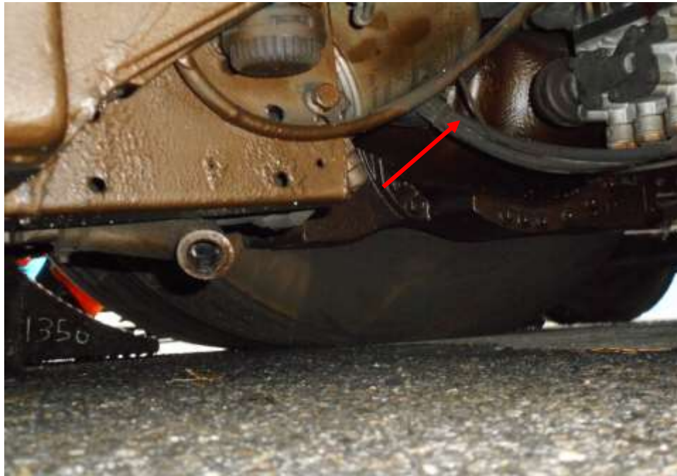
Photo 18 shows the brake pipe (arrowed) at the rear left wheel of the Motor Bus. The braking components were observed to be intact at the time of my inspection of the Motor Bus.
