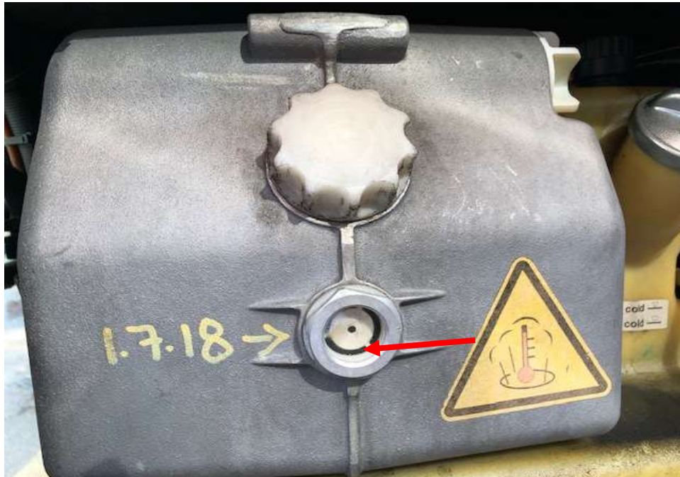
Photo 13 shows the engine coolant reservoir of the Motor Bus at the time of my inspection. The engine coolant was observed to be of insufficient level (arrowed).
