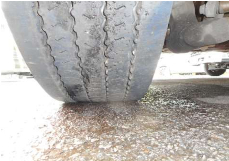
Photo 11 shows the condition of the front left tyres of the Motor Bus, which were observed to be in serviceable condition with remaining tread depth of approximately 12.3mm. There was also no tear, cut or burst mark(s) on the outer and the inner sidewalls as well as across the tread of the 8 tyres that were fitted on the Motor Bus.
