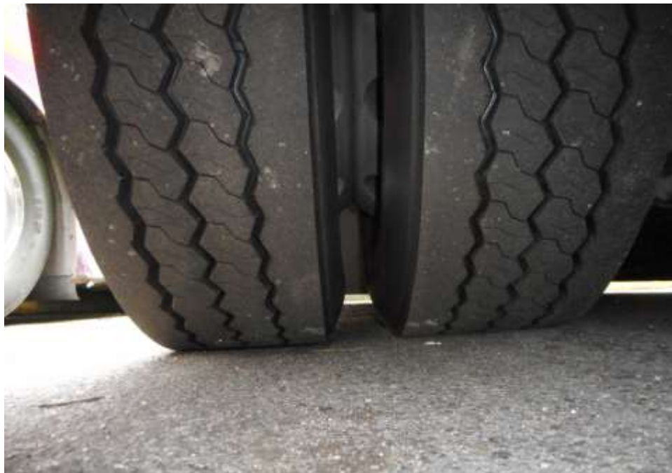
Photo 9 shows the condition of the rear right tyre of the Motor Bus, which was observed to be in serviceable condition with remaining tread depth of approximately 11.8mm. The tyre, which was wrapped around standard steel wheel rim, was also observed to be sufficiently inflated for vehicular operation.
