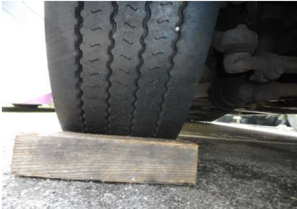
Photo 8 shows the condition of the front right tyre of the Motor Bus, which was observed to be in serviceable condition with remaining tread depth of approximately 11.7mm. The tyre, which was wrapped around standard steel wheel rim, was also observed to be sufficiently inflated for vehicular operation. There was no tear, cut or burst mark(s) on the outer and the inner sidewalls as well as across the tread of the 8 tyres that were fitted on the Motor Bus.
