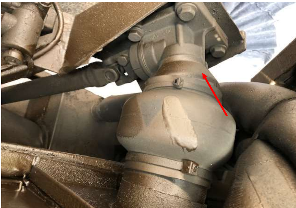
Photo 23 shows the steering box component (arrowed) at the undercarriage of the Motor Bus was found to be intact without any visible damage. There was also no sign of fluid stain(s) observed on the various undercarriage components.
