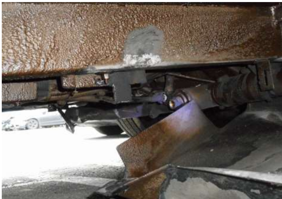
Photo 16 shows the undercarriage diesel fuel hose of the Motor Bus at the time of inspection. The fuel hose was observed to be damaged as a result of the accident.
