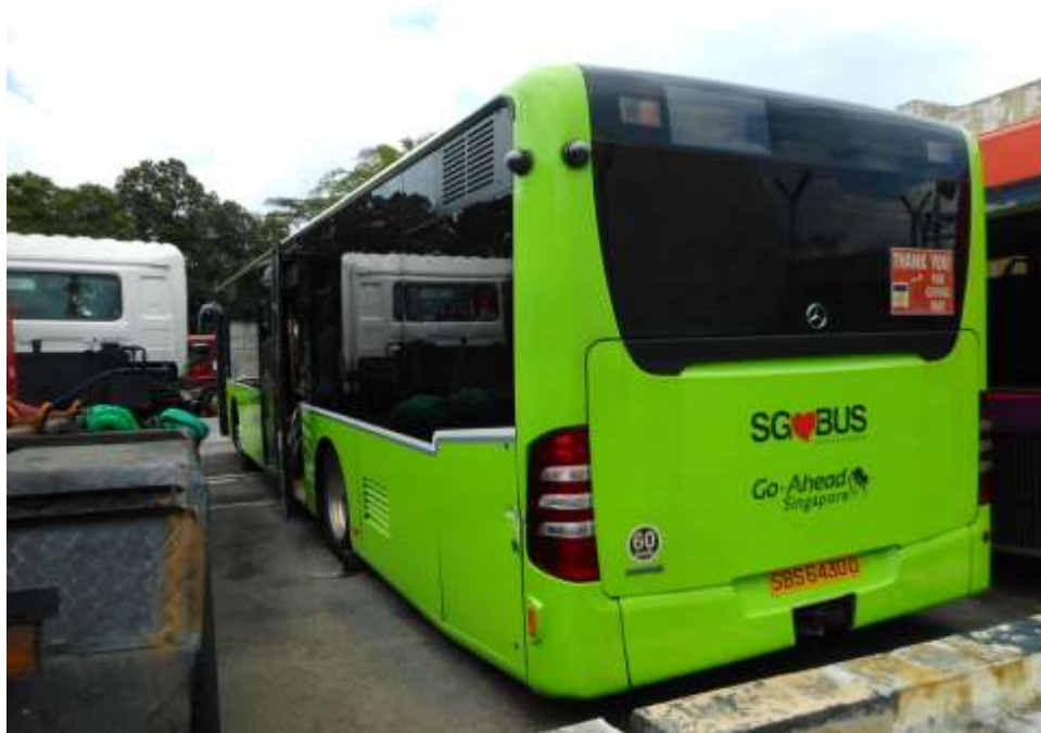
Photo 6 shows a general view of the left rear body of the Motor Bus at the time of my inspection. Its body panel and rear left headlamp was damaged as a result of the accident.
