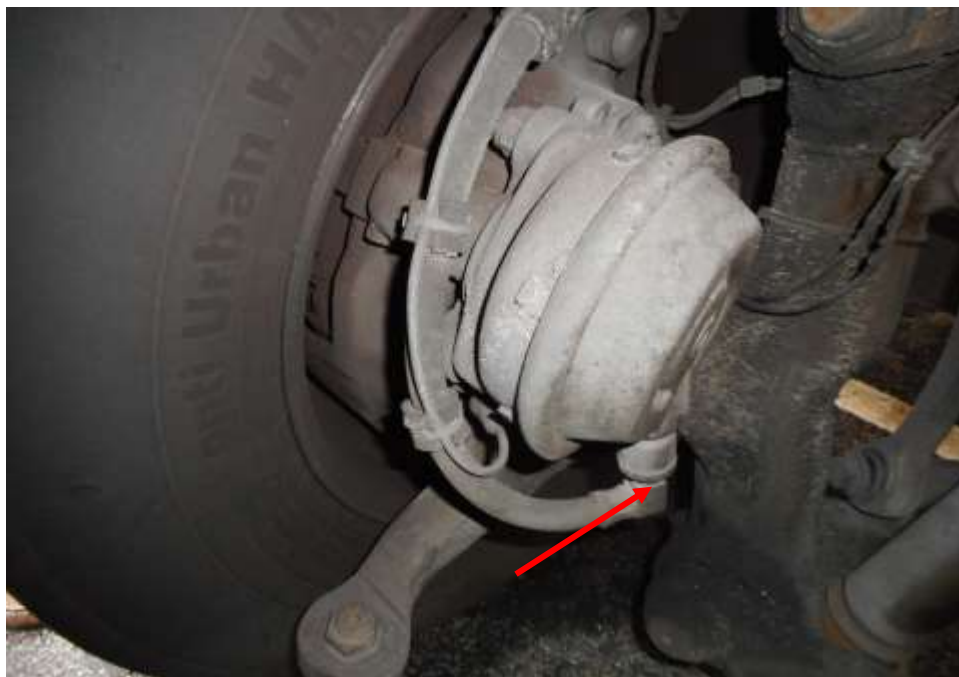
Photo 19 shows the brake pipe (arrowed) at the front right wheel of the Motor Bus. The braking components were observed to be intact at the time of my inspection of the Motor Bus.
