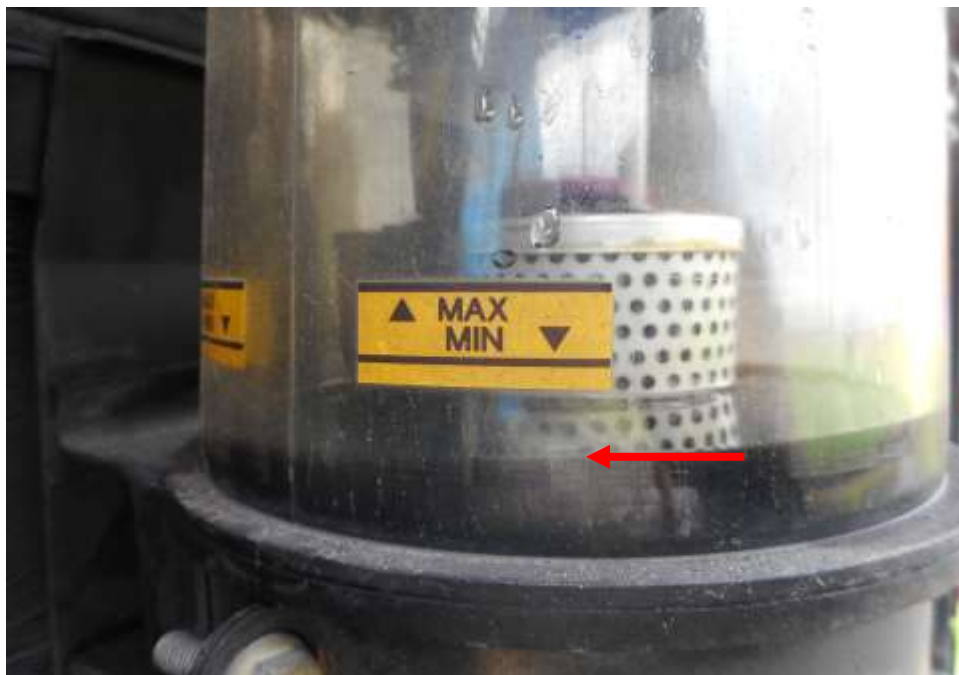
Photo 14 shows the power steering fluid reservoir of the Motor Bus at the time of my inspection. The power steering fluid was observed to be of insufficient level (arrowed).
