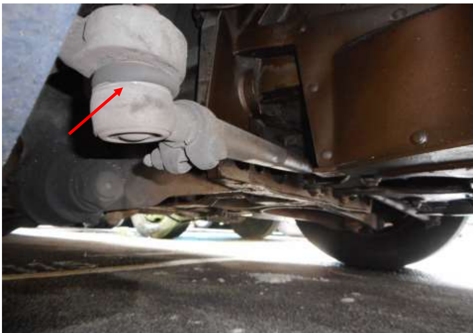
Photo 21 shows the various undercarriage components at the front right wheel of the Motor Bus, in particular the steering tie rod end (arrowed). The various steering components were all found to be intact without any visible damage. There was also no sign of fluid stain(s) observed on the various undercarriage components.
