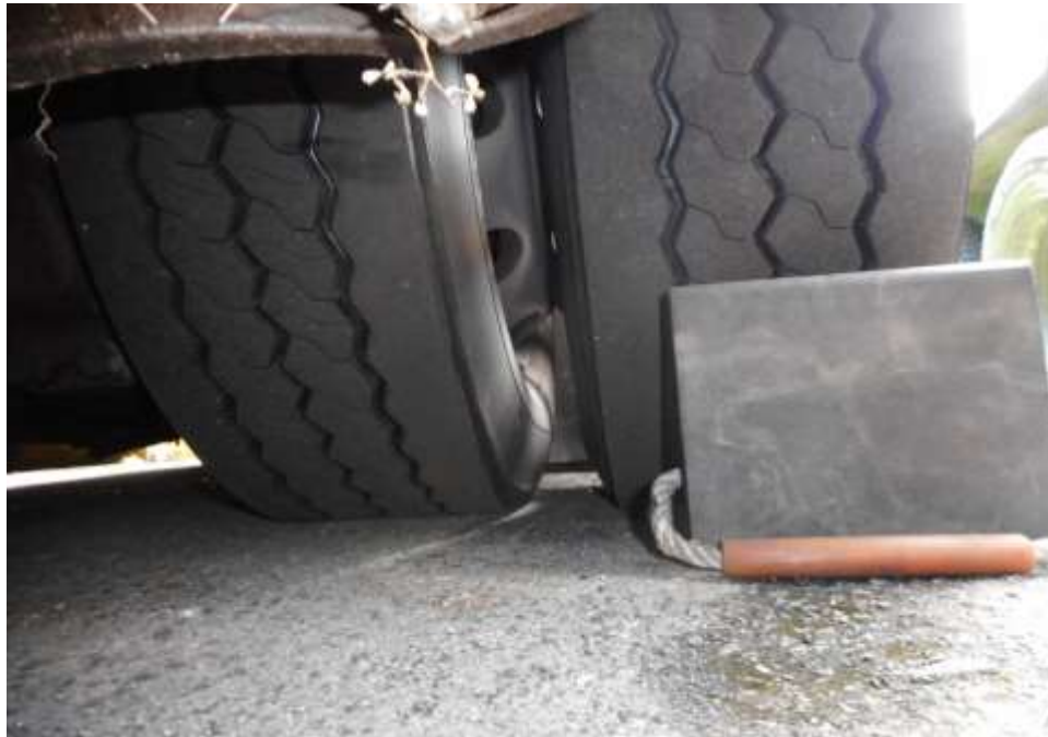
Photo 10 shows the condition of the rear left tyres of the Motor Bus, which was observed to be in serviceable condition with remaining tread depth of approximately 12.6mm. The tyres, which were wrapped around standard steel wheel rim, were also observed to be sufficiently inflated for vehicular operation. There was also no damage found on all 8 steel wheel rims of the Motor Bus.
