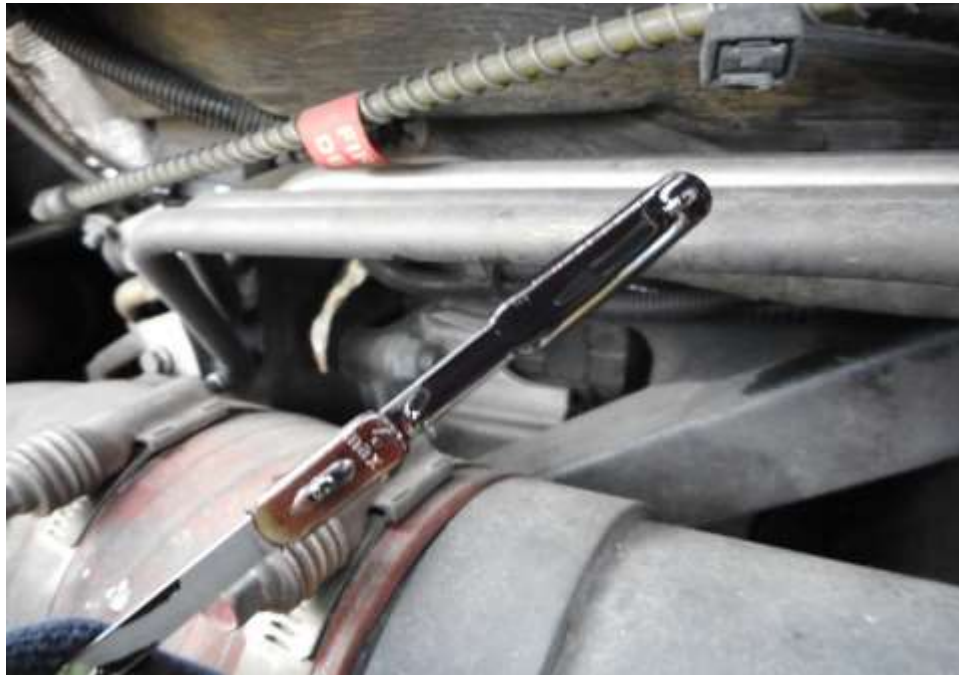
Photo 15 shows the engine oil dip stick system of the Motor Bus at the time of inspection. The engine oil was observed to be of sufficient level for operation and without any visible contamination.
