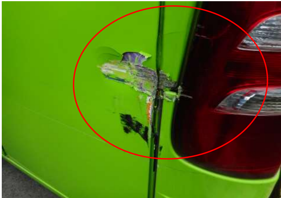
Photo 7 shows a close up view of the left rear body of the Motor Bus at the time of my inspection. Its body panel and rear left headlamp (circled) was damaged as a result of the accident.
