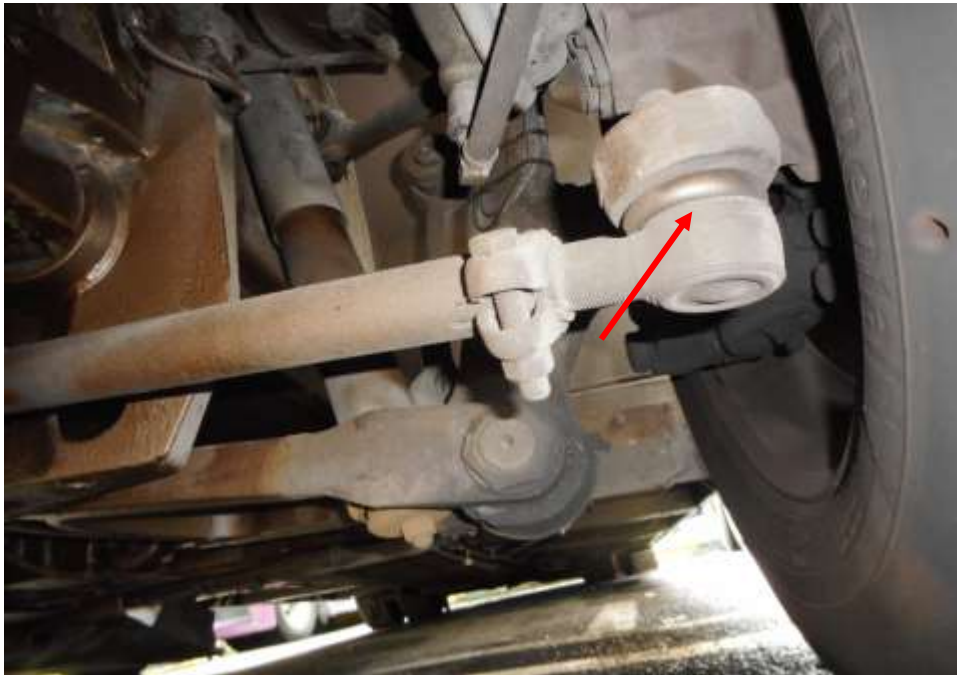
Photo 22 shows the various undercarriage components at the front left wheel of the Motor Bus, in particular the steering tie rod end (arrowed). The various undercarriage components of the Motor Bus were all found to be intact without any visible damage. There was also no sign of fluid stain(s) observed on the various undercarriage components.
