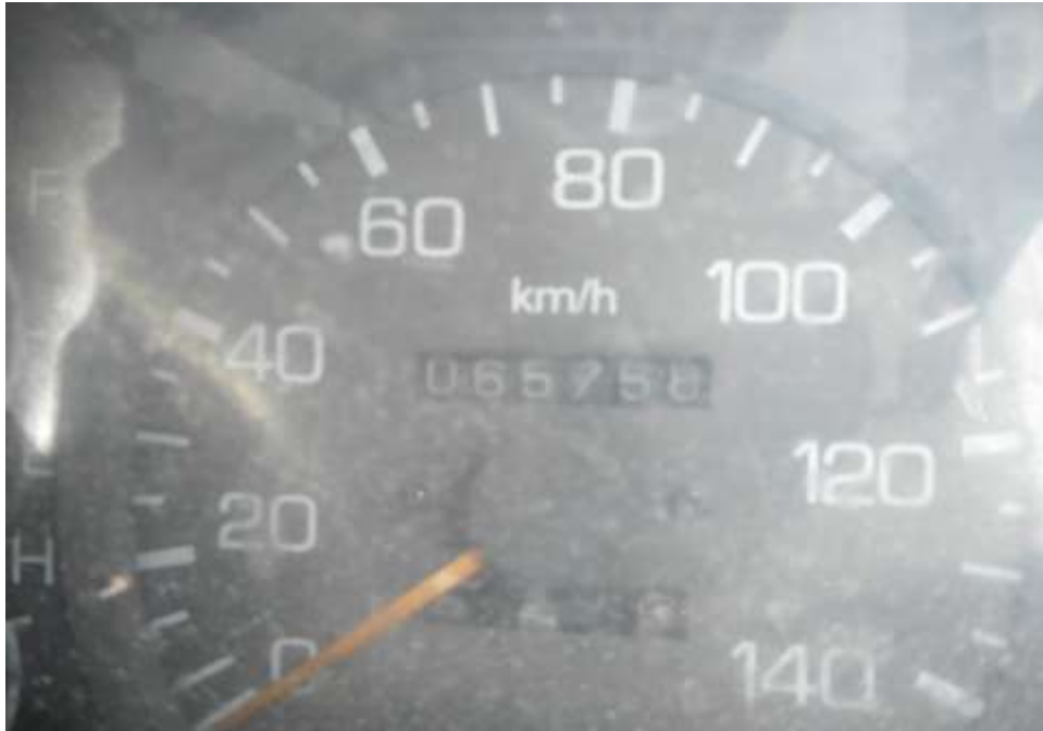
Photo 1 shows a general view of the instrument cluster of the Motor Trailer at the time of my inspection. The mileage of the Motor Trailer was 65,758km
