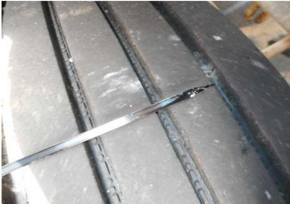
Photo 20 shows the engine oil dip stick of the Motor Trailer at the time of my inspection. The engine oil was observed to be of sufficient level and without any visible contamination.
