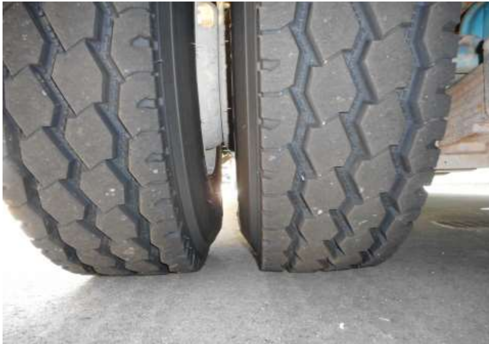
Photo 15 shows the condition of the left tyres of the trailer, which was observed to be in serviceable condition with remaining tread depth of approximately 10.9mm. The tyres, which were wrapped around standard steel wheel rim, were also observed to be sufficiently inflated for vehicular operation. There was also no damage found on all 6 steel wheel rims of the Motor Trailer.
