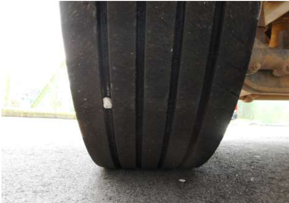
Photo 13 shows the condition of the front left tyres of the Motor Trailer, which were observed to be in serviceable condition with remaining tread depth of approximately 7.6mm. There was also no tear, cut or burst mark(s) on the outer and the inner sidewalls as well as across the tread of the 6 tyres that were fitted on the Motor Trailer.
