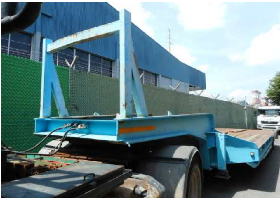
Photo 6 shows a general view of the front body of the trailer at the time of my inspection. The Motor Trailer was observed to be intact and unaffected by the accident.
