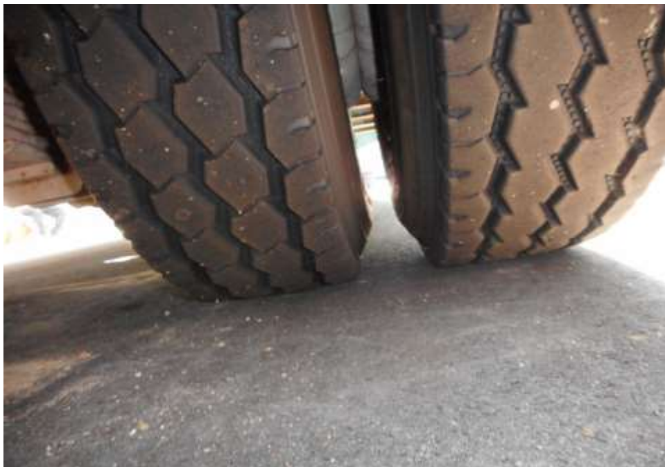
Photo 14 shows the condition of the right tyres of the trailer, which was observed to be in serviceable condition with remaining, tread depth of approximately 9.7mm. The tyre, which was wrapped around standard steel wheel rim, was also observed to be sufficiently inflated for vehicular operation.
