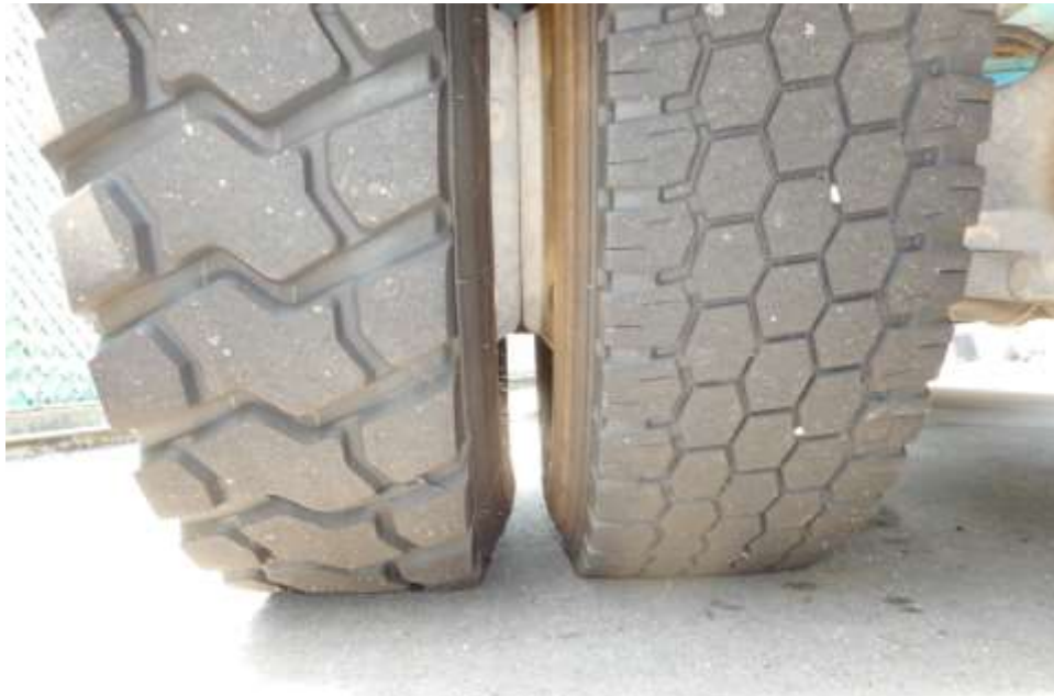
Photo 11 shows the condition of the rear right tyre of the Motor Trailer, which was observed to be in serviceable condition with remaining tread depth of approximately 11.3mm. The tyre, which was wrapped around standard steel wheel rim, was also observed to be sufficiently inflated for vehicular operation.
