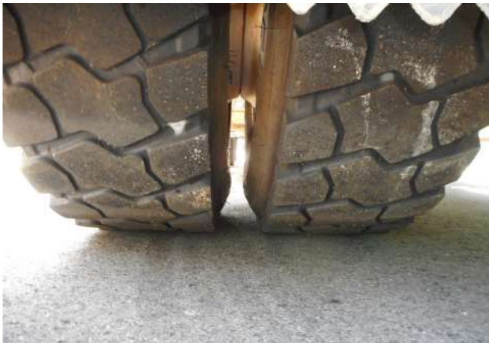
Photo 12 shows the condition of the rear left tyres of the Motor Trailer, which was observed to be in serviceable condition with remaining tread depth of approximately 5.4mm. The tyres, which were wrapped around standard steel wheel rim, were also observed to be sufficiently inflated for vehicular operation. There was also no damage found on all 6 steel wheel rims of the Motor Trailer.
