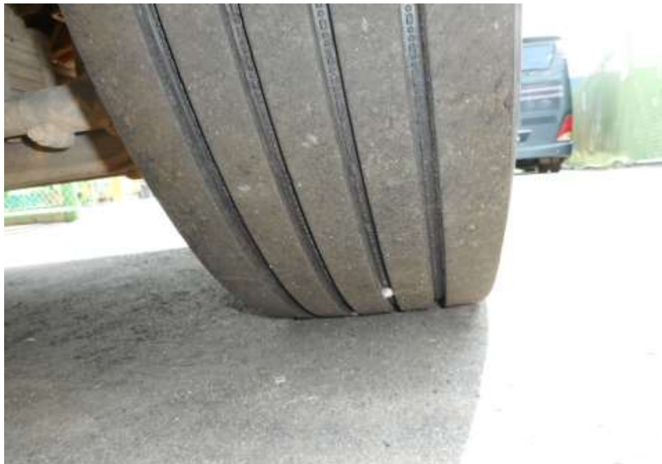
Photo 10 shows the condition of the front right tyre of the Motor Trailer, which was observed to be in serviceable condition with remaining tread depth of approximately 9.8 mm. The tyre, which was wrapped around standard steel wheel rim, was also observed to be sufficiently inflated for vehicular operation. There was no tear, cut or burst mark(s) on the outer and the inner sidewalls as well as across the tread of the 6 tyres that were fitted on the Motor Trailer.
