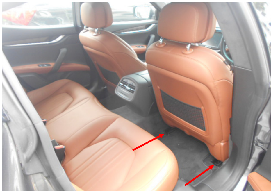
Photo 5 shows the seats of the Motor Car, which were secured via seat rails (arrowed) to the floor board. All the seats of the Motor Car were fitted with a retractable seat belt reel and pre-tensioner. The seat belts were also able to be fastened into the respective pre-tensions that were fitted on the side of each individual seat.
