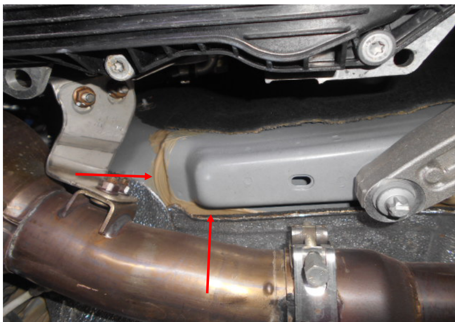
Photo 14 shows the floor board at the underside centre of the Motor Car. The original factory sealant at the joints along the non-detachable body panels were untouched, indicating no work was done on the non-detachable body panels of the Motor Car; and that these body panels were originally fitted.
