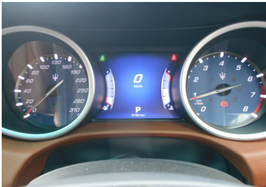
Photo 7 shows the respective warning lights no longer illuminated after the engine was started, indicating that there was no fault detected to the ABS, SRS, TPM and TCS systems of the Motor Car during the self-test. These electronic systems were hence in working condition at the time of my inspection.
