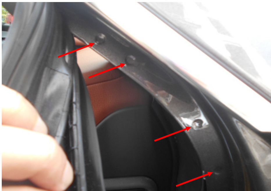
Photo 17 shows the right "A" pillar of the Motor Car. I did not find any weld marks other than original spot weld marks (arrowed) on the non-detachable body panels of the Motor Car, indicating that there was no re-welding works carried out; and that the non-detachable body panels of the Motor Car were originally fitted.
