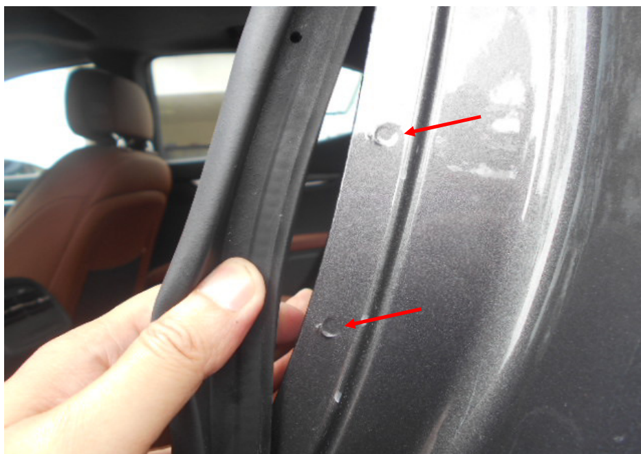
Photo 16 shows the left "C" pillar of the Motor Car. I did not find any weld marks other than original spot weld marks (arrowed) on the non-detachable body panels of the Motor Car, indicating that there was no re-welding works carried out; and that the non-detachable body panels of the Motor Car were originally fitted.
