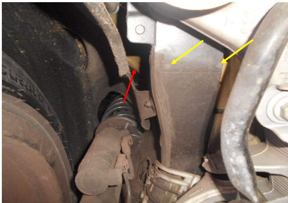
Photo 13 shows the chassis/structural body at the underside front left of the Motor Car. Visually, I did not find any weld marks other than original spot weld marks (yellow arrow) on the chassis/structural body of the Motor Car. The original factory sealant (red arrow) at the joints along the chassis/structural body was also untouched, indicating no work was done on the chassis/structural body of the Motor Car and that the chassis/structural body was originally fitted.
