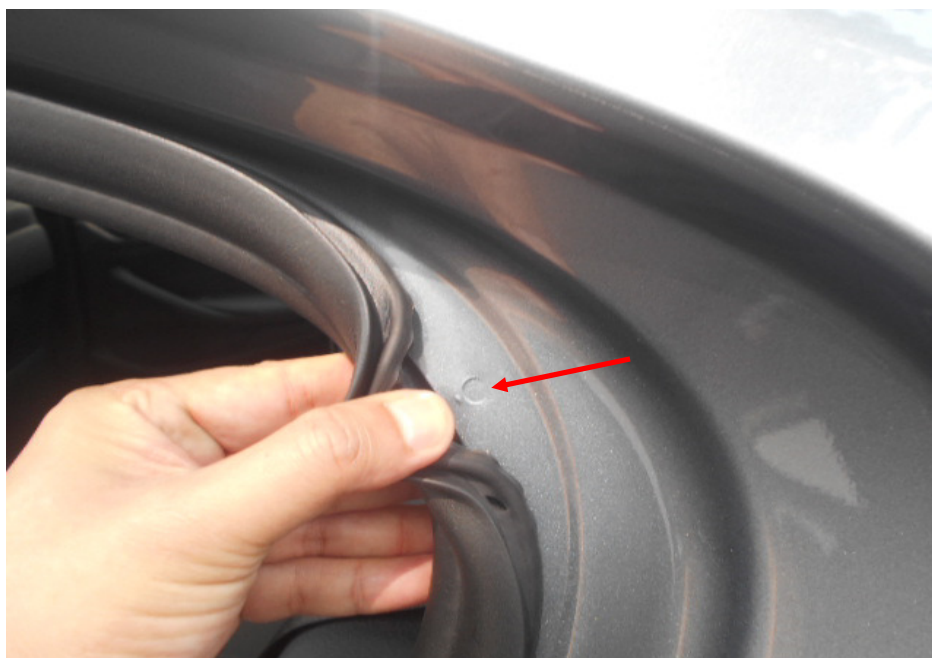
Photo 16 shows the rear left "C" pillar of the Motor Car. I did not find any weld marks other than original spot weld marks (arrowed) on the non-detachable body panels of the Motor Car, indicating that there was no re-welding works carried out; and that the non-detachable body panels of the Motor Car were originally fitted.
