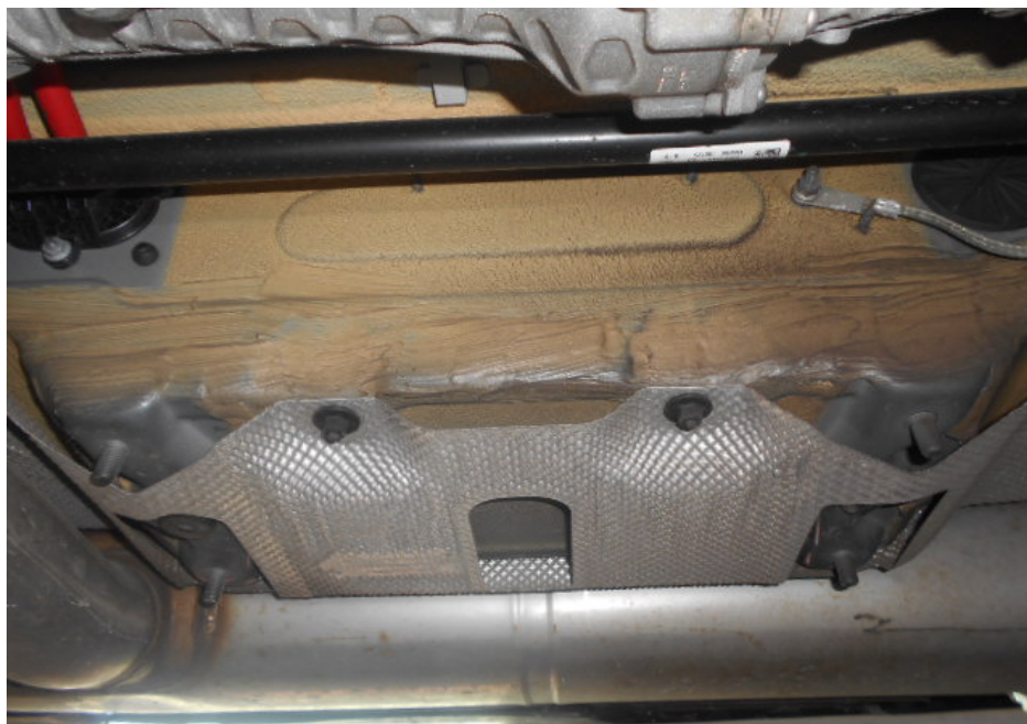
Photo 15 shows the floor board at the underside rear of the Motor Car. The original factory sealant at the joints along the non-detachable body panels were untouched, indicating no work was done on the non-detachable body panels of the Motor Car; and that the non-detachable body panels were originally fitted.
