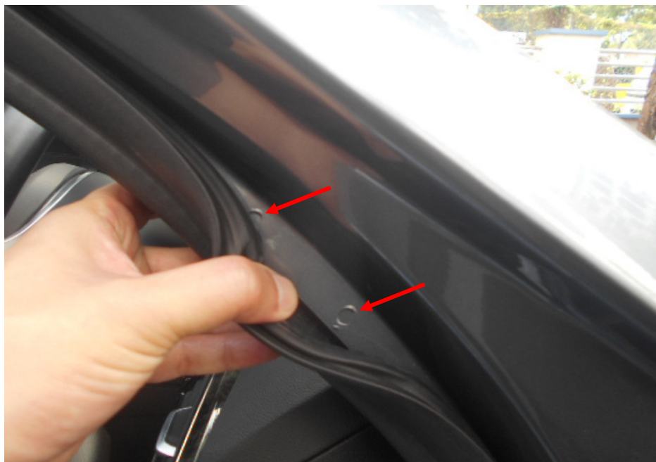
Photo 17 shows the front right “A” pillar of the Motor Car. I did not find any weld marks other than original spot weld marks (arrowed) on the non-detachable body panels of the Motor Car, indicating that there was no re-welding works carried out; and that the non-detachable body panels of the Motor Car were originally fitted.
