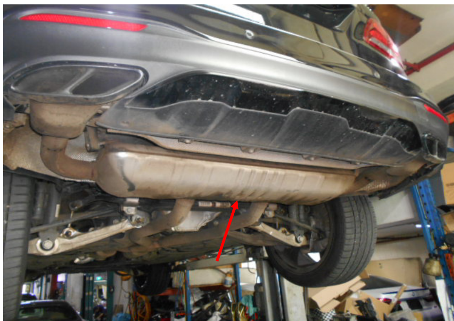
Photo 12 shows the Motor Car's rear exhaust muffler (arrowed). My examination of the Motor Car's exhaust system revealed no sign(s) or indication(s) of any cut or weld marks along its exhaust pipes and on its rear muffler.
