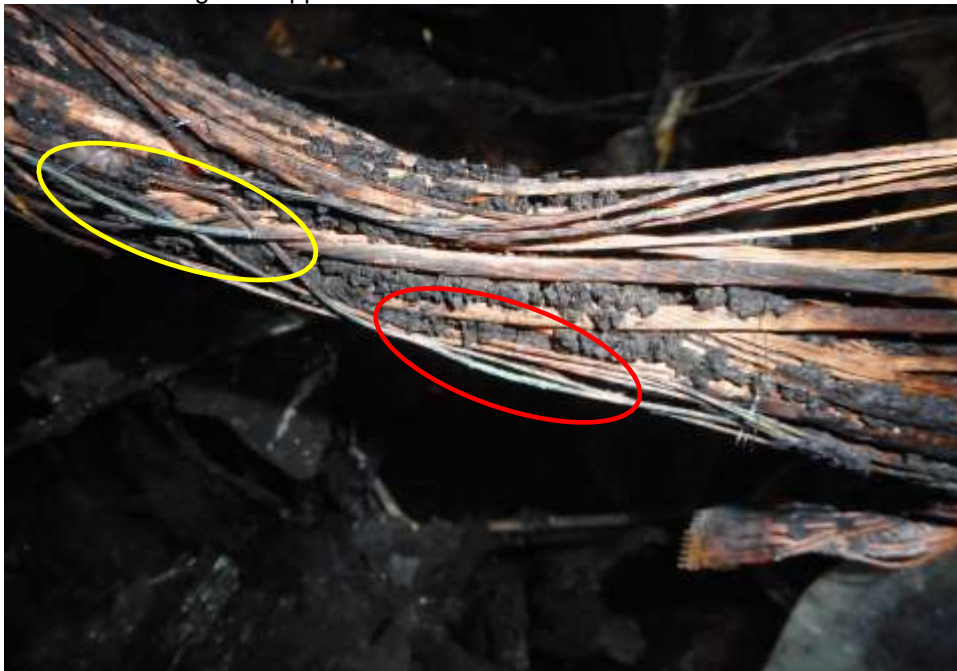
Photo 13 shows a close up view of the original wiring harness in the engine compartment. The original wiring harness (yellow and red circled) was observed with greenish residue on the surface. The presence of greenish residue indicates internal heating of copper wires, a sign of an electrical short circuit occurring. The greenish residue is normally left behind from oxidation as a result of chemical reaction involving the copper wires.
