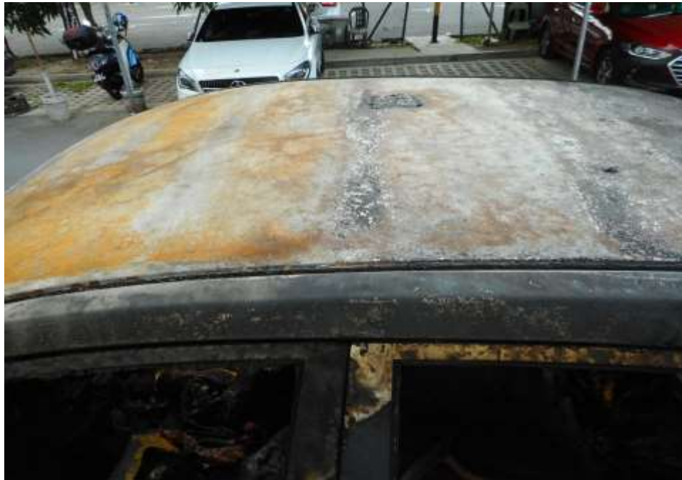
Photo 9 shows the exterior of the centre portion of the Insured Vehicle at the time of our inspection. The high heat intensity burn marks (whitish burn marks) and rust that had development found on the exterior surface indicates that the fire had originated from the frontal portion of the Insured Vehicle.
