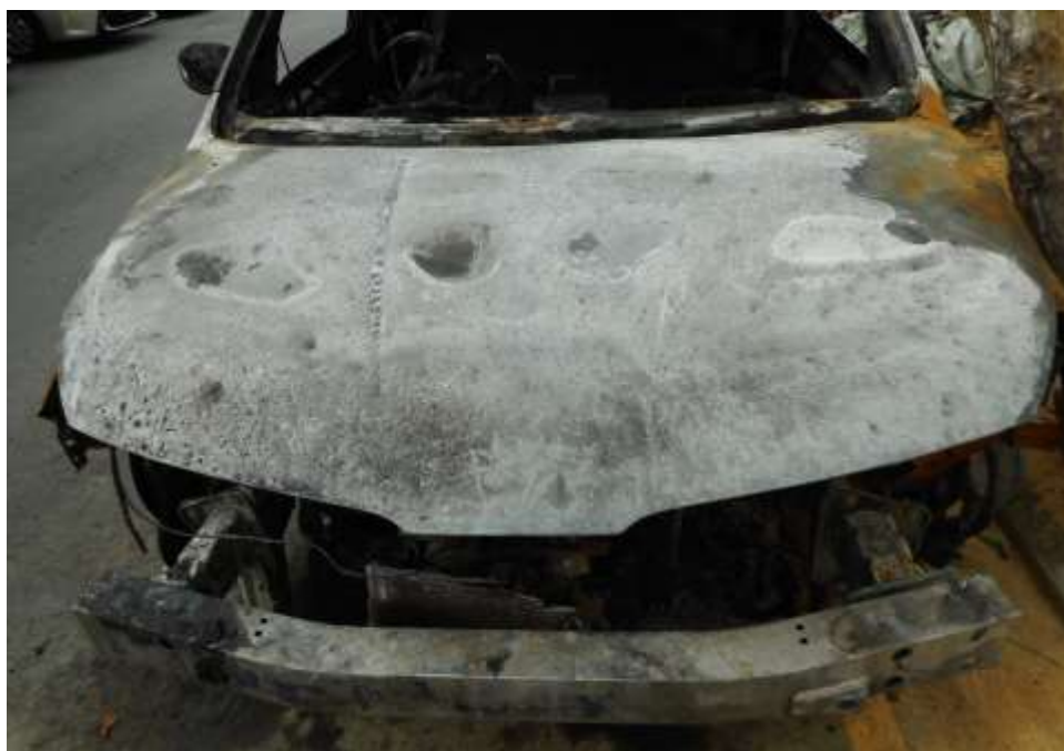
Photo 7 shows the exterior of the front bonnet of the Insured Vehicle at the time of our inspection. The high heat intensity burn marks (whitish burn marks) and rust that had development found on the exterior surface of the bonnet indicates that the fire had originated from the front portion of the Insured Vehicle.
