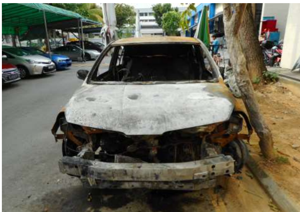
Photo 2 shows the general view of the front portion of the Insured Vehicle at the time of our inspection. The Insured Vehicle was observed to have sustained extensive fire damage all around. Its engine compartment and interior compartment were completely burnt. Rust had accumulated all over the front and centre portion of the Insured Vehicle as a result of exposure to environmental condition for a period of time.
