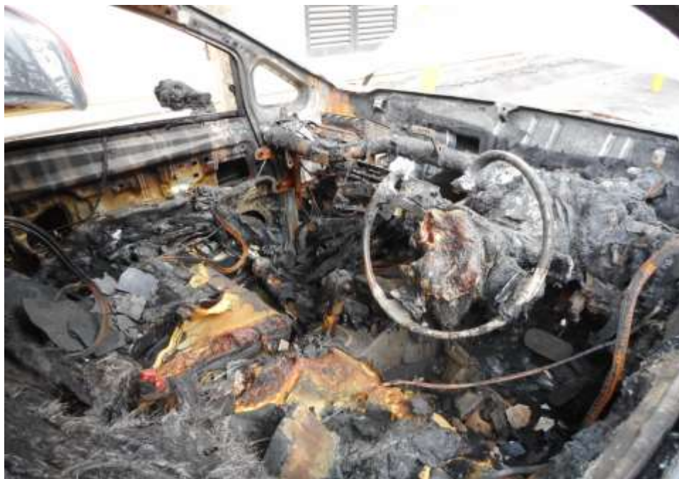
Photo 5 shows the general view of the interior compartment of the Insured Vehicle at the time of our inspection. Its interior compartment was completely burnt as a result of the fire.
