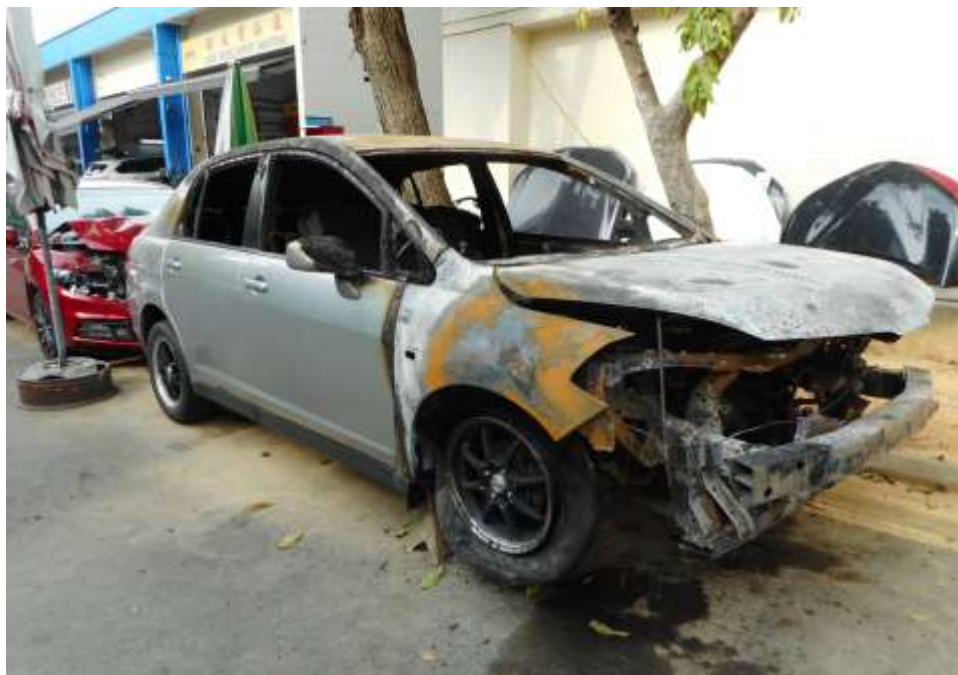
Photo 3 shows the general view of the right body of the Insured Vehicle at the time of our inspection. The Insured Vehicle was observed to have sustained extensive fire damage all around. Rust had accumulated all over the front and interior compartment of the Insured Vehicle as a result of exposure to environmental condition for a period of time.
