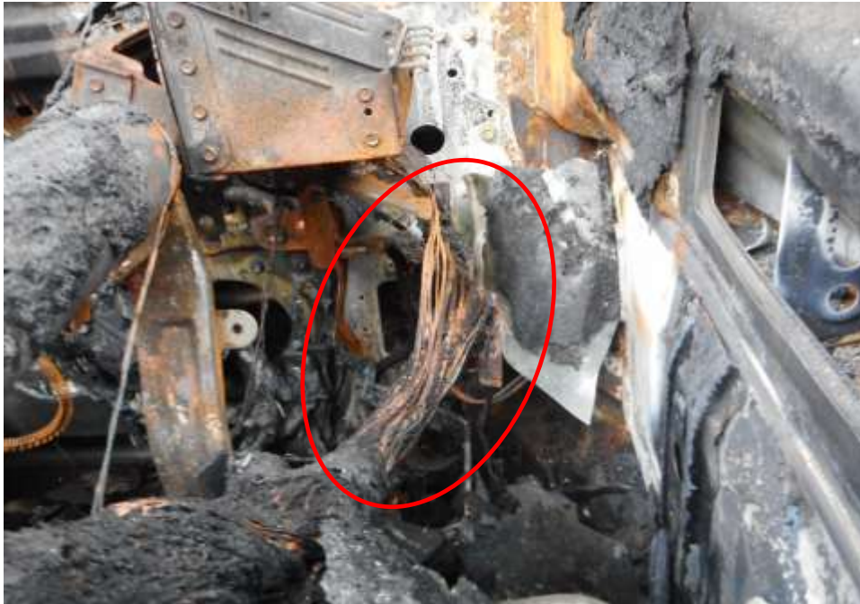
Photo 12 shows a general view of the original wiring harness in the engine compartment. The original wiring harness (circled) was observed with greenish residue on the surface. The presence of greenish residue indicates internal heating of copper wires, a sign of an electrical short circuit occurring. The greenish residue is normally left behind from oxidation as a result of chemical reaction involving the copper wires.
