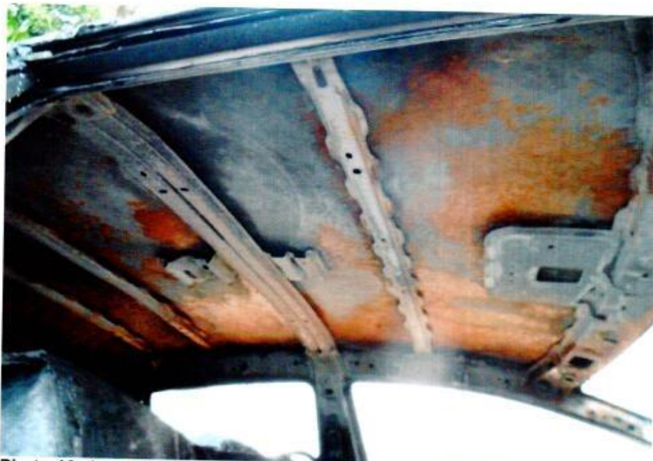
Photo 10 shows the underside of the front bonnet cover of the Insured Vehicle at the time of our inspection. The High heat intensity burn marks (whitish burn marks) and rust that had development found on the exterior surface of the bonnet indicates that the fire had originated from the front portion of the Insured Vehicle.
