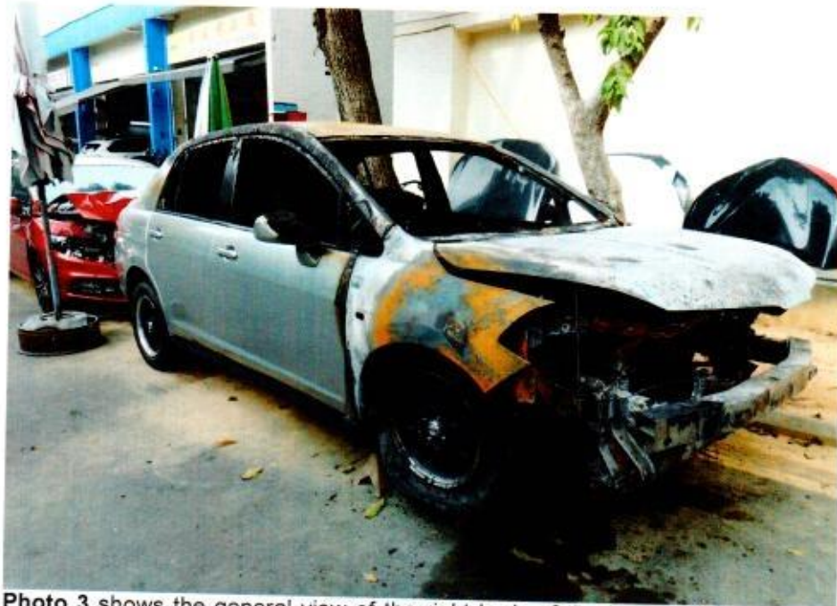
Photo 3 shows the general view of the right body of the Insured Vehicle at the time of our inspection. The Insured Vehicle was observed to have sustained extensive fire damage all around. Rust had accumulated all over the front and interior compartment of the Insured Vehicle as a result of exposure to environmental condition for a period of time.
