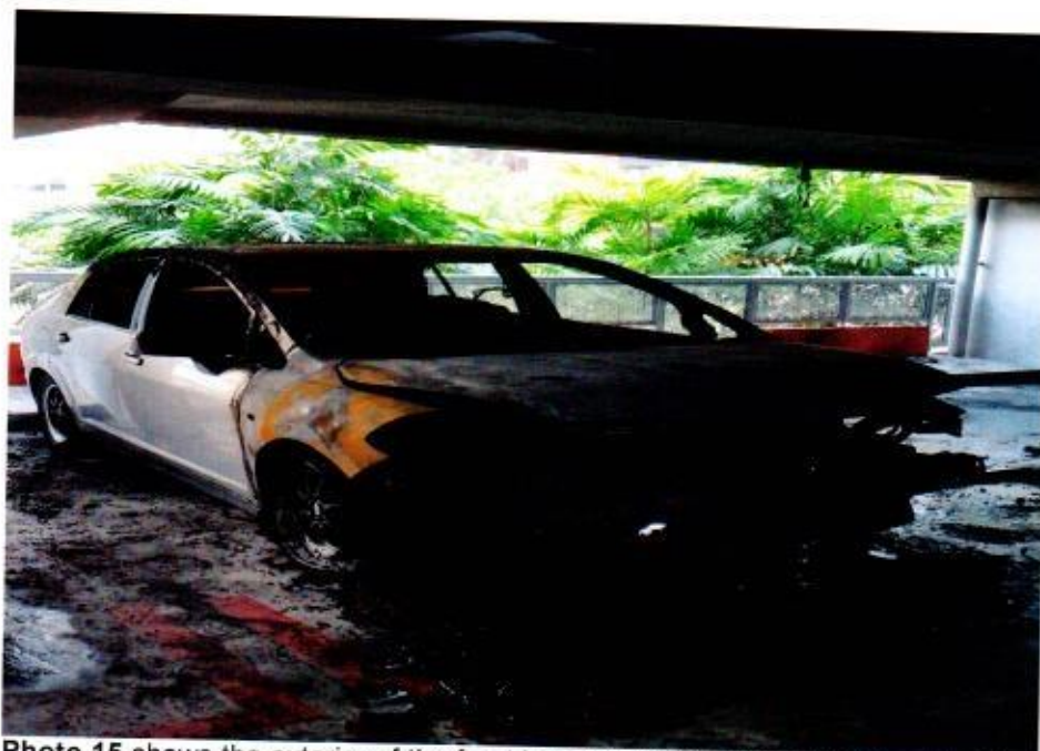
Photo 15 shows the exterior of the front bonnet of the Insured Vehicle at the time of our inspection. The high heat intensity burn marks (whitish burn marks) and rust that had development found on the exterior surface of the bonnet indicates that the fire had originated from the front portion of the Insured Vehicle. In general, the information that could be gathered from this photograph had corresponded to the events that were related to us by Mr Chow, location when the fire broke out.
