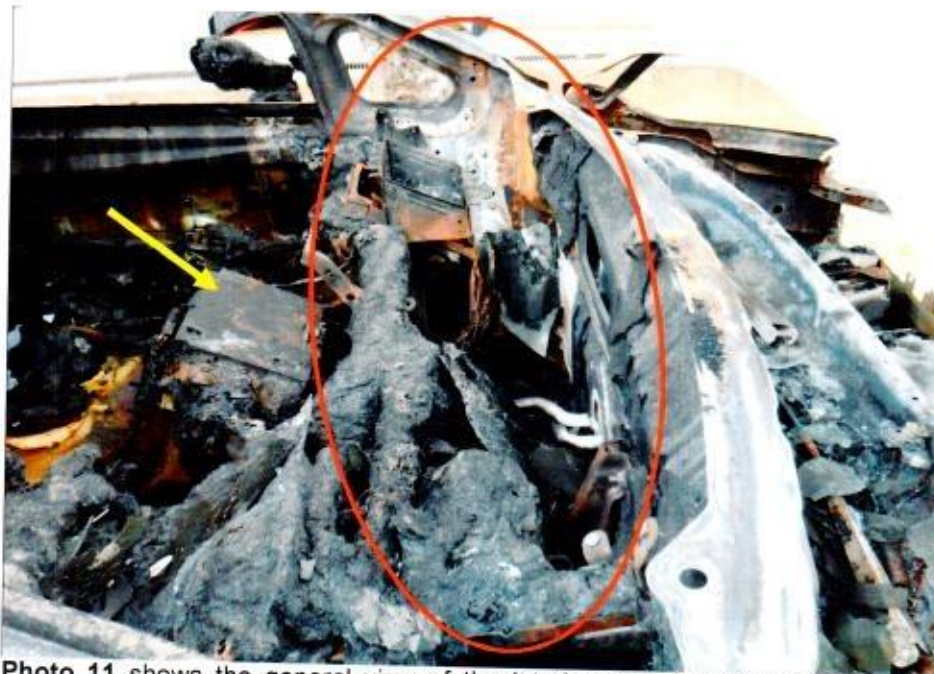
Photo 11 shows the general view of the interior compartment of the Insured Vehicle at the time of our inspection. The fire damage to the Insured Vehicle has affected its engine and interior compartment. Its interior dashboard (circled), radio head unit (yellow arrow), various original wiring harnesses was amongst the parts in the compartment that were found to have been affected as a result of the fire.
