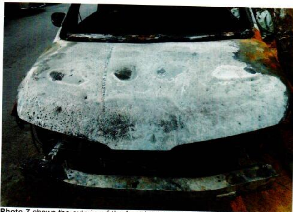
Photo 7 shows the exterior of the front bonnet of the Insured Vehicle at the time of our inspection. The high heat intensity burn marks (whitish burn marks) and rust that had development found on the exterior surface of the bonnet indicates that the fire had originated from the front portion of the Insured Vehicle.
