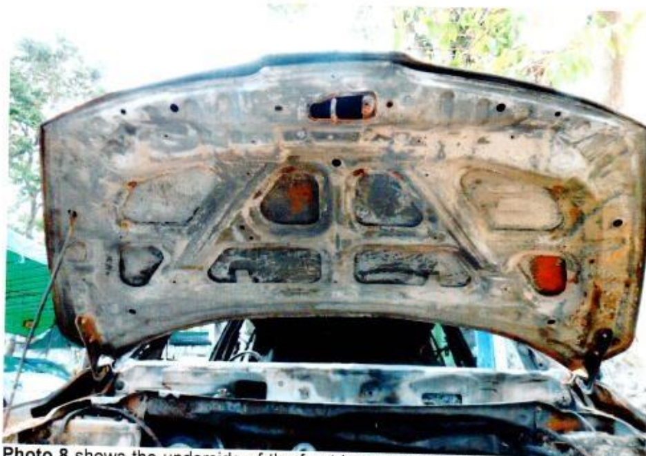
Photo 8 shows the underside of the front bonnet cover of the Insured Vehicle at the time of our inspection. The High heat intensity burn marks (whitish burn marks) and rust that had development found on the exterior surface of the bonnet indicates that the fire had originated from the front portion of the Insured Vehicle.
