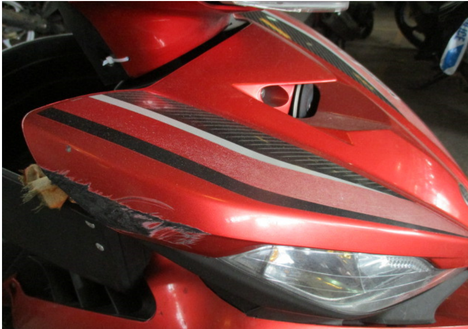
Photo 5 shows a closer view of the front cowling of the Motorcycle that had sustained damages of grazing nature as a result of the accident.
