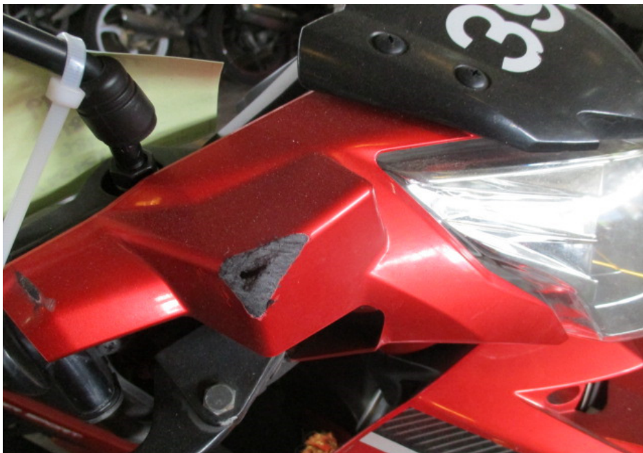
Photo 6 shows a close up view of the head cowling which was amongst the body parts of the Motorcycle that had sustained damage as a result of the accident.
