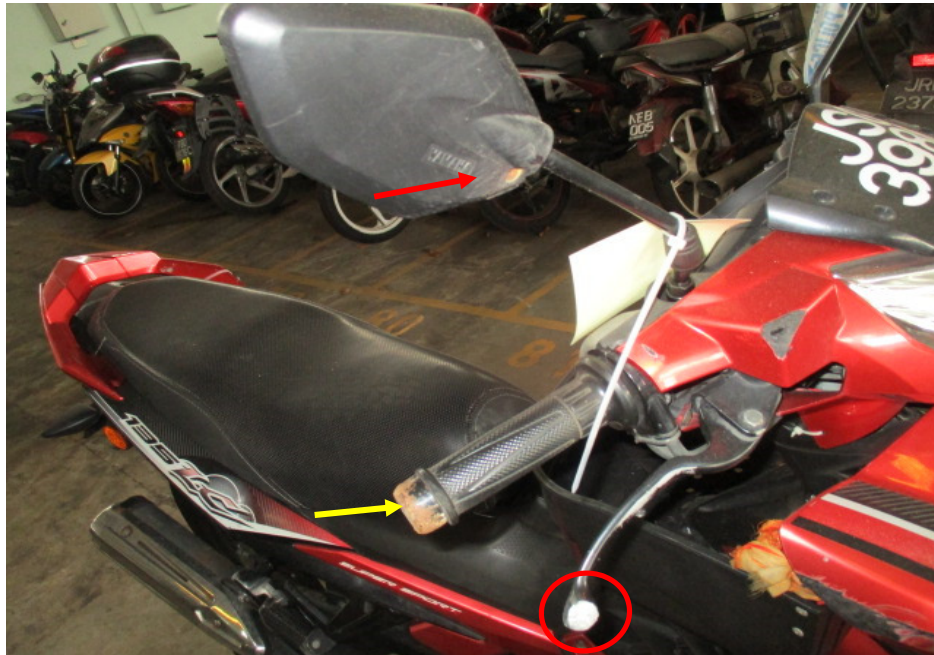
Photo 9 shows a closer view of the right handlebar end (yellow arrow), right side mirror (red arrow) and front brake lever (circled) which were amongst the body parts of the Motorcycle that had sustained damage as a result of the accident.
