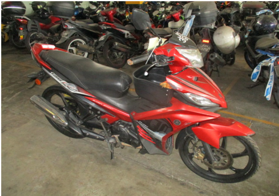
Photo 4 shows a general view of the right body of the Motorcycle at the time of our inspection. The Motorcycle was observed to have sustained damages at its frontal portion and right body. Amongst the body parts that were found to have been damaged include its head cowl, right side cowl, right handlebar end, right side mirror, front brake lever, rear brake pedal, right front footrest, right rear side cover and exhaust muffler, amongst others.
