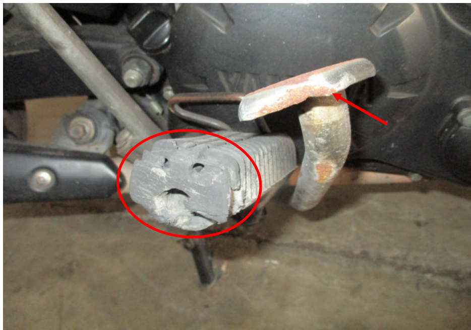
Photo 10 shows a closer view of the bent rear brake pedal (arrowed) and deformed right front footrest (circled) which were amongst the body parts of the Motorcycle that had sustained damage as a result of the accident.
