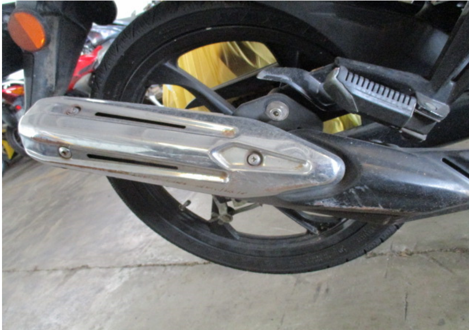
Photo 13 shows a closer view of the exhaust muffler and exhaust muffler heat shield of the Motorcycle that had sustained damages of grazing nature as a result of the accident.
