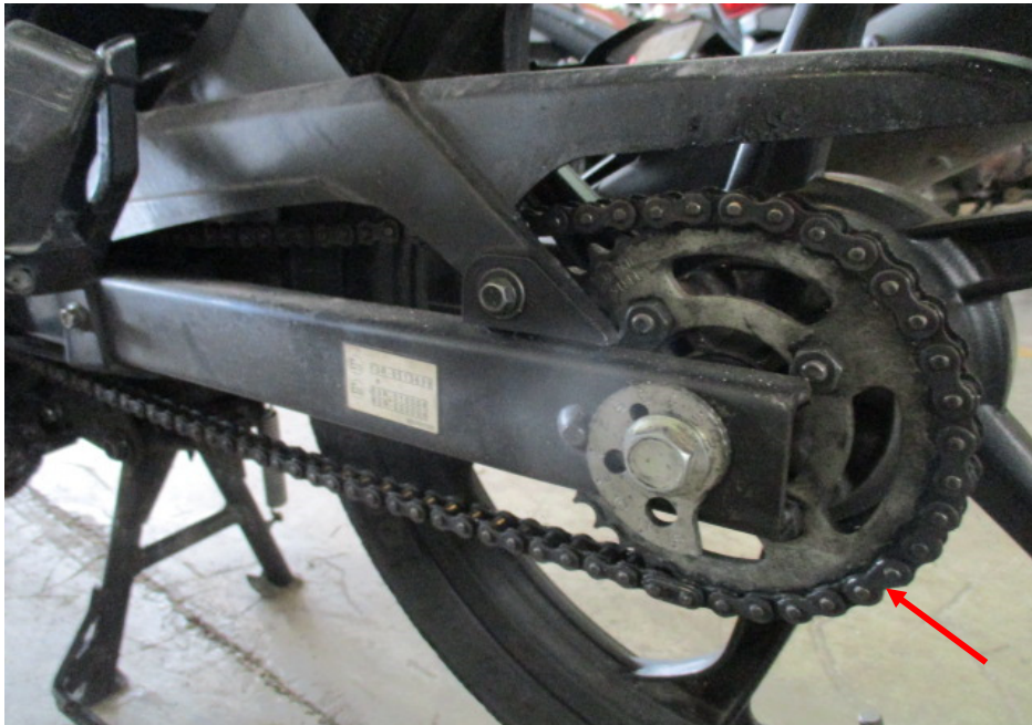
Photo 18 shows the general view of the gear train (arrowed) of the Motorcycle, which was observed to be intact with no misalignment. It was also adequately lubricated for operating purposes.
