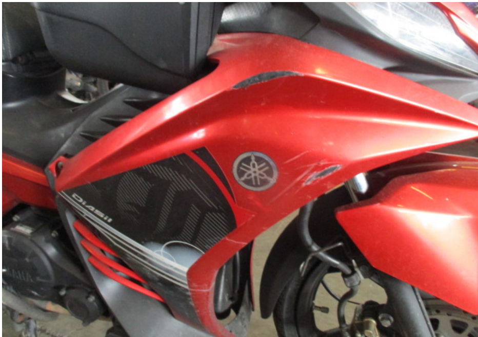
Photo 8 shows a closer view of the right cowl of the Motorcycle that had sustained damages of grazing nature as a result of the accident.
