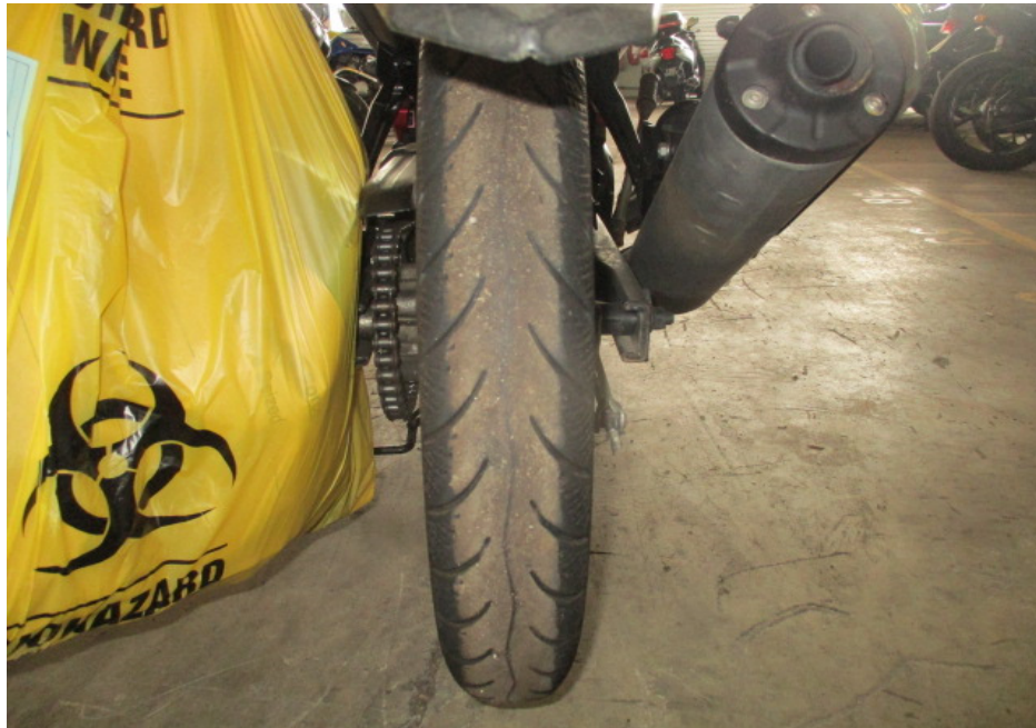
Photo 15 shows the condition of the Motorcycle's rear tyre. The rear tyre was observed to be bald at the centre portion. The tyre was also observed to be sufficiently inflated for vehicular operation. We did not observe any tear, burst mark(s) and/or punctured hole(s) on the sidewalls as well as across the tread of the rear tyre.
