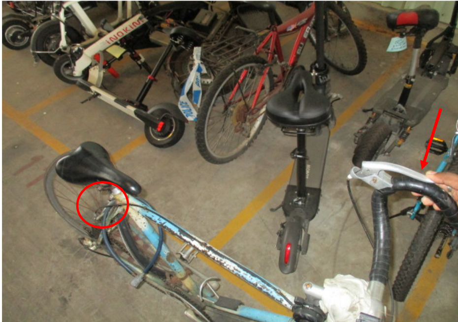
Photo 21 shows a static brake test conducted on the Bicycle's rear brake. It shows that the rear brake clamps responded to the gripping action (circled) after depressing the left hand brake lever (arrowed). However the rear brake clamp assembly was observed to be dislodged as a result of the accident, causing the rear rubber brake blocks to be misaligned from the rear wheel rim.
