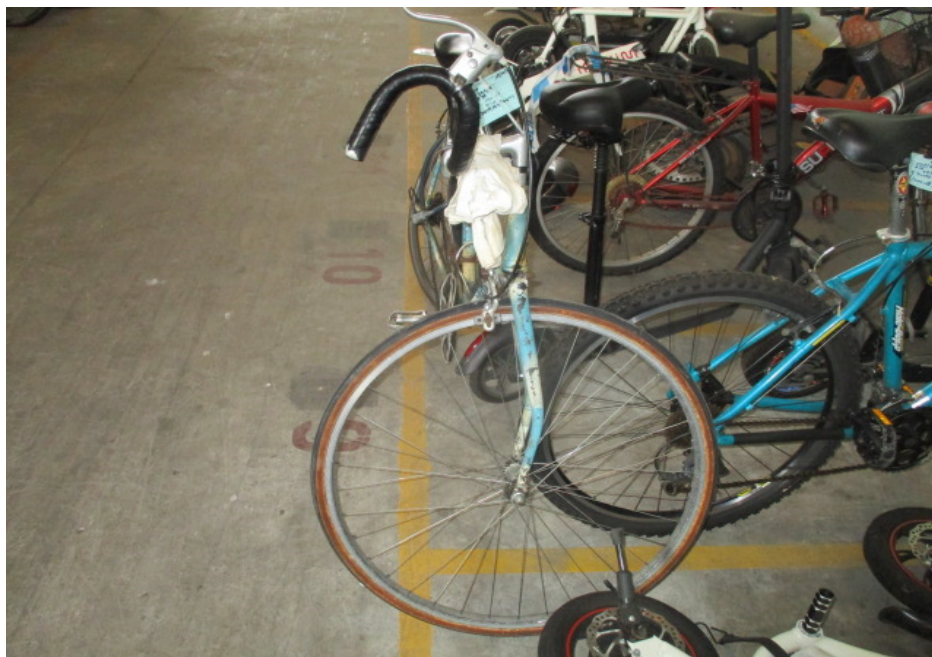
Photo 15 shows the front wheel of the Bicycle turned towards its full right. Turning the Bicycle's handle bar towards the right did not produce any abnormal free play and/or resistance. This would indicate that the steering system of the Bicycle was in serviceable condition at the time of our inspection.
