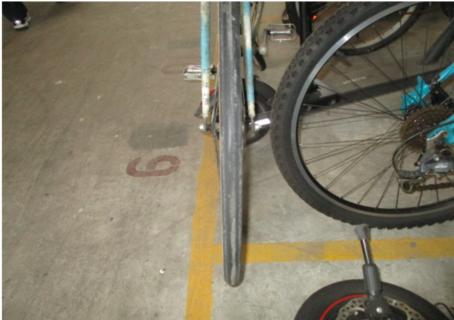
Photo 9 shows the front tyre of the Bicycle. The pattern of the tread was clearly visible. There was no tear, burst mark(s) and/or punctured hole(s) on the sidewalls as well as across the tread of the front tyre.
