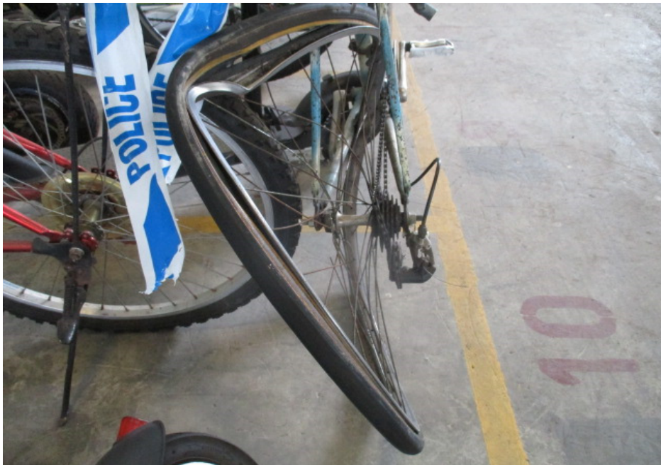
Photo 10 shows the rear tyre of the Motorcycle. The pattern of the tread was clearly visible. There was no tear, burst mark(s) and/or punctured hole(s) on the sidewalls as well as across the tread of the front tyre. However the rear tyre was observed to be deflated due to the bent rear wheel rim.
