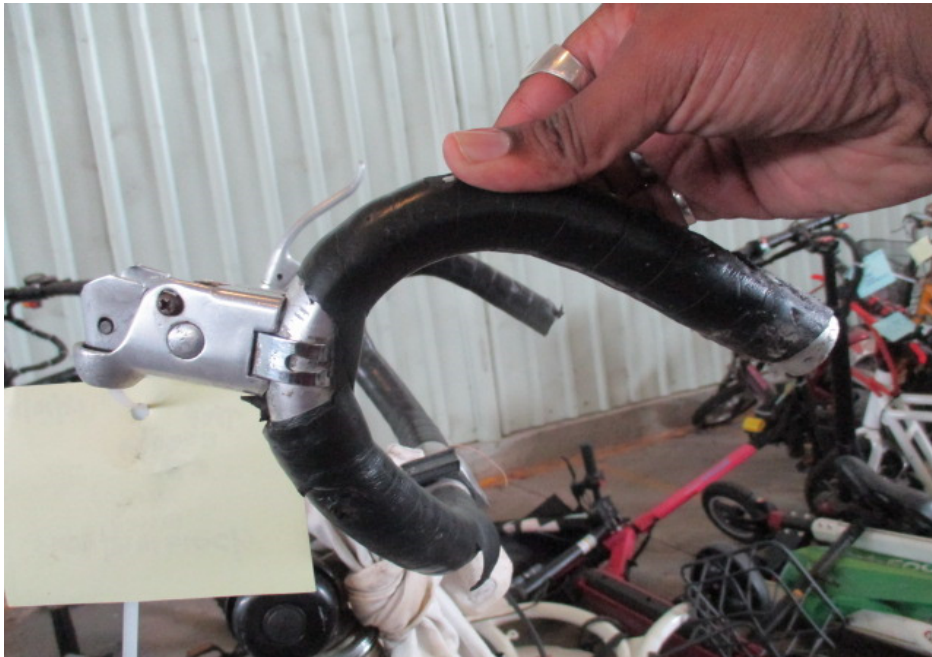
Photo 5 shows the damaged right handlebar grip of the Bicycle at the time of our inspection.
