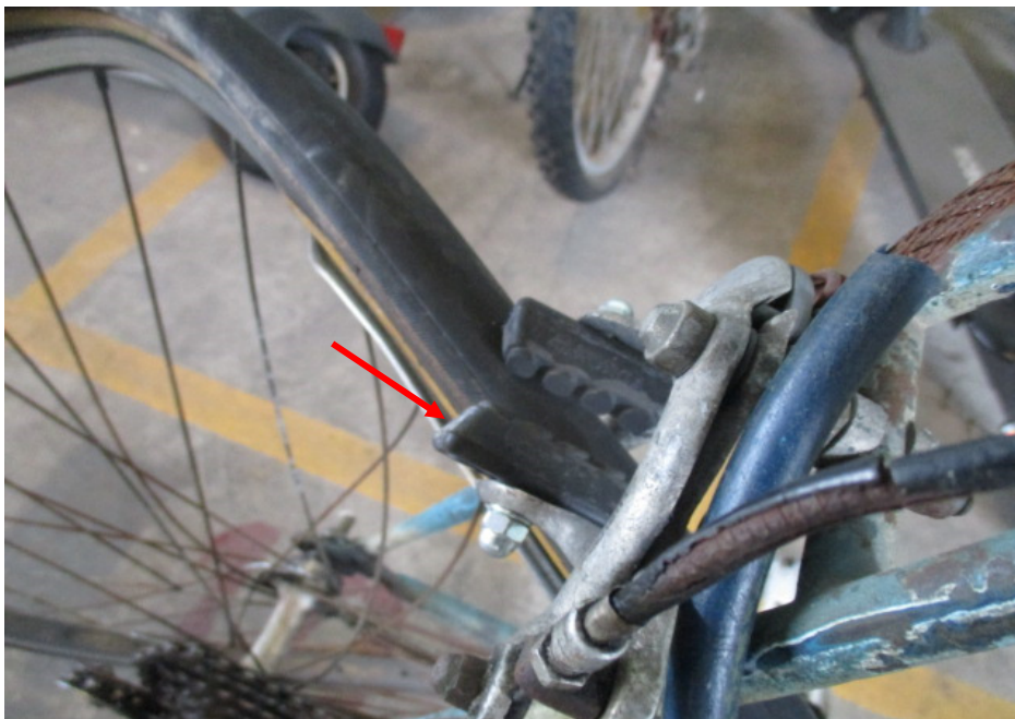
Photo 22 shows a close up view of the rear brake rubber brake blocks which responded to the gripping action after depressing the left hand brake lever. However they were observed to be misaligned from the rear wheel rim (arrowed) due to the dislodgement of the rear brake clamp assembly and broken rear wheel rim as a result of the accident.
