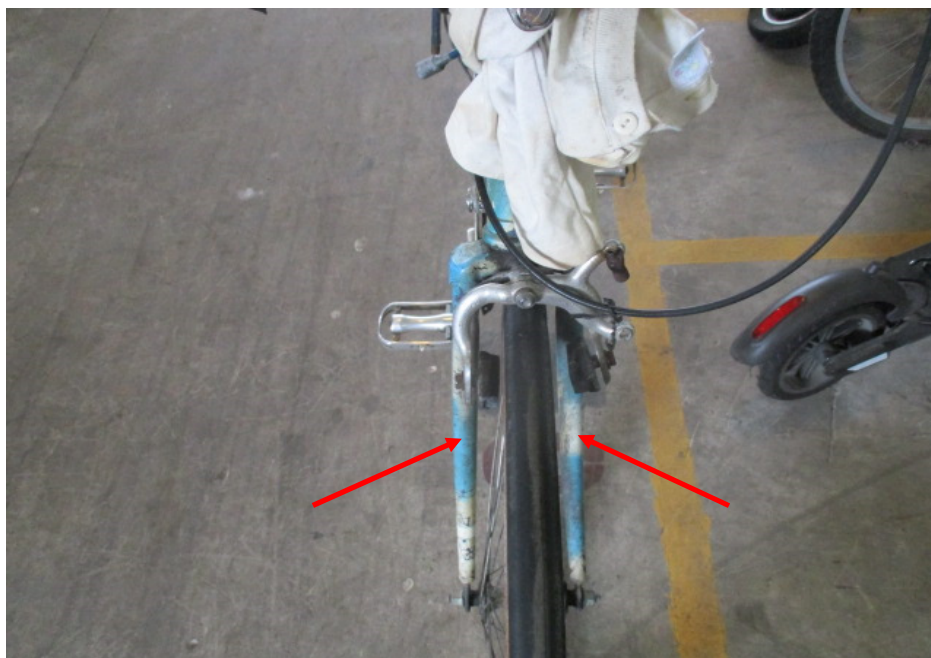
Photo 14 shows the front fork (arrowed) of the Bicycle. The front fork and fork bracket of the Bicycle were both found to be intact and undamaged. Turning the Bicycle's handle bar towards the left and right did not produce any abnormal free play. The steering system of the Bicycle was in serviceable condition at the time of our inspection.
