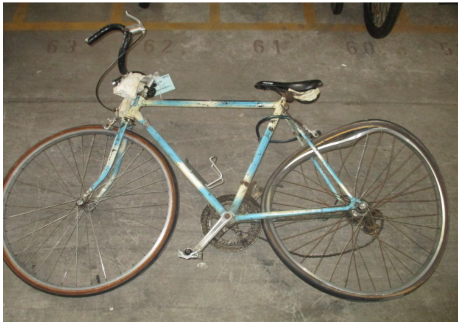
Photo 2 shows the left portion of the Bicycle at time of our inspection. The bicycle had sustained damages to its right and rear portion. The body parts that were found to have been damaged include its handlebar, frame, rear braking components & gear train, amongst others as a result of the accident.
