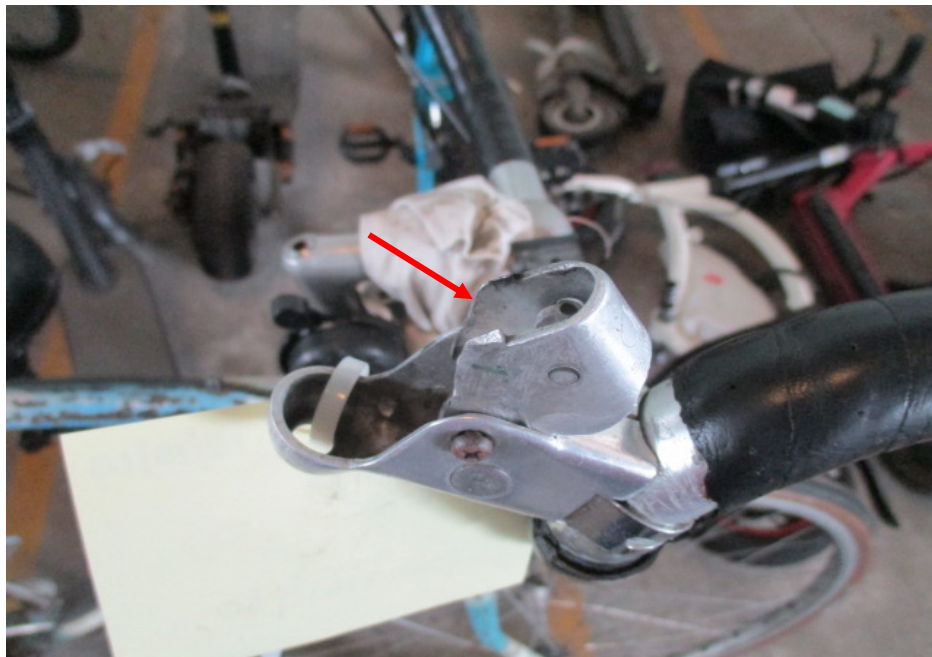
Photo 19 shows the broken front brake lever as a result of the accident (arrowed). Hence a static brake test could not be conducted on the Bicycle's front braking system.
