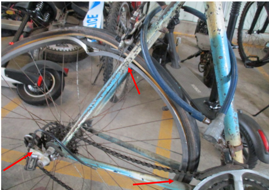
Photo 8 shows a close-up view of the rear sub frame and gear train (arrowed) of the Bicycle at the time of our inspection. These components were observed to be pushed against the rear tyre of the Bicycle as a result of the accident.
