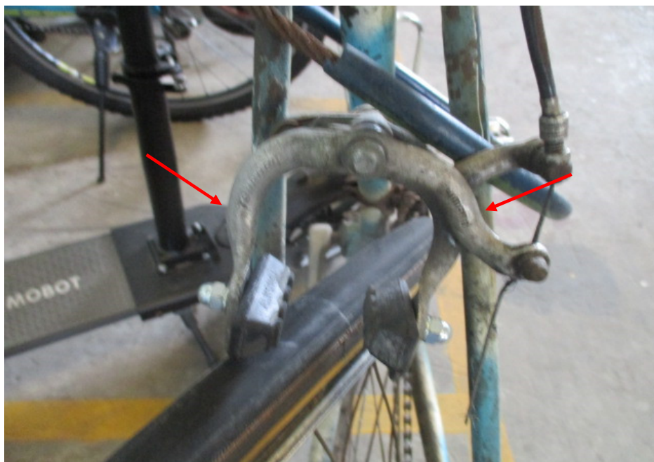
Photo 20 shows the rear brake clamp assembly which was observed to be dislodged as a result of the accident (arrowed).
