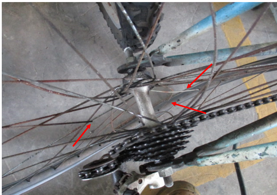
Photo 12 shows the broken spokes on the rear wheel rim of the Bicycle at the time of our inspection (arrowed).
