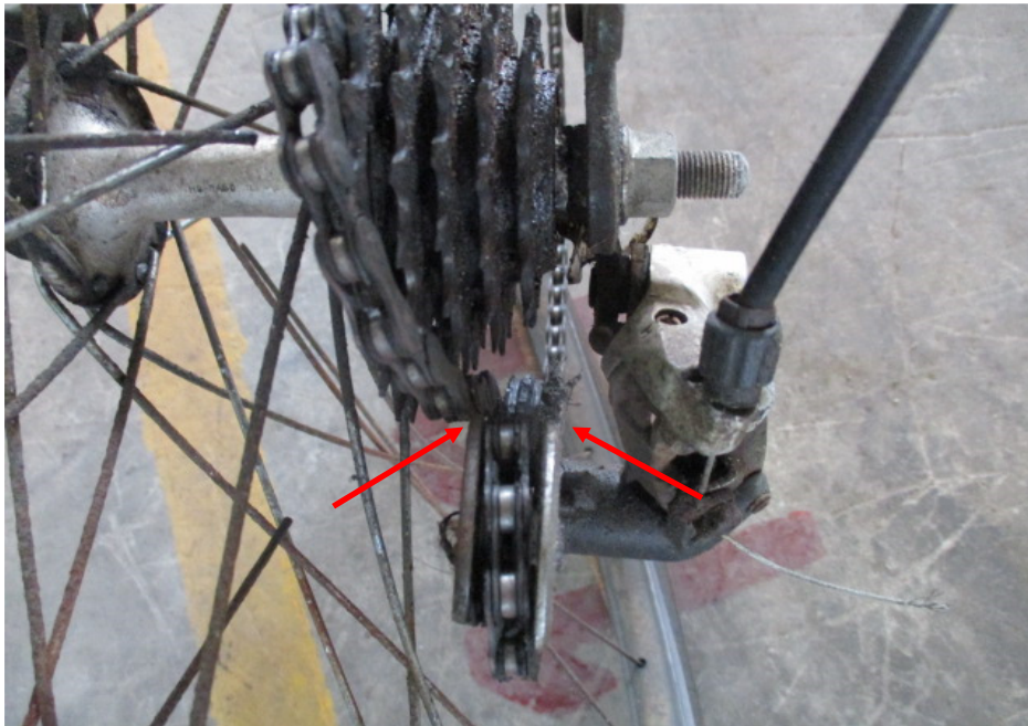
Photo 13 shows a close up view of the gear train of the Bicycle, which was observed to have sustained severe damages as a result of the accident (arrowed).
