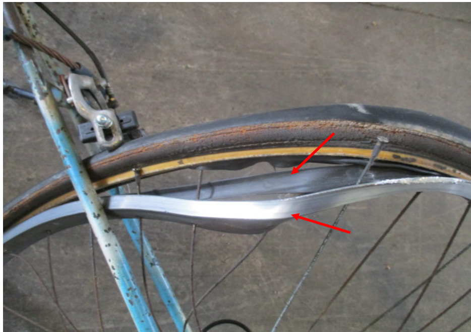
Photo 11 shows the bent rear wheel rim of the Bicycle at the time of our inspection (arrowed).
