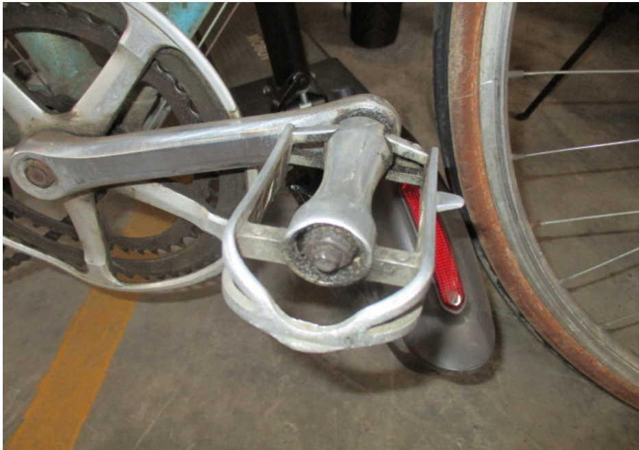
Photo 7 shows the damaged right pedal of the Bicycle at the time of our inspection.
