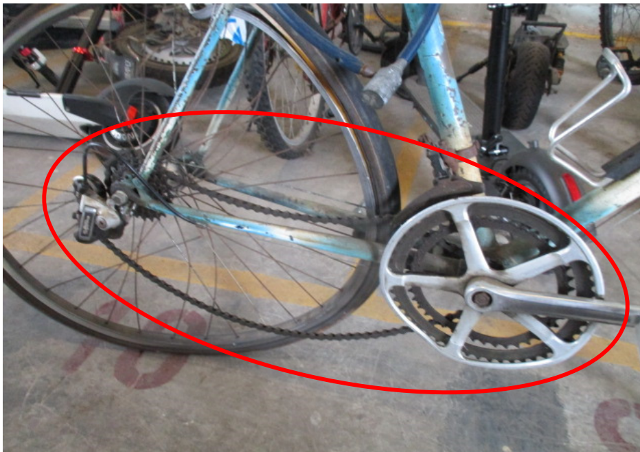
Photo 6 shows a close-up view of the drive train of the Bicycle at the time of our inspection. It was observed to have sustained damages at the circled area of the Bicycle due to the accident.
