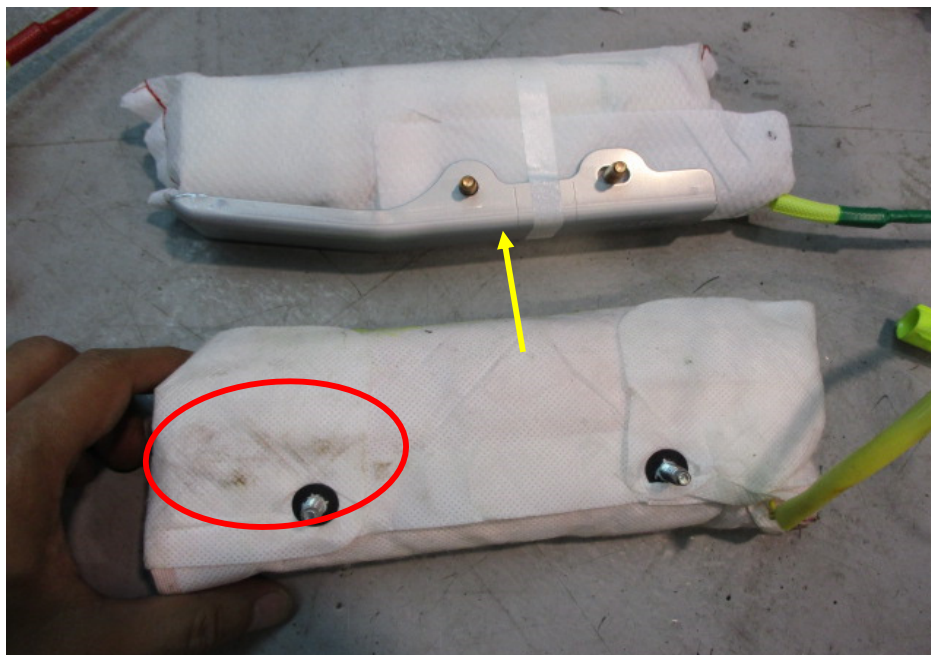
Photo 17 shows the back of the driver's seat airbag that was fitted on the Insured Vehicle in comparison with a new driver's seat airbag. Notably, the driver's seat airbag fitted on the Insured Vehicle was observed to be in a relatively dirty condition (red circle). A bracket (yellow arrow) on the exterior of the new driver's seat airbag was observed to be covered for the driver's seat airbag that was fitted on the Insured Vehicle. The covering of the bracket is an indication that the driver's airbag fitted on the Insured Vehicle was re-folded after activation; and is a re-used airbag.
