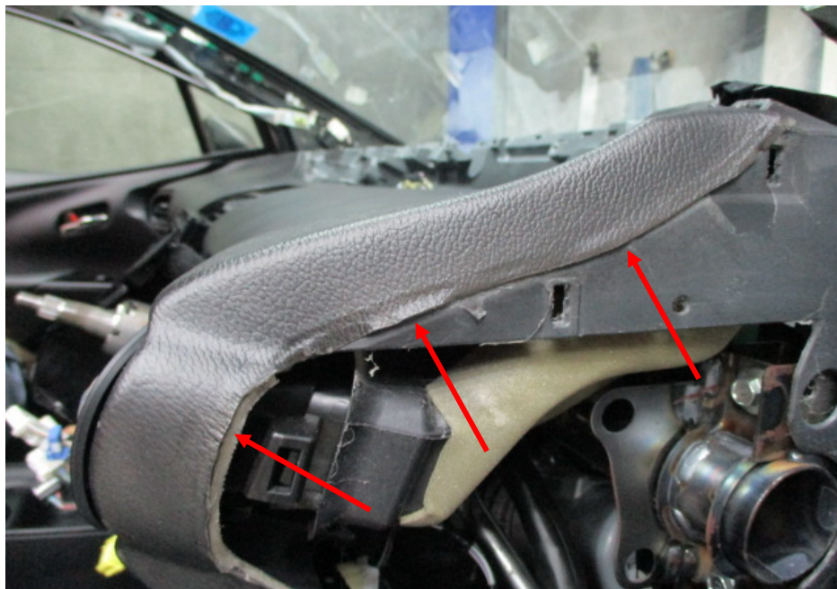
Photo 25 shows the front dashboard that was fitted on the Insured Vehicle. This was at the driver's side of the front dashboard. Signs of re-pasting (arrowed) of the front surface material onto the frame of the front dashboard was observed.
