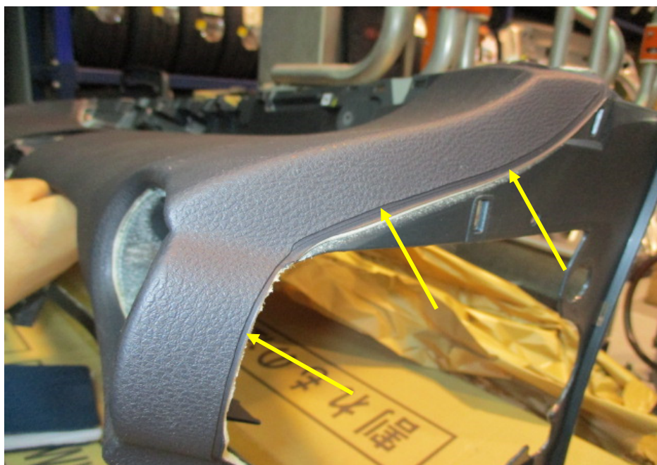
Photo 26 shows a new front dashboard, at the same area as shown in photograph 25 above. In comparison, the front surface material of the new front dashboard was nicely pasted onto the frame of the front dashboard. No peeling off, similar to photograph 25, of the ends of the front surface material were seen on the new front dashboard.
