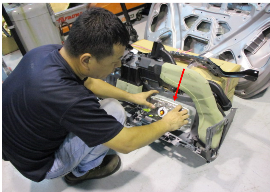
Photo 6 shows dismantling of the Insured Vehicle's front left passenger airbag (arrowed) after the front dashboard was dismantled.
