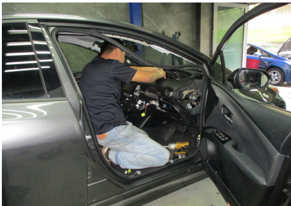
Photo 2 shows dismantling works being carried out to the Insured Vehicle in my presence. For this inspection, the driver's airbag, front left passenger airbag, driver's seat airbag, front left passenger seat airbag, left side curtain airbag, right side curtain airbag and front dashboard that were fitted on the Insured Vehicle were all dismantled and physically compared with new parts.
