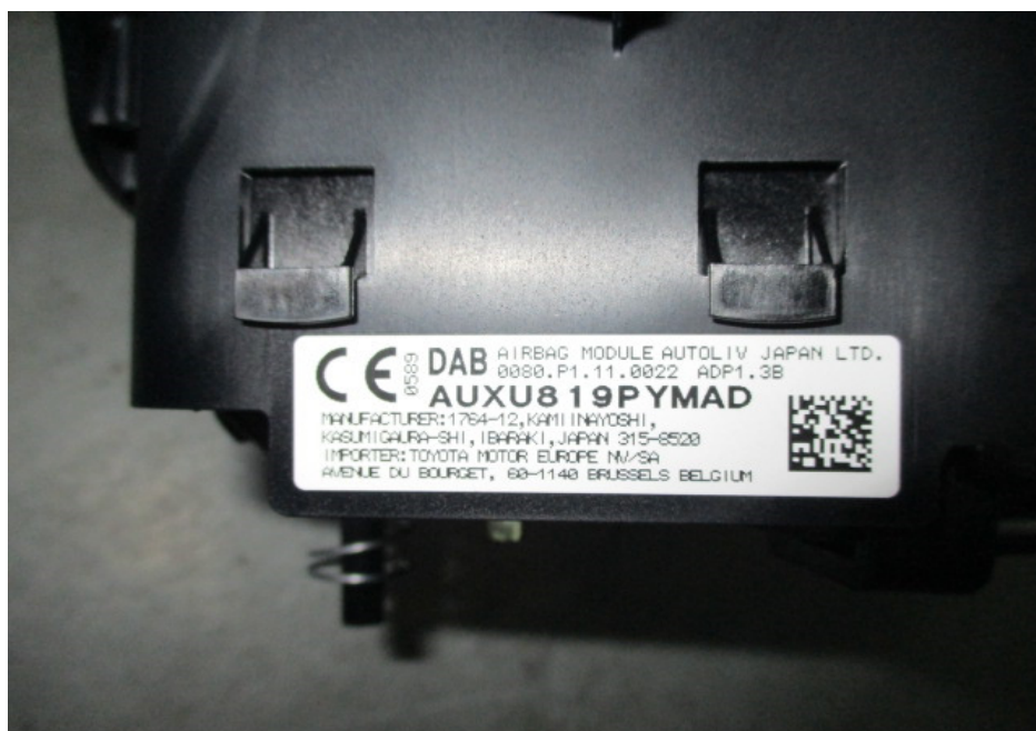
Photo 5 shows a closer view of the sticker label that was pasted on the cover of a new driver's airbag. The sticker label had indicated the manufacturer and importer of the driver's airbag.
