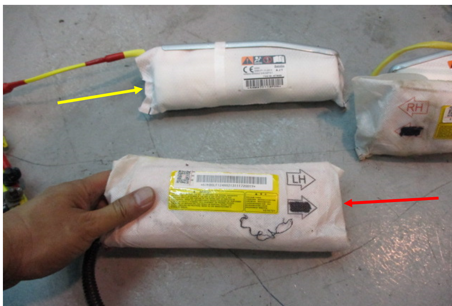
Photo 18 shows a closer view of the comparison between the front left passenger seat airbag (red arrow) that was fitted on the Insured Vehicle with a new front left passenger seat airbag (yellow arrow).
