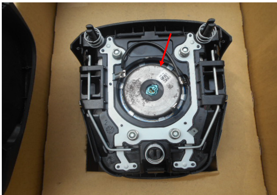
Photo 6 shows a closer view of the driver's airbag for a similar make and model vehicle. The airbag propellant (arrowed) was observed to be smaller in size as compared to the propellant for the driver's airbag of the Insured Vehicle. There was also no sticker label on the propellant for the driver's airbag for a similar make and model vehicle.
