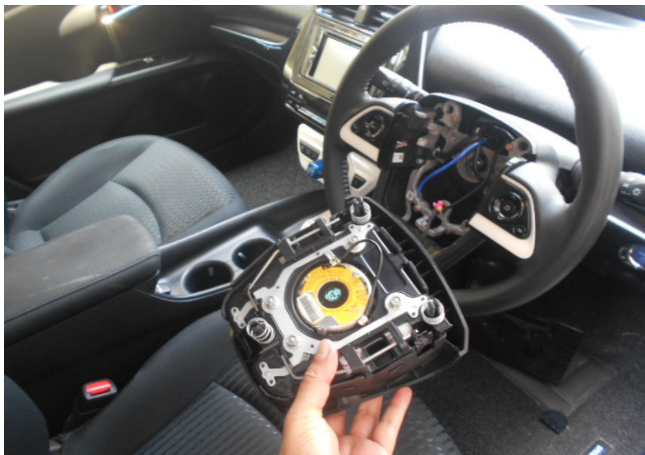
Photo 3 shows a back view of the driver's airbag of the Insured Vehicle after it was removed from the steering wheel of the Insured Vehicle.
