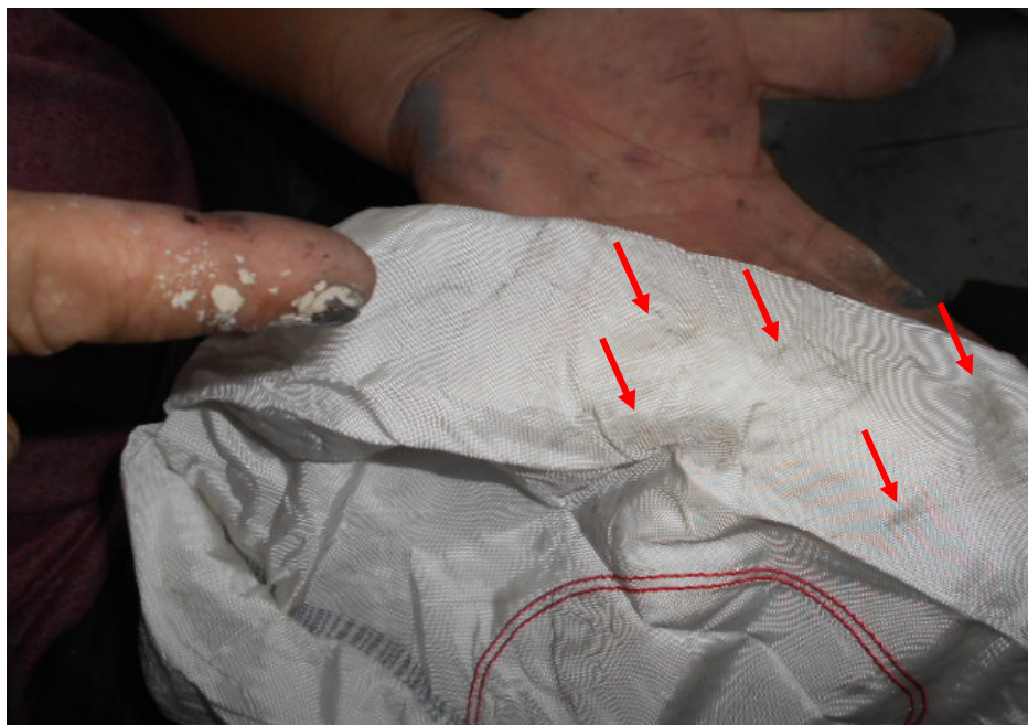
Photo 9 shows the airbag after it was unfolded. The airbag was found to be dirty with black stain marks (arrowed) at multiple areas.
