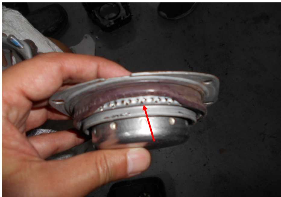
Photo 12 shows airbag propellant not completely sealed at one area, exposing the airbag propellant (arrowed).
