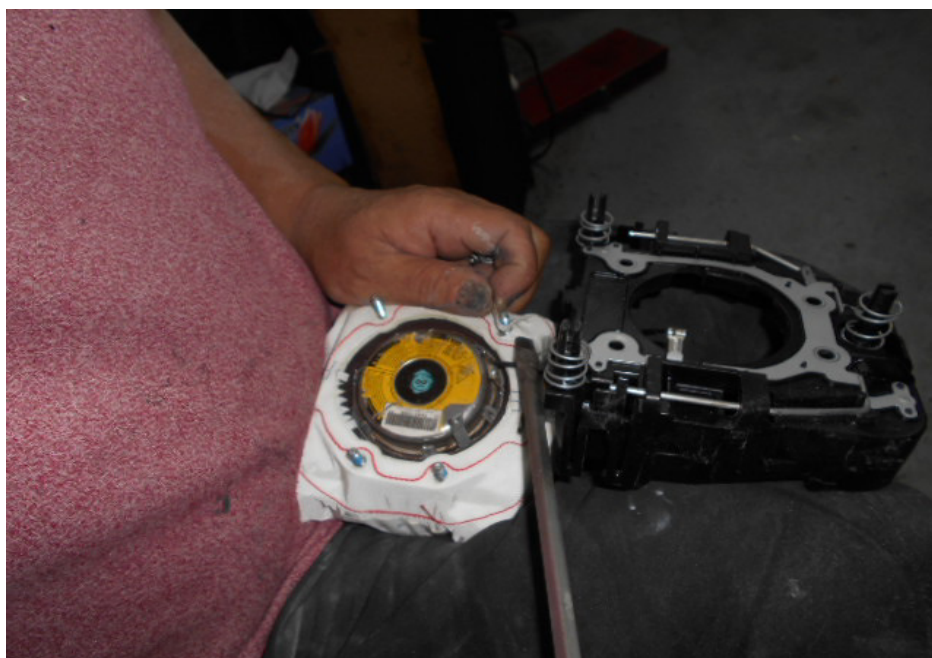
Photo 8 shows dismantling of the driver's airbag of the Insured Vehicle. This was carried out for the purpose of checking the interior of the driver's airbag of the Insured Vehicle. Dismantling was carried out by an airbag specialist in my presence.
