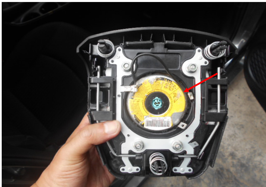
Photo 5 shows a closer view of the driver's airbag of the Insured Vehicle. The size of the airbag propellant (arrowed) was observed to be bigger when compared with a driver's airbag for a similar make and model vehicle. The sticker label on the propellant was also observed to be partially torn off and worn looking.
