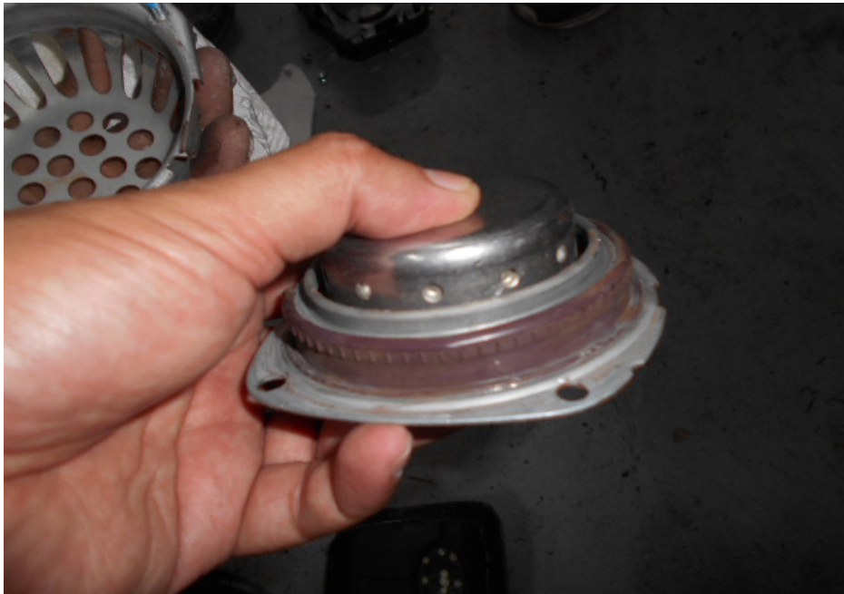
Photo 13 shows other areas of the airbag propellant for the driver's airbag of the Insured Vehicle. On comparison, the other areas of the propellant were observed to be completely sealed.
