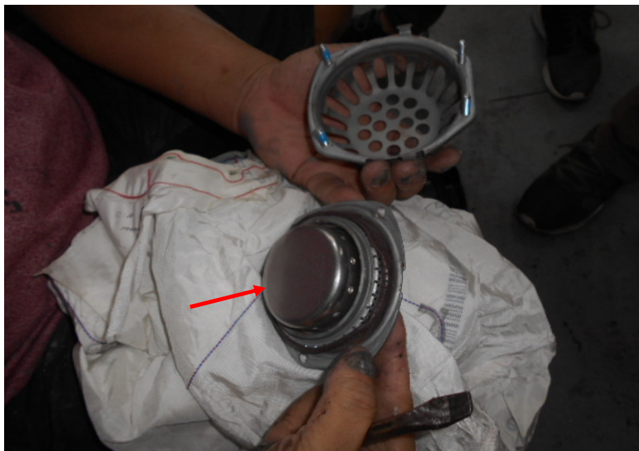
Photo 11 shows the bigger size airbag propellant (arrowed) for the driver's airbag of the Insured Vehicle after the airbag was removed.
