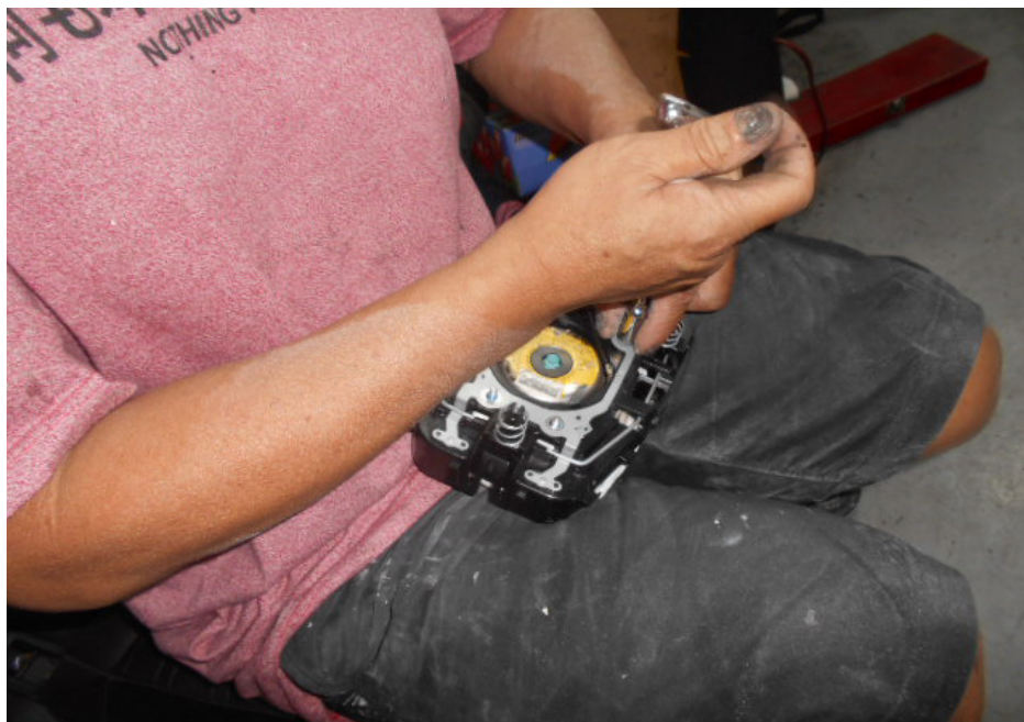
Photo 7 shows dismantling of the driver's airbag of the Insured Vehicle. This was carried out for the purpose of checking the interior of the driver's airbag of the Insured Vehicle. Dismantling was carried out by an airbag specialist in my presence.
