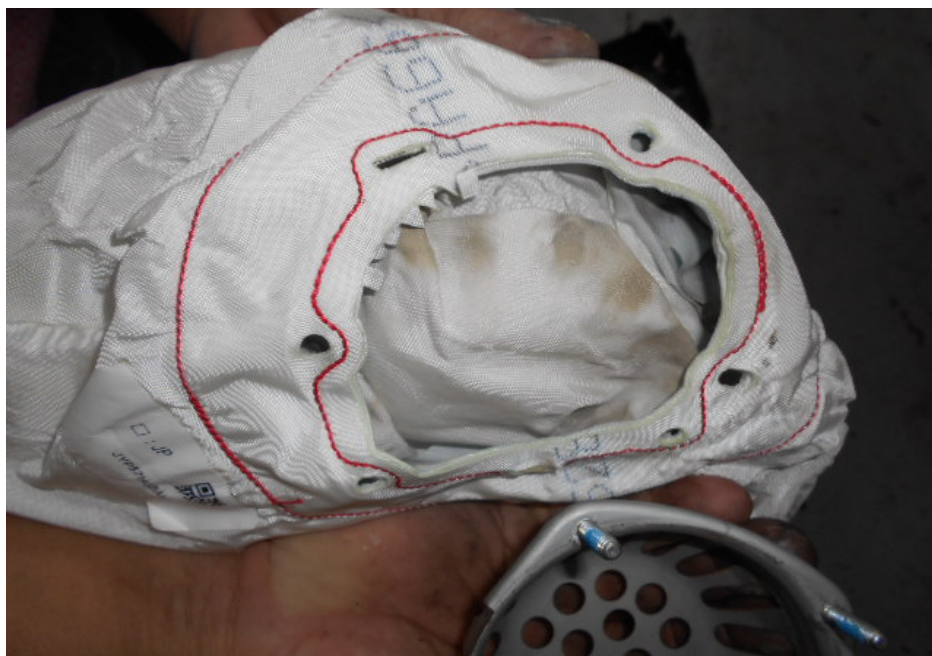
Photo 10 shows the airbag after it was unfolded. The airbag was found to be dirty with black stain marks at multiple areas.
