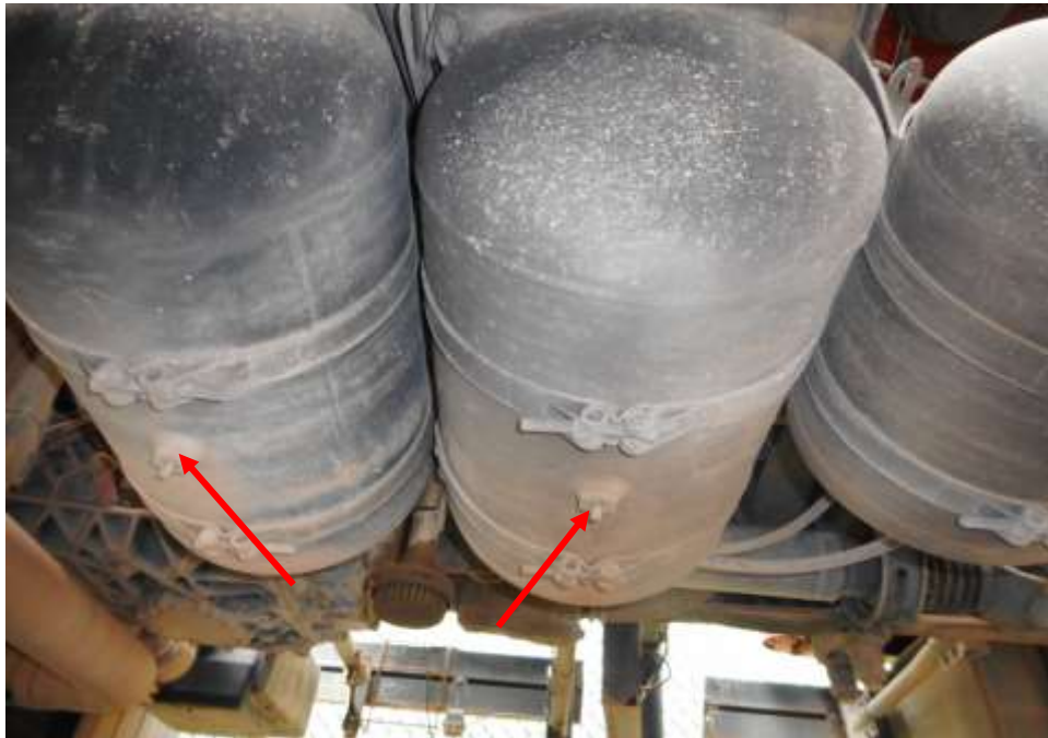
Photo 20 shows the air brake cylinders (arrowed) at the undercarriage of the Motor Lorry. I did not observe any leakage of air brake fluid at the time of my inspection of the Motor Lorry. My static tests of the Motor Lorry's braking system, along with my visual examination of the various mechanical components in the braking system had indicated that there was no internal leakage of pressure/vacuum. Hence the braking system of the Motor Lorry was likely to be in serviceable condition at the material time of accident.
