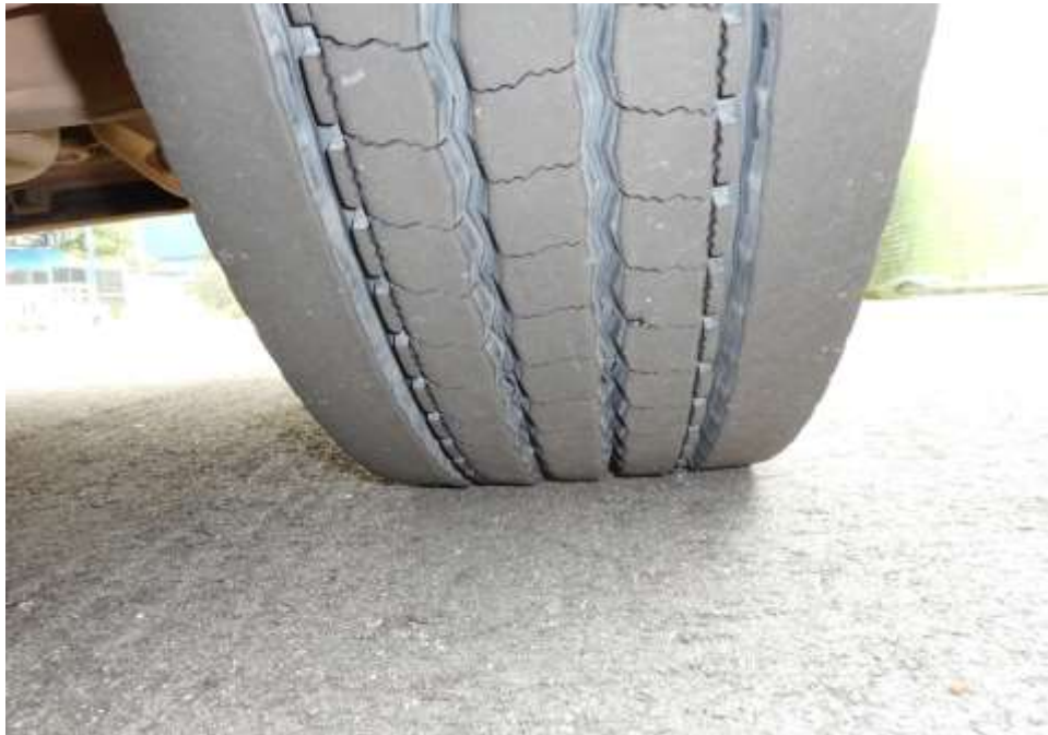
Photo 6 shows the condition of the front right tyre of the Motor Lorry, which was observed to be in serviceable condition with remaining tread depth of approximately 14 mm. The tyre, which was wrapped around standard steel wheel rim, was also observed to be sufficiently inflated for vehicular operation. There was no tear, cut or burst mark(s) on the outer and the inner sidewalls as well as across the tread of the 10 tyres that were fitted on the Motor Lorry.
