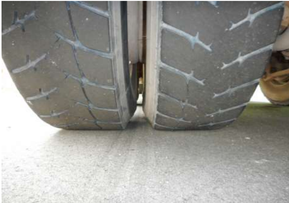
Photo 8 shows the condition of the rear left tyres of the Motor Lorry, which was observed to be in serviceable condition with remaining tread depth of approximately 5.6mm. The tyres, which were wrapped around standard steel wheel rim, were also observed to be sufficiently inflated for vehicular operation. There was also no damage found on all 10 steel wheel rims of the Motor Lorry.
