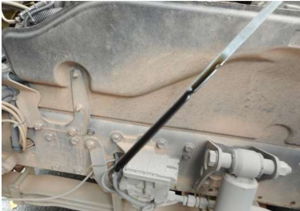
Photo 14 shows the engine oil level display of the Motor Lorry at the time of my inspection. The engine oil was observed to be of sufficient level.
