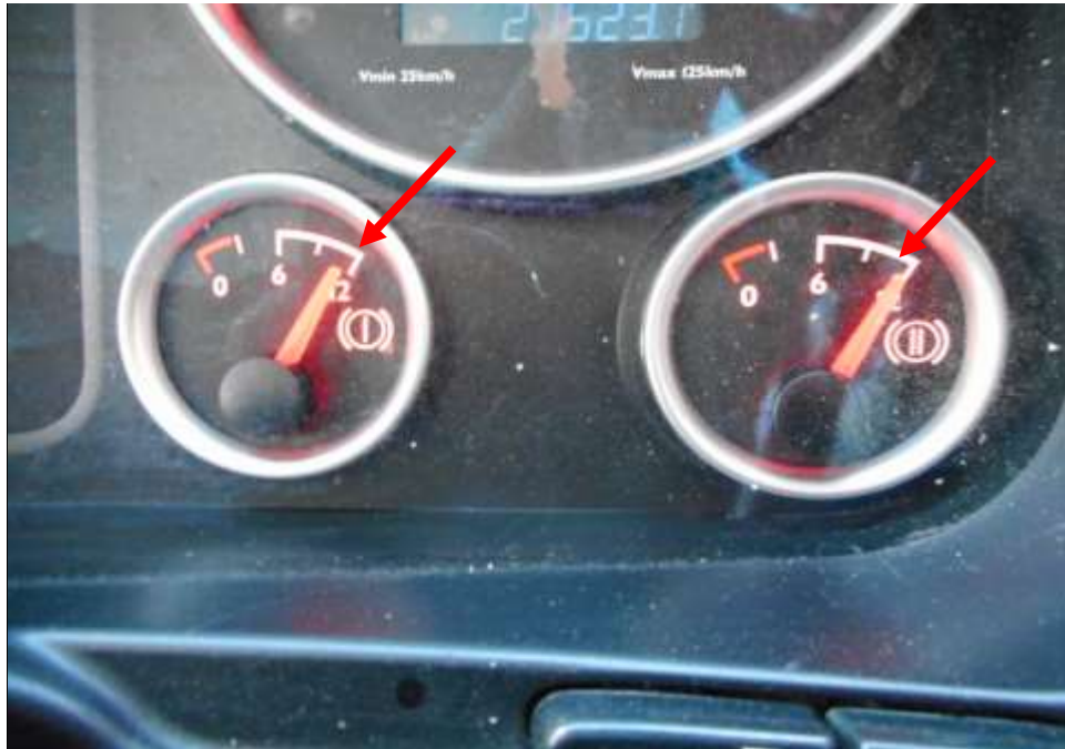
Photo 11 shows the air in the air brake cylinders of the Motor Lorry at the time of my inspection. The air in the cylinder was observed to be of sufficient level & serviceable at the time of the accident.
