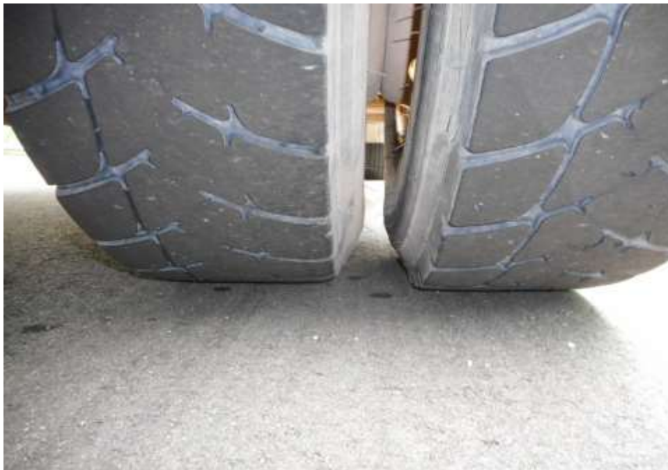
Photo 7 shows the condition of the rear right tyre of the Motor Lorry, which was observed to be in serviceable condition with remaining tread depth of approximately 6.7mm. The tyre, which was wrapped around standard steel wheel rim, was also observed to be sufficiently inflated for vehicular operation.
