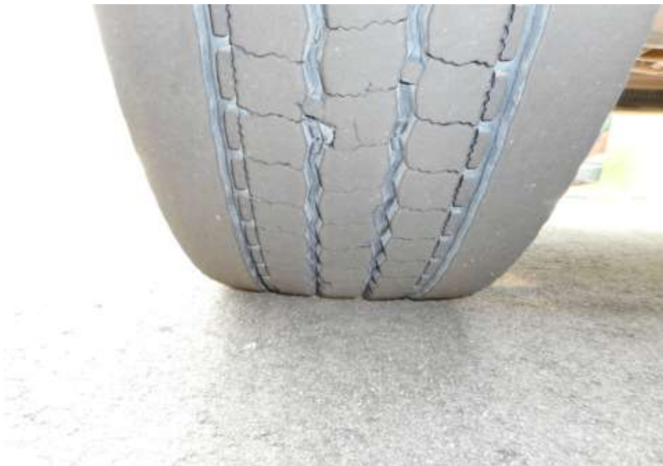
Photo 9 shows the condition of the front left tyres of the Motor Lorry, which were observed to be in serviceable condition with remaining tread depth of approximately 9.6mm. There was also no tear, cut or burst mark(s) on the outer and the inner sidewalls as well as across the tread of the 10 tyres that were fitted on the Motor Lorry.
