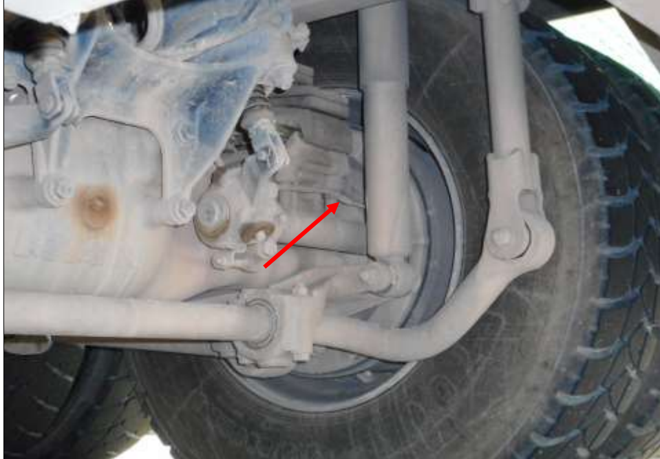
Photo 16 shows the brake pipe (arrowed) at the rear right wheel of the Motor Lorry. I did not observe any leakage of brake fluid at the time of my inspection of the Motor Lorry. My static tests of the Motor Lorry's braking system, along with my visual examination of the various mechanical components in the braking system, had indicated that there was no internal leakage of pressure/vacuum. Hence the braking system of the Motor Lorry was likely to be in serviceable condition at the material time of accident.
