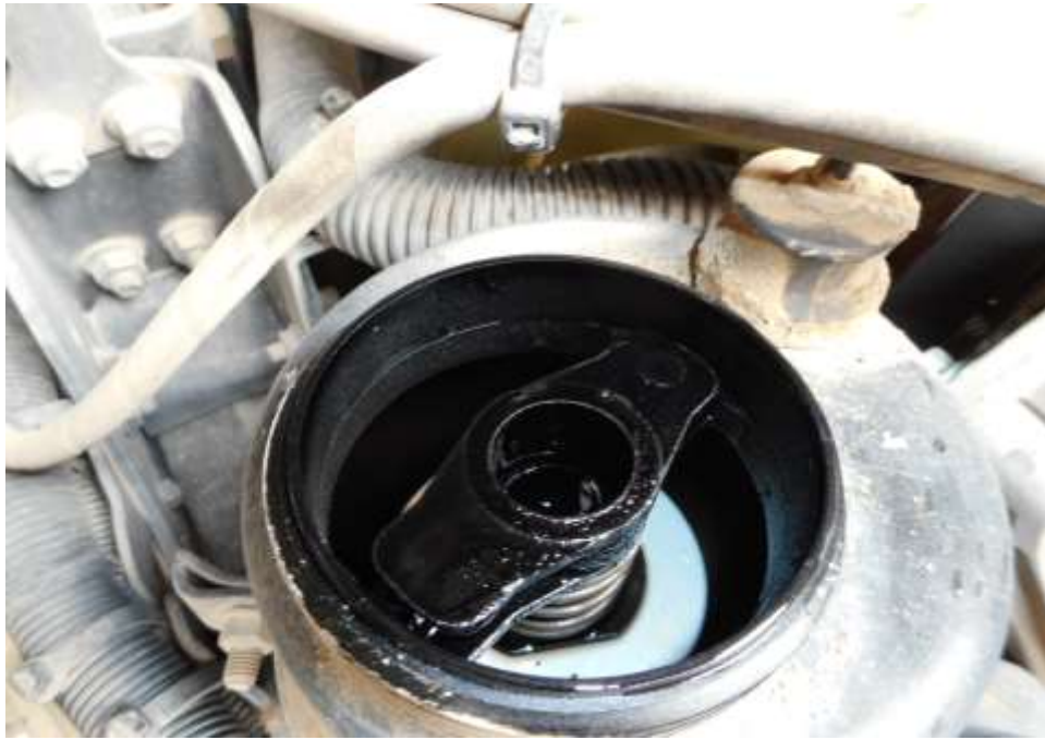
Photo 13 shows the power steering fluid reservoir of the Motor Lorry at the time of my inspection. The power steering fluid was observed to be of sufficient level and without any visible contamination.
