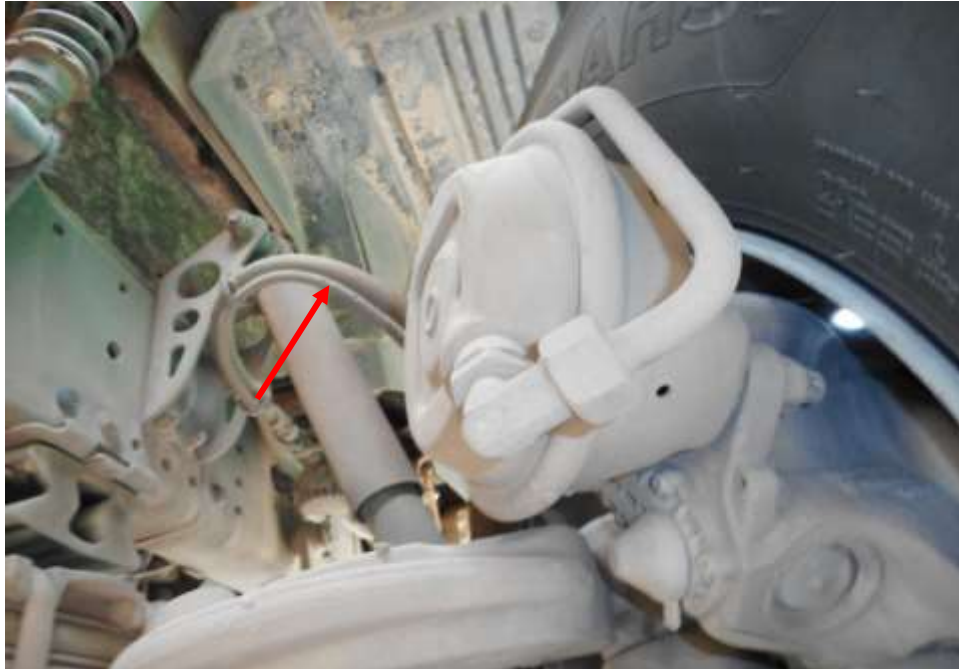
Photo 19 shows the brake pipe (arrowed) at the front right wheel of the Motor Lorry. I did not observe any leakage of brake fluid at the time of my inspection of the Motor Lorry. My static tests of the Motor Lorry's braking system, along with my visual examination of the various mechanical components in the braking system had indicated that there was no internal leakage of pressure/vacuum. Hence the braking system of the Motor Lorry was likely to be in serviceable condition at the material time of accident.
