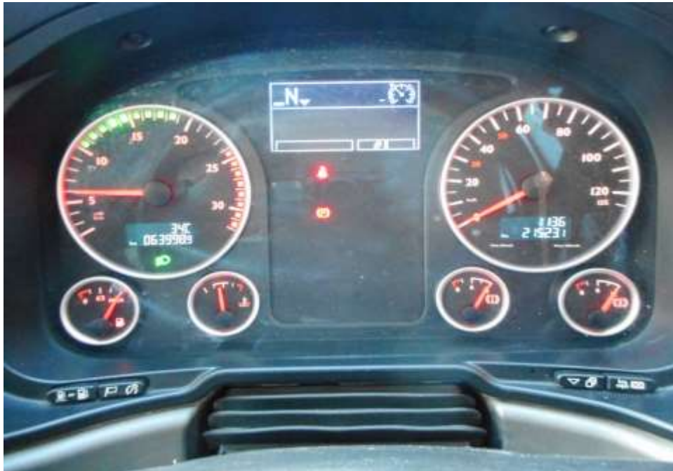
Photo 26 shows no warning lights illuminated on the instrument panel of the Motor Lorry after the engine was cranked. This would suggest that there was no abnormality to the various electronic operating systems of the Motor Lorry, like the ABS etc.
