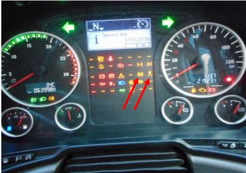
Photo 25 shows the warning light for Anti-Lock Brake System (ABS) and Traction Control System (TC) (arrowed) appearing on the instrument panel of the Motor Lorry during the self-test of its various electronic operating systems when its engine was cranked.
