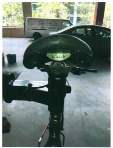
a. The saddle rails have twisted and are no longer balanced with one rail higher than the other. This cause the saddle to be lopsided and no longer support the rider with proper comfort and stress relieve. Continue usage may cause the rails to deform further. This is common and may occur during falls and accidents while riding. Saddle replacement is recommended.
