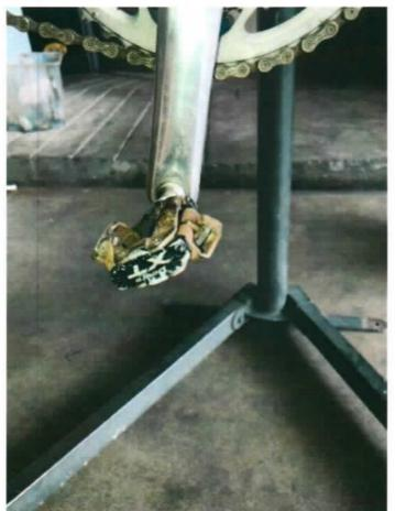
a. The pedal mounting and dismounting is no longer functioning as well as before. This could be due to the sudden impact causing urgent dismount or involuntarily dismount during the impact. Replacement is recommended.
