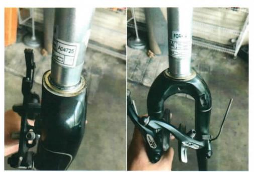
c. Stem has been taken out to inspect handlebar's bore area and the fork's steerer.
