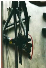
a. The hanger is slightly bent and requires servicing. Shifting is not functioning precisely and the derailleur cage is very closed to the wheel's spokes at the lowest gearing.
