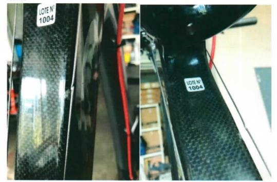
a. Frame's down tube has a dent along at the part where the cable was damaged. The cable damaged is highly caused by external impact against an object with shape angle where the impact penetrates thru and caused the dent on the carbon frame.
