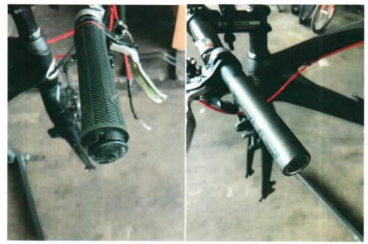
Right handlebar grip's Lock-on hardware is missing. This is possibly knocked off due to the impact against the floor. Replacement recommended.
