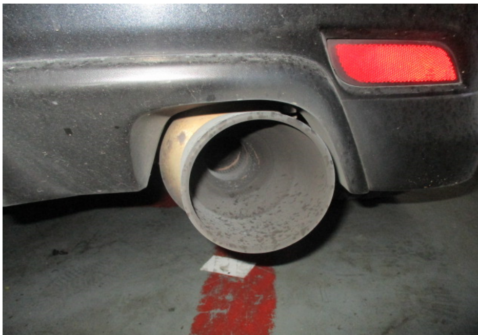
Photo 13 shows a front view of the non-standard rear exhaust muffler that was found to be fitted on the Insured Vehicle at the time of our inspection.
