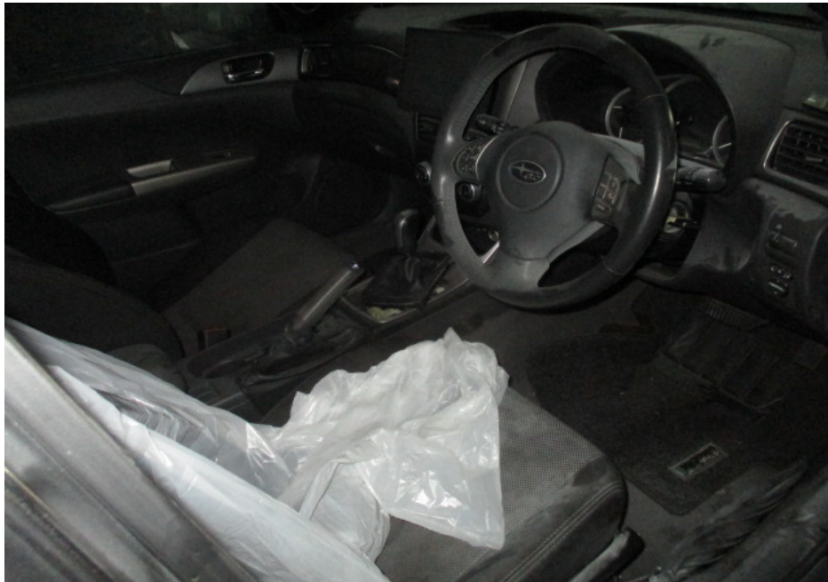
Photo 5 shows the interior compartment of the Insured Vehicle at the time of our inspection. The interior compartment of the Insured Vehicle was relatively unaffected by the fire.
