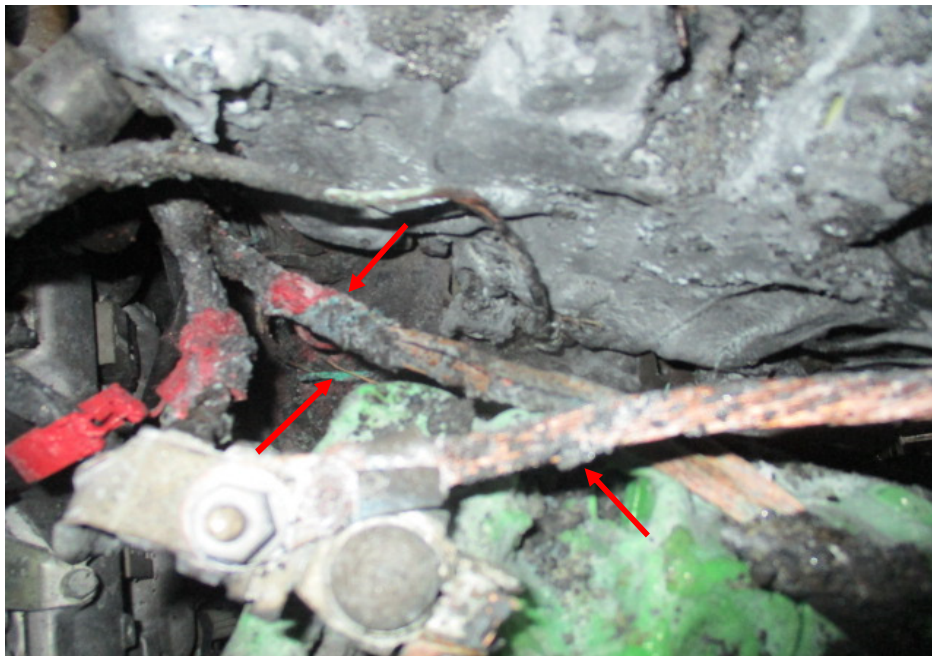
Photo 23 shows a close up view of the greenish residue on the wirings leading from the battery of the Insured Vehicle (red arrows). The presence of such greenish residue suggests occurrence of an electrical short circuit.
