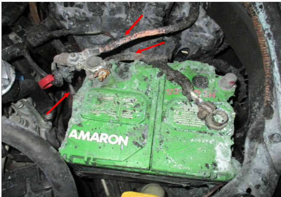
Photo 21 shows a closer view the greenish residue on the wirings at the left portion of the engine compartment (red arrows). The presence of such greenish residue suggests occurrence of an electrical short circuit.
