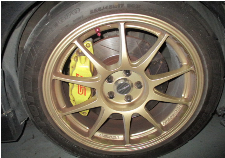
Photo 12 shows the non-standard rim found to be fitted on the Insured Vehicle at the time of our inspection. The 17- inch alloy rims fitted on the Insured Vehicle were not the standard type for the Insured Vehicle.
