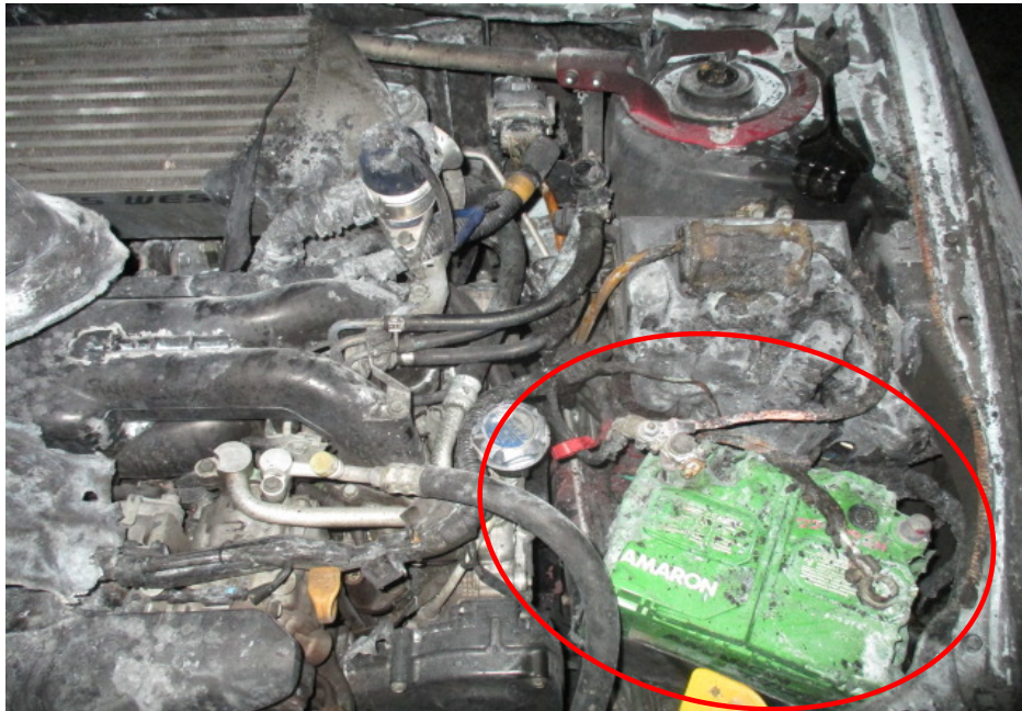
Photo 20 shows the wirings around the left portion of the engine compartment which is near to the vicinity where the fire to the Insured Vehicle had likely started. We observed greenish residue on the wirings leading from the battery of the Insured Vehicle (circled). The presence of greenish residue indicates internal heating of copper wires, a sign of an electrical short circuit occurring. The greenish residue is normally left behind from oxidation as a result of chemical reaction involving the copper wires.
