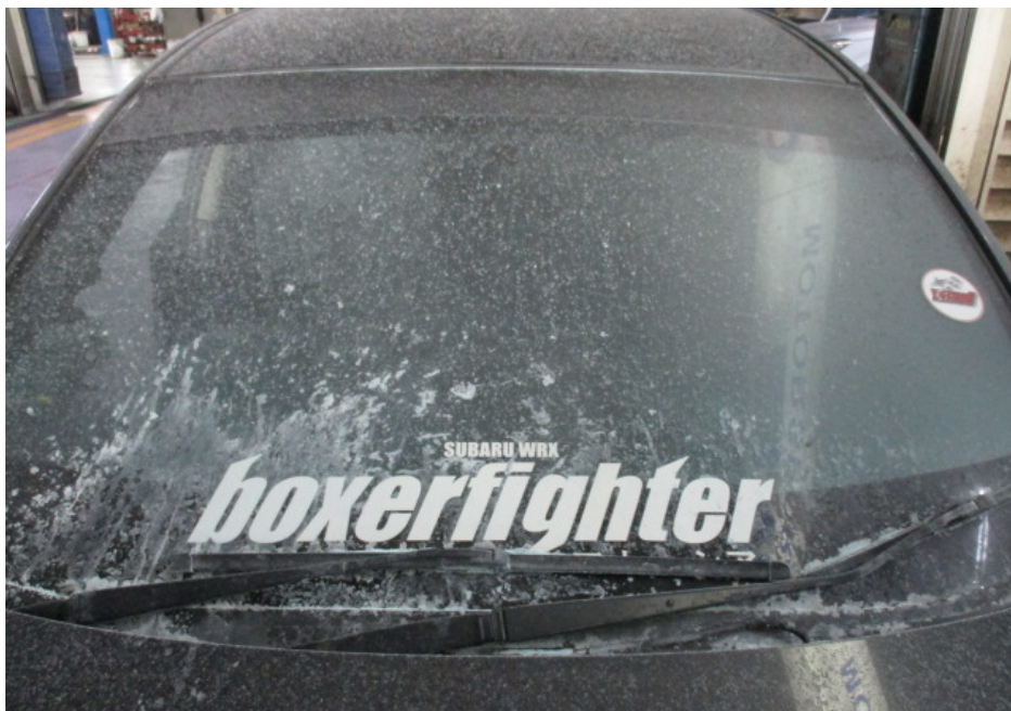
Photo 4 shows a closer view of the front windscreen of the Insured Vehicle at the time of our inspection. The front windscreen had sustained minimal fire damage.
