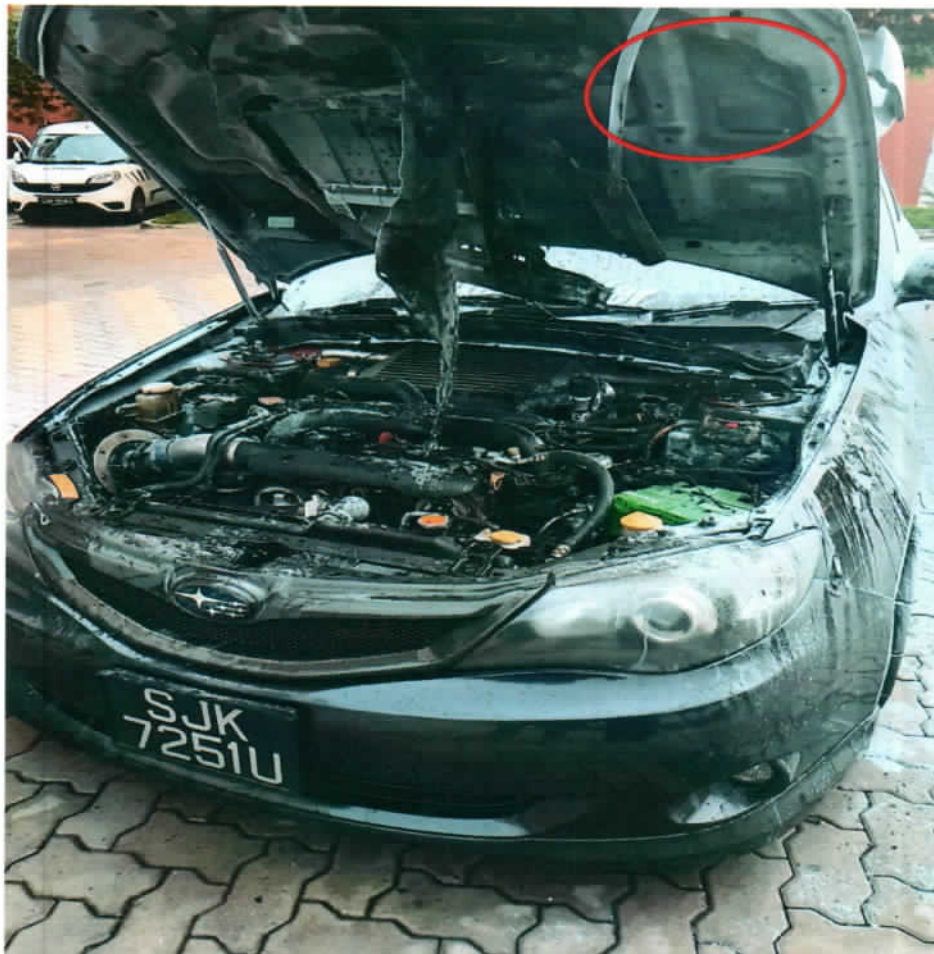
Photo 26 shows the Insured Vehicle at the incident location after the fire was extinguished. In general, the information that could be gathered from this photograph had corresponded to the events that were related to us by Mr Kwek. Whitish burn marks were observed on the underside of the front bonnet, at the left portion (circled) which indicates that the fire had started in the left portion of the engine compartment.
