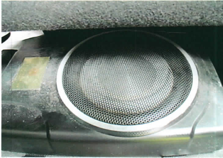
Photo 16 shows the aftermarket subwoofer that was found to be additionally fitted onto the Insured Vehicle upon our inspection.
