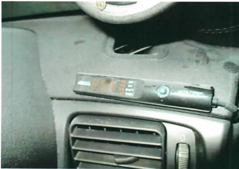
Photo 7 shows the auto timer that was found to be additionally fitted onto the Insured Vehicle upon our inspection.
