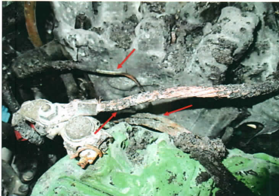
Photo 22 shows a close up view of the greenish residue on the wirings leading from the battery of the Insured Vehicle (red arrows). The presence of such greenish residue suggests occurrence of an electrical short circuit.
