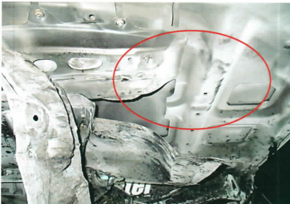
Photo 18 shows the whitish burn marks that were found on the left portion of the underside of the front bonnet of the Insured Vehicle (circled). Such whitish burn marks are a result of exposure to prolonged heat intensity, which may indicate where the fire had started. Hence the fire to the Insured Vehicle can be determined to have originated towards the left portion of the engine compartment.
