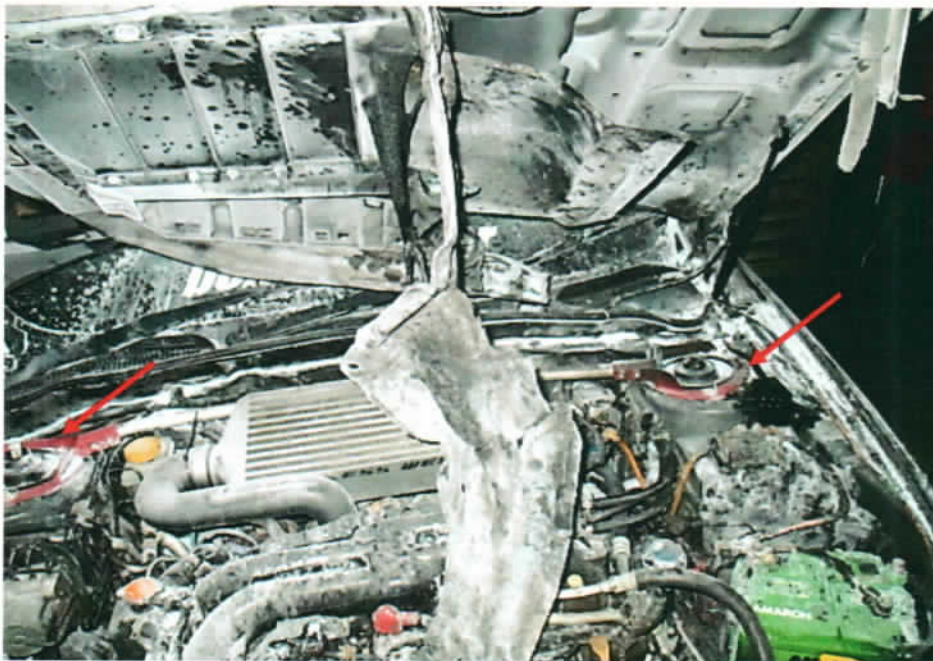
Photo 11 shows the engine strut bar (arrowed) fitted on the Insured Vehicle. However it had sustained minor fire damage.
