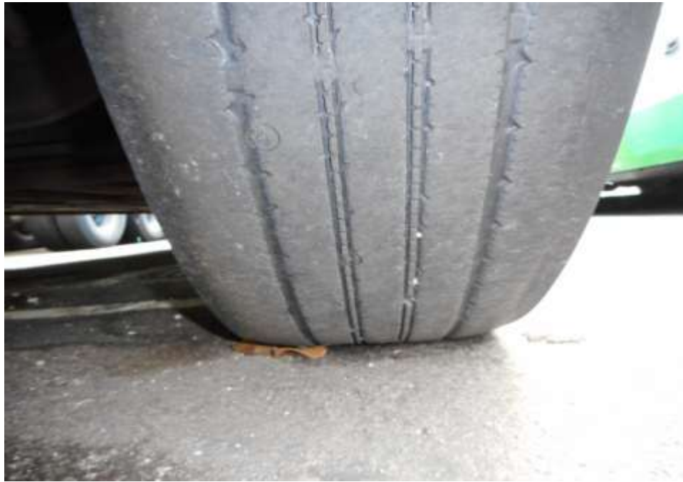
Photo 10 shows the condition of the front left tyres of the Motor Bus, which were observed to be in serviceable condition with remaining tread depth of approximately 2.7mm. There was also no tear, cut or burst mark(s) on the outer and the inner sidewalls as well as across the tread of the 6 tyres that were fitted on the Motor Bus.
