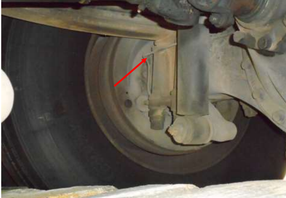
Photo 16 shows the brake pipe (arrowed) at the rear left wheel of the Motor Bus. I did not observe any leakage of brake fluid at the time of my inspection of the Motor Bus. My static tests of the Motor Bus's braking system, along with my visual examination of the various mechanical components in the braking system, had indicated that there was no internal leakage of pressure/vacuum. Hence the braking system of the Motor Bus was likely to be in serviceable condition at the material time of accident.
