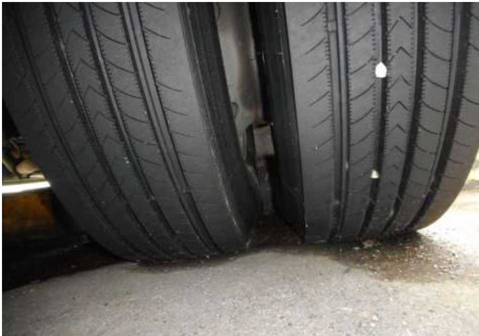
Photo 9 shows the condition of the rear left tyres of the Motor Bus, which was observed to be in serviceable condition with remaining tread depth of approximately 13.3mm. The tyres, which were wrapped around standard steel wheel rim, were also observed to be sufficiently inflated for vehicular operation. There was also no damage found on all 6 steel wheel rims of the Motor Bus.
