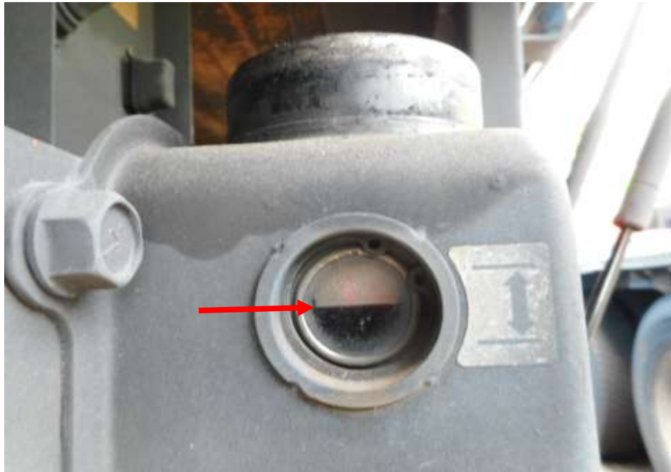
Photo 13 shows the power steering fluid reservoir of the Motor Bus at the time of my inspection. The power steering fluid was observed to be of sufficient level (arrowed) and without any visible contamination.
