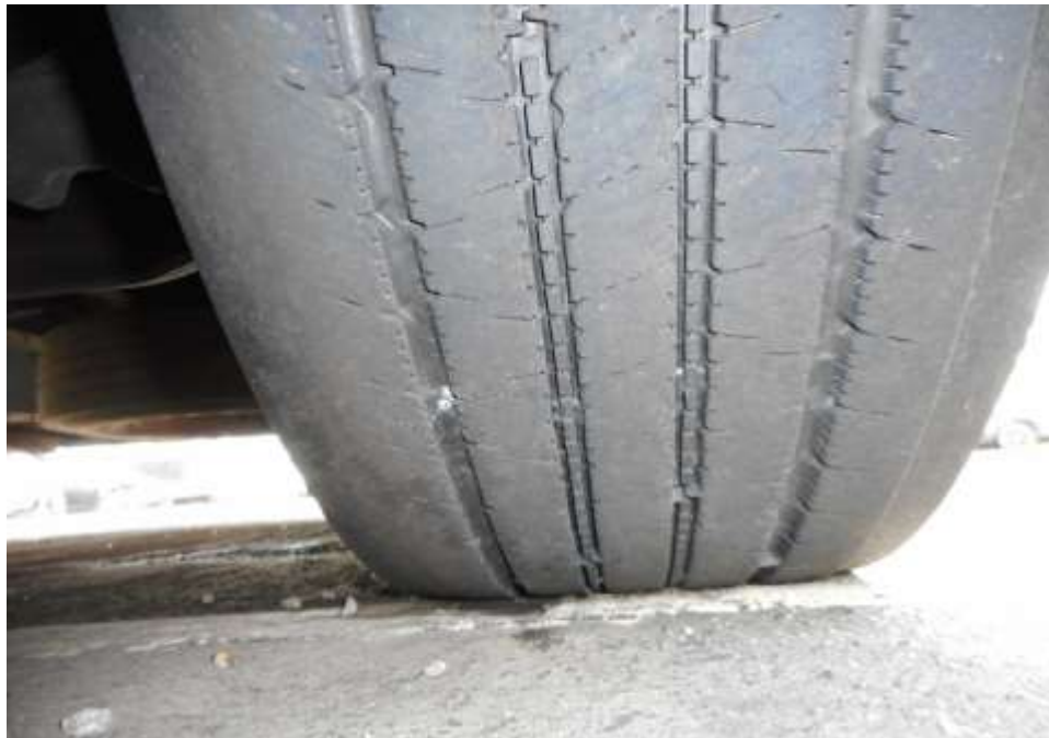
Photo 7 shows the condition of the front right tyre of the Motor Bus, which was observed to be in serviceable condition with remaining tread depth of approximately 6.1mm. The tyre, which was wrapped around standard steel wheel rim, was also observed to be sufficiently inflated for vehicular operation. There was no tear, cut or burst mark(s) on the outer and the inner sidewalls as well as across the tread of the 6 tyres that were fitted on the Motor Bus.
