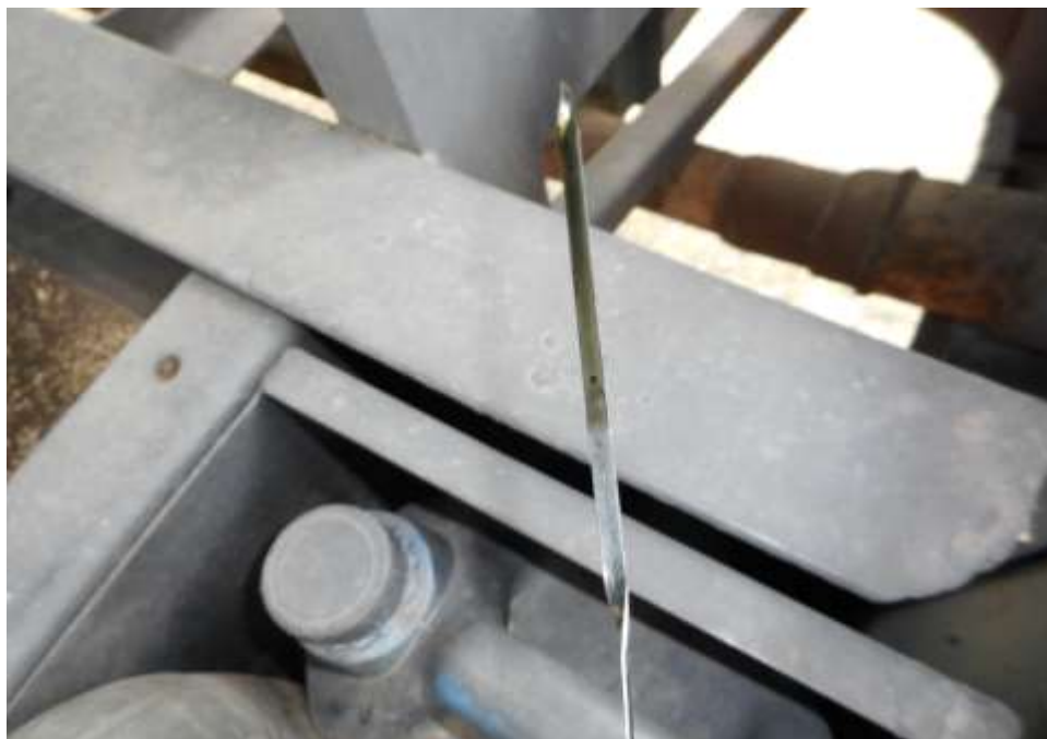
Photo 14 shows the engine oil dip stick of the Motor Bus at the time of my inspection. The engine oil was observed to be sufficient level for operation and without any visible contamination.
