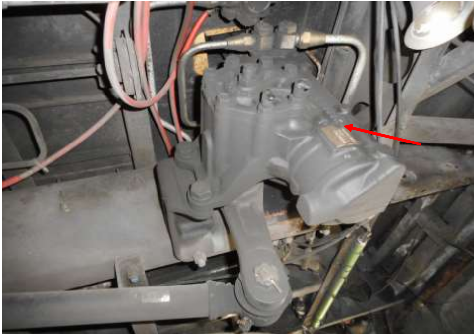
Photo 22 shows the steering box component (arrowed) at the undercarriage of the Motor Bus was found to be intact without any visible damage. There was also no sign of fluid stain(s) observed on the various undercarriage components.
