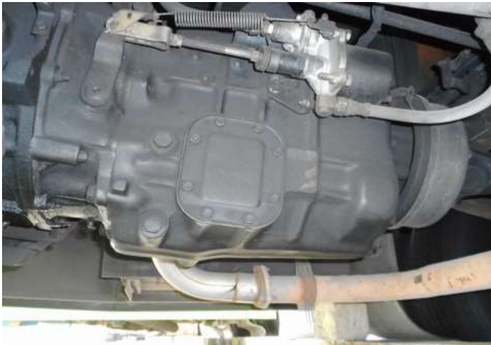
Photo 23 shows the undercarriage of the Motor Bus, at the area where the engine housing located. We observed minor fresh fluid stains on the surface of the engine oil sump. However the Motor Bus is still in serviceable condition.
