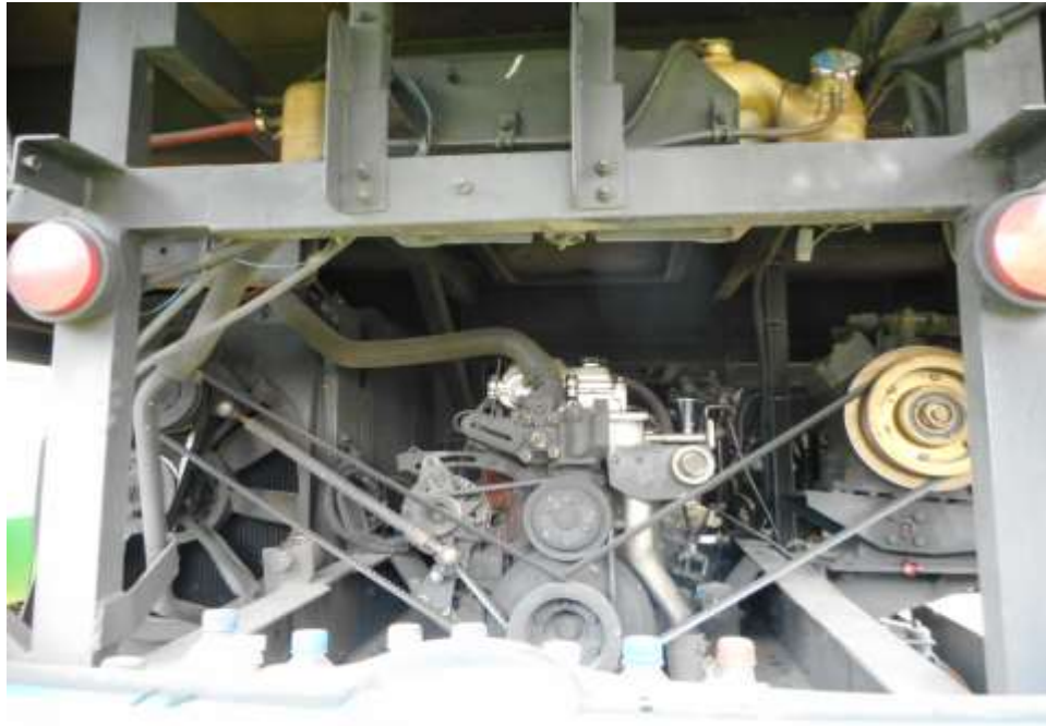
Photo 11 shows a general view of the Motor Bus's engine compartment, which was accessed by lifting the rear cabin of the Motor Bus. The various parts and components inside the engine compartment were unaffected by the accident. There was also no sign(s) or indication(s) of fresh fluid leakage and/or fluid stain within the engine compartment
