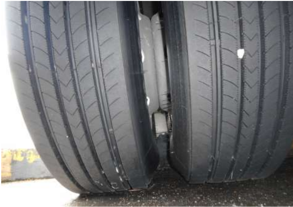
Photo 8 shows the condition of the rear right tyre of the Motor Bus, which was observed to be in serviceable condition with remaining tread depth of approximately 13.3mm. The tyre, which was wrapped around standard steel wheel rim, was also observed to be sufficiently inflated for vehicular operation.
