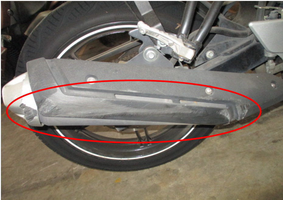
Photo 13 shows a closer view of the exhaust muffler and exhaust muffler heat shield which was amongst the body parts of the Motorcycle that had sustained damages of grazing nature as a result of the accident (circled).
