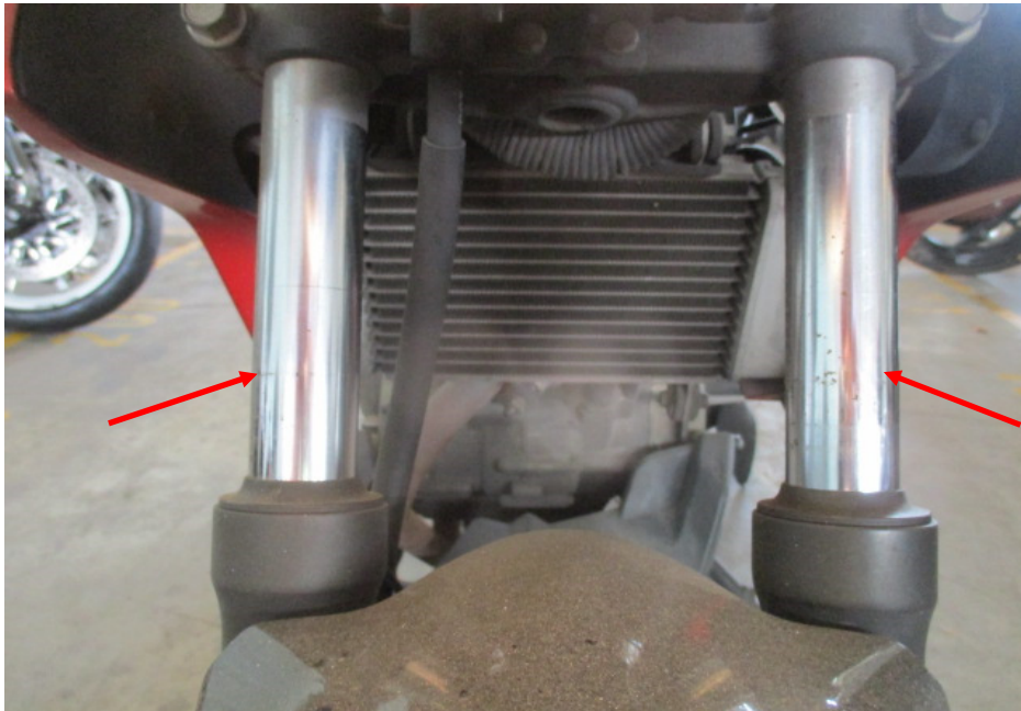
Photo 21 shows the front fork (arrowed) of the Motorcycle. The front fork and fork bracket of the Motorcycle were both found to be intact and undamaged. Turning the Motorcycle's handle bar towards the left and right did not produce any abnormal free play. The steering system of the Motorcycle was in serviceable condition at the time of our inspection.
