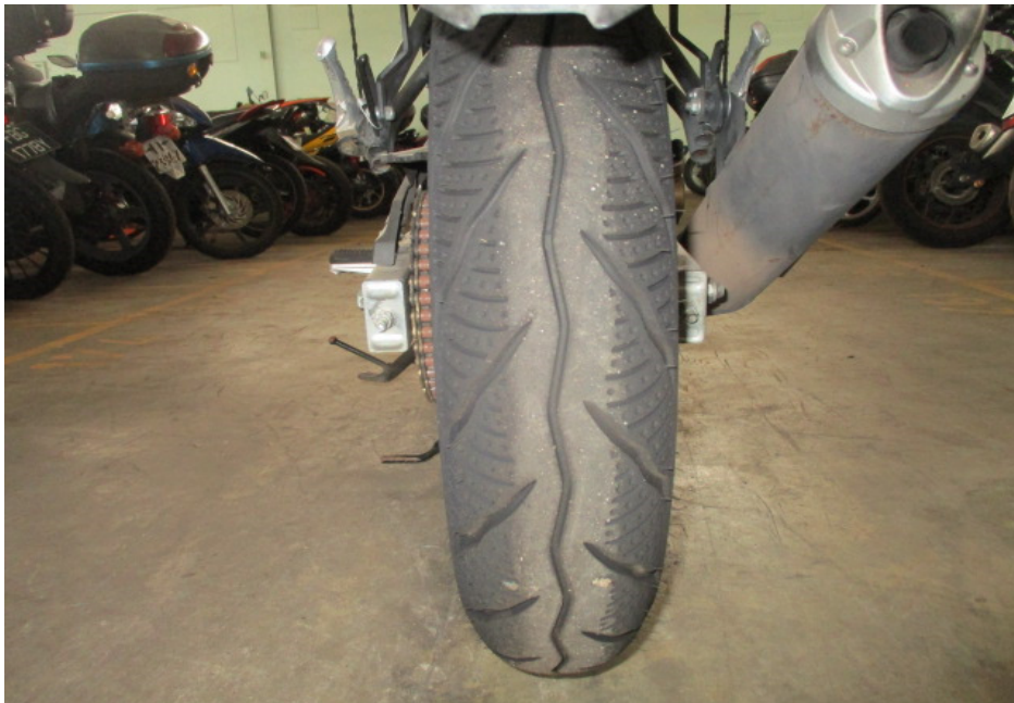
Photo 16 shows the condition of the Motorcycle's rear tyre. The rear tyre was observed to be in serviceable condition with remaining tread depth of approximately 4mm. The tyre was also observed to be sufficiently inflated for vehicular operation. We did not observe any tear, burst mark(s) and/or punctured hole(s) on the sidewalls as well as across the tread of the rear tyre.
