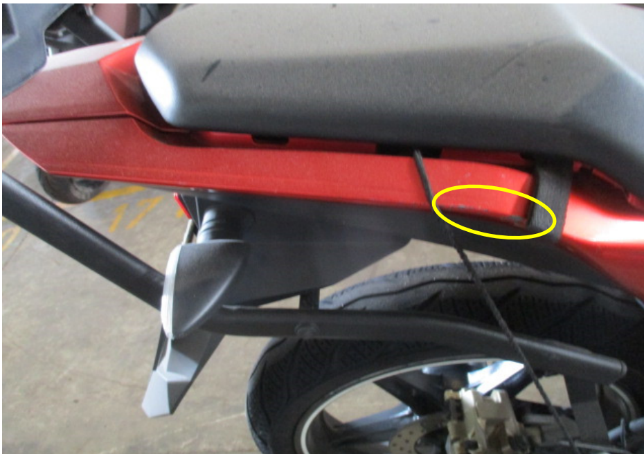
Photo 12 shows the damaged right rear side cover of the Motorcycle as a result of the accident (circled).
