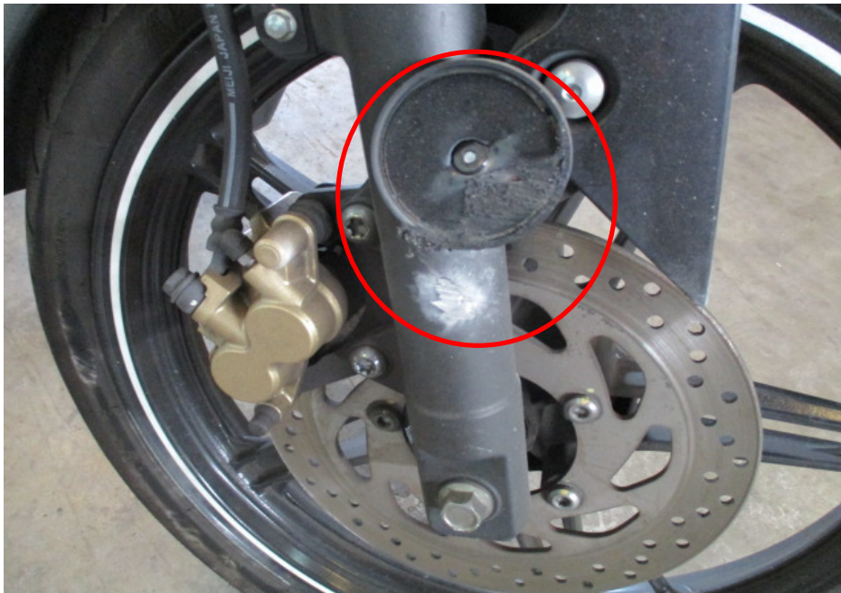
Photo 8 shows a closer view of the right outer fork tube and right reflector cover (circled) which were amongst the body parts of the Motorcycle that had sustained damages of grazing nature as a result of the accident.
