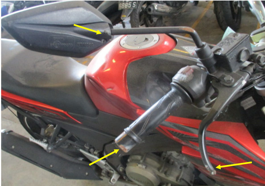
Photo 9 shows the front brake lever, right handlebar end and right side mirror (arrowed), which were amongst the body parts of the Motorcycle that had sustained damage as a result of the accident.
