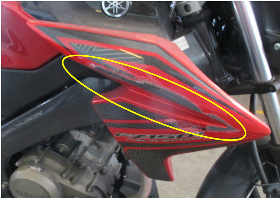
Photo 6 shows a close up view of the right side cowling (circled) which was amongst the body parts of the Motorcycle that had sustained damage as a result of the accident.
