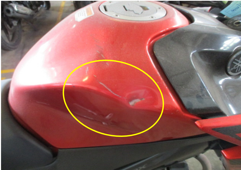
Photo 11 shows a closer view of the petrol tank (circled) which was amongst the body parts of the Motorcycle that had sustained damage as a result of the accident.
