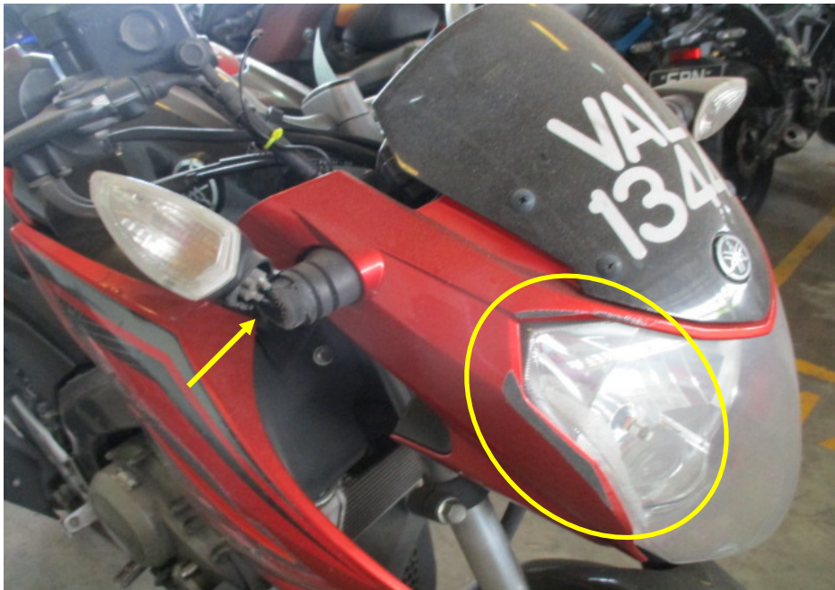
Photo 5 shows a closer view of the headlamp assembly (circled) and right front signal lamp (arrowed) which were amongst the body parts at the front body of the Motorcycle that had sustained damage as a result of the accident.
