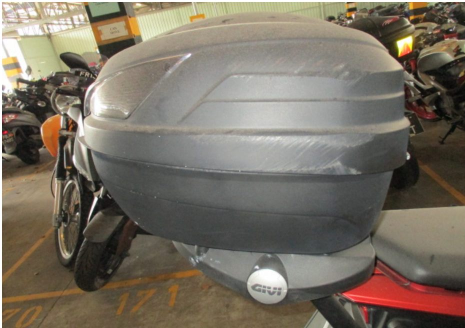
Photo 14 shows a closer view of the top box rack and top box which were amongst the body parts of the Motorcycle that had sustained damages of grazing nature as a result of the accident.
