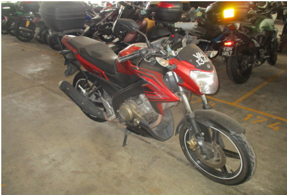
Photo 4 shows a general view of the right body of the Motorcycle at the time of our inspection. The Motorcycle was observed to have sustained damages along its frontal portion and right body. Amongst the body parts that were found to have been damaged include its headlamp assembly, right cowling, right front signal lamp, front mudguard, right outer fork tube, front brake lever, right side mirror, petrol tank, rear brake pedal, right front footrest, right rear side cover, exhaust muffler heat shield and top box, amongst others.
