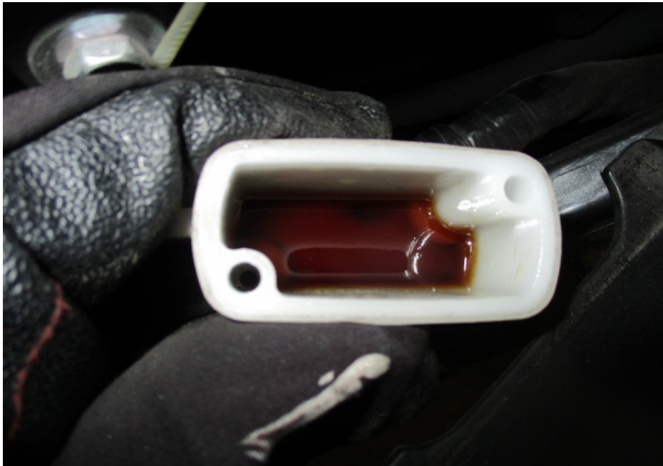
Photo 27 shows the brake fluid reservoir for the rear brake of the Motorcycle. The brake fluid was observed to be of sufficient level and without contamination for operational purposes.
