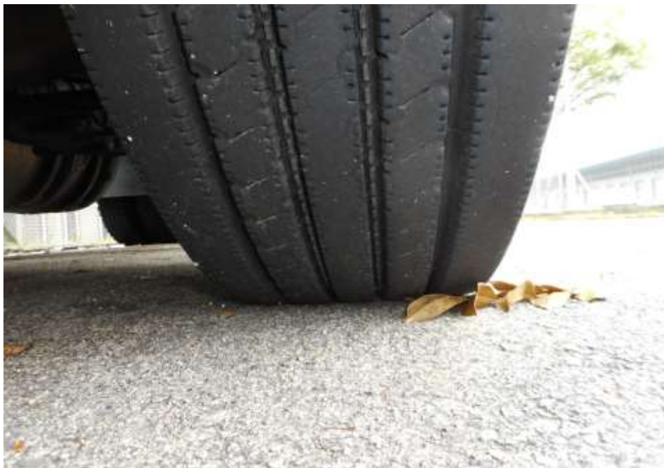
Photo 12 shows the condition of the front left tyres of the Motor Trailer, which were observed to be in serviceable condition with remaining tread depth of approximately 12.4mm. There was also no tear, cut or burst mark(s) on the outer and the inner sidewalls as well as across the tread of the 10 tyres that were fitted on the Motor Trailer.
