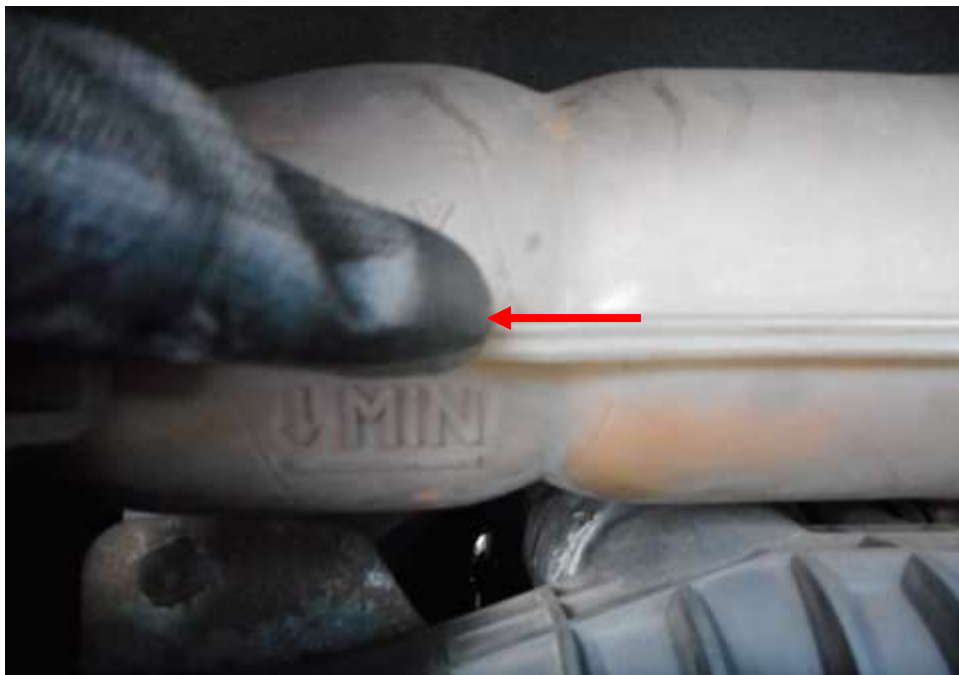
Photo 17 shows the engine coolant reservoir of the Motor Trailer at the time of my inspection. The engine coolant was observed to be of sufficient level (arrowed) and without any visible contamination.
