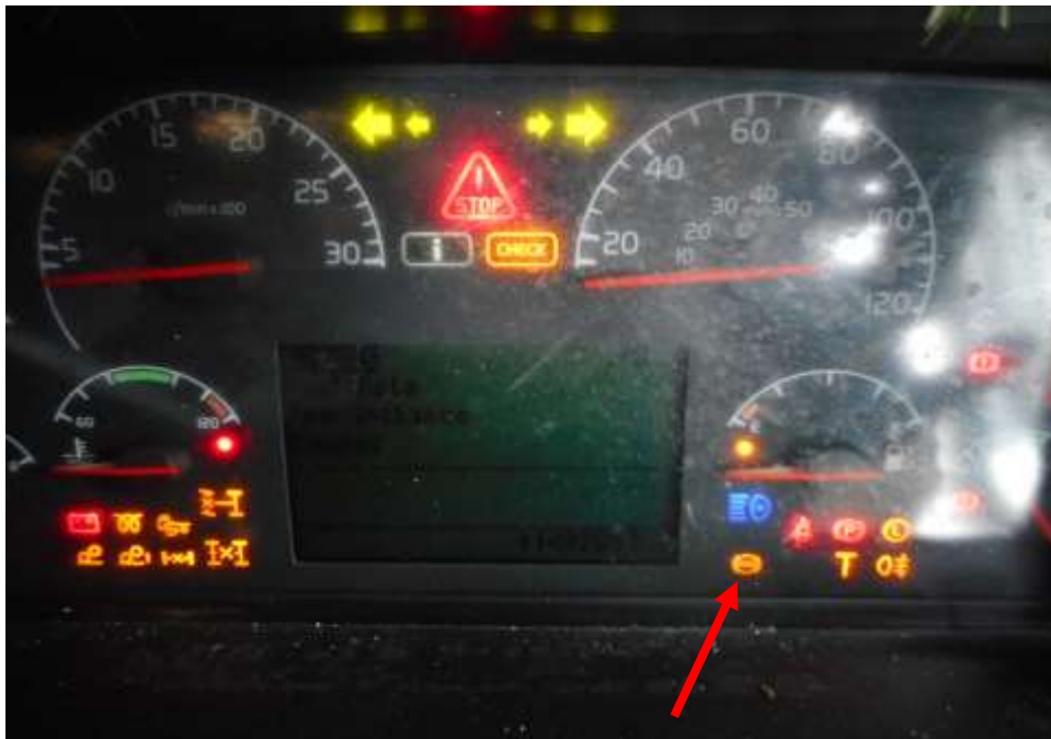
Photo 29 shows the warning light for Anti-Lock Brake System (ABS) (arrowed) appearing on the instrument panel of the Motor Trailer during the self-test of its various electronic operating systems when its engine was cranked.
