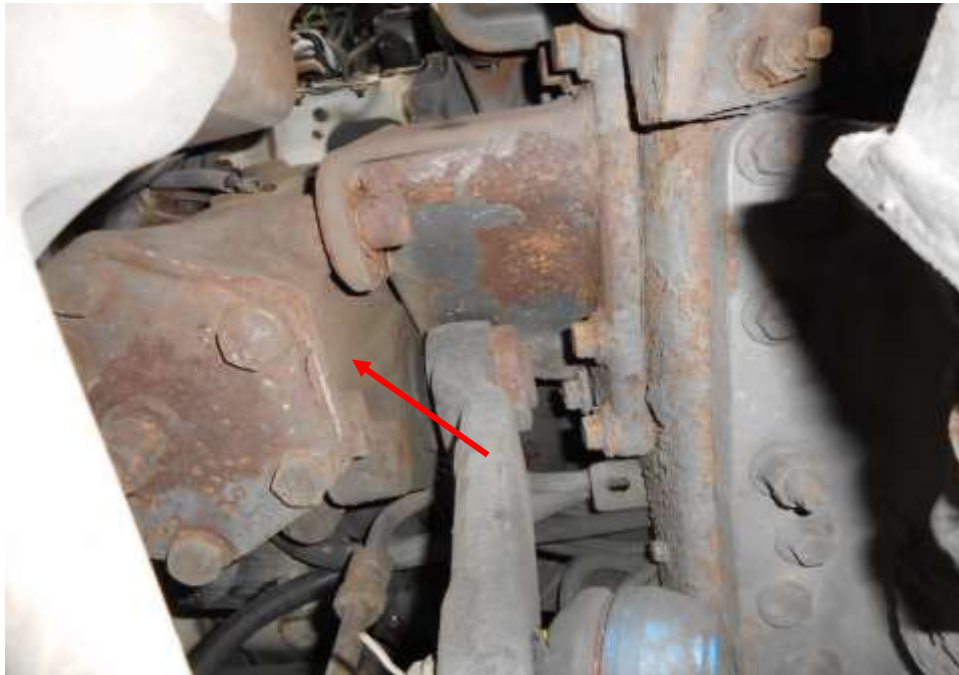
Photo 27 shows the steering box component (arrowed) at the undercarriage of the Motor Trailer was found to be intact without any visible damage. There was also no sign of fluid stain(s) observed on the various undercarriage components.
