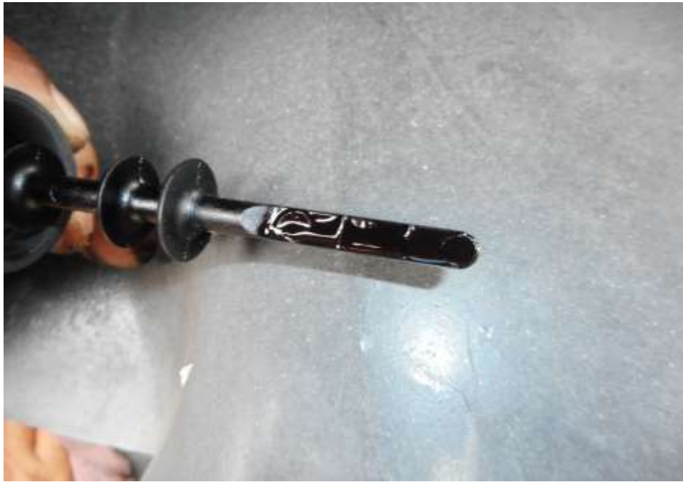
Photo 18 shows the power steering fluid reservoir of the Motor Trailer at the time of my inspection. The power steering fluid was observed to be of sufficient level and without any visible contamination.
