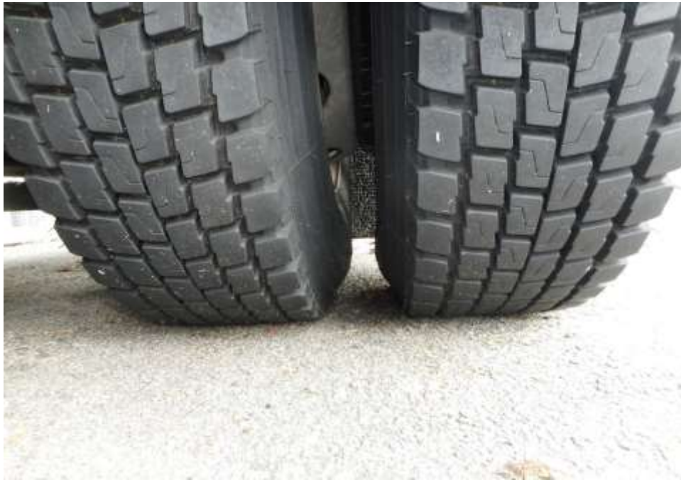
Photo 11 shows the condition of the rear left tyres of the Motor Trailer, which was observed to be in serviceable condition with remaining tread depth of approximately 12.8mm. The tyres, which were wrapped around standard steel wheel rim, were also observed to be sufficiently inflated for vehicular operation. There was also no damage found on all 10 steel wheel rims of the Motor Trailer.
