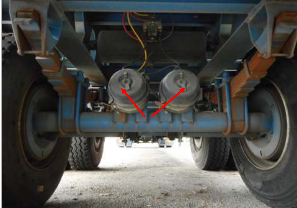
Photo 21 shows the brake pipe (arrowed) at the rear left and right wheel of the Motor Trailer. I did not observe any leakage of brake fluid at the time of my inspection of the Motor Trailer. My static tests of the Motor Trailer's braking system, along with my visual examination of the various mechanical components in the braking system, had indicated that there was no internal leakage of pressure/vacuum. Hence the braking system of the Motor Trailer was likely to be in serviceable condition at the material time of accident.
