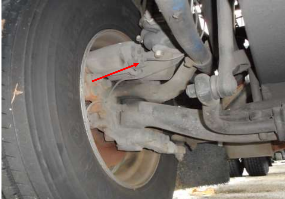
Photo 22 shows the brake pipe (arrowed) at the front right wheel of the Motor Trailer. I did not observe any leakage of brake fluid at the time of my inspection of the Motor Trailer. My static tests of the Motor Trailer's braking system, along with my visual examination of the various mechanical components in the braking system, had indicated that there was no internal leakage of pressure/vacuum. Hence the braking system of the Motor Trailer was likely to be in serviceable condition at the material time of accident.
