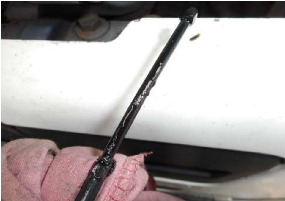
Photo 19 shows the engine oil dip stick of the Motor Trailer at the time of my inspection. The engine oil was observed to be of sufficient level and without any visible contamination.
