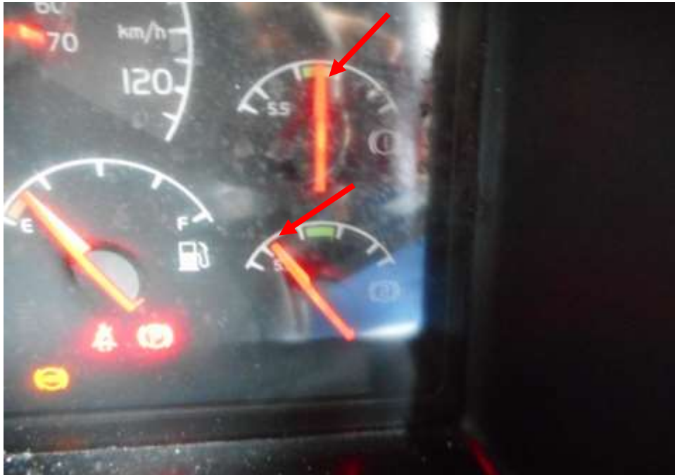
Photo 16 shows the air in the air brake cylinders of the Motor Trailer at the time of my inspection. The air in the cylinder was observed to be of sufficient level & serviceable at the time of the accident.
