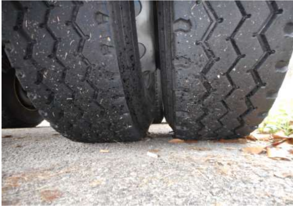
Photo 13 shows the condition of the right tyres of the trailer, which was observed to be in serviceable condition with remaining tread depth of approximately 12.1mm. The tyre, which was wrapped around standard steel wheel rim, was also observed to be sufficiently inflated for vehicular operation.
