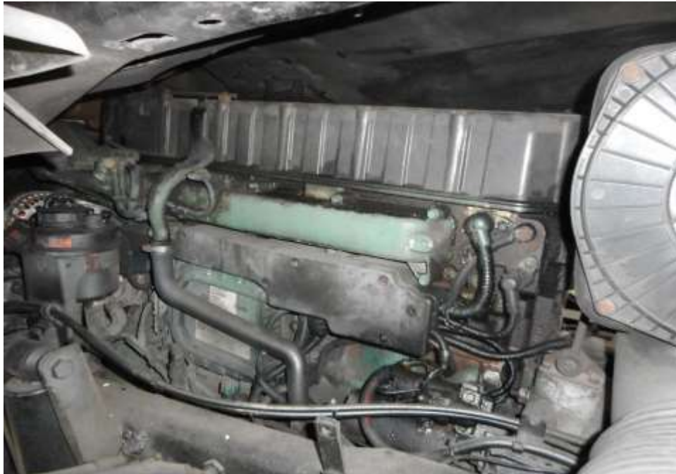
Photo 15 shows a general view of the Motor Trailer's engine compartment, which was accessed by lifting the front cabin of the Motor Trailer. The various parts and components inside the engine compartment were unaffected by the accident. There was also no sign(s) or indication(s) of fresh fluid leakage and/or fluid stain within the engine compartment
