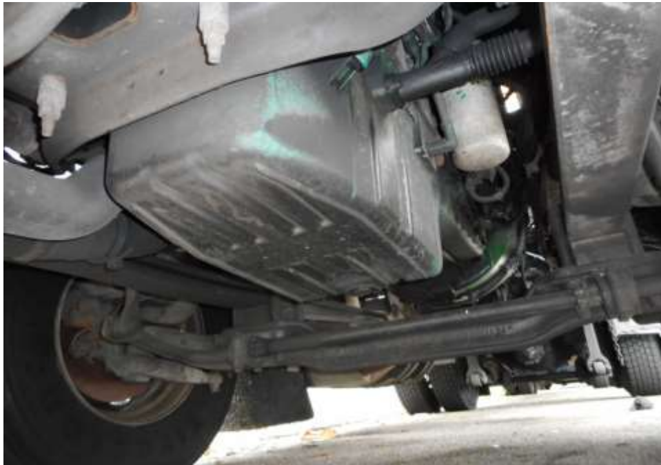
Photo 20 shows the undercarriage of the Motor Trailer, at the area where the engine housing located. I did not find any sign(s) or indication(s) of fluid leak and/or fluid stain(s) on the underside of the Motor Trailer.
