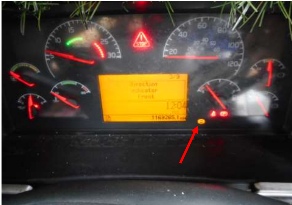
Photo 30 shows the ABS warning lights illuminated on the instrument panel of the Motor Trailer after the engine was cranked. This would suggest that there was an electrical fault to the ABS systems of the Motor Trailer.
