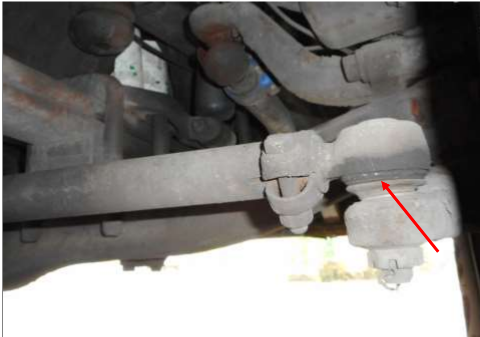
Photo 25 shows the various undercarriage components at the front right wheel of the Motor Trailer, in particular the steering tie rod end (arrowed). The various steering components were all found to be intact, suggesting that the steering system of the Motor Trailer was likely to be in serviceable condition at the material time of accident. There was also no sign of fluid stain(s) observed on the various undercarriage components.
