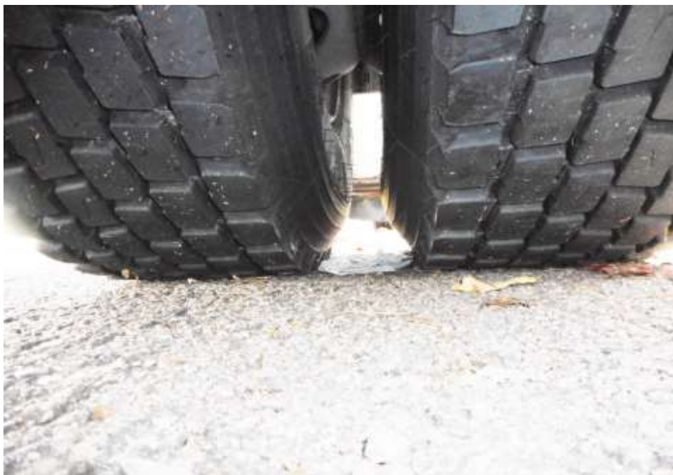
Photo 10 shows the condition of the rear right tyre of the Motor Trailer, which was observed to be in serviceable condition with remaining tread depth of approximately 11mm. The tyre, which was wrapped around standard steel wheel rim, was also observed to be sufficiently inflated for vehicular operation.
