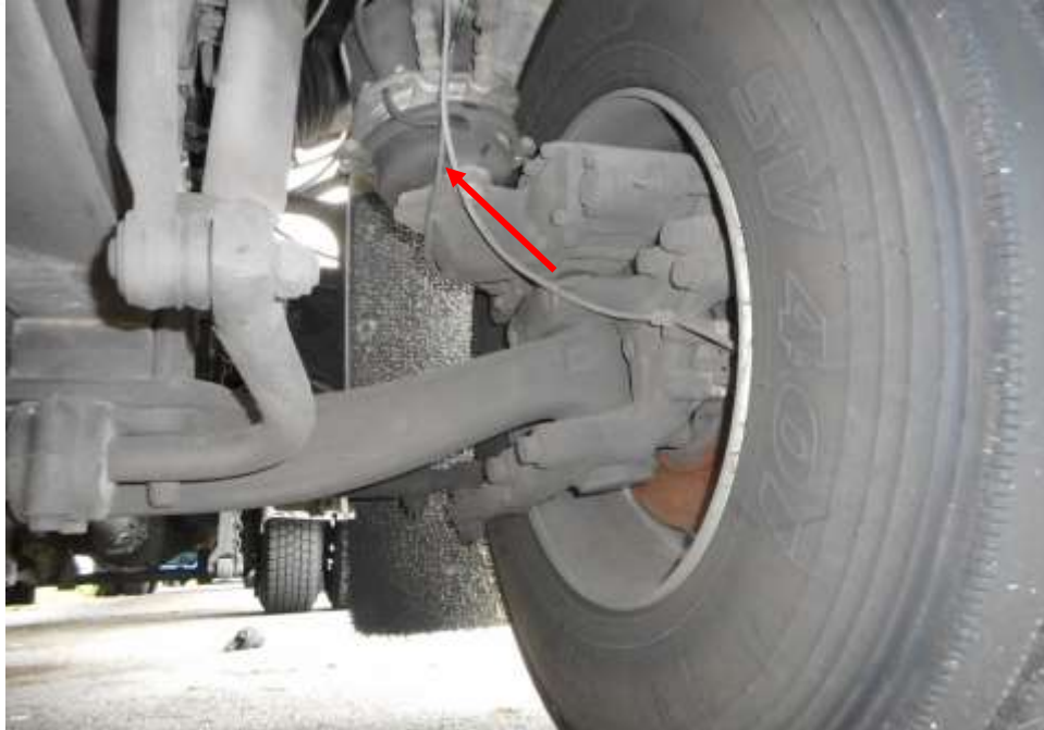
Photo 23 shows the brake pipe (arrowed) at the front left wheel of the Motor Trailer. I did not observe any leakage of brake fluid at the time of my inspection of the Motor Trailer. My static tests of the Motor Trailer's braking system, along with my visual examination of the various mechanical components in the braking system had indicated that there was no internal leakage of pressure/vacuum. Hence the braking system of the Motor Trailer was likely to be in serviceable condition at the material time of accident.
