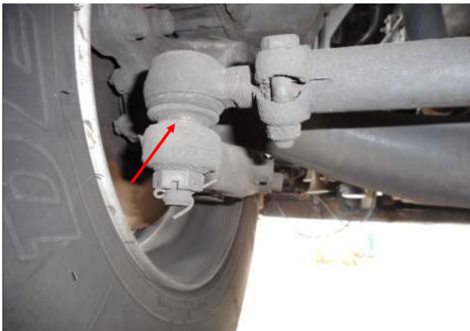
Photo 26 shows the various undercarriage components at the front left wheel of the Motor Trailer, in particular the steering tie rod end (arrowed). The various undercarriage components of the Motor Trailer were all found to be intact without any visible damage. There was also no sign of fluid stain(s) observed on the various undercarriage components.
