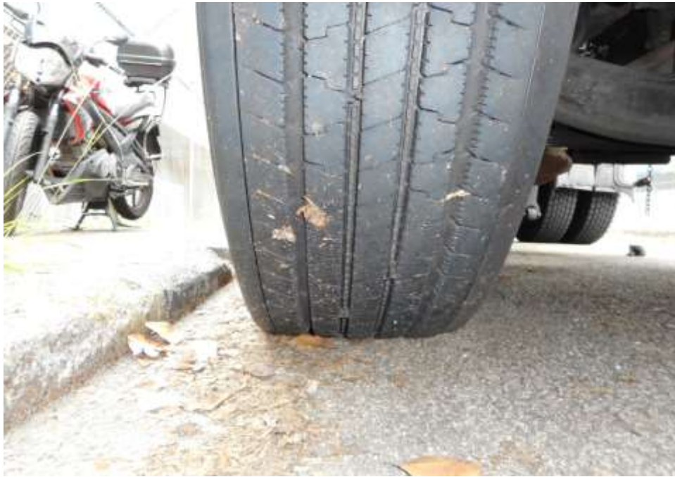
Photo 9 shows the condition of the front right tyre of the Motor Trailer, which was observed to be in serviceable condition with remaining tread depth of approximately 11.7 mm. The tyre, which was wrapped around standard steel wheel rim, was also observed to be sufficiently inflated for vehicular operation. There was no tear, cut or burst mark(s) on the outer and the inner sidewalls as well as across the tread of the 10 tyres that were fitted on the Motor Trailer.
