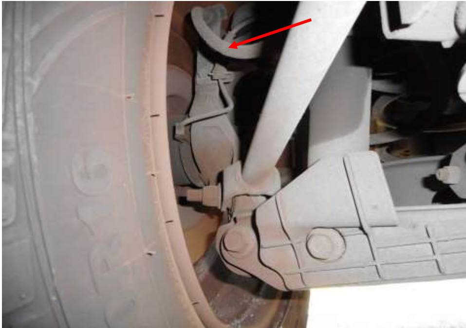
Photo 16 shows the brake hose/pipe (arrowed) at the rear left wheel of the Motor Taxi. I did not observe any leakage of brake fluid at the time of my inspection of the Motor Taxi. Static tests of the Motor Taxi's braking system had indicated that there was no internal leakage of pressure/vacuum. The undercarriage components of the Motor Taxi were also all found to be intact and without any visible damage.
