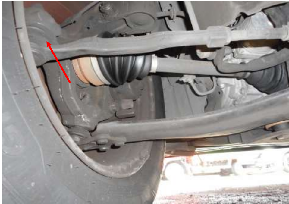
Photo 22 shows the various undercarriage components at the front left wheel of the Motor Taxi, which had included the steering tie rod (red arrow). The various undercarriage components of the Motor Taxi were all found to be intact without any visible damage.
