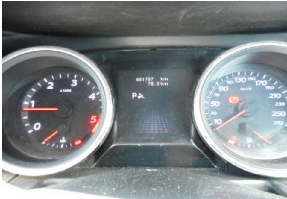
Photo 24 shows no warning lights illuminated on the instrument panel of the Motor Taxi after the engine was cranked. This would suggest that there was no abnormality to the various electronic operating systems of the Motor Taxi, like the ABS and SRS etc.
