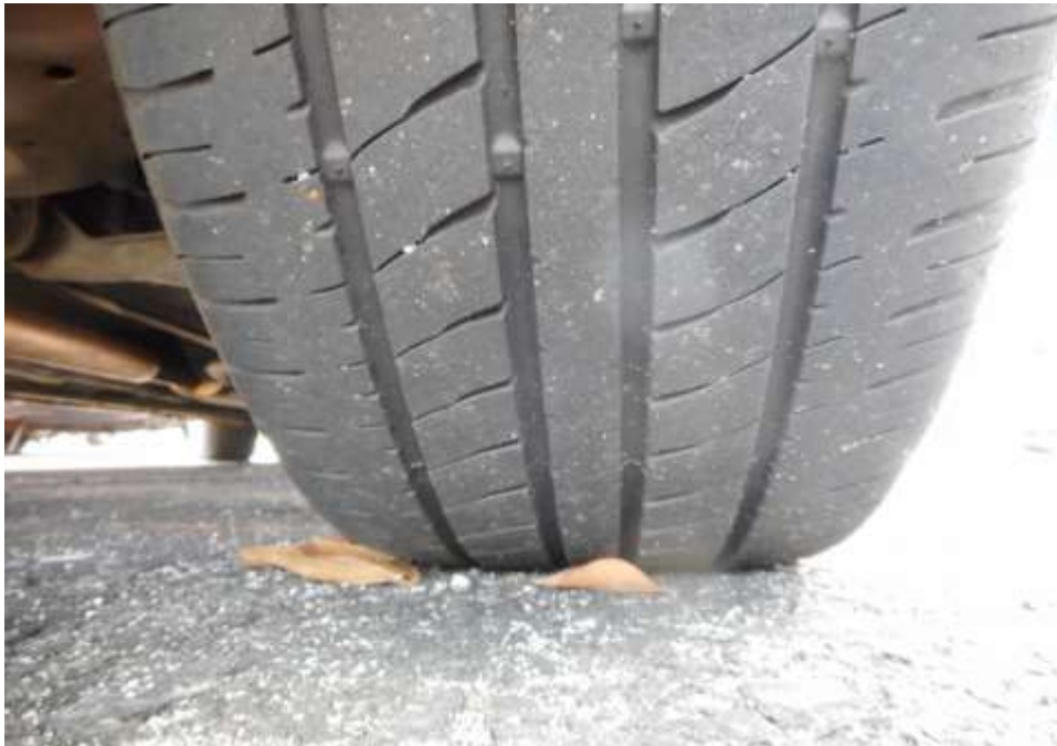
Photo 8 shows the condition of the rear right tyre of the Motor Taxi, which was observed to be in serviceable condition with remaining tread depth of approximately 4.8mm. The tyre was also observed to be sufficiently inflated for vehicular operation with no tear, cut or burst mark(s).
