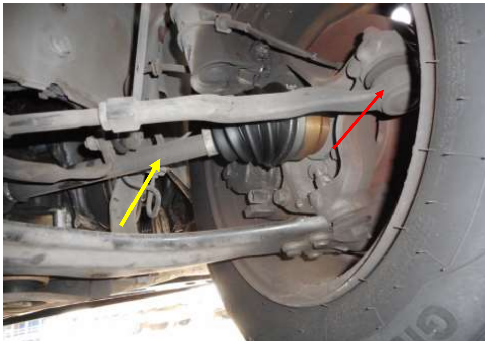
Photo 21 shows the various undercarriage components at the front right wheel of the Motor Taxi, in particular the steering tie rod (red arrow) and drive shaft (yellow arrow). The various steering components were all found to be intact, suggesting that the steering system of the Motor Taxi was likely to be in serviceable condition at the material time of accident. There was also no sign of fluid stain observed on the various undercarriage components at the front right wheel of the Motor Taxi.
