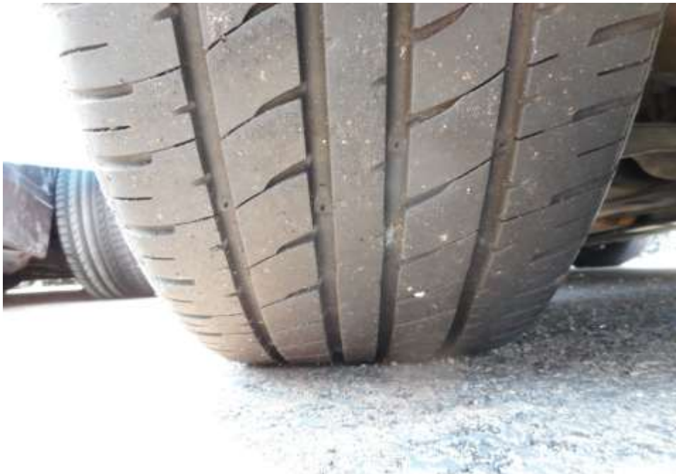
Photo 9 shows the condition of the rear left tyre of the Motor Taxi, which was observed to be in serviceable condition with remaining tread depth of approximately 6.1mm. The tyre, which was wrapped around steel wheel rim, was also observed to be sufficiently inflated for vehicular operation. The 4 tyres of the Motor Taxi were wrapped around standard steel wheel rims.
