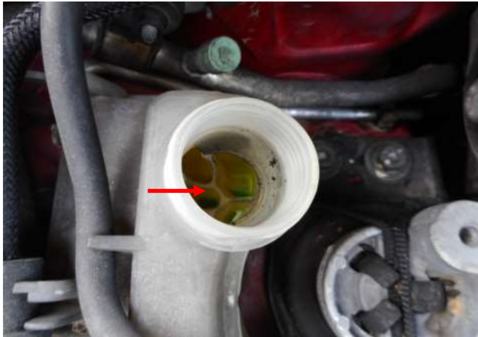
Photo 13 shows checks being carried out to the engine coolant of the Motor Taxi at the time of my inspection. The engine coolant was observed to be of sufficient level (arrowed) and without any visible contamination.
