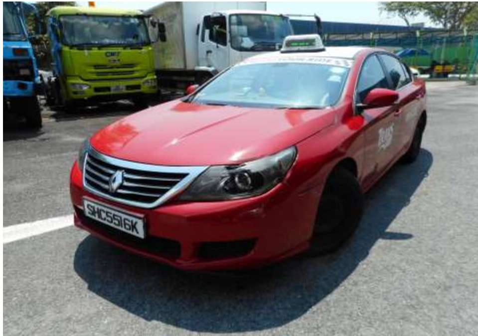
Photo 20 shows the front left wheel of the Motor Taxi turned to its full right. During my steering system test, I did not experience any abnormal free play and/or resistance when I had turned the steering wheel towards the left and right. This would suggest that the steering system of the Motor Taxi was likely to be in serviceable condition at the material time of accident.
