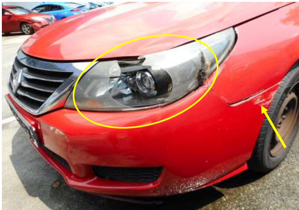
Photo 3 shows the close up view of the Motor Taxi's front body at the time of my inspection. The Motor Taxi was observed to have sustained damage at its front bumper (arrowed) and front left headlamp (circled) as a result of the accident.
