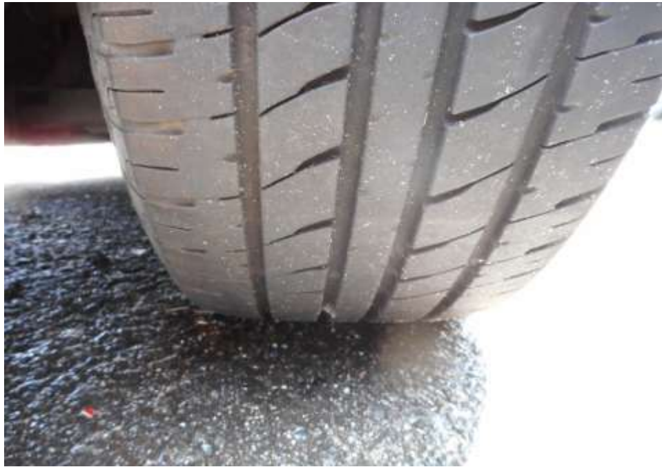
Photo 10 shows the condition of the front left tyre of the Motor Taxi, which was observed to be in serviceable condition with remaining tread depth of approximately 6mm. There was also no tear, cut or burst mark(s) on the outer and the inner sidewalls as well as across the tread of the Motor Taxi's 4 tyres.
