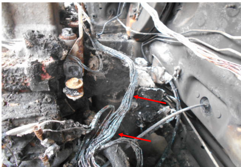
Photo 11 shows a closer view of the stretch of wirings with greenish residue (arrowed). The wirings were originally fitted wirings located at the rear of the Motor Car's engine compartment. The greenish residue indicates internal heating of copper wires, a sign of an electrical short circuit occurring. The greenish residue is normally left behind from oxidation as a result of chemical reaction involving the copper wires.
