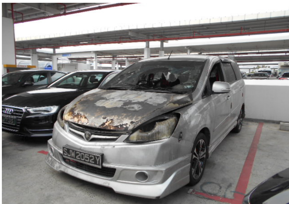
Photo 2 shows a general view of the front left body of the Motor Car at the time of my inspection. The fire damage to the Motor Car was observed to be confined to its frontal portion. Its front bumper, front bonnet, front left headlamp and front left fender were amongst the body parts that were found to have been affected as a result of the fire.
