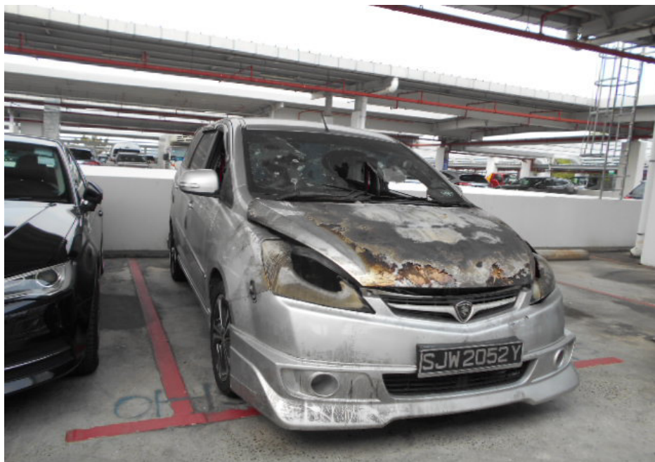
Photo 1 shows a general view of the front right body of the Motor Car at the time of my inspection. The fire damage to the Motor Car was confined to its frontal portion. Its engine compartment and interior compartment had sustained damage of burnt nature whilst its rear portion was unaffected. Its front bumper, front bonnet, front grille and front right headlamp were amongst the body parts that were found to have been affected as a result of the fire.
