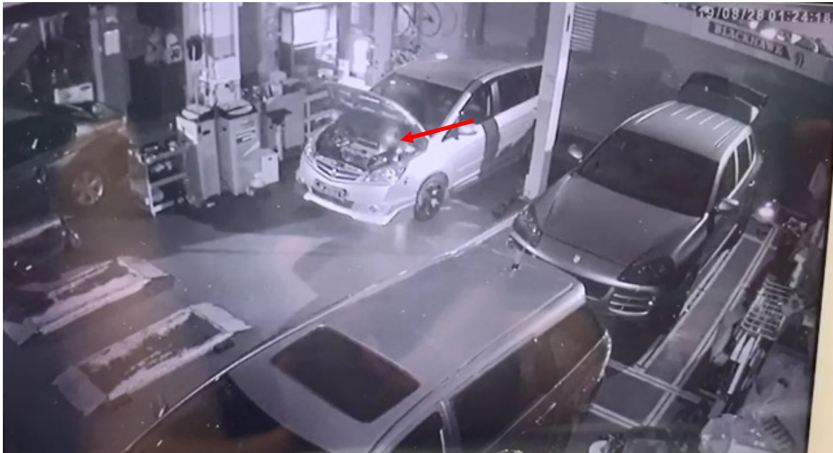
Photo 6 shows the premise of Hup Soon Batteries (screenshot from video footage retrieved from a CCTV camera inside the premise of Hup Soon Batteries). At about 0124hrs, a flame (arrowed) was first seen at the rear of the Motor Car's engine compartment, slightly towards the left from the rear centre. At this point in time, there was no one inside the premise. This would indicate that the flame at the rear of the Motor Car's engine compartment had self-ignite.
