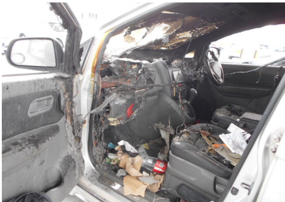
Photo 4 shows the interior compartment of the Motor Car, which was observed to be partially burnt and/or melted at the front area. The front windscreen, front dashboard, plastic trims and roof upholstery were amongst the parts that were found to have been burnt and/or melted as a result of the fire.
