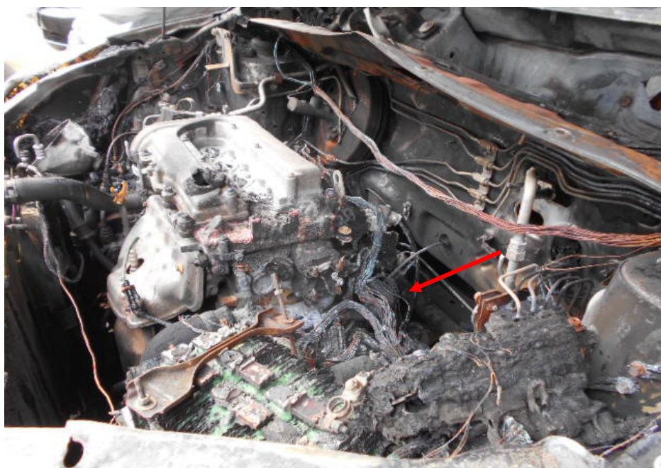
Photo 13 shows a general view of where the starter motor of the Motor Car is located. This was at the rear of the engine compartment (arrowed), in the vicinity of where the flame was first seen on the Motor Car.
