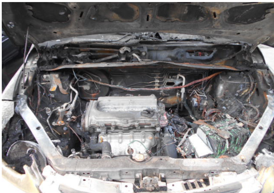
Photo 3 shows the engine compartment of the Motor Car at the time of my inspection. The engine compartment of the Motor Car was observed to have sustained moderate damage of burnt nature. The battery, fuse box, air intake, various piping and hoses were amongst the parts within the engine compartment that were burnt and/or melted as a result of the fire.
