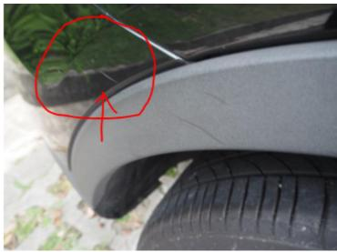
Rear bumper only 1 scratch line what repair need to be done? Only putty and spray paint. Re-inspection need if there is any dent.
