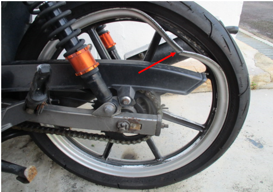
Photo 12 shows the broken rear wheel rim (arrowed) of the Motorcycle at the time of our inspection.
