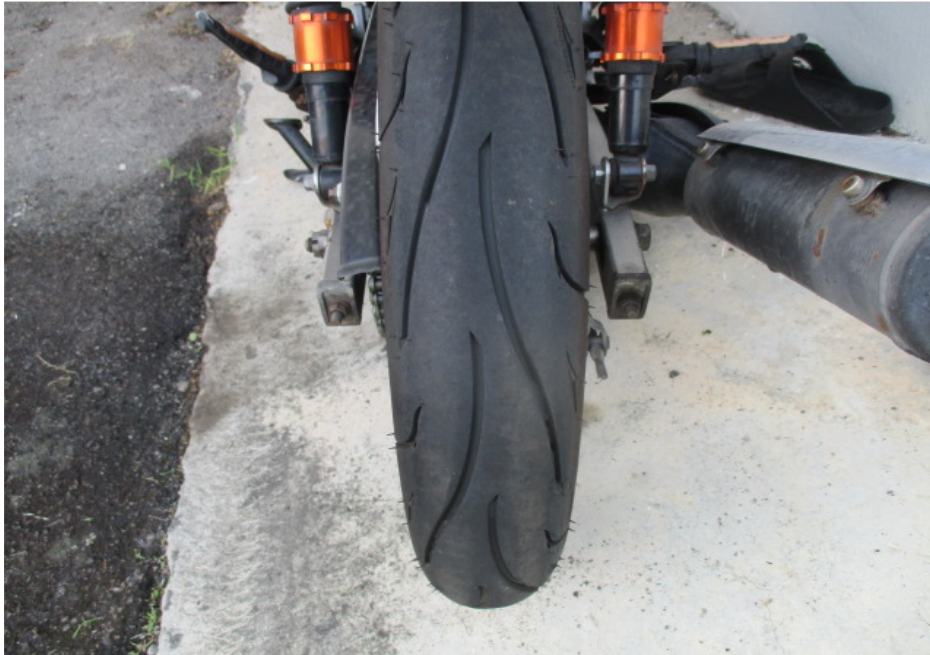
Photo 13 shows the condition of the Motorcycle's rear tyre. The rear tyre was observed to be in serviceable condition with remaining tread depth of approximately 4mm. However the rear tyre was observed to be deflated as a result of the broken rear wheel rim. We did not observe any tear, burst mark(s) and/or punctured hole(s) on the sidewalls as well as across the tread of the rear tyre.
