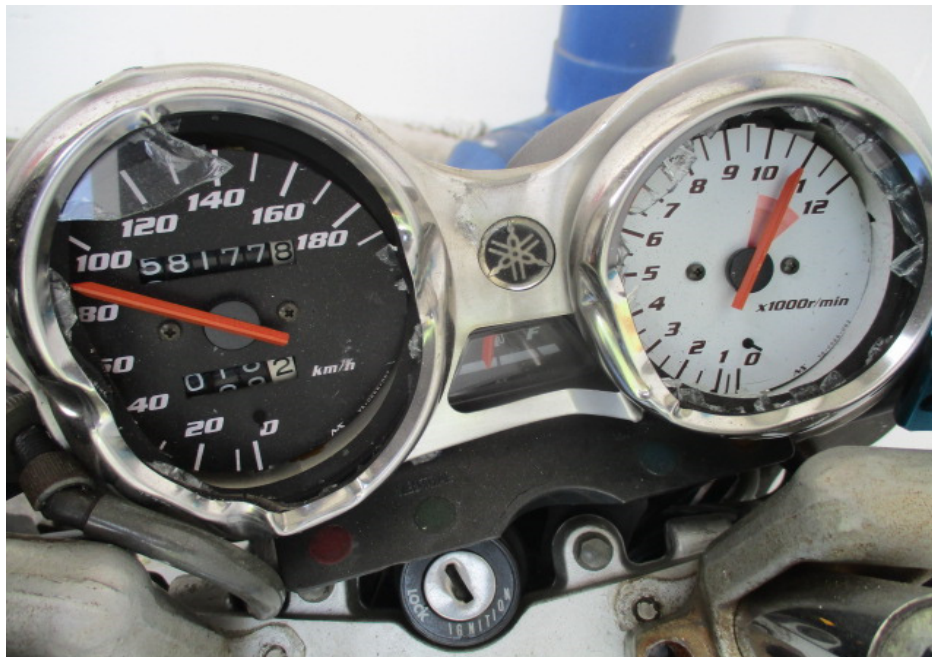
Photo 7 shows a close up view of the broken speedometer gauge of the Motorcycle as a result of the accident.
