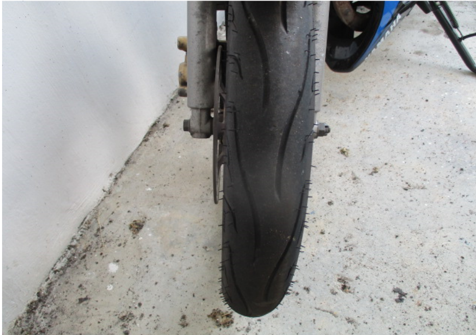
Photo 11 shows the condition of the Motorcycle's front tyre. The front tyre was observed to be in serviceable condition with remaining tread depth of approximately 3mm. The tyre was also observed to be sufficiently inflated for vehicular operation. We did not observe any tear, burst mark(s) and/or punctured hole(s) on the sidewalls as well as across the tread of the front tyre.
