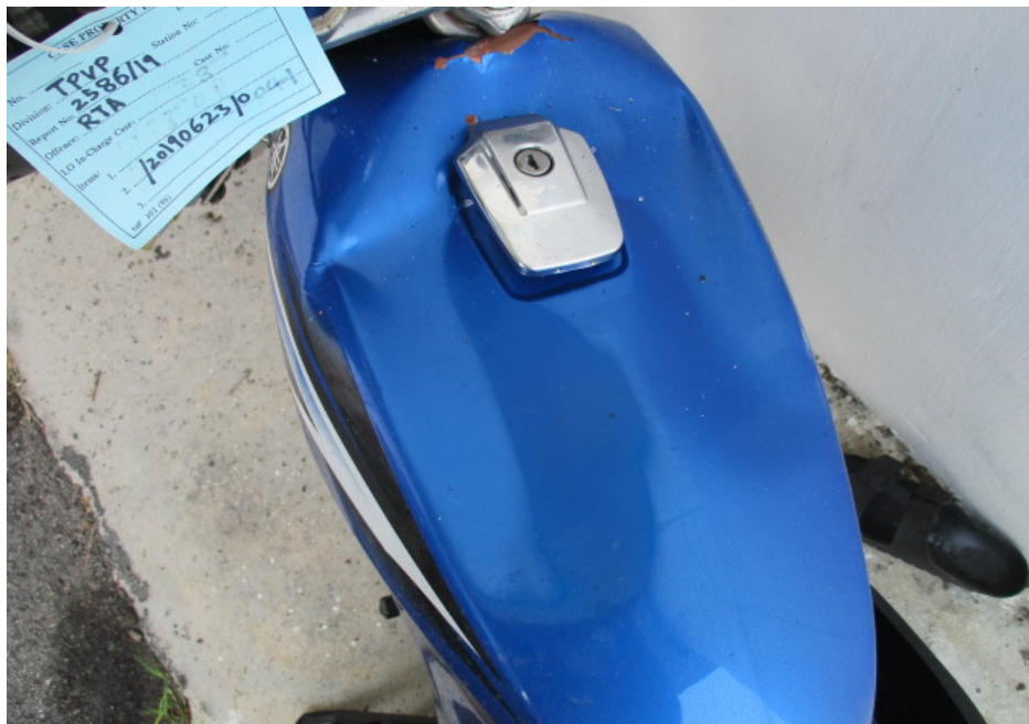
Photo 8 shows a closer view of the dented petrol tank, which was amongst the body parts of the Motorcycle that had sustained damage as a result of the accident.
