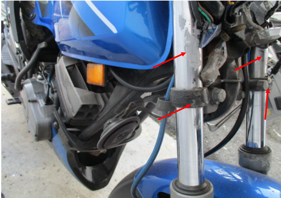
Photo 18 shows the front forks of the Motorcycle. The inner tube of the front forks and fork brackets were damaged as a result of the accident (arrowed). We were hence not able to conduct any tests on the steering system of the Motorcycle.
