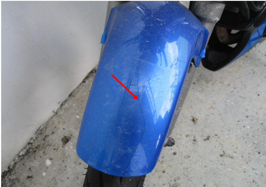
Photo 5 shows the general view of the cracked front mudguard (arrowed) of the Motorcycle as a result of the accident.
