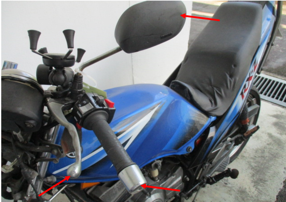
Photo 9 shows the clutch lever, left handlebar end and left side mirror which were amongst the body parts of the Motorcycle that had sustained damages of grazing nature as a result of the accident (arrowed).
