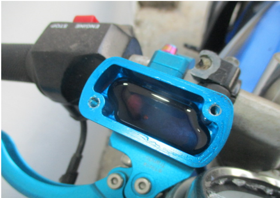
Photo 21 shows the brake fluid reservoir for the front brake of the Motorcycle. The brake fluid was observed to be of sufficient level and without contamination for operational purposes.
