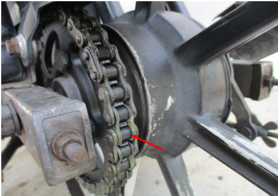
Photo 17 shows a closer view of the gear train (arrowed) of the Motorcycle, which was observed to be intact with no misalignment. It was also adequately lubricated for operating purposes.
