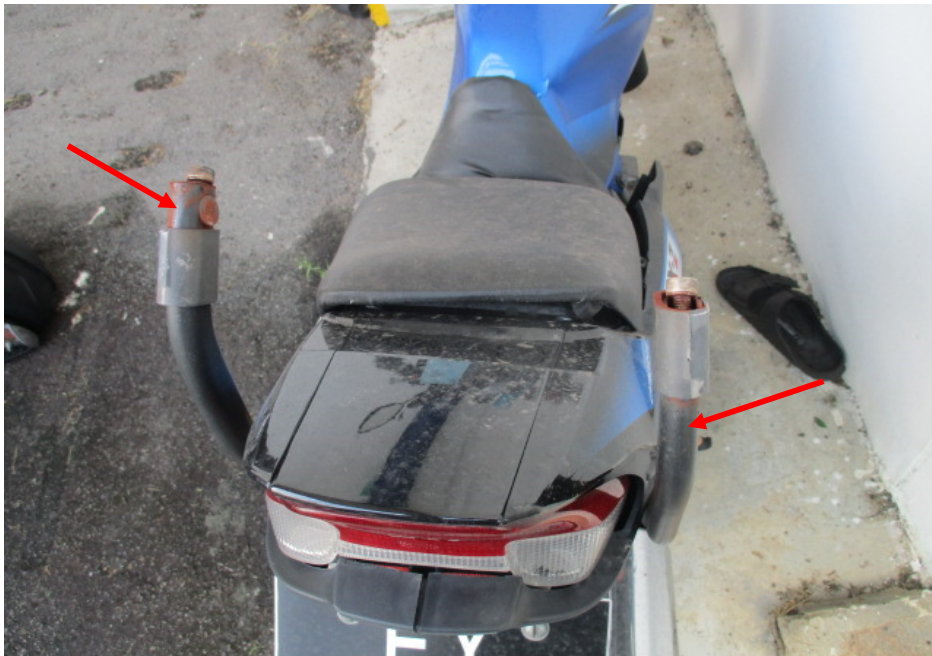
Photo 10 shows the bent top box rack (arrowed) of the Motorcycle as a result of the accident.
