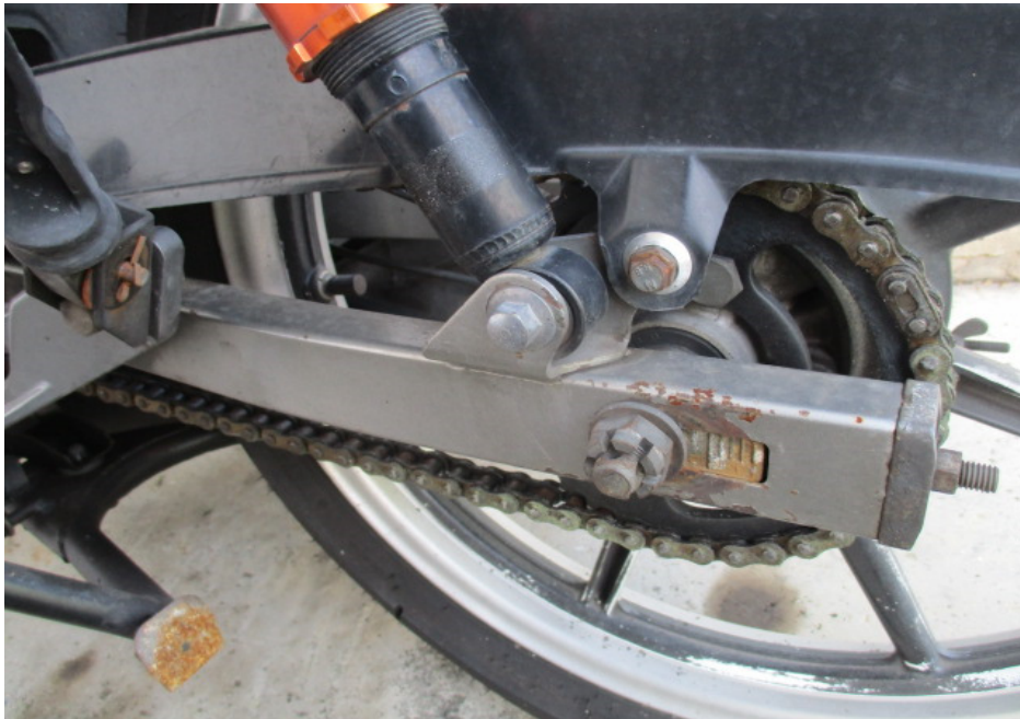
Photo 16 shows the general view of the gear train of the Motorcycle, which was observed to be intact with no misalignment. It was also adequately lubricated for operating purposes.
