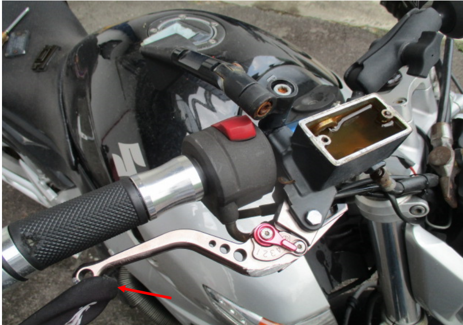
Photo 25 shows the front brake lever being depressed. There was some resistance felt (spongy like feel) upon pressing the front brake lever (arrowed). This would indicate that there is no leakage of pressure/vacuum in the brake system.
