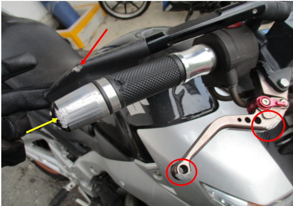
Photo 8 shows a closer view of the right handlebar end (yellow arrow), right side mirror (red arrow) and front brake lever (circled) which were amongst the body parts of the Motorcycle that had sustained damage as a result of the accident.
