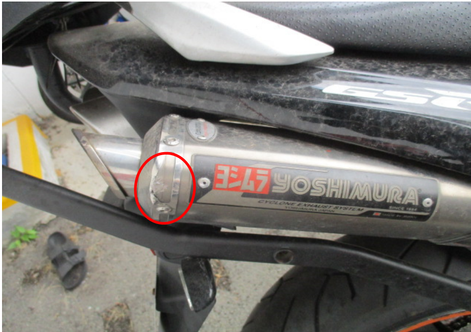
Photo 12 shows a closer view of the right exhaust muffler of the Motorcycle that had sustained damages of grazing nature as a result of the accident (circled).
