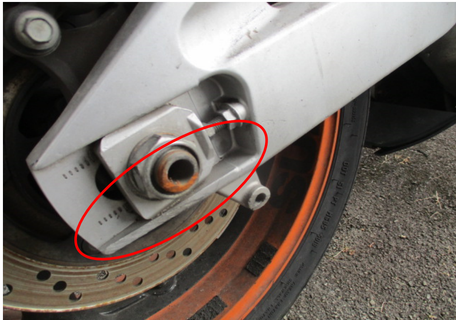
Photo 11 shows a closer view of the swingarm and rear wheel axle nut which were amongst the body parts of the Motorcycle that had sustained damages of grazing nature as a result of the accident (circled).
