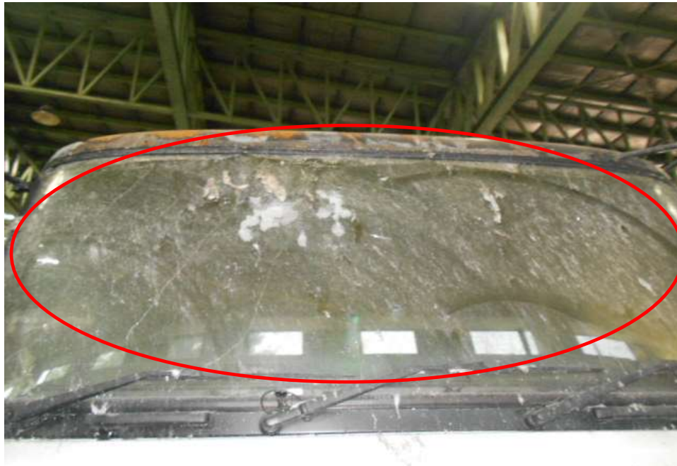
Photo 2 shows the close up view of the Insured Vehicle's cabin windscreen at the time of our inspection. The front windscreen of the Insured Vehicle had sustained heat and smoke damaged as a result of the fire (circled).
