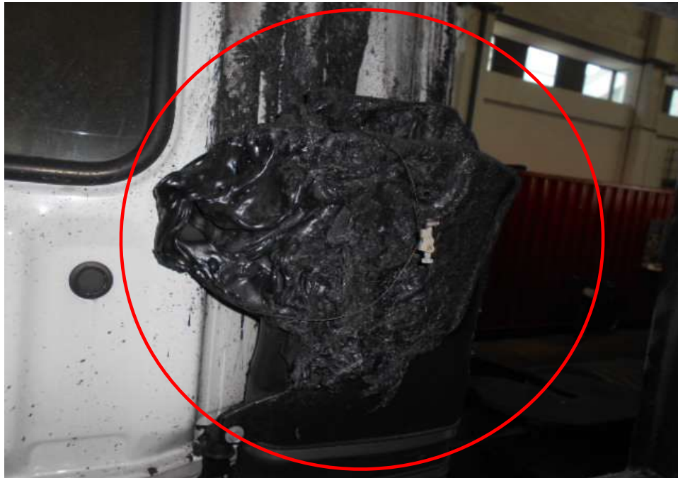
Photo 7 shows the close up view of the right side of the Insured Vehicle at the time of our inspection. The air filter box had sustained fire damage, smoke damage, melted from the top and fallen downwards as a result of the fire (circled).
