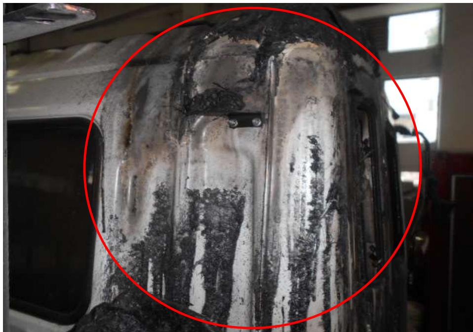
Photo 6 shows the close up view of the right side of the Insured Vehicle at the time of our inspection. The air filter box had sustained fire damage, smoke damage and melted as a result of the fire (circled).
