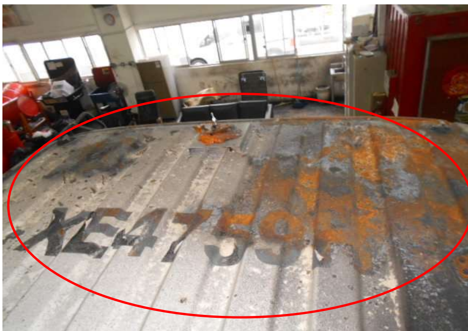
Photo 11 shows the fire damage at the exterior portion of the cabin top of the Insured Vehicle. The high heat intensity burn marks (whitish burn marks) found on the exterior surface of its cabin top as well as rust that had also developed on (circled) this indicates that the fire to the Insured Vehicle had originated from the exterior of the Insured Vehicle.
