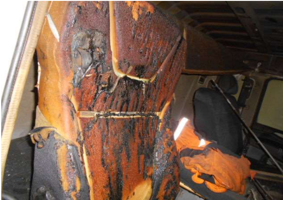
Photo 14 shows the close up view of the interior compartment of the Insured Vehicle at the time of our inspection. Its driver's chair material had suffered heat, smoke damage and melted down as a result of the fire.
