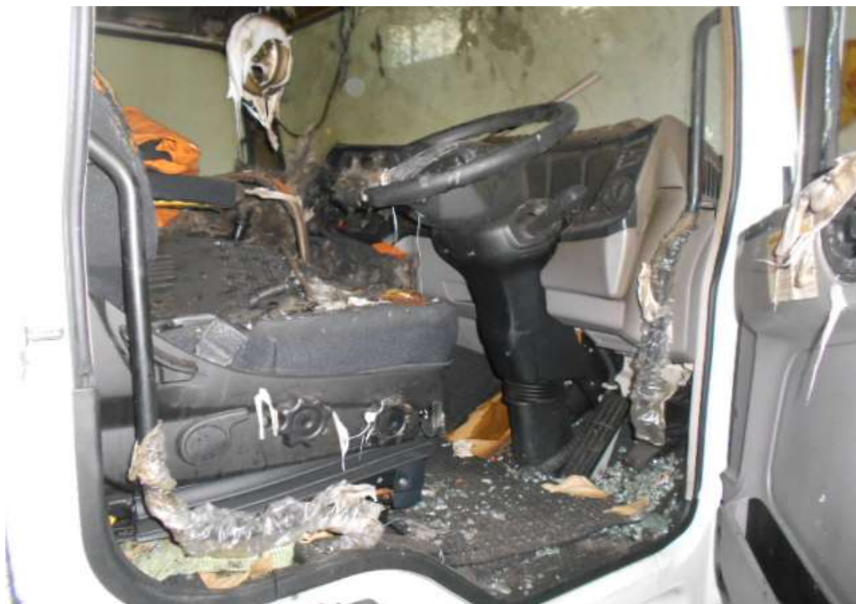
Photo 12 shows the general view of the interior compartment of the Insured Vehicle at the time of our inspection. Its interior compartment had suffered heat, smoke damage and melted as a result of the fire.
