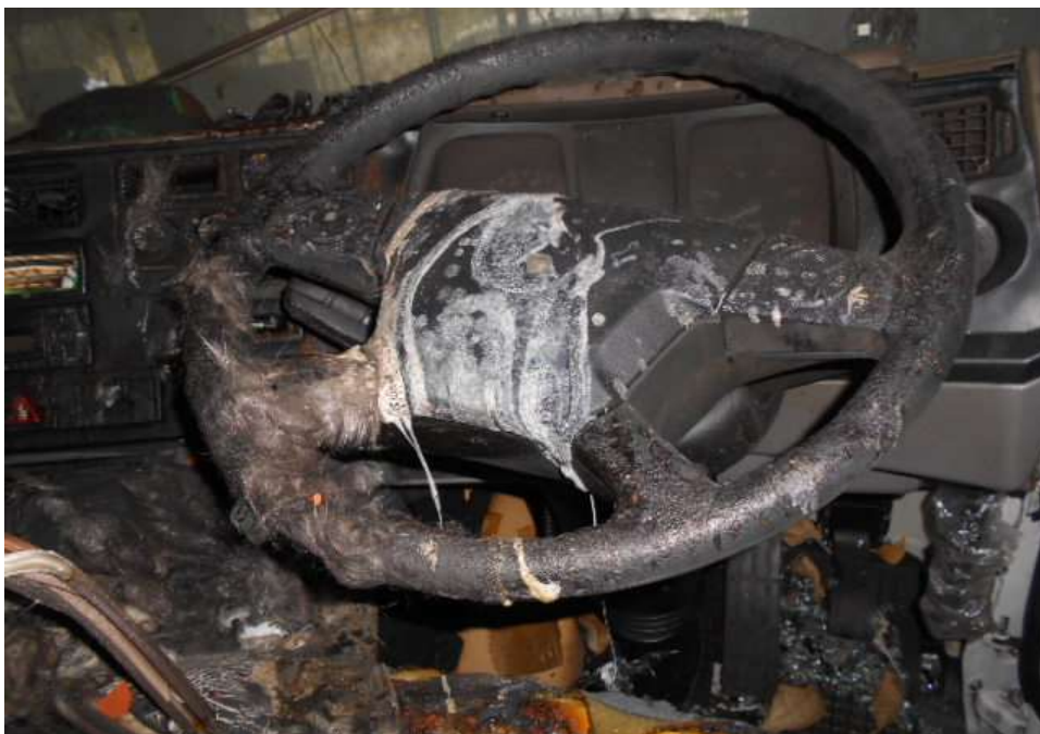
Photo 15 shows the close up view of the interior compartment of the Insured Vehicle at the time of our inspection. Its driver's steering wheel and dashboard material had suffered heat, smoke damage and melted down as a result of the fire.
