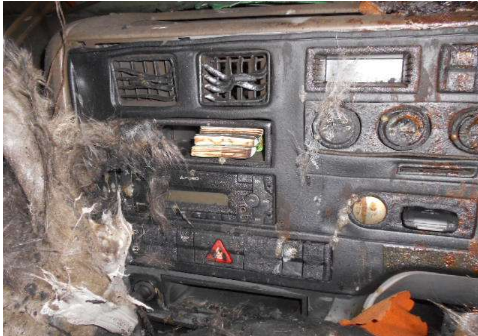
Photo 16 shows the close up view of the interior compartment of the Insured Vehicle at the time of our inspection. Its cabin instrument panels and dashboard components had suffered heat, smoke damage and melted down as a result of the fire.
