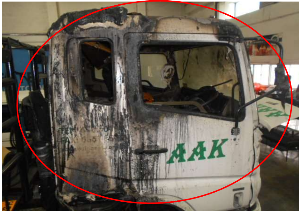
Photo 5 shows the general view of the right side of the Insured Vehicle at the time of our inspection. The door panel, air filter box and side mirror had sustained fire damage, smoke damage and melted as a result of the fire (circled).
