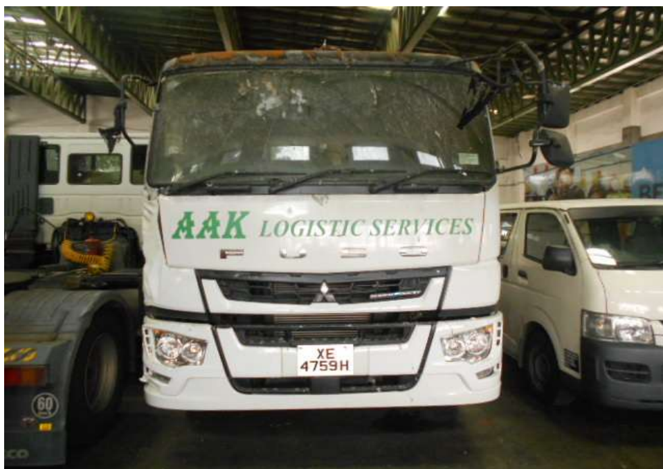
Photo 1 shows the front view of the Insured Vehicle at the time of our inspection. The heat and smoke damage to the Insured Vehicle was confined to its cabin portion. The rear portion of the Insured Vehicle was relatively unaffected by the fire.
