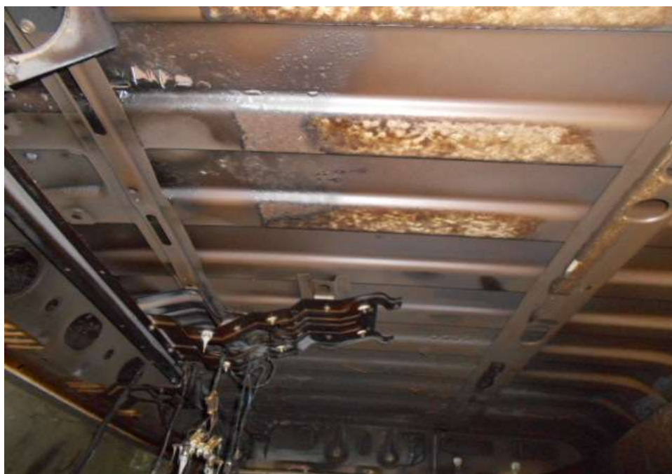
Photo 13 shows the close up view of the interior compartment of the Insured Vehicle at the time of our inspection. Its roof lining material had suffered heat, smoke damage and fallen off as a result of the fire.
