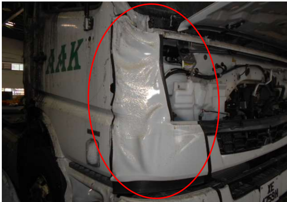
Photo 4 shows the close up view of the right side of the Insured Vehicle at the time of our inspection. The body panel had sustained heat damage and melted as a result of the fire (circled).
