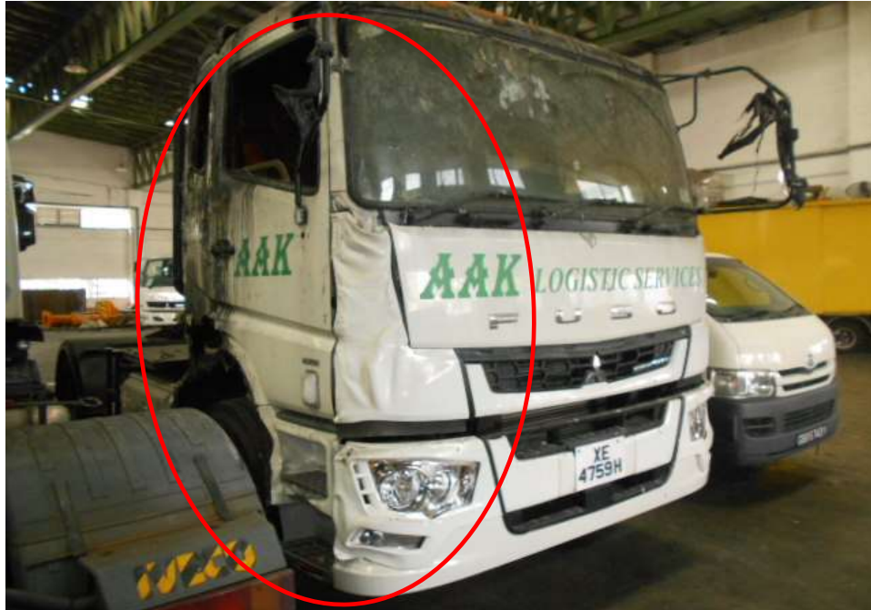
Photo 3 shows the right side view of the Insured Vehicle at the time of our inspection. The exterior body of the Insured Vehicle was affected by the heat. The body and door panels had sustained heat and smoke damage as a result of the fire (circled).
