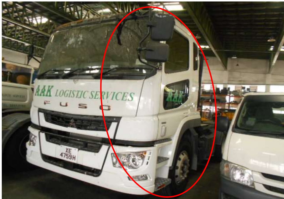
Photo 8 shows the left side view of the Insured Vehicle at the time of our inspection. The exterior body of the Insured Vehicle was affected by the fire. The body, door panels and side mirror had sustained fire and smoke damage as a result of the fire (circled).
