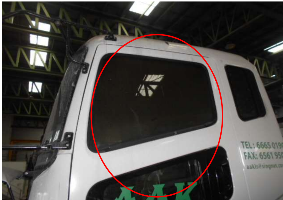
Photo 9 shows the close up view of the left side of the Insured Vehicle at the time of our inspection. The exterior body of the Insured Vehicle was affected by the fire. The body, door panels and windscreen had sustained fire and smoke damage as a result of the fire (circled).
