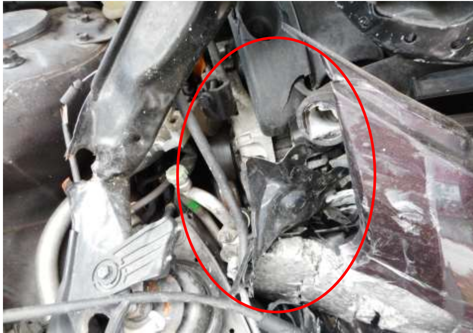
Photo 5 shows a close up view of the Motor Car's engine compartment at the time of my inspection. Due to the induced impact of the accident, the Motor Car's ignition system (red circle) and various components in the engine compartments were also damaged as a result of the accident.
