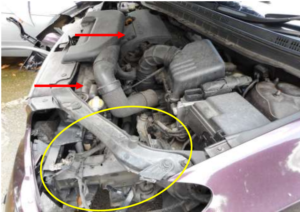
Photo 3 shows a close up view of the Motor Car's engine compartment at the time of my inspection. Its battery was missing (yellow circle). Due to the induced impact of the accident, the Motor Car's engine system, ignition system, cooling system (red arrows) and various components in the engine compartments were also damaged as a result of the accident.
