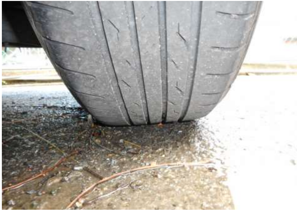
Photo 11 shows the condition of the rear left tyre of the Motor Car, which was observed to be in serviceable condition with remaining tread depth of approximately 3.2mm. The tyre was also observed to be sufficiently inflated for vehicular operation with no tear, cut or burst mark(s).
