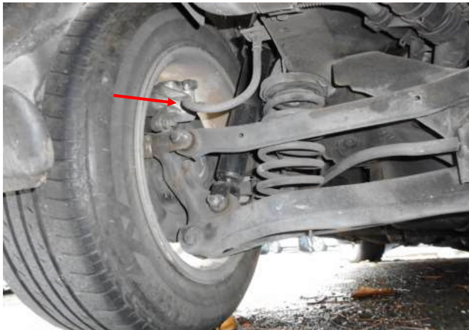
Photo 16 shows the brake hose/pipe (arrowed) at the rear left wheel of the Motor Car and it was observed to be intact
