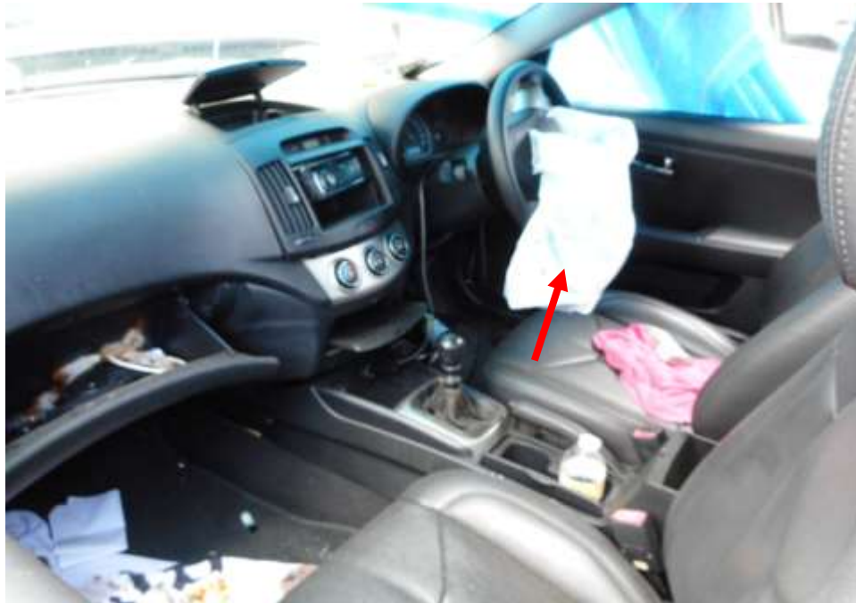
Photo 13 shows the deployment of the Supplemental Restraint System (SRS) airbag (arrowed), as a result of the accident.
