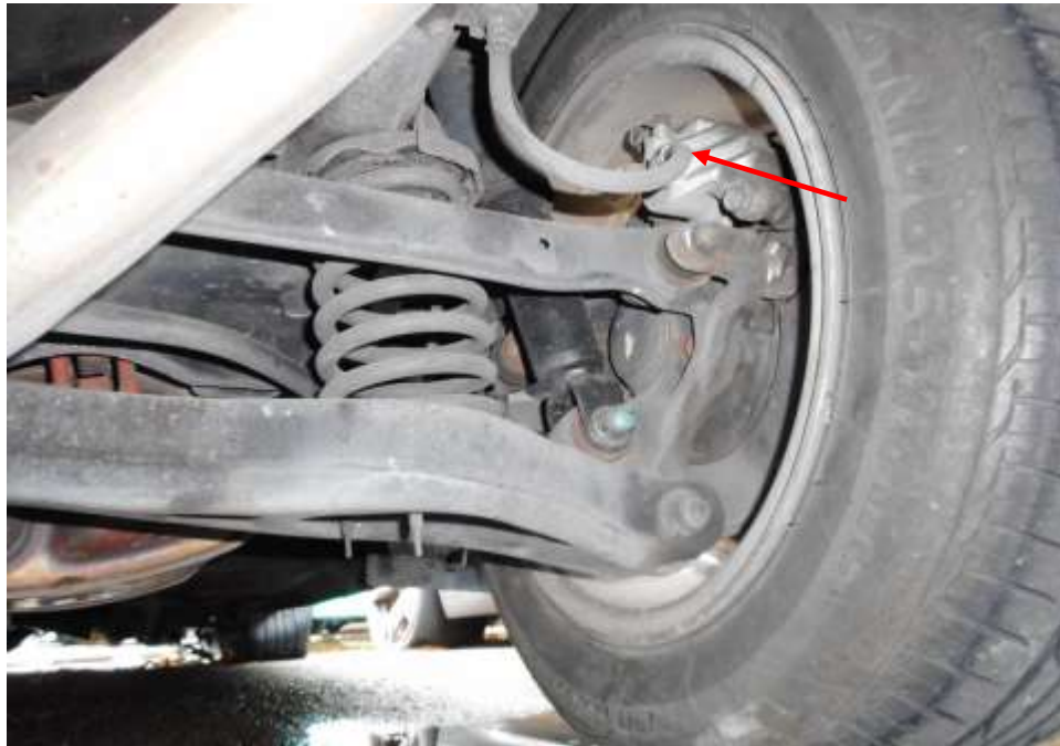
Photo 17 shows the brake hose/pipe (arrowed) at the rear right wheel of the Motor Car and it was observed to be intact
