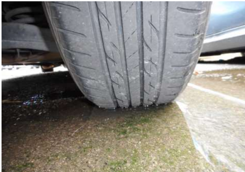
Photo 10 shows the condition of the rear right tyre of the Motor Car, which was observed to be in serviceable condition with remaining tread depth of approximately 4.3mm. The tyre was also observed to be sufficiently inflated for vehicular operation with no tear, cut or burst mark(s).
