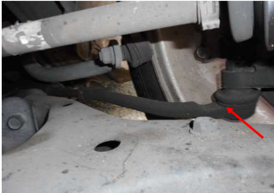
Photo 19 shows the various undercarriage components at the front left wheel of the Motor Car, the steering tie rod (red arrow) was found to be intact.
