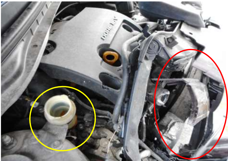
Photo 4 shows a close up view of the Motor Car's engine compartment at the time of my inspection. Due to the induced impact of the accident, the Motor Car's braking system (yellow circle), cooling system (red circle) and various components in the engine compartments were also damaged as a result of the accident.
