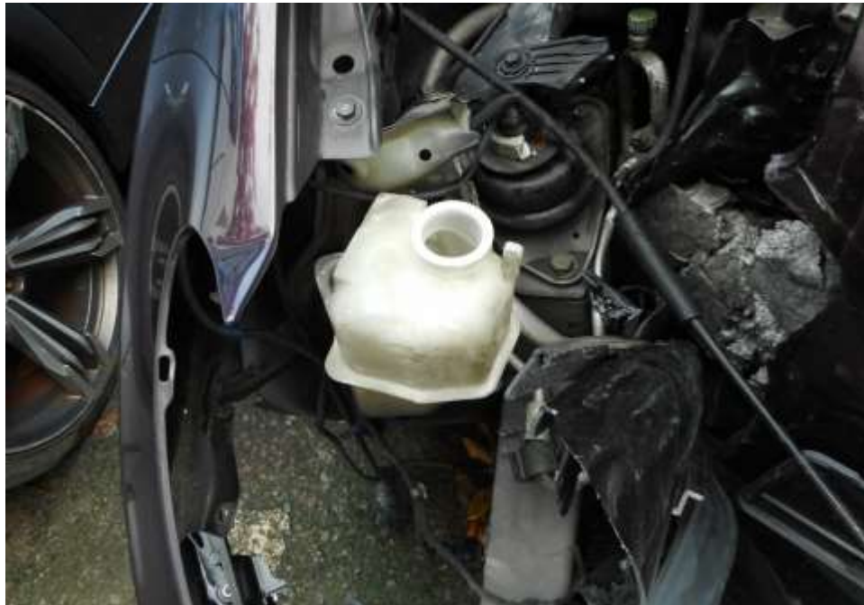
Photo 15 shows coolant reservoir of the Motor Car at the time of my inspection. The coolant level was observed to be of insufficient as a result of the accident.
