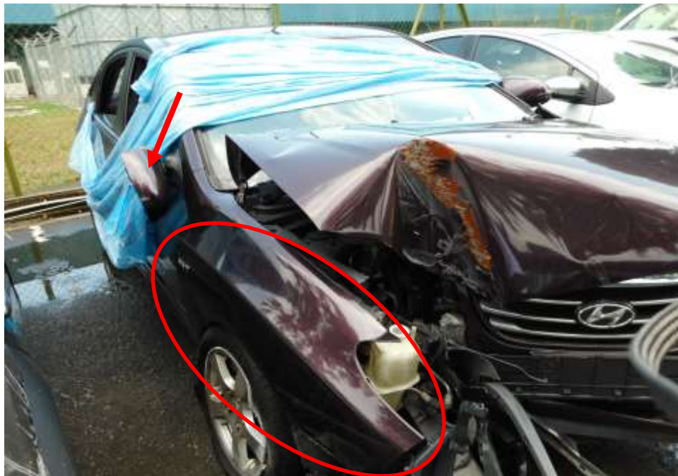
Photo 6 shows the general view of the Motor Car's right body at the time of my inspection. Its front right fender (red circle) and right rear mirror (red arrow) was amongst the body parts that were damaged as a result of the accident.
