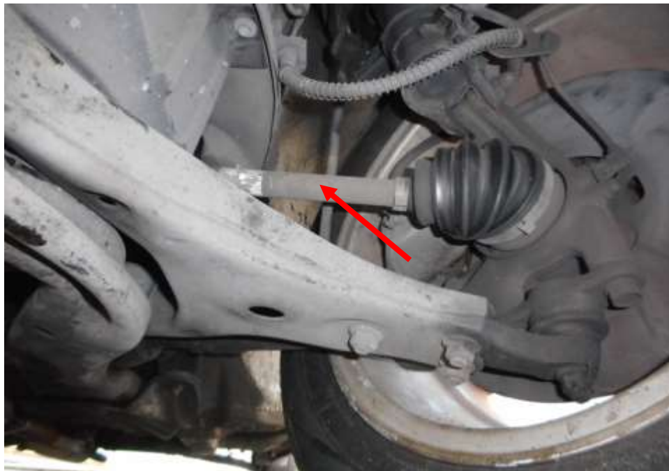
Photo 18 shows the various undercarriage components at the front left wheel of the Motor Car, the driveshaft (red arrow) was found to be intact.
