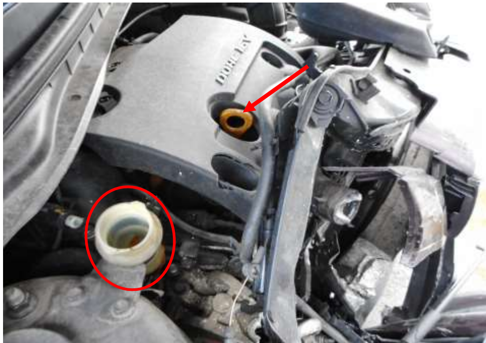
Photo 14 shows a general view of the Motor Car's engine compartment and the various parts and components inside the engine compartment. The brake fluid reservoir (circled) and the engine oil dip stick (arrowed) was insufficient and stuck as a result of the accident
