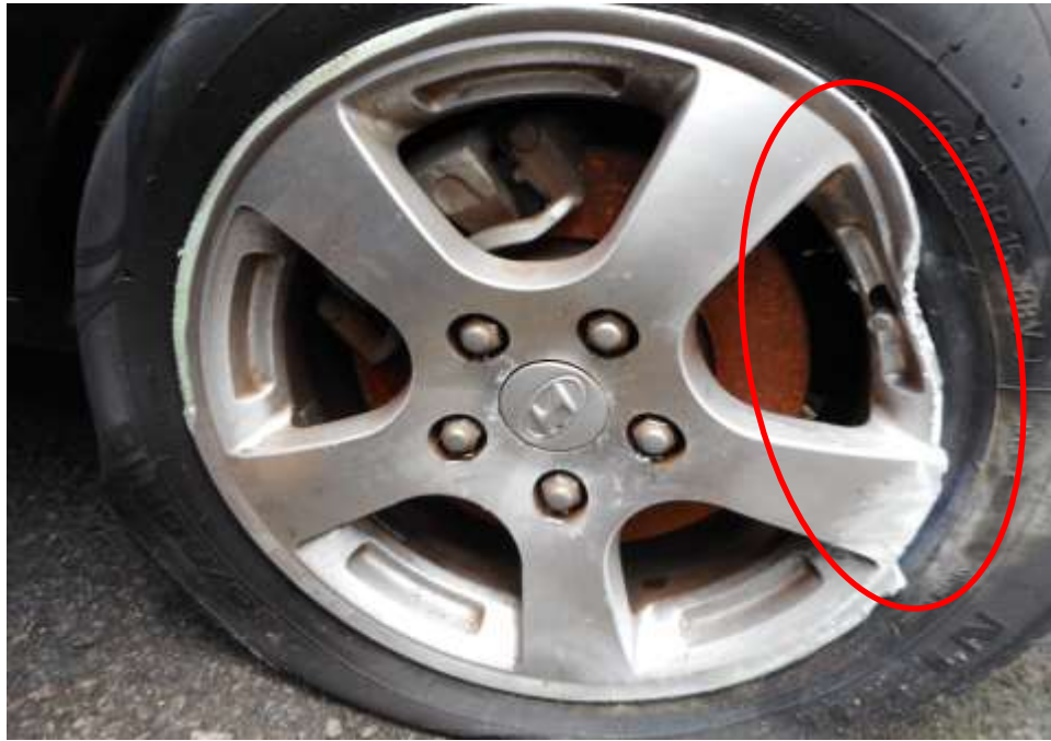
Photo 9 shows the condition of the front right tyre of the Motor Car, the rim was observed to be damaged (circled) as a result of the accident and the tyre was observed to be in deflated condition due to the air leakage from the damaged rim. The remaining tread depth of the tyre was approximately 5.1mm. There was also no tear, cut or burst mark(s) on the outer and the inner sidewalls as well as across the tread of the Motor Car's 4 tyres.
