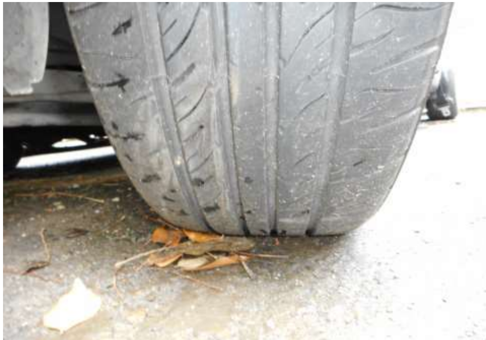
Photo 12 shows the condition of the front left tyre of the Motor Car, which was observed to be in serviceable condition with remaining tread depth of approximately 4.8mm. The tyre, which was wrapped around alloy wheel rim, was also observed to be sufficiently inflated for vehicular operation. There were minor scratches on the surface of the wheel rim as a result of the accident.
