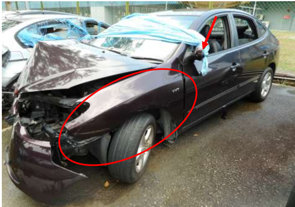
Photo 7 shows the general view of the Motor Car's left body at the time of my inspection. Its front left fender (red circle) and left rear mirror (red arrow) was amongst the body parts that were damaged as a result of the accident.
