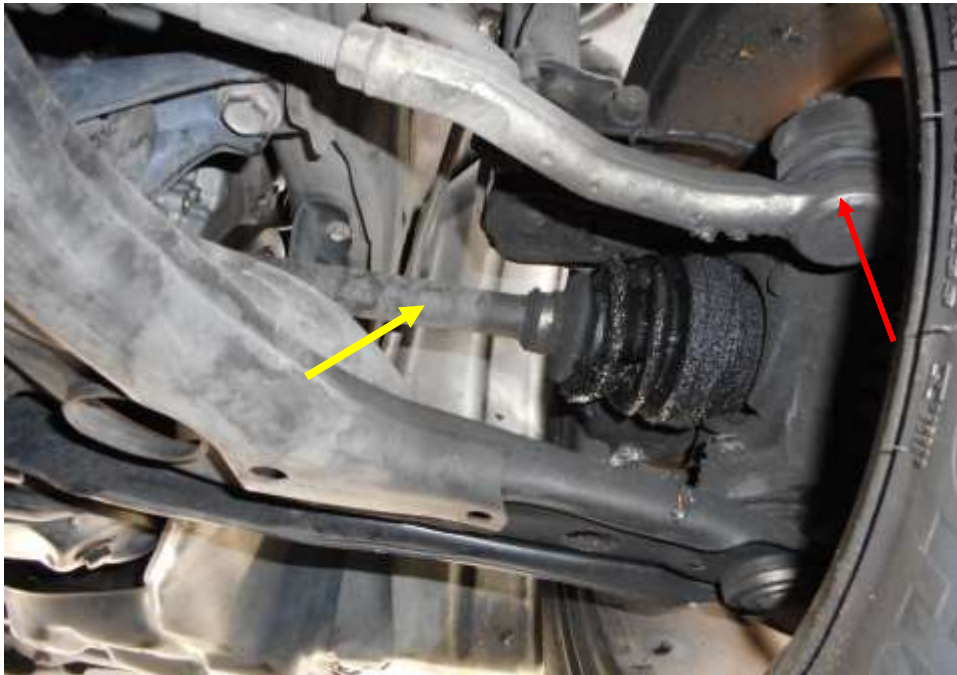
Photo 26 shows the various undercarriage components at the front right wheel of the Motor Car, the steering tie rod (red arrow) and the driveshaft was found to be intact suggesting that it was serviceable at the time of the accident.
