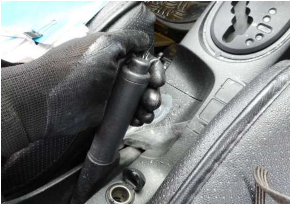
Photo 27 shows the static test conducted on the handbrake of the Motor Car by pulling and releasing it multiple times and it did not reveal any abnormalities suggesting that it is in serviceable condition at the time of the accident.
