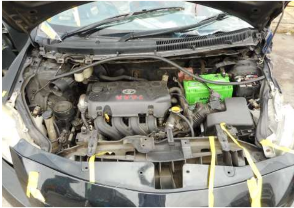
Photo 15 shows a general view of the Motor Car's engine compartment and the various parts and components inside the engine compartment. There was also no sign(s) or indication(s) of fluid leakage and/or fluid stain within the engine compartment.
