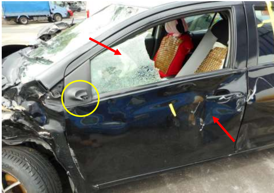
Photo 7 shows the close up view of the Motor Car's left body at the time of my inspection. Its front left door panel, front left windscreen (red arrow) and left rear mirror (yellow circle) was amongst the body parts that were damaged as a result of the accident.
