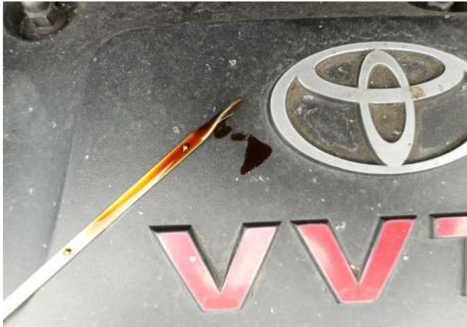
Photo 16 shows checks being carried out to the engine oil of the Motor Car at the time of my inspection. The engine oil on the indicator dip stick was observed to be of sufficient level and without any visible contamination.
