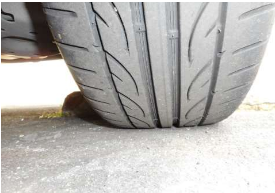
Photo 12 shows the condition of the rear left tyre of the Motor Car, which was observed to be in serviceable condition with remaining tread depth of approximately 4.9mm. The tyre was also observed to be sufficiently inflated for vehicular operation with no tear, cut or burst mark(s).
