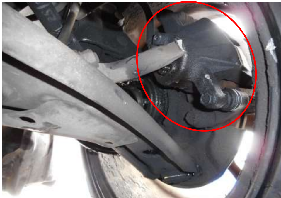
Photo 23 shows the brake caplier (circled) at the front left wheel of the Motor Car. We observed old brake and fresh brake fluid stain on the surface on the brake caplier. The leakage was cause by the induced impact of the collision as a result of the accident.
