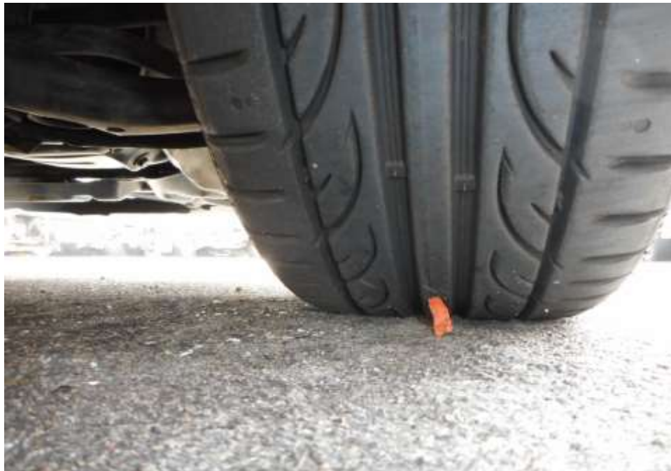
Photo 10 shows the condition of the front right tyre of the Motor Car, which was observed to be in serviceable condition with remaining tread depth of approximately 5.9mm. The tyre was sufficiently inflated for vehicular operation. There was also no tear, cut or burst mark(s) on the outer and the inner sidewalls as well as across the tread of the Motor Car's 4 tyres.
