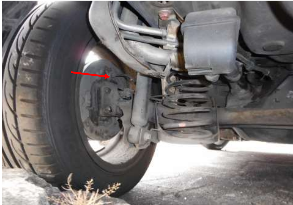
Photo 20 shows the brake hose/pipe (arrowed) at the rear left wheel of the Motor Car. It was observed to be intact and undamaged by the accident.
