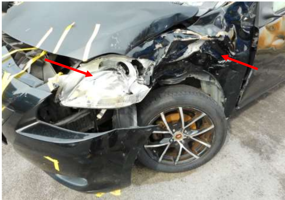
Photo 6 shows a close up view of the Motor Car's left body at the time of my inspection. Its front left headlamp and front left fender (arrowed) was amongst the body parts that were damaged as a result of the accident.
