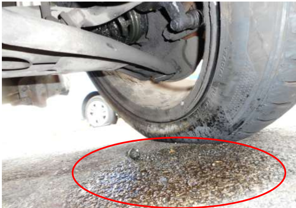
Photo 25 shows the front left wheel, a patch of brake fluid stain (circled) on the ground from the leaking brake caplier and a ball bearing which is part of the CV joint assembly (arrowed) which have fallen out, both is caused by the induced impact as a result of the accident.
