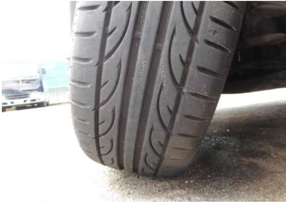
Photo 13 shows the condition of the front left tyre of the Motor Car, which was observed to be in serviceable condition with remaining tread depth of approximately 5.9mm. The tyre, which was wrapped around alloy wheel rim, was also observed to be sufficiently inflated for vehicular operation. There were minor scratches on the surface of the wheel rim as a result of the accident.
