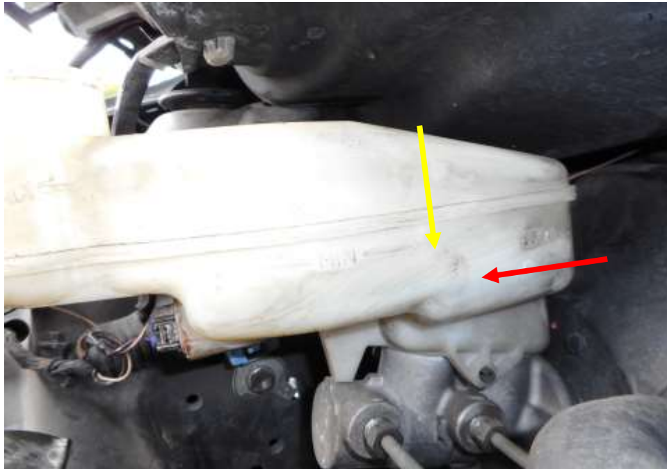
Photo 17 shows the brake fluid reservoir of the Motor Car at the time of my inspection. The brake fluid was observed to be of insufficient level (red arrow) and below the minimum mark (yellow arrow). A leakage was observed at the brake caplier as a result of the accident.
