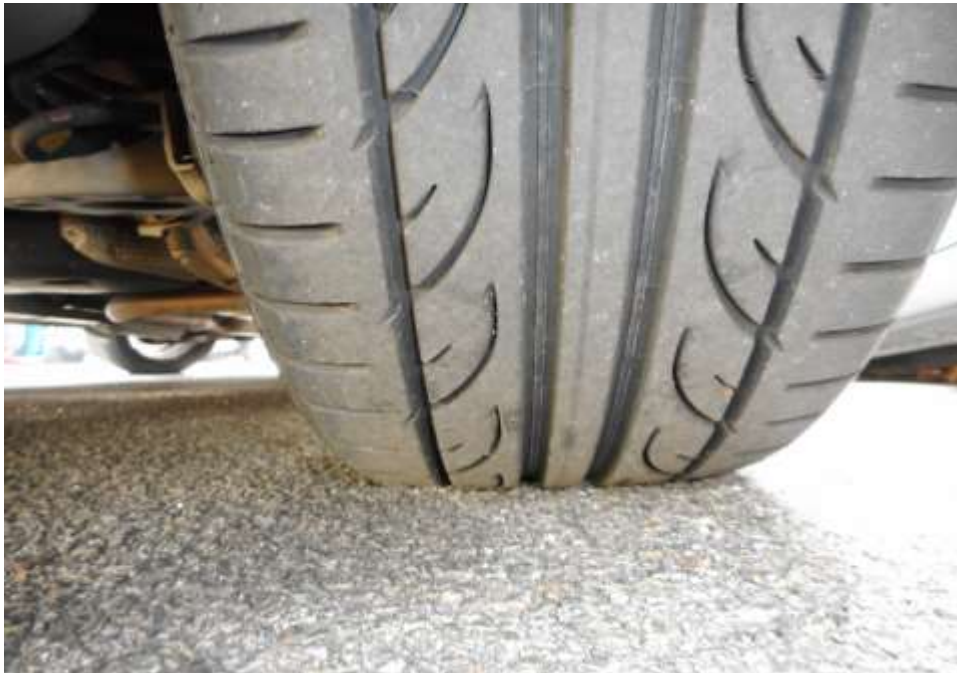
Photo 11 shows the condition of the rear right tyre of the Motor Car, which was observed to be in serviceable condition with remaining tread depth of approximately 4.9mm. The tyre was also observed to be sufficiently inflated for vehicular operation with no tear, cut or burst mark(s).
