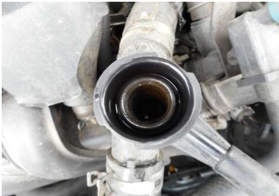
Photo 18 shows checks being carried out to the engine coolant of the Motor Car at the time of my inspection. The engine coolant was observed to be of sufficient level and without any visible contamination.
