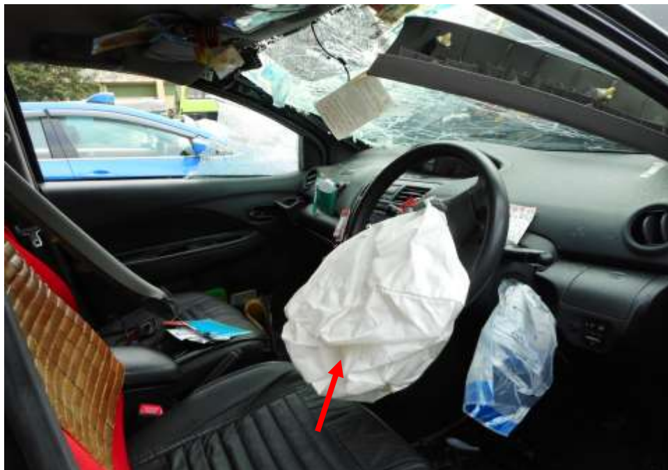
Photo 14 shows the deployment of the Supplemental Restraint System (SRS) airbag (arrowed), as a result of the accident.
