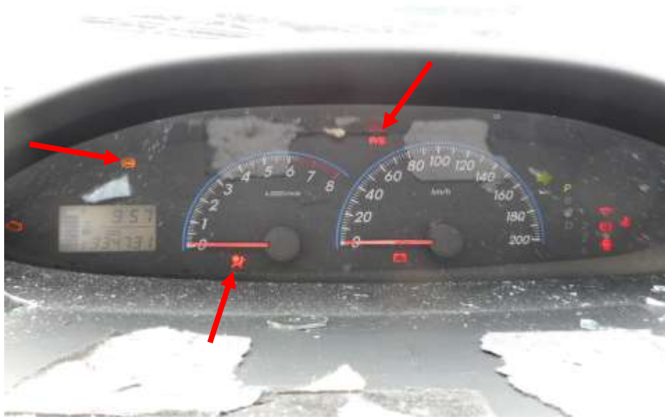
Photo 28 shows the warning light for Anti-Lock Brake System (ABS), Electric Power Steering System (EPS) and Supplemental Restraint System (SRS) appearing on the instrument panel of the Motor Car during the self-test of its various electronic operating systems when its engine was cranked.
