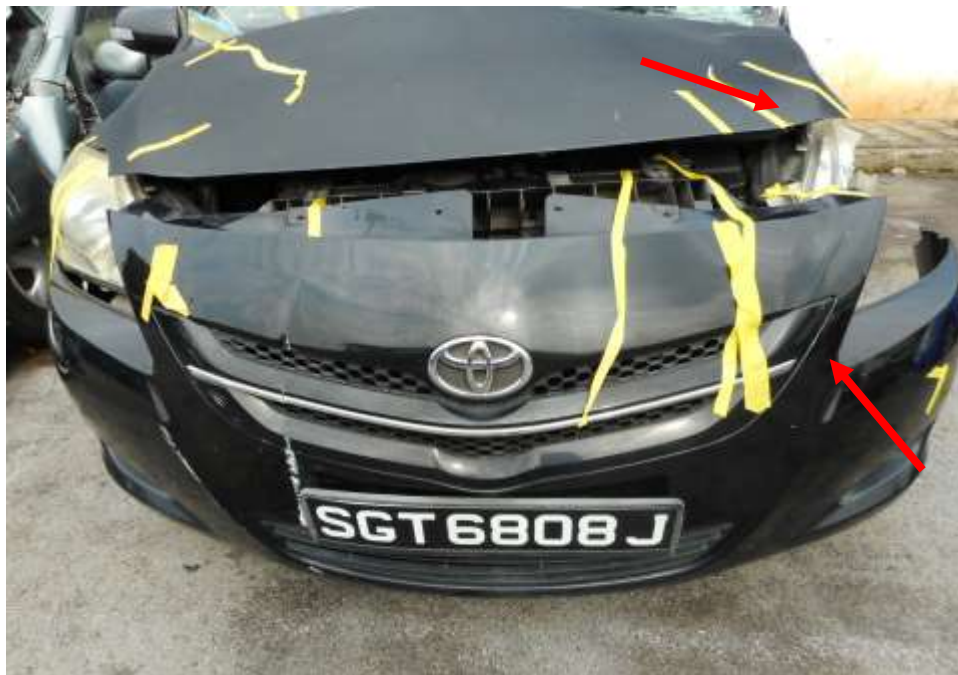
Photo 4 shows a close up view of the Motor Car's front body at the time of my inspection. Its front bonnet and front bumper body panel (arrowed) was amongst the body parts that were damaged as a result of the accident.
