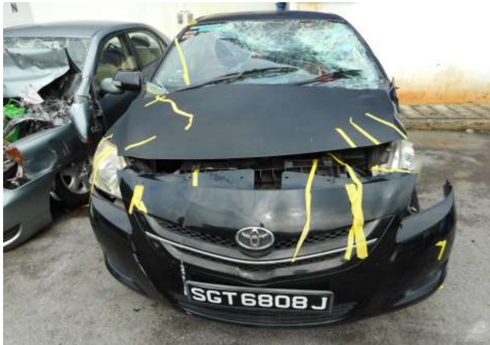
Photo 2 shows a general view of the Motor Car's front body at the time of my inspection. The Motor car was observed to have sustained moderate damage at its front and left side portion. Its front windscreen, front bonnet, front bumper, front left headlamp, front left fender, front left door panel, front left windscreen and left rear mirror was amongst the body parts that were damaged as a result of the accident. The Supplemental Restraint System (SRS) was activated as a result of the accident.
