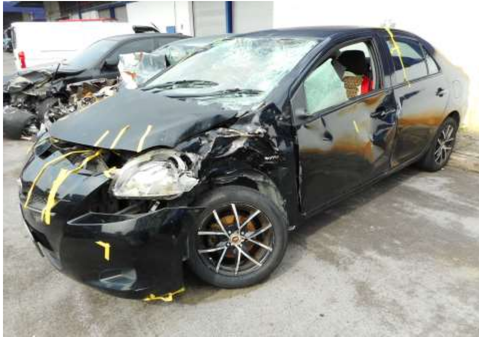
Photo 5 shows the general view of the Motor Car's left body at the time of my inspection. Its front left headlamp, front left fender, front left door panel, front left windscreen and left rear mirror was amongst the body parts that were damaged as a result of the accident.
