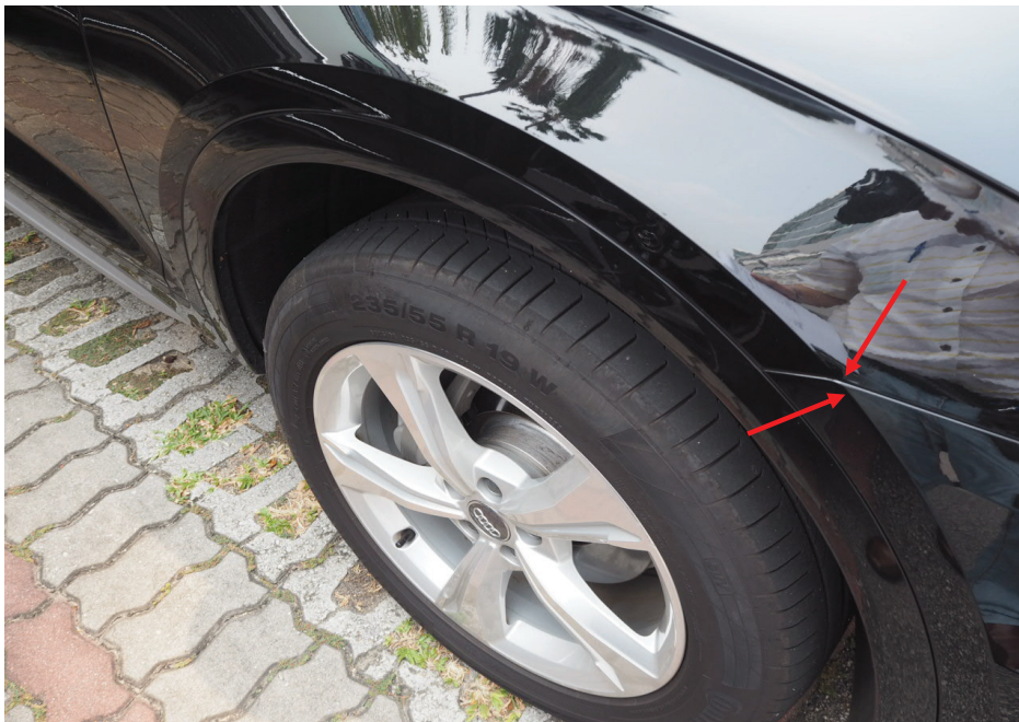
Photo 6 shows a close up view of the right corner edge of the front bumper of the Audi. We observed that there was no misalignment at the corner edges (red arrows).
