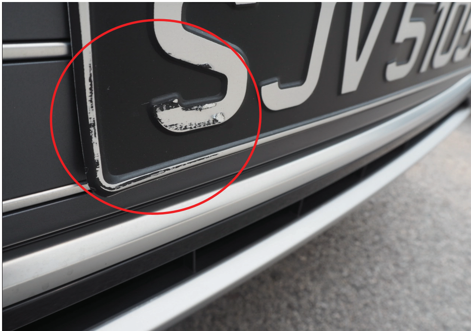
Photo 5 shows a close up view of the black marks on the lower portion of the alpha- numeric letterings of the Audi's front number plate (circled).
