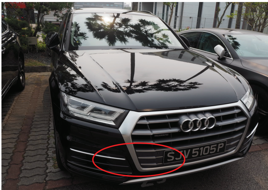
Photo 1 shows the general view of the front portion of the Audi at the time of the Pre- Repair Survey conducted by LKK Auto Consultants Pte. Ltd. which was taken about 4 days after the accident. The damage to the Audi was observed to be confined to the right portion of its front bumper and front number plate.
