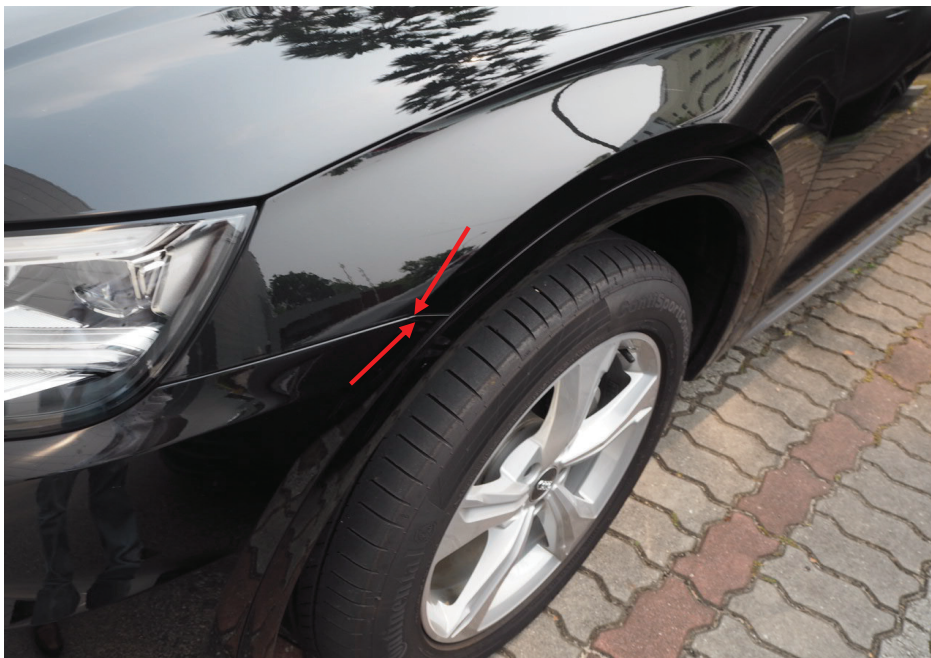
Photo 7 shows a close up view of the left corner edge of the front bumper of the Audi. We observed that there was no misalignment at the corner edges (red arrows).
