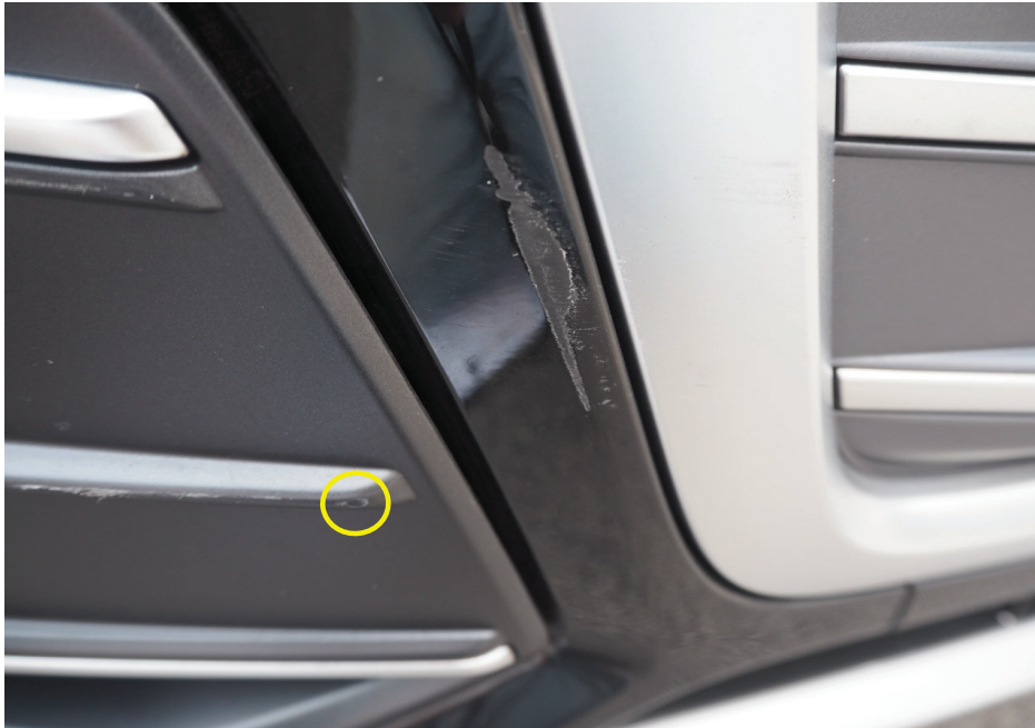
Photo 4 shows a close up view of the circular indentation on the front right grille of the Audi (circled).
