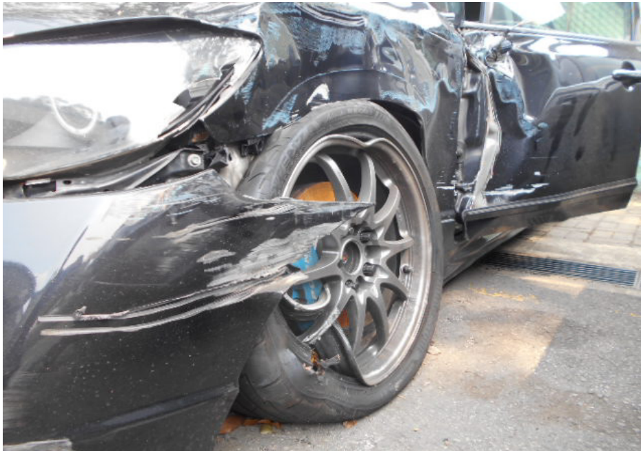
Photo 3 shows a closer view of the damage to the front bumper, front left wheel rim, front left fender, front left headlamp and front left door of the insured vehicle.
