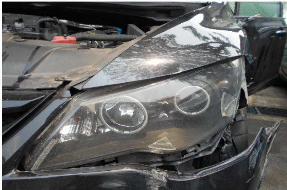
Photo 12 shows the aftermarket front left headlamp that was fitted on the insured vehicle. This aftermarket front headlamp is LTA compliant.
