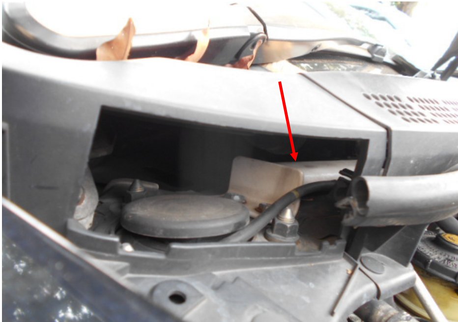
Photo 9 shows the additionally fitted front strut bar (arrowed) that was found inside the engine compartment of the insured vehicle. This strut bar is LTA compliant and improves the stability of the insured vehicle during cornering.
