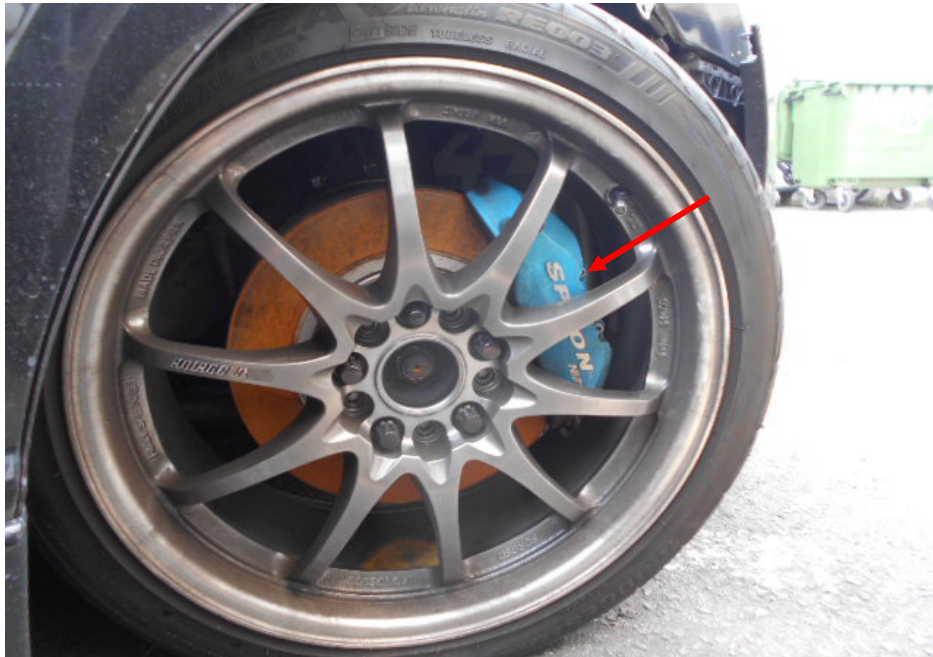
Photo 11 shows the aftermarket front brake caliper (arrowed) that was fitted on the front right wheel of the insured vehicle. The front brake system of the insured vehicle is LTA compliant. The overall braking efficiency will be enhanced.
