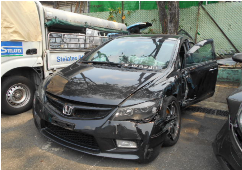
Photo 2 shows the front left body of the insured vehicle at the time of my inspection. The insured vehicle sustained relatively moderate damage at its left front portion. Without dismantling of any exterior body parts, I had observed damage to its front bumper, front left headlamp, front left fender, front left door and left wing mirror amongst others.
