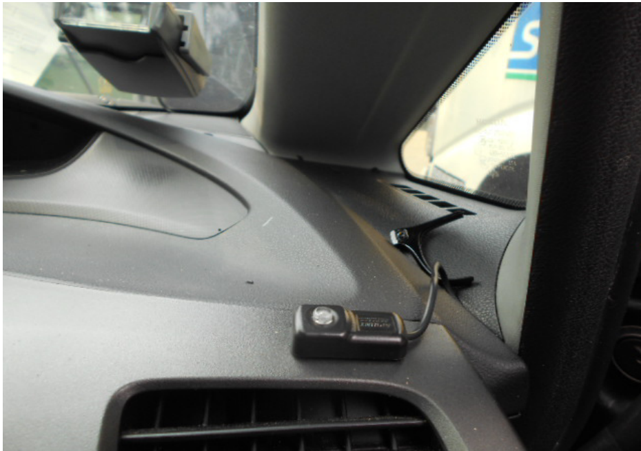
Photo 15 shows the accessory for the additionally fitted boost sprinter device that was fitted on the insured vehicle at the time of my inspection. The boost sprinter device is LTA compliant. It enhances the acceleration/throttle response of the insured vehicle.
