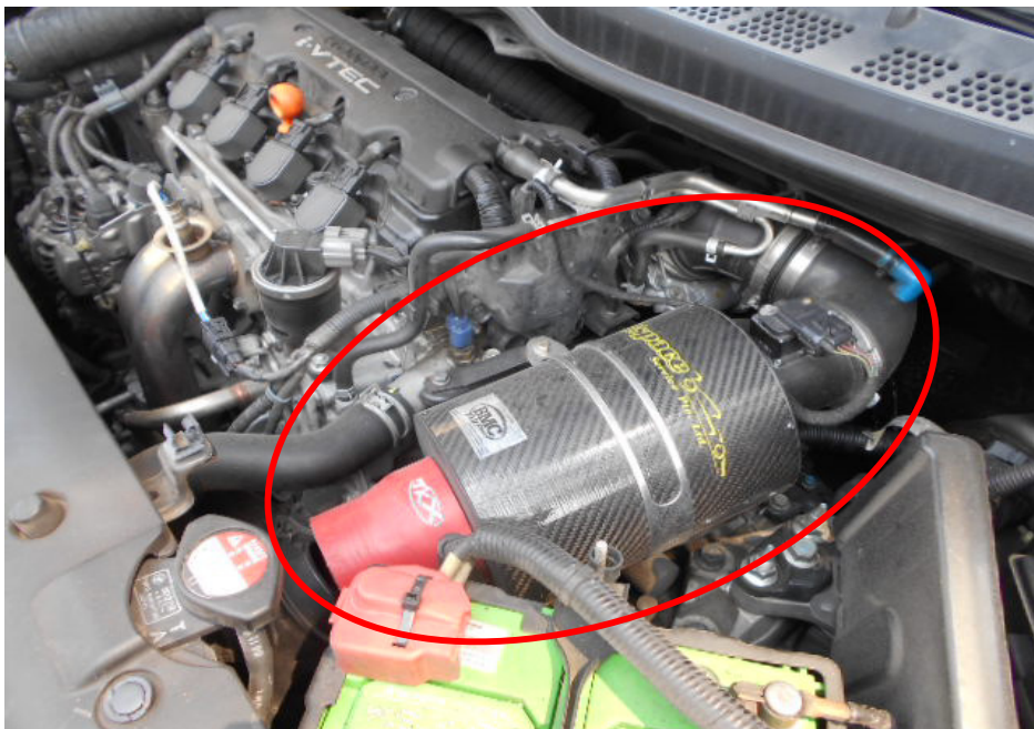
Photo 8 shows the aftermarket air intake system with piping (circled) that was fitted on the insured vehicle at the time of my inspection. This air intake system fitted on the insured vehicle is LTA compliant. The overall engine performance of the insured vehicle will be improved.
