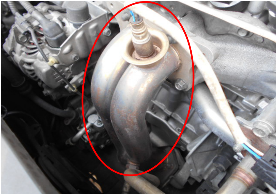
Photo 7 shows another view of the aftermarket exhaust manifold (circled) that was fitted on the insured vehicle at the time of my inspection. This exhaust manifold fitted on the insured vehicle is not LTA compliant. Owner does not have any approval letter from LTA for the aftermarket exhaust manifold. The overall engine performance of the insured vehicle will be improved.
