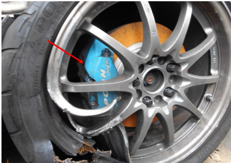
Photo 10 shows the aftermarket front brake caliper (arrowed) that was fitted on the front left wheel of the insured vehicle. The front brake system of the insured vehicle was observed to be of an aftermarket brand.
