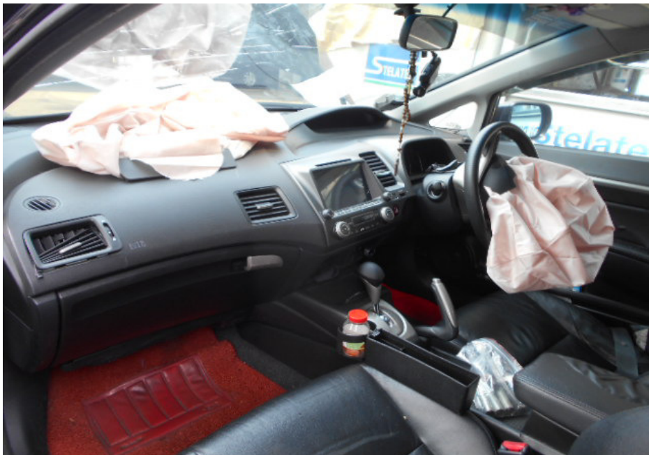
Photo 4 shows the interior compartment of the insured vehicle at the time of my inspection. The driver's airbag and front left passenger's airbag were observed to be deployed. The driver's seat belt and front left passenger's seat belt were also found to be locked when I tested.
