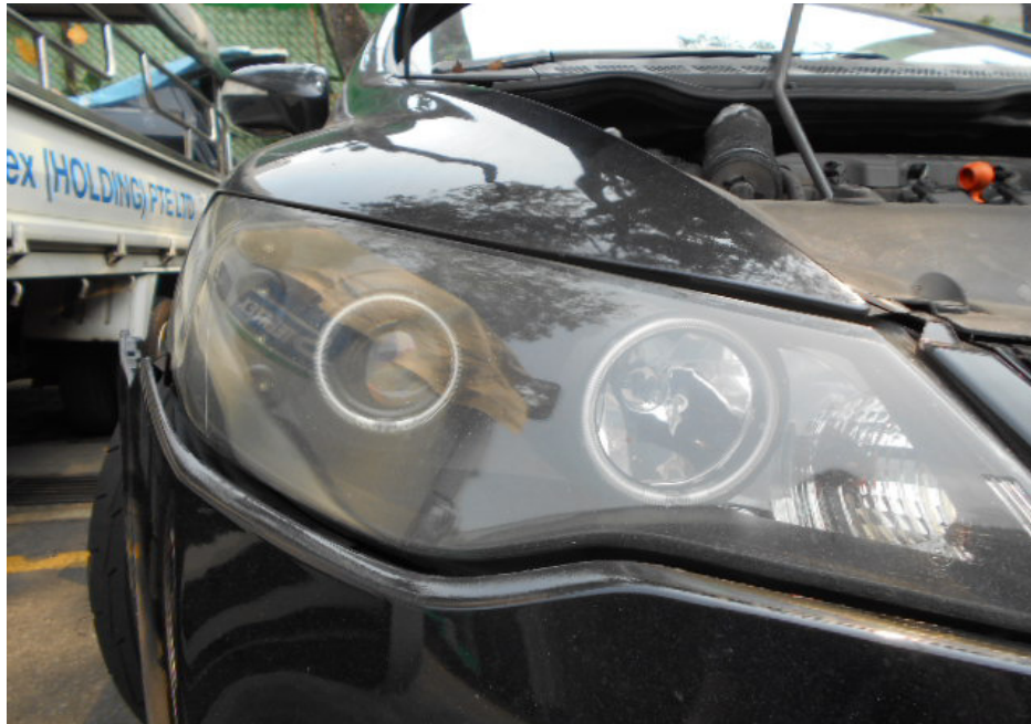
Photo 13 shows the aftermarket front right headlamp that was fitted on the insured vehicle. This aftermarket front headlamp is LTA compliant and a cosmetic type of modification.
