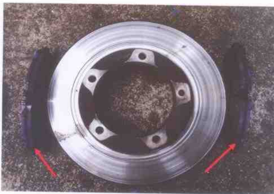
Photo 9 shows the front right inner and outer brake pads (arrowed) and the front right disc brake of the Insured Vehicle. The brake pad's braking material was observed to be of sufficient level. However the other outer side of the brake pad was missing at the time of my inspection, which will reduce the braking efficiency of the Insured Vehicle.
