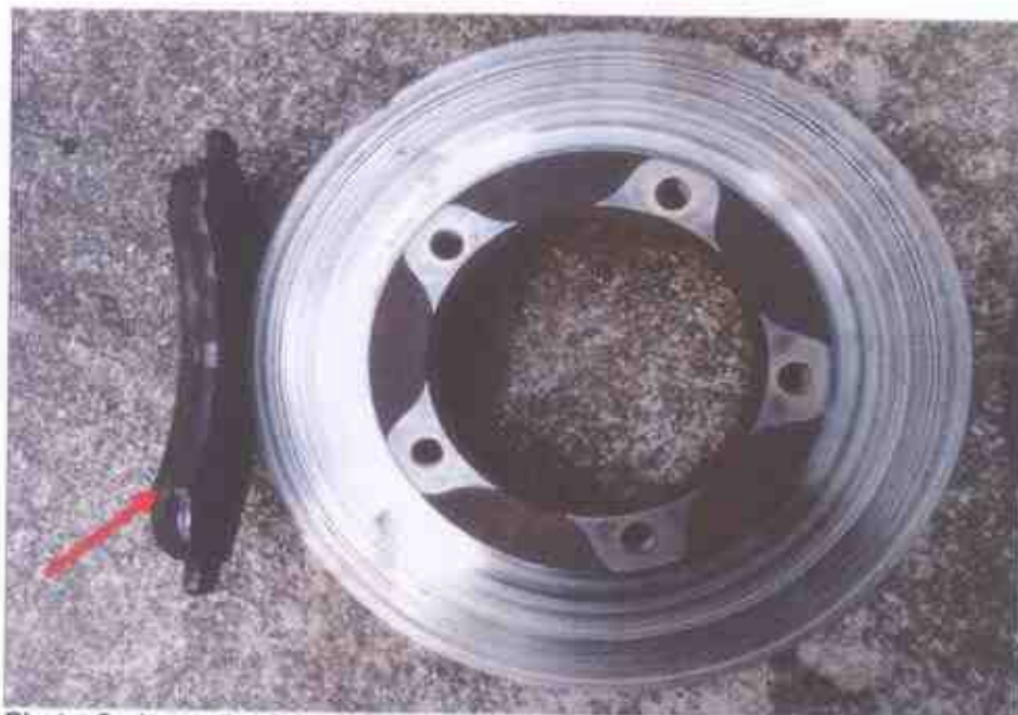
Photo 8 shows the front left inner brake pad (arrowed) and the front left disc brake of the Insured Vehicle. The brake pad's braking material was observed to be of sufficient level. However the other outer side of the brake pad was missing at the time of my inspection, which will cause the braking efficiency of the Insured Vehicle to be reduced.
