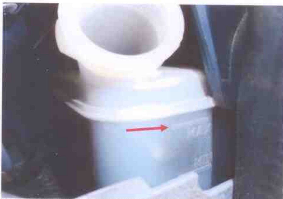
Photo 6 shows the brake fluid reservoir of the Insured Vehicle at the time of my inspection. The brake fluid was observed to be of sufficient level (arrowed) and without any visible contamination.
