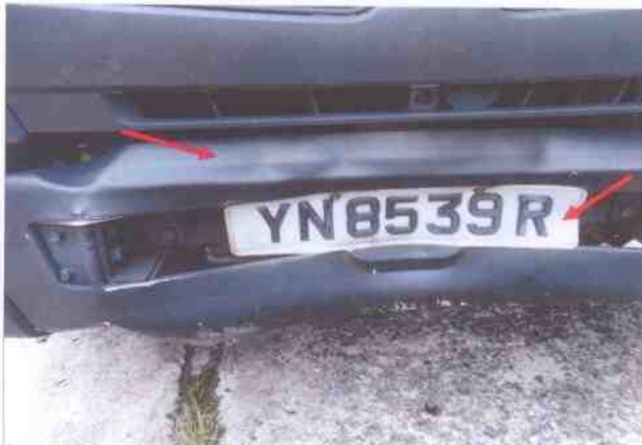
Photo 2 shows the close up view of the front portion of the Insured Vehicle at the time of our inspection. The damage to the Insured Vehicle was confined to its front bumper portion and number plate (arrowed) is amongst the body parts that were found to have been affected as a result of the accident.
