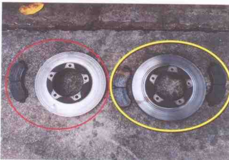
Photo 7 shows both front left (red circle), right (yellow circle) disc brakes and the 3 of 4 brake-pads of the Insured Vehicle. Front left outer brake pad was missing at the time of my inspection.
